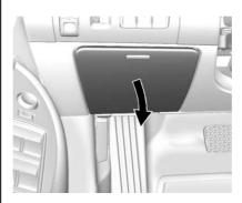
If equipped with storage behind the fuse box cover, push on the cover and release to open.
