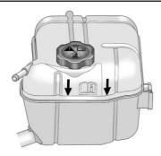
If coolant is visible but the coolant level is not at or above the mark pointed to, add a 50/50 mixture of clean drinkable water and DEX-COOL coolant.
