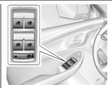
Power windows work when the ignition is on, in ACC/ACCESSORY, or when Retained Accessory Power (RAP) is active. See Retained Accessory Power (RAP) ▷ 155.
