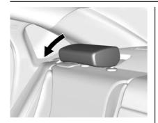
On some models, the rear head restraints can be folded forward to allow for better visibility when the rear seat is unoccupied. To fold the head restraint, grasp the top of the head restraint and pull the head restraint forward and down until it locks in place.
