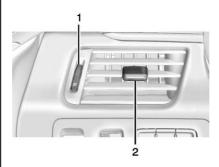
Move the thumbwheels (1) up or down to open or close off the airflow.
