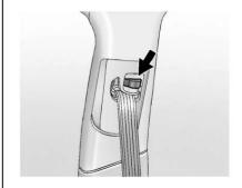
Push down on the release button and move the height adjuster to the desired position. The adjuster can be moved up by pushing the slider/ trim up. After the adjuster is set to the desired position, try to move it down without pushing the release button to make sure it has locked into position.
