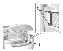
The vehicle may have a convenience net in the trunk. The net (1) attaches to the convenience net hooks (2). Put small loads behind the net. Do not use the net for heavy loads.
