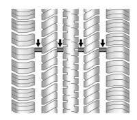
Treadwear indicators are one way to tell when it is time for new tires. Treadwear indicators appear when the tires have only 1.6 mm (1/16 in)
