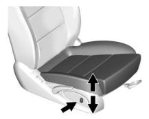
Press and hold the top or bottom of the switch to raise or lower the seat. Release the switch when the desired height is reached.
