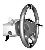
If equipped, press the control to move the steering wheel up and down or forward and rearward.
