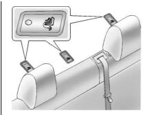
The top tether anchors are under the covers, behind the rear seat, on the filler panel. Be sure to use an anchor located directly behind the seating position where the child restraint will be placed.
