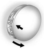
To open the fuel door, push and release the rearward center edge of the door.
