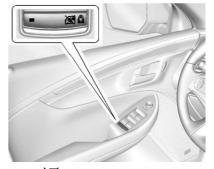
Press to activate the safety locks on the rear doors. The indicator light in the switch will illuminate when activated.
