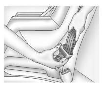
Tilt the latch plate to adjust the belt if needed.
