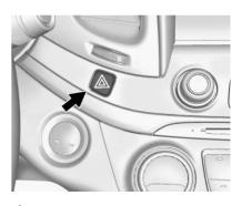
: Press this button to make the front and rear turn signal lamps flash on and off. Press again to turn the flashers off.
