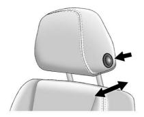
To adjust the head restraint forward or rearward, press the button on the side of the head restraint and move it forward or rearward until the desired locking position is reached. Try to move the head restraint after the button is released to make sure that it is locked in place.
