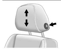
To raise or lower the head restraint, press the button on the side of the head restraint, and pull up or push the head restraint down and release the button. Pull and push on the head restraint after the button is released to make sure that it is locked in place.
