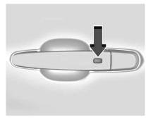
Use the Keyless Access system to lock and unlock the doors. When the doors are locked and the
