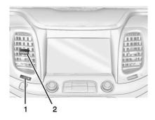
Move the thumbwheels (1) left or right to open or close off the airflow.
