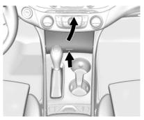
Push the cover down and release to access. To close, push the cover again and release. If equipped, there will be a wireless charger inside. See *Wireless Charging* ♀ 92.
