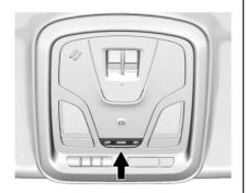
The interior lamps control in the overhead console controls both the front and rear interior lamps.
