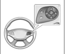
$\triangle$  or  $\nabla$ : Press to move up or down in a list, or on the main view press to cycle through the different Info app pages.
