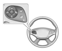
\*\* : Press to turn the system on or off. A white Adaptive Cruise Control indicator comes on.
