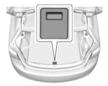
There is storage under the load floor for small items. Pull the load floor handle to access.
