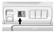
The brightness of the instrument panel lighting and steering wheel controls can be adjusted.
