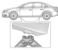
Position the jack lift head at the jack location nearest the flat tire. The location is indicated by a notch on the bottom edge of the body side. The jack must not be used in any other position.
