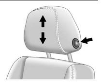
To raise or lower the head restraint, press the button on the side of the head restraint, and pull up or push the head restraint down and release the button. Pull and push on the head restraint after the button is released to make sure it is locked in place.
