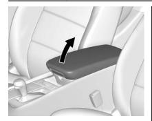
Press the button and lift to access. There is a removable tray on the top of the console. There is an auxiliary input jack, USB port(s), and accessory power outlet inside.
