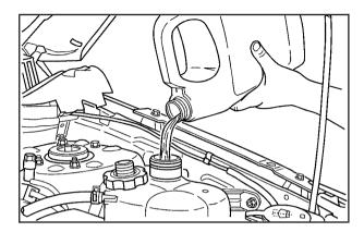
3. Fill the coolant surge tank with the proper DEX-COOL® coolant mixture, to the COLD line.
