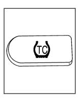
The traction control system can be turned off by pressing the traction control button, located on the instrument panel above the audio system. The traction control system can be activated again by pressing the traction control button.
