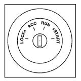
With the key in the ignition switch, you can turn it to four different positions. A warning tone will sound if you open the driver's door when the key has not been removed from the ignition.
