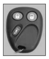
button on the remote keyless entry transmitter one time to lock the doors. The headlamps will flash once. This also arms the content theft-deterrent system.
