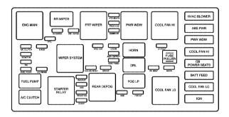
The engine compartment fuse block is located on the driver's side of the engine compartment.
