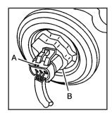
When replacing the low/high-beam bulb, press the clip (A) on the electrical connector and pull it straight off. Turn the bulb retaining ring (B) counterclockwise to remove it and then pull the bulb assembly straight out.
