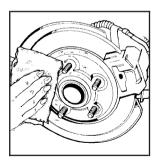
11. Remove any rust or dirt from the wheel bolts. mounting surfaces and spare wheel.
