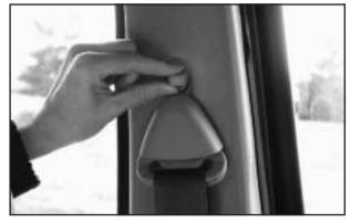
To move it up or down, squeeze the release button and move the height adjuster to the desired position. After you move the adjuster to where you want it, try to move it down without squeezing the release button to make sure it has locked into position.
