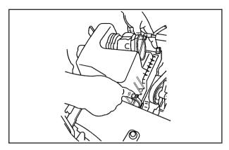
Undo the clamps on the filter cover. To remove the cover, pull up on the front and then pull the cover out.
