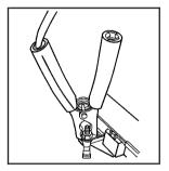
To access the remote positive (+) terminal, remove the fuse block cover.
