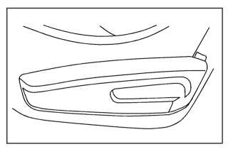
4. Lift the recliner lever located on the outside of the seat cushion and fold the seatback forward until it locks in the folded position. Pull up on the seat to ensure it is locked in place.
