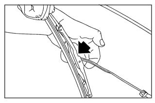
4. Pull up the release clip, located at the connecting point of the blade and the arm. Then, pull the blade assembly down toward the glass to remove it from the wiper arm.
