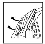
3. The front grill bar is attached to the headlamp lens with a hidden clip. Gently pull the radiator cover/front grill toward you and pull the front grill trim bar away from the headlamp lens.
