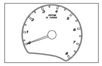
The tachometer shows your engine speed in revolutions per minute (rpm).
