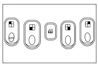
The window switches are located below the shift lever on the center console.
