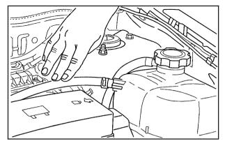
4. With the coolant surge tank pressure cap off, start the engine and let it run until you can feel the upper radiator hose getting hot. Watch out for the engine cooling fans.
