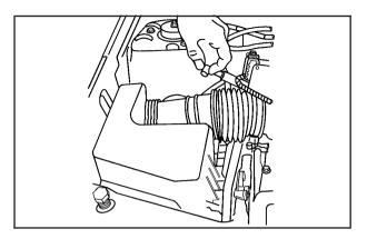
3. Disconnect the crank case ventilation tube.
