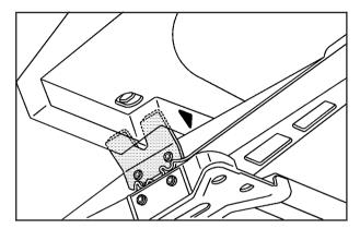
With the jack head positioned correctly on the metal jacking flange, the setup should look like this from underneath.
