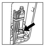
2. Install the jack in the left side panel of cargo area and secure with the wing-bolt.
