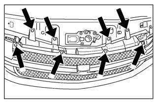
2. Remove the fastener plugs that hold down the radiator cover/front grill.
