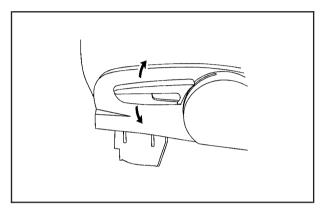
If your vehicle is equipped with a manual driver seat height adjuster, it is located on the outboard side of the seat toward the front of the seat cushion. To raise the seat, ratchet the lever upward until the seat is at the desired height. To lower the seat, ratchet the lever downward until the seat is at the desired height.
