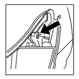
Carefully slide the taillamp housing outward to clear the stud (see arrow) and then rearward and away from the body of the vehicle.
