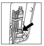
5. Remove the wing-bolt on the jack, and remove the jack.
