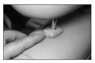
Press the button on the side of the head restraint to adjust it.
