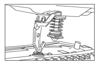
2. Then go to the front of the vehicle and lift up on the secondary hood release lever.
