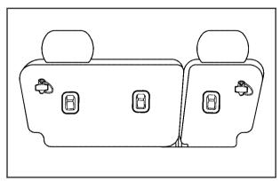
Anchor the top strap to one of the anchor points shown.
