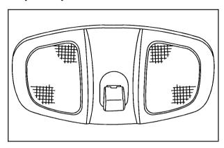
Your vehicle may have lamps located on the headliner above the rearview mirror. Push on the lens in the lamp to turn them on and off.
