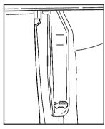
Pull the handle located inside the vehicle.
