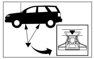
Find the arrow on the plastic lower body panel. Position the jack head under the metal jacking flange and not the plastic lower body panel.
