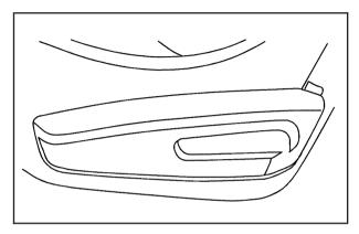
To adjust the seatback, lift the lever on the outboard side of the seat toward the back of the seat cushion and move the seatback to where you want it. Then release the lever to lock the seatback in place.
