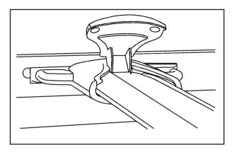
To slide the crossrails pull up on the end levers of the crossrails to slide them to where you want them. This will release the crossrail and allow you to slide it. Once in place, press down on the levers to lock them into place.
