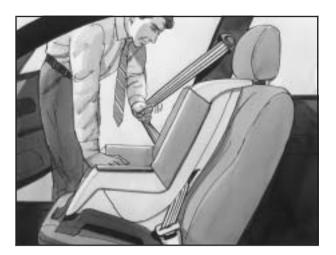
Pull the rest of the shoulder belt all the way out of the retractor to set the lock.
