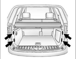
The vehicle may be equipped with four cargo tie-downs located in the rear compartment.
