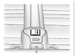
Push the lever down to completely engage into the side rail holes. If the lever is not tight, then the cross rail is not engaged in a side rail hole.
