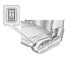
If available, the "1" and "2" buttons on the outboard side of the driver seat are used to manually save and recall the driver seat and outside mirror positions. These manually stored positions are referred to as Button Memory positions.
