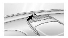
Do not cover the light sensor on top of the instrument panel or the headlamps will come on when they are not needed.
