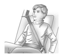
Buckle, position, and release the safety belt as described previously in this section. Make sure the shoulder portion of the belt is on the shoulder and not falling off of it. The belt should be close to, but not contacting, the neck.
