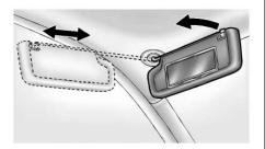
Pull the sun visor down to block glare. Detach the sun visor from the center mount to pivot to the side window, or to extend along the rod, if available.
