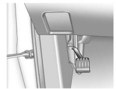
To set the parking brake, hold the regular brake pedal down, then push the parking brake pedal down.
