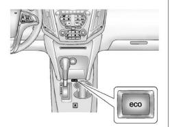
Press the "eco" (economy) button by the shift lever to turn this feature on or off. The "eco" light in the instrument cluster will come on when engaged. See *Fuel Economy Light on page 5-20*. A Driver Information Center (DIC) message "ECO MODE ON" is also displayed. See *Fuel System Messages on page 5-28* for more information.
