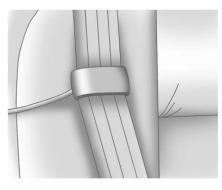
3. The belt should not be twisted and it should lie flat. The elastic cord must be under the belt and the guide on top.
