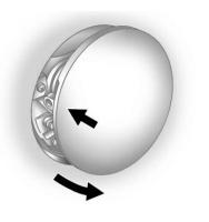
The tethered fuel cap is behind the fuel door on the vehicle's passenger side. To open the fuel door, push the rearward center edge in and release. When applied pressure is removed, the fuel door will spring partially open.
