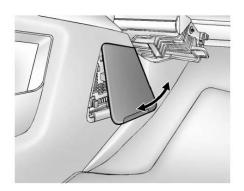
The instrument panel fuse block is located on the passenger side panel of the center console. To access the fuses, open the fuse panel door from the passenger side by pulling it out. To reinstall the door, insert the tabs on the top of the door into the console first, then push the door back into its original location.
