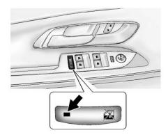
✓ (Window Lockout): This feature prevents the rear passenger windows from operating, except from the driver position. Press at to activate the rear window lockout switch. The indicator light comes on when activated.
