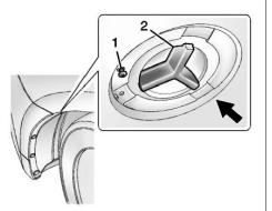
Remove screw (1) and turn access port cap (2) counterclockwise to remove.
