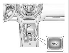
Press the "eco" (economy) button by the shift lever to turn this feature on or off. The "eco" light in the instrument cluster will come on when engaged, and a Driver Information Center (DIC) message "ECO MODE ON" displays. See Fuel Economy Mode on page 9-29.
