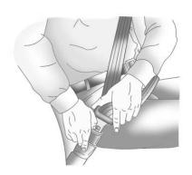
To unlatch the belt, push the button on the buckle.
