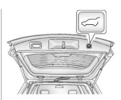
Press and release  $\leftarrow$  on the liftgate adjacent to the latch to close the liftgate.
