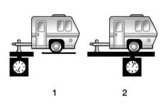
If a weight-carrying hitch or a weight-distributing hitch is being used, the trailer tongue (1) should weigh 10 to 15 percent of the total loaded trailer weight (2).
