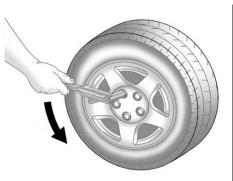
Turn the wheel wrench counterclockwise to loosen all the wheel nuts, but do not remove them yet.
