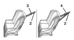
A top tether (3, 4) anchors the top of the child restraint to the vehicle. A top tether anchor is built into the vehicle. The top tether attachment (2) on the child restraint connects to the top tether anchor in the vehicle in order to reduce the forward movement and rotation of the child restraint during driving or in a crash. Your child restraint may have a single tether (3) or a dual tether (4). Either will have a single attachment (2) to secure the top tether to the anchor.
