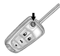
Press this button to extend the key. The key can be used for the ignition and all locks.
