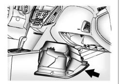
2. Push the stop tab upwards until the stop tab is under the instrument panel assembly and the glove box is released.
