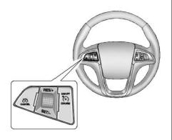
**ON/OFF** O **CRUISE:** Press to turn the cruise control system on and off.
