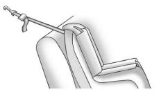
If the position being used does not have a headrest or head restraint and a single tether is being used, route the tether over the seatback.
