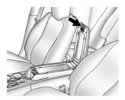
For vehicles with a center console storage, lift the lever on the front to open.
