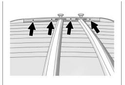
The roof rack cross rails can be locked in four positions along the roof rack side rails. These are the only positions that the cross rails will lock.
