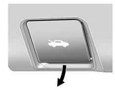
1. Pull the release handle located below the instrument panel to the left of the steering wheel.
