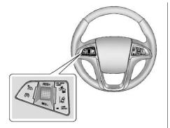
To turn LDW on and off, press the LANE DEPART button on the steering wheel. The control indicator will light when LDW is on.
