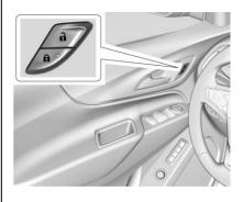
: Press to lock the doors. The indicator light in the switch will come on when the door is locked.
