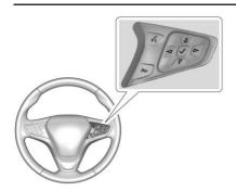
Press  $\triangleleft$  or  $\triangleright$  to select VEHICLE menu, then use  $\triangle$  or  $\nabla$  to scroll through the menu items to select TCS/StabiliTrak.
