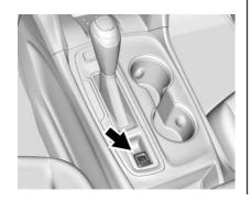
The Electric Parking Brake (EPB) can always be activated, even if the ignition is off. To prevent draining the battery, avoid repeated cycles of the EPB when the engine is not running.
