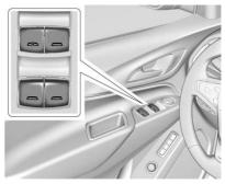
Power windows work when the ignition is on, in ACC/ACCESSORY, or in Retained Accessory Power (RAP). See Retained Accessory Power (RAP) ⇒ 221.
