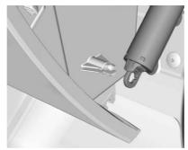
Disconnect the glove box door damper (1) from the glove box door assembly by squeezing the pivot (2) to release the damper ring.
