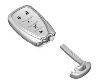
Press the button on the side of the transmitter and pull the key out.
