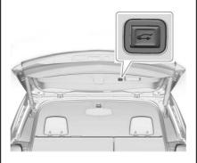
Press on the bottom of the liftgate next to the pull cup to close.
