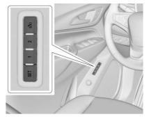
If equipped, memory seats allow two drivers to store and recall their unique seat positions for driving the vehicle, and a shared exit position for getting out of the vehicle. Other feature positions may also be set, such as power mirrors and power steering wheel, if equipped. Memory positions are linked to RKE transmitter 1 or 2 for automatic memory recalls.
