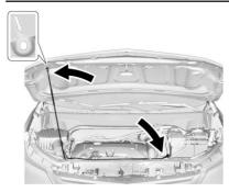
Release the hood prop from its retainer, located above the radiator. Securely place the hood prop into the slot on the underside of the hood. To close the hood:
