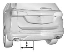
To operate, kick your foot straight up in one swift motion under the rear bumper between the left exhaust pipe and the license plate, then pull it back.
