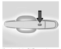
If equipped, the RKE transmitter must be within 1 m (3 ft) of the liftgate or door being opened. Press the button on the door handle to open. See *Remote Keyless Entry* (RKE) System Operation ⇒ 32.
