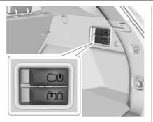
If equipped, the rear seatbacks can also be folded forward by pulling the levers on the passenger side of the rear cargo area.
