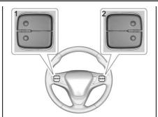
The favorite and volume switches are on the back of the steering wheel.
