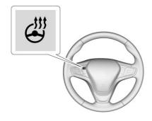
: If equipped with a heated steering wheel, press to turn on or off. A light near the button displays when the feature is turned on.
