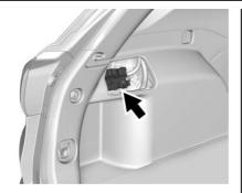
Remove the trim plate to access the fuse block.
