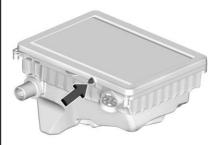
Align the air cleaner/filter with the indicated point on the base of the air cleaner/filter housing
