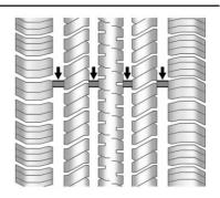
Treadwear indicators are one way to tell when it is time for new tires. Treadwear indicators appear when the tires have only 1.6 mm (1/16 in) or less of tread remaining. See *Tire Inspection* ♀ 333 and *Tire Rotation* ♀ 333.
