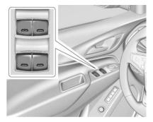
Power windows work when the ignition is on, in ACC/ACCESSORY, or when Retained Accessory Power (RAP) is active. See Retained Accessory Power (RAP) ⇒ 221.
