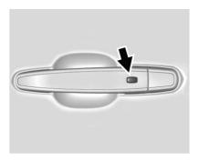
Press the button on the driver door handle when the RKE transmitter is within 1 m (3 ft) of the driver door handle. When unlocking from the driver door, the first press unlocks that door; press again within five seconds to unlock all passenger doors. See Remote Keyless Entry (RKE) System Operation ⇒ 32.
