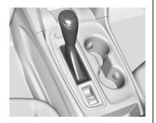
**P**: This position locks the front wheels. Use P (Park) when starting the engine because the vehicle cannot move easily.
