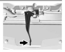
Go to the front of the vehicle to find the secondary hood release handle. The handle is under the front edge of the hood near the center. Push the handle to the right and raise the hood.
