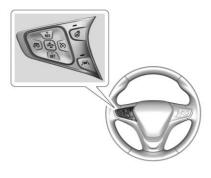
ৈ: Press to turn the cruise control system on and off. A white indicator comes on in the instrument cluster when cruise is turned on.
