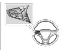
: Press to turn the cruise control system on and off. A white indicator comes on in the instrument cluster when cruise is turned on.
