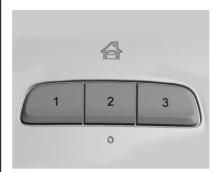
If equipped, the Universal Remote System allows for garage door openers, security systems, and home automation devices to be programmed to work with these buttons in the vehicle.
