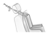
If the position you are using has an adjustable headrest or head restraint and you are using a dual tether, raise the headrest or head restraint and route the tether under the headrest or head restraint and in between the headrest or head restraint posts.
