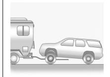
To tow the vehicle from the front with the rear wheels on the ground:
