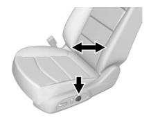
If equipped, press and hold the front or rear of the control to increase or decrease lumbar support.
