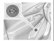
To operate the power liftgate, the vehicle must be in P (Park). The taillamps flash when the power liftgate moves.
