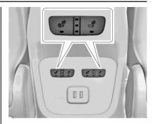
If equipped, the rear heated seat buttons are on the rear of the center console.
