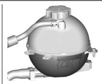
Check to see if coolant is visible in the coolant surge tank. If the coolant inside the coolant surge tank is boiling, do not do anything else until it cools down. If coolant is visible but the coolant level mark is not visible, add a 50/50 mixture of clean, drinkable water and DEX-COOL coolant at the coolant surge tank to the top rib on the middle of the tank, but be sure the cooling system is cool before this is done. See *Engine Overheating*
