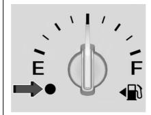
For the base level cluster, this light comes on when the fuel tank is low on fuel. The light turns off when fuel is added. If it does not, have the vehicle serviced.
