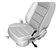
Move the lever up or down to raise or lower the seat.
