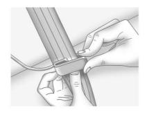
Place the guide over the belt, and insert the two edges of the belt into the slots of the guide.
