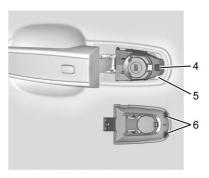
Insert the two tabs (6) at the back of the cap between the seal (5) and the metal base (4).
