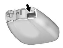
Separate the two halves of the transmitter using a flat tool inserted into the area near the key slot.
