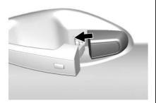
Slide the cap forward and press the forward edge to install the cap in place.
