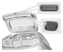
To open the liftgate from the outside, press and on the RKE transmitter to unlock all doors, then use the center touch pad.
