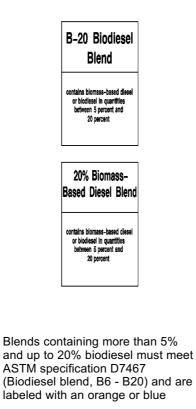
pump label. To reduce the risk of poor quality fuel, purchase biodiesel blends from a fuel supplier or fueling station that sells BQ-9000<sup>®</sup> certified biodiesel. See www.bq-9000.org for a list of certified marketers. For detailed information on the use of biodiesel, see *Biodiesel*  $\Leftrightarrow$  253.
