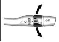
**INT**: Move the lever up to INT for intermittent wipes, then adjust the band to control the frequency of wipes.
