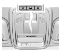
$\stackrel{}{\ll}$ : Press to turn the lamps off, even when a door is open.
