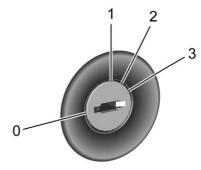
The ignition switch has four different positions.
