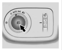
If equipped with front fog lamps, the button is on the exterior lamp control, on the outboard side of the steering wheel. To turn on the fog lamps, the ignition must be on and the exterior lamp control must be in  $300^{\circ}$  or  $30^{\circ}$ .
