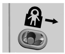
The safety lock is on the inside edge of the rear doors. To use the safety lock:
