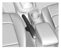
With the brake pedal applied, pull up firmly on the parking brake handle without pressing the release button. See *Shifting Into Park*  $\Rightarrow$  219 or *Parking*  $\Rightarrow$  221. If the ignition is in the ON/RUN position, the brake system warning light will come on. See *Brake System Warning Light*  $\Rightarrow$  128.
