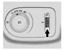
This feature controls the brightness of the instrument panel controls and the infotainment display. The thumbwheel is next to the exterior lamp control.
