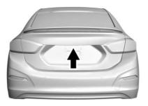
To open the trunk from outside the vehicle, press 25 twice on the Remote Keyless Entry (RKE)
