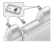
The top tether anchors are under the covers on the rear seatback filler panel. Be sure to use an anchor located on the same side of the vehicle as the seating position where the child restraint will be placed.
