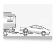
To tow the vehicle with the two rear wheels on the ground and the front wheels on a dolly:
