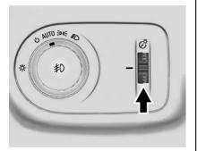
This feature controls the brightness of the instrument panel controls and the infotainment display. The thumbwheel is to the left of the steering column on the instrument panel.
