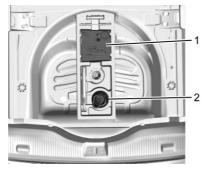
2. Remove the compressor (1) and the tire sealant canister (2).
