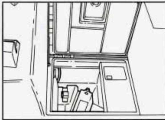
The jack, wheel nut socket and wheel lock key are in the rear storage compartment behind the passenger's seat. Open the compartment door and remove the plastic tray. Lift the jack, wheel nut socket and wheel lock key out of the foam container. You should have a jack, wheel wrench, socket and a wheel lock key.
