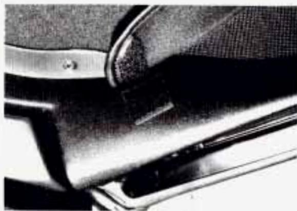
7. Fasten the strips for the headliner at the rear of each window opening.
