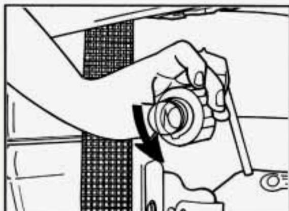
2. Push the bulb in, turn it counterclockwise, then pull it out.
