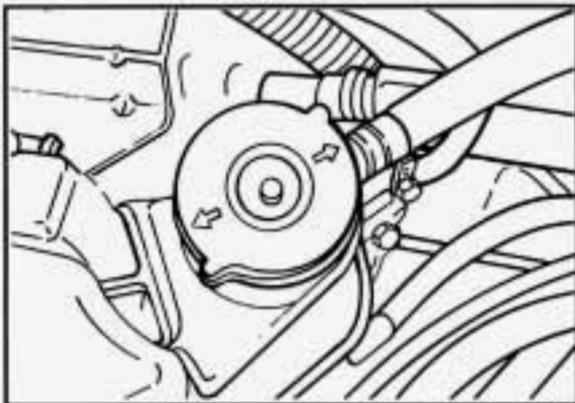
9. Shut the engine off and replace the pressure cap. Be sure the arrows on the pressure cap line up like this.
