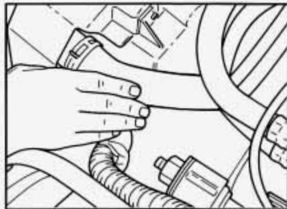
6. Start the engine and let it run until you can feel the upper radiator hose getting hot. Watch out for the engine fans.
