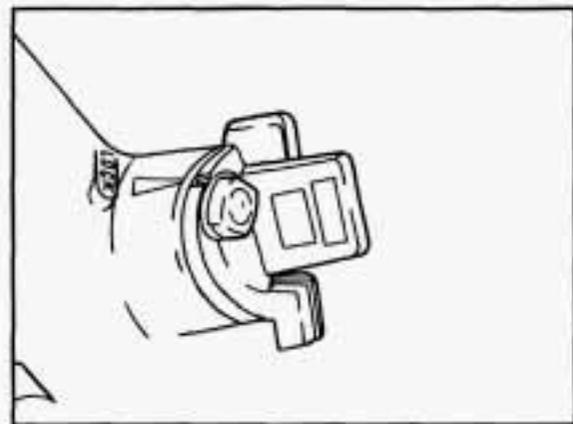
**Key Release Button:** If you have a manual transmission, your ignition lock has a key release button. You must press the button before you can take your key out of the ignition lock.
