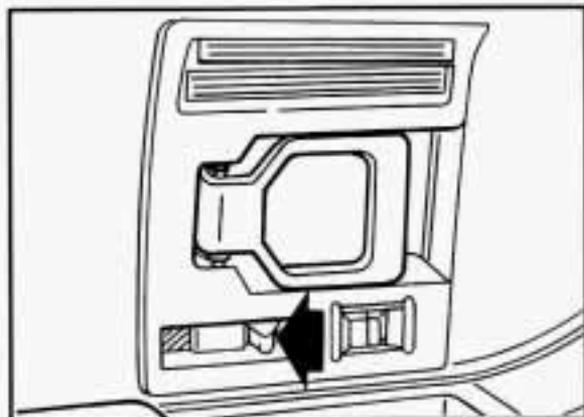
To lock the door from the inside, move the lock control on the door back. To unlock it, move the lock control on the door forward.
