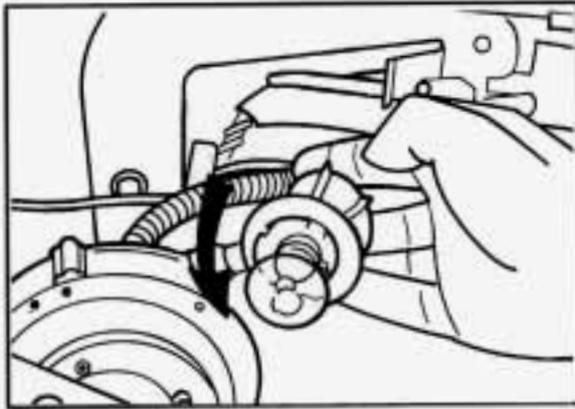
4. Push the bulb in, turn it counterclockwise, then pull it out.
