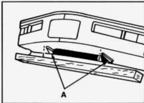
Position 4x4 wood beam across sling chains contacting under fascia just ahead of curb protect brackets (A).
