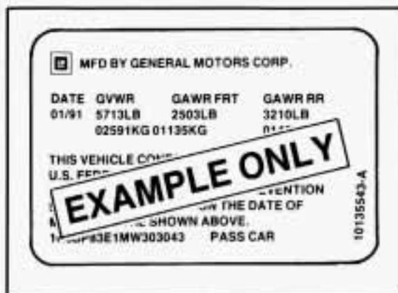
The other label is the Certification label, found on the rear edge of the driver's door. It tells you the gross weight capacity of your vehicle, called the GVWR (Gross Vehicle Weight Rating). The GVWR includes the weight of the vehicle, all occupants, fuel and cargo. Never exceed the GVWR for your vehicle, or the Gross Axle Weight Rating (GAWR) for either the front or rear axle.
