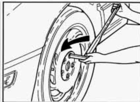
Remove the plastic wheel nut caps using the socket end of the wheel wrench. Store the caps somewhere until you have the flat tire repaired or replaced.
