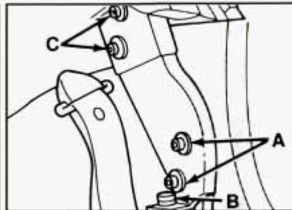
7. Insert the two upper bolts (C) into both receiver brackets. You may have to lift the hardtop slightly to install the lock pillar bracket.
