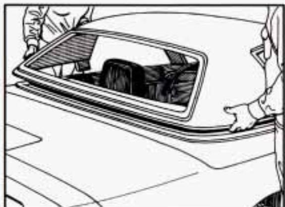
10. With one person on each side, gently lift the hardtop about eight inches (200 mm) straight up. Remove the hardtop over the rear of the vehicle.
