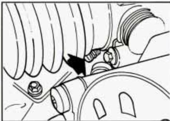
3. After the engine cools, open the air bleed valves on the throttle body. . .
