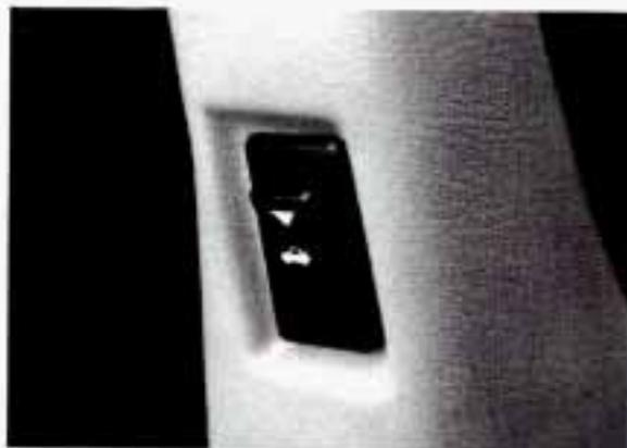
If you have a coupe, this switch is on the rear of the driver's door. It works with the door open and the transmission in any gear. Push it down to release the hatch.
