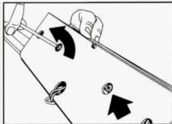
4. Remove the two screws on the underside of the assembly.
