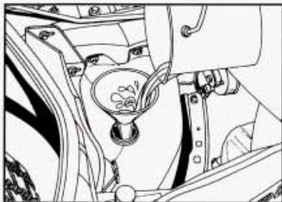
If you need to add more coolant, add the proper mix at the coolant recovery tank, but only when your engine is cool. If the tank is very low or empty, also add coolant to the coolant high fill reservoir. See "Engine Overheating" in the Index for information.
