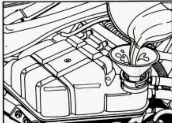
3. Fill the coolant high fill reservoir with the proper mix, up to the base of the filler neck.
