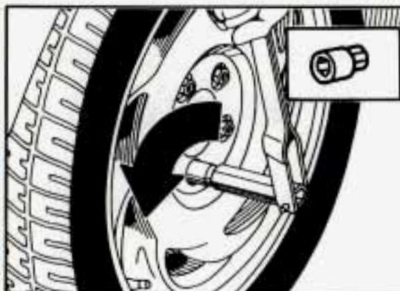
Attach the wheel nut socket to the wheel wrench and loosen all the wheel nuts. Don't remove them yet.
