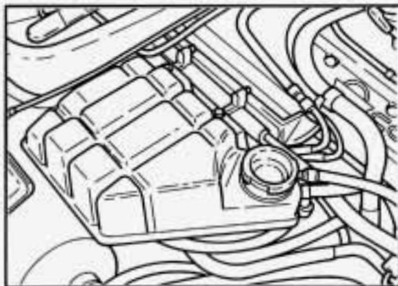
5. Put the cap back on the coolant recovery tank, but leave the coolant high fill reservoir pressure cap off.
