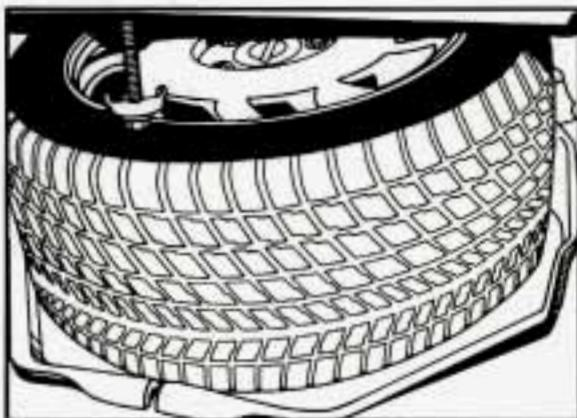
Put the flat road tire on the tray. Lift the latch bolt, push it toward the front of the vehicle, and the bolt will drop down to the lower position.
