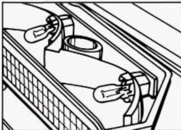
6. Rock the bulb back and forth while pulling up to remove it.
