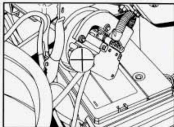
6. Positive (+) goes to positive (+) and negative (-) goes to negative (-) or a metal engine part. Connect the red positive (+) cable to the positive (+) terminal of the vehicle with the dead battery. Use a remote positive (+) terminal if the vehicle has one.
