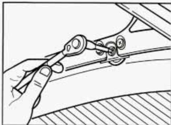
4. The two rear bolts are on the roof, one above each seat. You'll see three bolts on each side. Loosen the middle one. (The ratchet won't work for the other two.) The bolts will stay in the roof panel.
