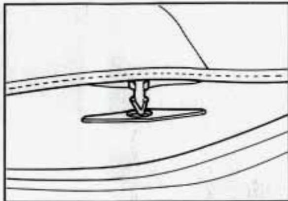
6. Lower the rear of the top so the latch pins align with the holes in the lid. To secure the rear of the top, push down firmly on both corners.
