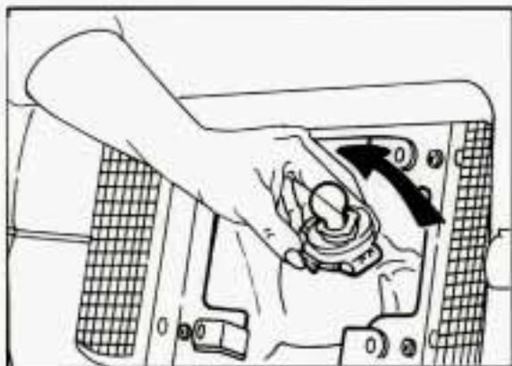
2. Push the bulb in, turn it counterclockwise, then pull it out.
