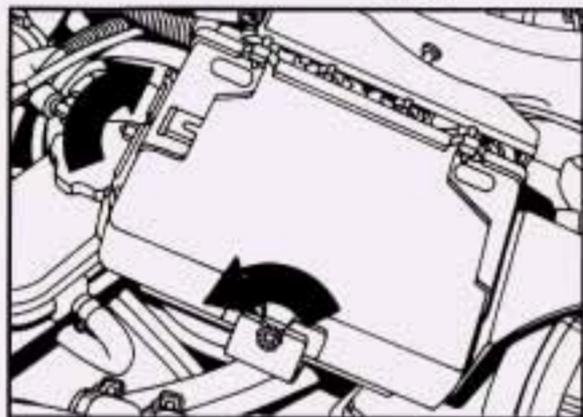
Remove the nut on the outboard side of the unit. Then loosen the front and inboard nuts. For the LT5 engine, loosen the two inboard nuts. Move the ECM unit to either side.
