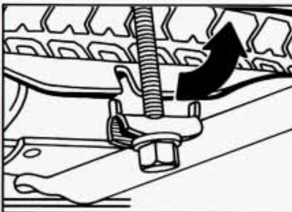
While holding the tray up with the wheel wrench, pull the latch bolt to release it from the tray. If it won't come free, loosen it a little more.
