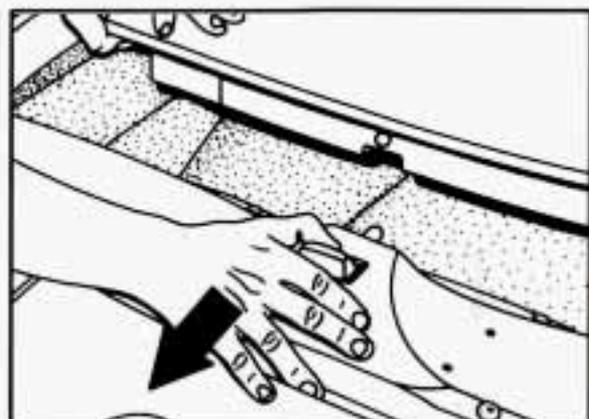
2. Store the roof panel with its top up and its rear pointing forward. Slide the rear corners of the roof panel into the brackets and push forward.
