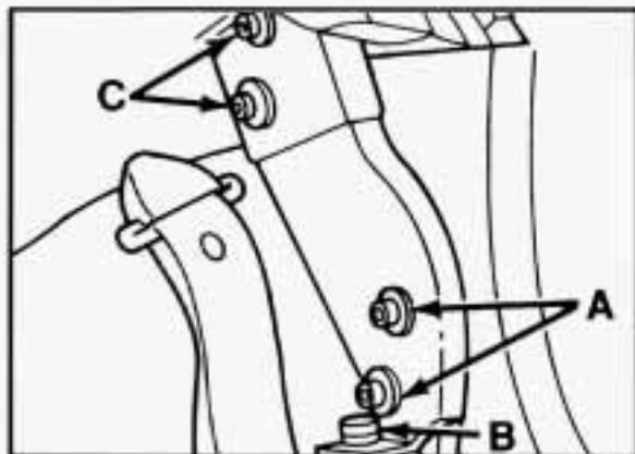
5. Using the wrench, remove the two lower bolts (A) from the lock pillar bracket on each side.
