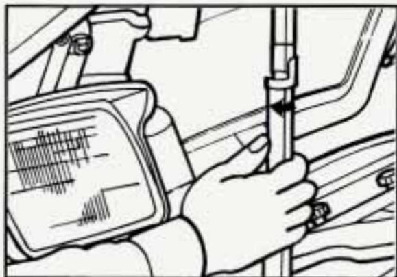
Then release the hood strut by moving it to the centered position and lowering the hood. Lower the hood until it is about 12 inches (300 mm) above the engine, then release it.
