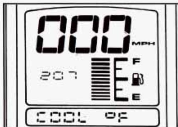
For numeric gauge measurements, press the "GAUGES" button on the Trip Monitor until "COOL" appears. The number that appears next to the fuel gauge is the coolant temperature. If "LO" appears, the temperature is below 32°F (0°C).
