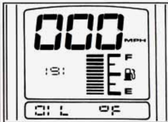
For numeric gauge measurements, press the "GAUGES" button on the Trip Monitor until "OIL" appears. The number that appears next to the fuel gauge is the oil temperature. If "LO" appears, the temperature is below 32°F (0°C).
