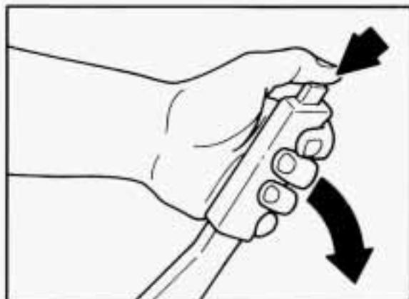
**To release the parking brake:** Hold the brake pedal down. Pull the parking brake lever up until you can push in the release button. Hold the release button in as you move the lever all the way down.
