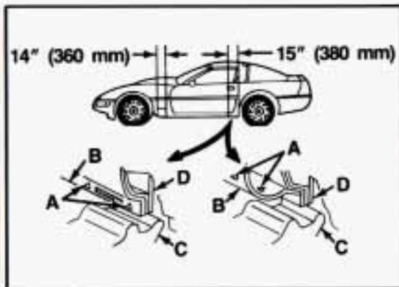
Position the jack under the vehicle. There are two locator triangles (A) on the panels (B) near each wheel. Raise the lift head (C) until it fits firmly under the steel rocker flange (D) between the triangles nearest the flat tire.
