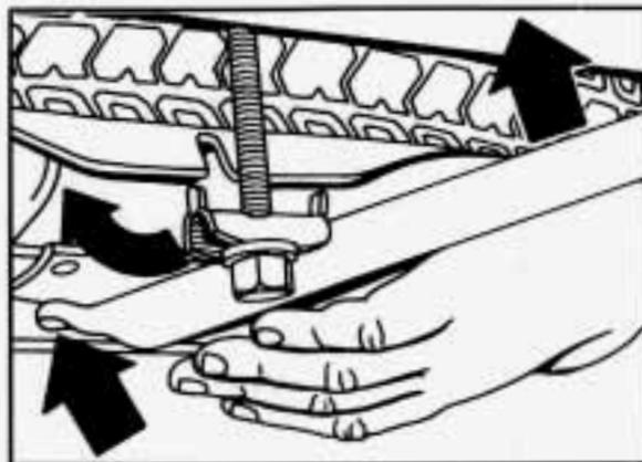
Put the hooked end of the wheel wrench into the slot in the tray. Lift the tray using the wheel wrench and insert the latch bolt into the notch in the tray. To raise the tray, use the socket end of the wheel wrench to turn the latch bolt clockwise. Turn the latch bolt until it is snug.
