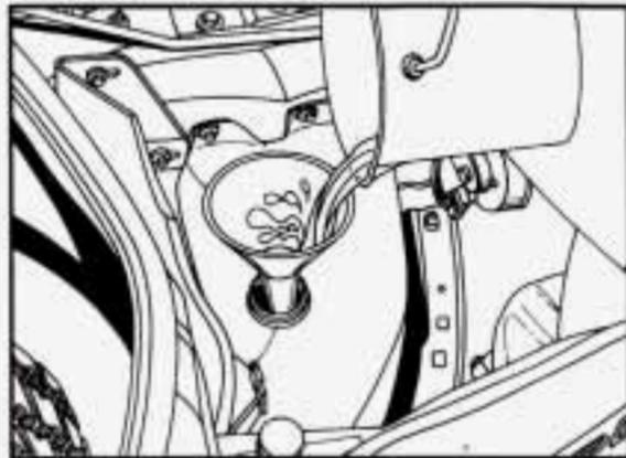
10. Then fill the coolant recovery tank to the proper level.
