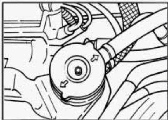
8. Shut the engine off and replace the pressure cap. At any time during this procedure if coolant begins to flow out of the filler neck, reinstall the pressure cap. Be sure the arrows on the cap line up like this.
