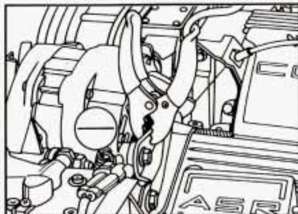
9. The other end of the negative cable doesn't go to the dead battery. It goes to a heavy, unpainted metal part on the engine of the vehicle with the dead battery. Attach the cable at least 18 inches (45 cm) away from the dead battery, but not near engine parts that move. The electrical connection is just as good there, but the chance of sparks getting back to the battery is much less.
