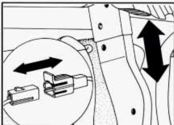
8. Slide both lock pillar brackets down and forward from the receiver brackets. You may need to lift the hardtop slightly to remove the brackets.
