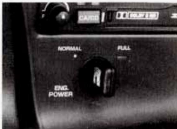
To change the power setting, put your engine power key into the switch. Turn the key to the setting you want and let go. The key will return to the center position.
