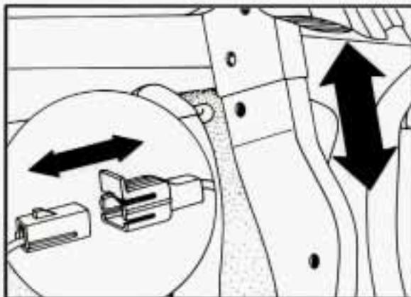
5. Move both seatbacks forward. Slide the lock pillar bracket into the receiver bracket until the scribed line is even with the lower edge of the receiver bracket.
