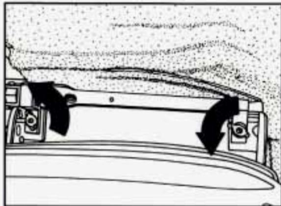
The equipment you'll need is behind the driver's seat and in the rear storage compartment behind the passenger's seat. Move the driver's seat all the way forward and fold the seatback forward. The wheel wrench is on the floor behind the seat. Loosen the wingnuts and slide the wheel wrench out of the clamps.
