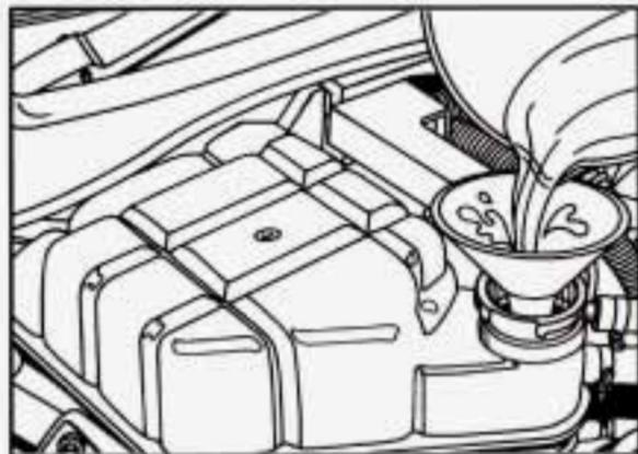
4. Fill with the proper mix. Add coolant until you see a steady stream of coolant coming from the bleed valves.
