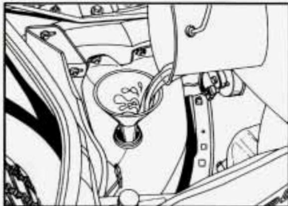
4. Then fill the coolant recovery tank to the "HOT" mark on the dipstick.
