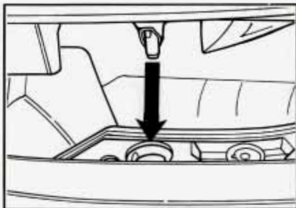
3. Turn the latch handles outward. Pull the top up and forward until it lines up with the windshield.
