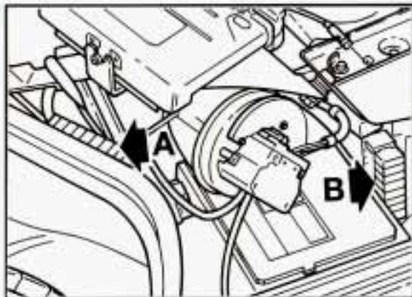
The other two fuse blocks are in the engine compartment. One is part of the Forward Lamp wiring harness (A), and the other is part of the ECM-Engine wiring harness (B).
