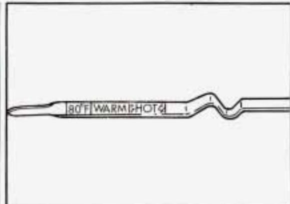
3. Check both sides of the dipstick, and read the lower level. The fluid level must be in the cold area for a cold check or in the "HOT" area or cross-hatched area for a hot check.
