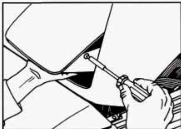
4. Remove the two screws from both sides of the cover. Before you remove the last screw, put your hand under the cover to hold it.
