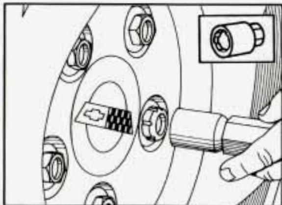
Each wheel will have one locknut. A special wheel lock key (removal tool) and instructions are provided. Attach the wheel lock key to the wheel wrench. Remove the locking wheel nut by turning counterclockwise.
