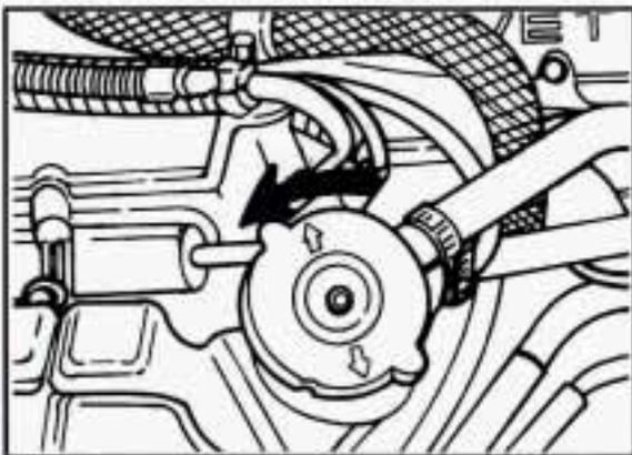
**How to Add Coolant to the Coolant High Fill Reservoir (5.7L LT5 (Code J) Engine)**
