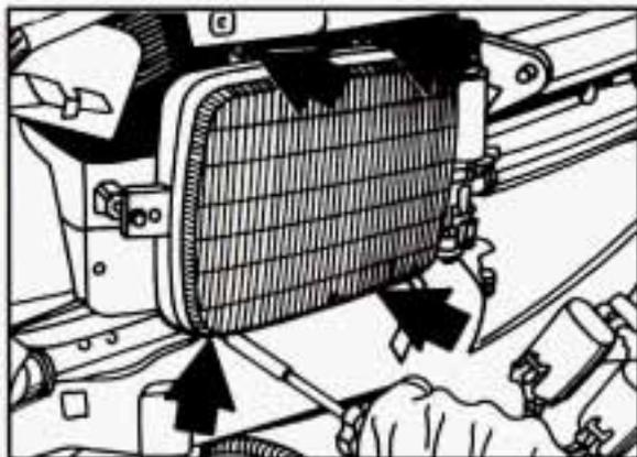
6. Remove the four screws from the retainer near each corner of the headlight. Don't move the large-head adjusting screws or your headlight will not be aimed properly.
