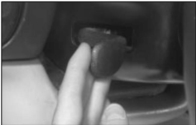
A tilt wheel allows you to adjust the steering wheel.
