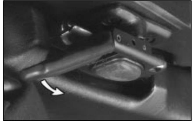
2. Unlock the front of the convertible top by lowering the latch handles and turning them inward. Push the latch handles back to the up position.
