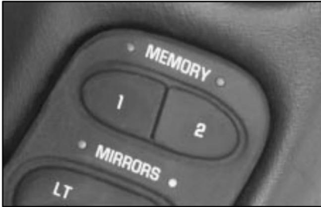
MEMORY can store and recall the settings for the driver's seat position, the outside rearview mirror positions, comfort control temperature, fan speed and mode settings, telescopic steering wheel (if equipped), radio presets, tone, volume, playback mode (AM/FM, tape or CD), last displayed station, compact disc position and tape direction.
