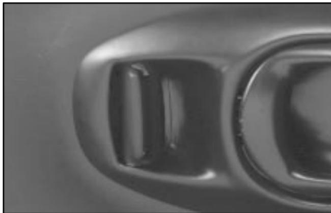
To lock the door from the inside, move the lock control on the door forward. To unlock it, move the lock control on the door backward.
