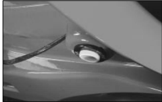
4. Tilt the driver's seatback forward and press the storage compartment release button located on the underside of the storage compartment lid (C) behind the driver's seat. Then raise the storage compartment lid (C). While attempting to raise the lid, if the lid does not release and you hear three chimes, check to make sure the trunk lid is closed. Also, the lid will not release if the alarm is turned on or the trunk lid is open.
