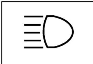
To change the headlamps from low beam to high or high to low, push the turn signal lever all the way forward.
