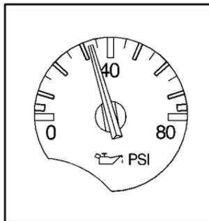
The engine oil pressure gage shows the engine oil pressure in psi (pounds per square inch) or kPa (kilopascals) when the engine is running.
