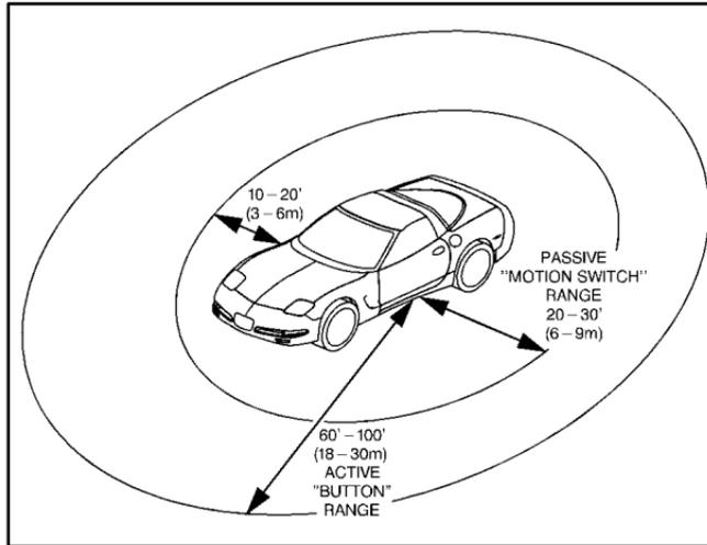
The active range (using one of the four buttons) of the key fob transmitter is approximately 60 to 100 feet (18 to 30 m). The passive range (having the slider switch set to ON) is approximately 10 to 20 feet (3 to 6 m) on the passenger's side of the vehicle and 20 to 30 feet (6 to 9 m) on the driver's side.
