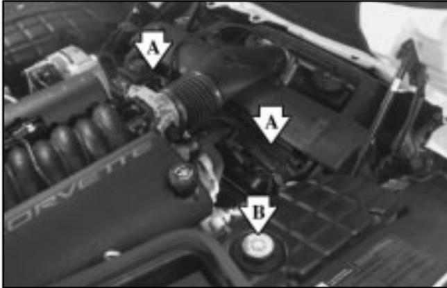
A. Electric Engine Cooling Fans
