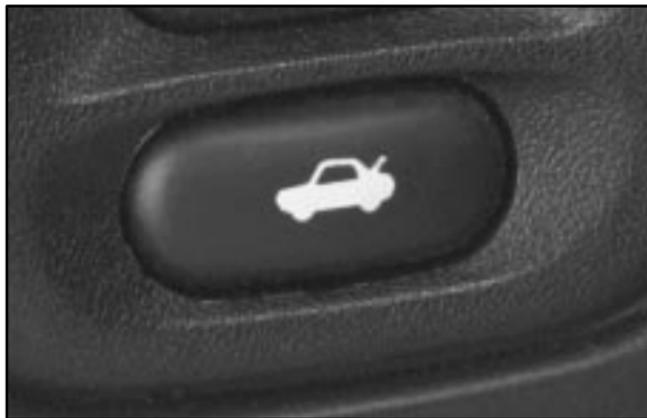
To use the remote hatch/trunk lid release on automatic transmission vehicles, your vehicle must be in PARK (P) or NEUTRAL (N). For manual transmissions, set the parking brake. See "Parking Brake" in the Index.
