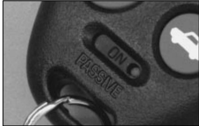
You can turn on the passive feature by moving the transmitter's slider switch to ON. Now, when you move toward your vehicle with the key fob transmitter, the system will automatically disarm your theft-deterrent system and unlock the driver's door or both depending on how the system is programmed. If it's dark enough outside, your interior lamps will come on.
