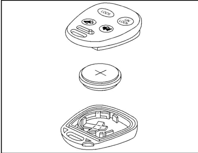
1. Insert a coin into the slot on the back of the transmitter and gently pry apart the front and back.
