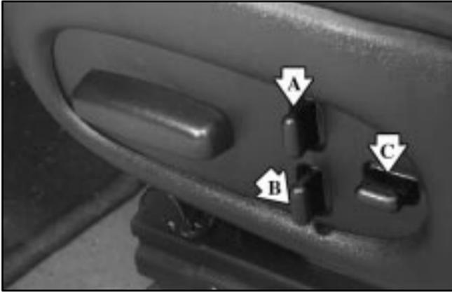
In addition to the power seat control, there are three other switches that help you change the shape of the seat. There are two lumbar supports for the middle (A) and lower (B) back. There's also a side bolster switch (C) that adjusts the sides of the seat around you to give you more lateral support.
