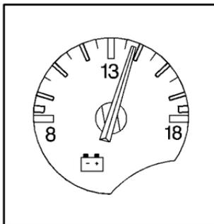
When the key is in ON with the engine not running, the voltmeter shows the voltage output of your battery.
