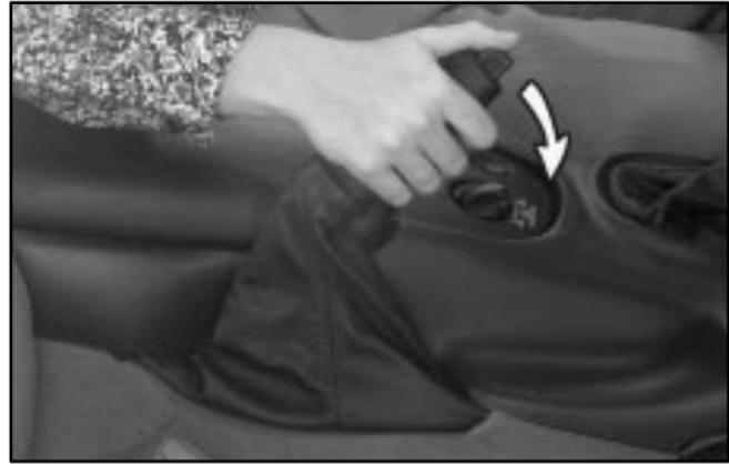
To release the parking brake, hold the brake pedal down. Hold the release button in as you move the parking brake lever all the way down.
