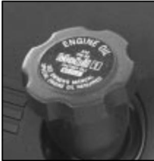
The engine oil fill cap is on top of the passenger's side valve cover.
