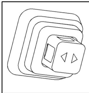
The switch to operate the telescopic steering wheel is located on the right-hand side of the steering column.
