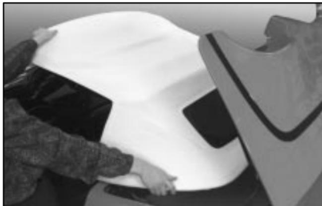
5. Push forward on the front edge (A) of the convertible top to allow the rear edge (B) of the convertible top to be rotated to its full-down position.
