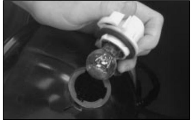
4. Remove the bulb from the socket.
