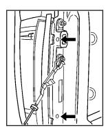
Remove the two rear lamp assembly screws near the tailgate latch.
