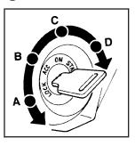
With the key in the ignition switch, you can turn to four different positions.
