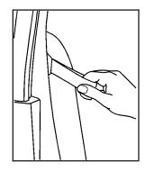
Pull the loop, located on the outboard side of the seatback, forward until you hear a click.
