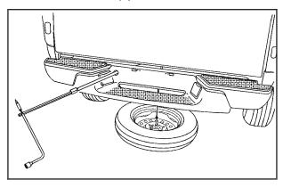
Insert the hoist end (chiseled end) of the extension tool (C) through the hole in the rear bumper and into the funnel-shaped guide. The chiseled end of the extension is used to lower the spare tire. Turn the wheel wrench (D) counterclockwise to lower the spare tire to the ground. Continue to turn the wheel wrench until the spare tire can be pulled out from under the vehicle.
