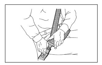
To unlatch the belt, just push the button on the buckle. The belt should go back out of the way. When the safety belt is not in use, slide the latch plate up the safety belt webbing. The latch plate should rest on the stitching on the safety belt, near the guide loop on the side wall.
