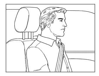
Adjust the head restraint so that the top of the restraint is closest to the top of your head. This position reduces the chance of a neck injury in a crash.
