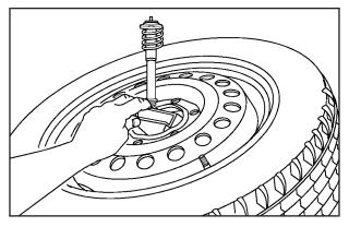
Tilt the retainer downward and through the wheel opening. Make sure the retainer is fully seated across the underside of the wheel.
