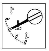
This gage shows the engine coolant temperature.
