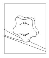
If your vehicle has this feature, there is a knob located on the outboard side of the driver's seat.
