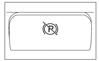
To release the parking brake, hold the regular brake pedal down. Pull the bottom edge of the lever, located above the parking brake pedal, with the parking brake symbol, directly rearward to release the parking brake.
