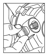
9. Put the wheel nuts back on with the rounded end of the nuts toward the wheel. Tighten each wheel nut by hand. Then use the wheel wrench to tighten the nuts until the wheel is held against the hub.
