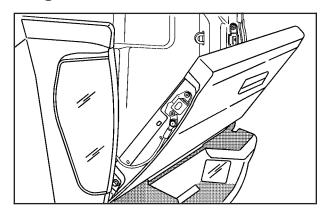
You can open the tailgate by pulling up on the outside handle while pulling the tailgate down.
