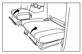
To access the storage compartments you will need to lift the cushion on the bottom of the rear seats. This will expose the storage boxes under the seat.
