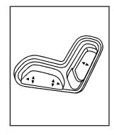
If your vehicle has power reclining seatbacks, use the vertical power seat control located on the outboard side of the seat.
