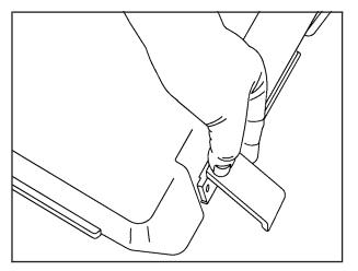
To open a storage box, unhook the bottom and lift the two latches on each side of the storage box.
