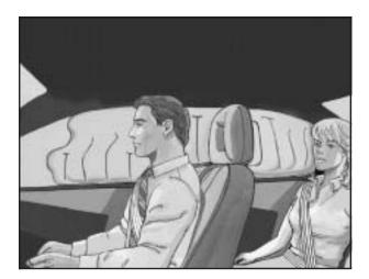
If your vehicle has a roof-mounted side impact airbag for the right front passenger and the person seated directly behind that passenger, it is located in the ceiling above the side windows.
