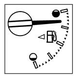
When the ignition is on, the fuel gage tells you about how much fuel you have remaining in the fuel tank. Here are four things that some owners ask about. None of these indicate a problem with your fuel gage:
