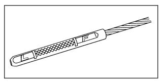
If the oil is below the cross-hatched area (L), you will need to add at least one quart/liter of oil. But you must use the right kind. This section explains what kind of oil to use. For engine oil crankcase capacity, see Capacities and Specifications on page 5-104.
