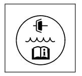
The hydraulic clutch fluid reservoir cap has this symbol on it. See *Engine Compartment Overview on page 5-12* for reservoir location.
