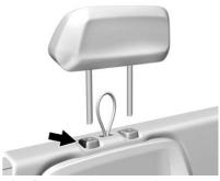
2. Press the button on the passenger side headrest and pull up.
