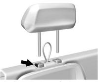
Press the button for the passenger side headrest at the top of the seatback and pull up.
