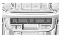
Turn the Tow/Haul Mode on and off by pressing the button on the center stack. When the Tow/Haul Mode is enabled, a light on the instrument cluster will come on. Also see "Tow/Haul Mode" under *Towing Equipment* ⇒ 212.
