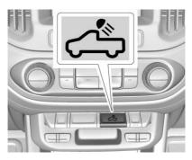
The cargo lamp provides more light in the cargo area of the vehicle, if needed. The lamps inside the pickup box also turn on, if equipped.
