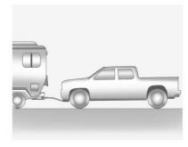
Only dinghy tow four-wheel-drive vehicles that have an N (Neutral) and a Four-Wheel Drive Low (4 (1) setting.
