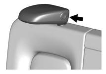
The rear outboard head restraints are designed to be folded. When folding the seatback down, the head restraint must first be manually folded forward out of the way to fold the seatback down
