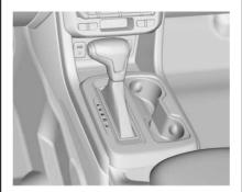
**P**: This position locks the drive wheels. Use P (Park) when starting the engine because the vehicle cannot move easily. When parked on a hill, especially when the vehicle has a heavy load, you might notice an increase in the effort to
