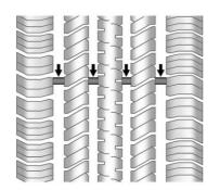
Treadwear indicators are one way to tell when it is time for new tires. Treadwear indicators appear when the tires have only 1.6 mm (1/16 in) or less of tread remaining. Some commercial truck tires may not have treadwear indicators. See *Tire Inspection* ♀ 275 and *Tire Rotation* ♀ 275 for additional information.
