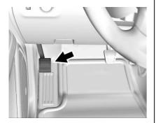
Set the parking brake by holding the regular brake pedal down, then pushing down the parking brake pedal.
