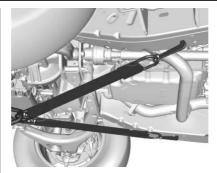
The vehicle is equipped with specific attachment points to be used to pull the vehicle onto a flatbed car carrier from a flat road surface. Do not use these attachment points to pull the vehicle from snow, mud or sand.
