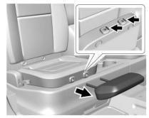
If installed as a seat cushion extension, first press both buttons on the front of the seat cushion to remove the headrest.
