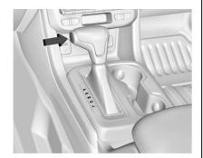
Range Selection Mode helps control the vehicle's transmission and vehicle speed while driving downhill or towing a trailer by letting you select a desired range of gears.
