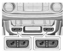
If equipped, the buttons are on the center stack. To operate, the engine must be running.
