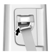
Push up on the release button and move the height adjuster to the desired position.
