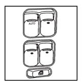
For vehicles with power windows, the switches on the driver door armrest control each window. The switch on each passenger door controls only that doors window.
