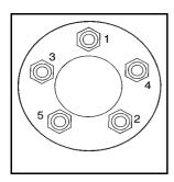
15. Tighten the wheel nuts firmly in a crisscross sequence, as shown.
