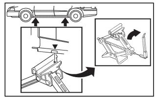
Position the jack lift head at the rear jack location nearest the rear tire. The rear location is about 4 inches (10 cm) in front of the rear wheel opening.
