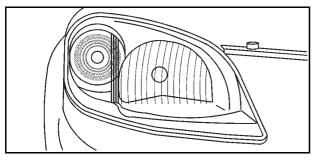
2. Record the distance from the ground to the aim dot on the low-beam headlamp.
