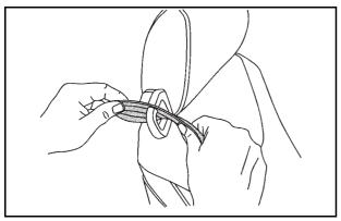
If the seat has a safety belt guide, and the safety belt is not routed through the guide, slide the edge of the belt webbing through the opening on the guide. Be sure the belt is not twisted.
