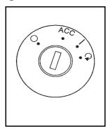
The ignition switch has four different positions.
