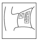
The cruise control buttons are located on the left side of the steering wheel.
