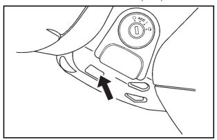
Remove the cover from the bottom of the steering column.
