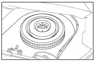
Lift the trunk liner to access the spare tire and tools.
