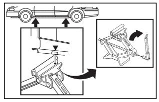
Position the jack lift head at the jack location nearest the flat tire. The front location is about 8 inches (20 cm) behind the front wheel opening. The rear location is about 4 inches (10 cm) in front of the rear wheel opening.
