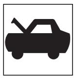
Pull the interior hood release lever with this symbol on it. It is located under the instrument panel on the driver's side of the vehicle.
