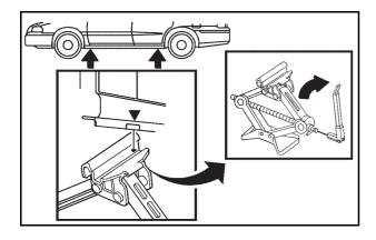
Position the jack lift head at the jack location nearest the flat tire. The front location is about 8 inches (20 cm) behind the front wheel opening.
