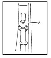
Press the release button (A) and move the height adjuster to the desired position. The adjuster can be moved up by pushing up on the shoulder belt guide.
