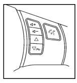
If equipped, some audio controls can be adjusted using the controls on the right side of the steering wheel.
