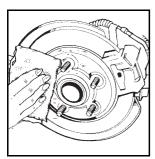
Remove any rust or dirt from the wheel bolts, mounting surfaces, and spare wheel. 11. Place the compact spare tire on the wheel-mounting surface.
