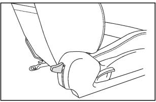
Push down the easy entry seat handle located on the rear of the seatback on the outboard side to release the seatback.
