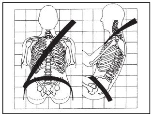
Sit up straight and always keep your feet on the floor in front of you. The lap part of the belt should be worn low and snug on the hips, just touching the thighs. In a
