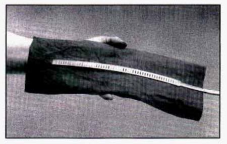
When it is cool, remove the coolant recovery tank cap and look at the dipstick.
