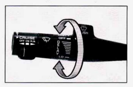
You can control the windshield wipers by turning the band with the wiper symbol on it.
