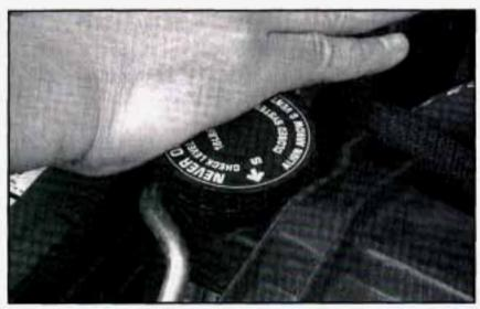
Then keep turning the pressure cap, but now push down as you turn it. Remove the pressure cap.
