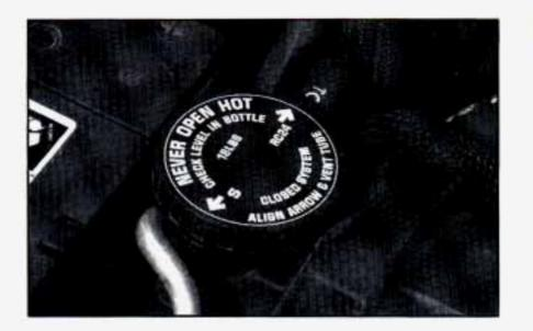
Then replace the pressure cap. At any time during this procedure if coolant begins to flow out of the filler neck, reinstall the pressure cap. Be sure the arrows on the pressure cap line up like this.
