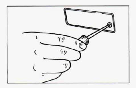
Replacing a rear sidemarker bulb:
