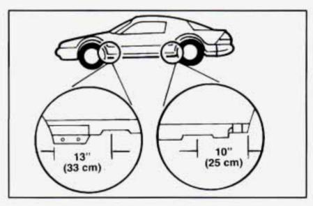
Position the jack under the vehicle. There is a notch in the vehicle's rocker flange. Raise the jack head until it fits firmly into the notch nearest the flat tire.
