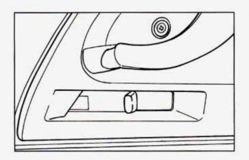
From the inside, to lock the door, move the lock control on the door backward.
