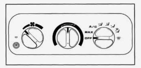
The air conditioning system uses the same controls as the heating system, except that the air control knob has two extra settings, described below.
