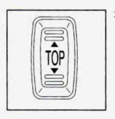
Make sure there is nothing or anyone on or around the top. Push and hold down or the down arrow ▼ on the convertible top switch.
