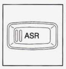
To turn the system off, press the ASR switch on the instrument panel.
