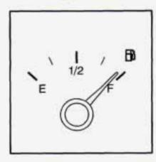
Your fuel gage shows about how much fuel is in your tank. The fuel gage works only when the ignition is in the RUN. When the gage pointer first indicates empty (E) you still have a little fuel left (about one to two gallons) (3.8 to 7.6 litres), but you need to get more fuel right away.
