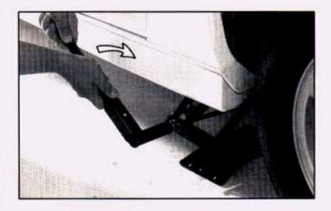
3. Raise the vehicle by rotating the wheel wrench to the right. Raise the vehicle far enough off the ground so there is enough room for the spare tire to fit.
