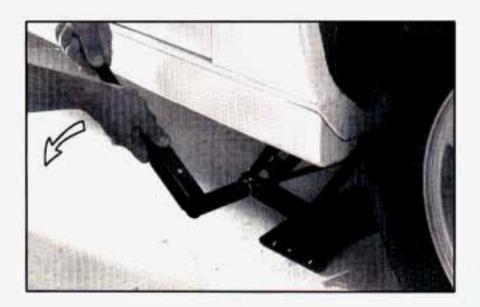
6. Lower the vehicle by rotating the wheel wrench left. Lower the jack completely.
