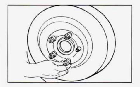
Replace the wheel nuts with the rounded end of the nuts toward the wheel. Tighten each nut by hand until the wheel is held against the hub.
