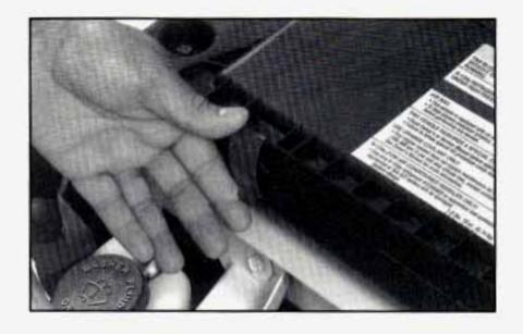
Unlatch the two clamps located on the front of the filter.
