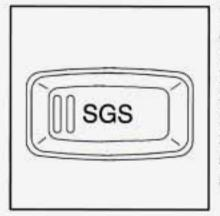
Your vehicle may be equipped with a Second-Gear Start feature. Press the Second Gear Start (SGS) switch on the instrument panel to provide more traction when you are starting on ice or other slippery surfaces.
