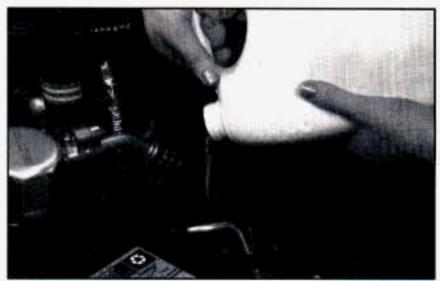
Fill the radiator with the proper DEX-COOL<sup>®</sup>
