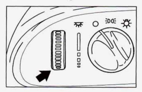
This switch controls the brightness of your instrument panel lights. Turn the switch to brighten or dim the lights. If you turn the switch all the way up, your courtesy lamps will come on.
