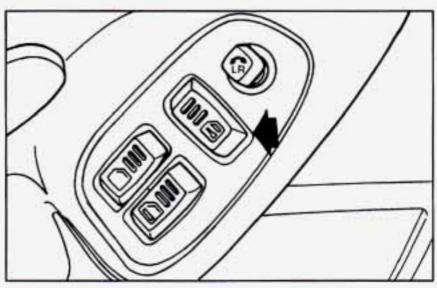
Press the power door lock switch to lock or unlock both doors at once. Note: Operating the power locks may affect the Vehicle and Content Theft-Deterrent/Alarm System (if you have this option). See "Vehicle and Content Theft-Deterrent /Alarm System" in the Index.
