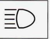
To change the headlamps from low beam to high or high to low, pull the turn signal lever all the way toward you. Then release it.
