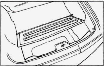
The close-out panel can be closed for hidden storage in the rear area of your vehicle. It can also help reduce noise in the vehicle when placed in the upright position, closing out the rear end area.
