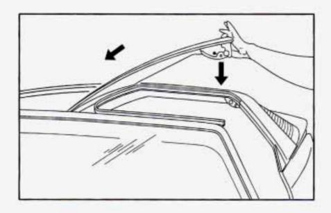
When installing the panels to the roof, keep the outboard edge of the panel raised about three inches above the roof while placing the inboard edge of the panel under the center roof.
