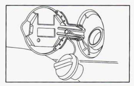
While refueling, hang the cap by the tether from the pin on the fuel door.
