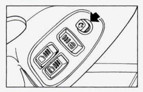
The power mirror control is on the driver's door. To adjust either mirror, turn the switch to left (L) or right (R). Then use the control to adjust the mirror.
