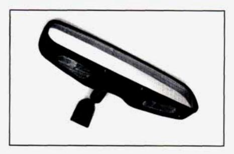
Your inside rearview mirror includes two map lamps. Each lamp has its own switch. Use the switch closest to the lamp to turn it on. The lamps will also go on when a door is opened.
