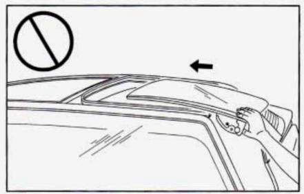
After the inboard edge of the panel is in position under the center roof rail, lower the outboard edge of the panel into position, close the latch and lock the T-top.
