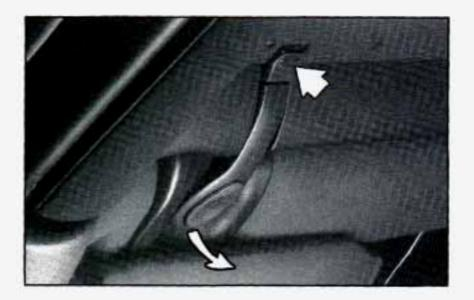
Unlock the front of the convertible top by pushing on the smaller part of the latch, then pulling down on the larger part of the latch. Be sure the hook on the latch that attaches into the hole at the windshield releases.
