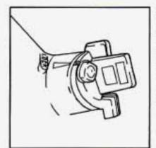
If you have a manual transmission, your ignition lock has a key release button. You must press the button before you can take your key out of the ignition lock.
