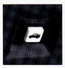
Press the switch under the lamp control below the instrument panel to unlock the hatch from inside your vehicle.
