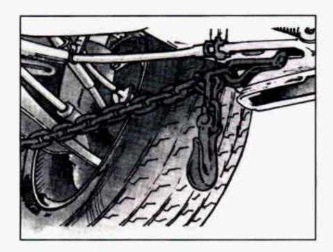
Attach T-hook chains to slots in frame, rearward of the front wheels, on both sides.
