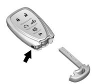
The key, inside the Remote Keyless Entry (RKE) transmitter, can be used for all locks.
