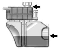
Fill the surge tank top chamber with the proper mixture to the bottom of the fill neck. The top chamber needs to be completely full. Fill the surge tank bottom chamber through the service port to approximately half.
