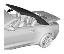
Lift and move the convertible top forward by pulling on both sides of the front bow into the fully closed position.
