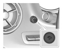
The knob for this feature is on the left side of the instrument panel. The brightness of the instrument cluster display, infotainment display and controls, steering wheel controls, and all other illuminated controls, as well as featured status indicators can be adjusted at night or in areas with limited lighting or when parklamps are ON.
