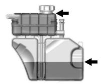
It is normal to see coolant moving in the upper coolant hose return line when the engine is running. It is also normal to see bubbles entering the surge tank through the small hose.
