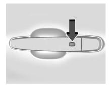
The RKE transmitter must be within 1 m (3 ft) of the trunk or door being opened. Press the button on the door handle to open. See "Keyless Access Operation" in Remote Keyless Entry (RKE) System Operation ⇒ 7.
