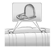
On coupe models, the top tether anchors are on the rear seatback filler panel.
