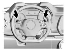
Tap Shift allows you to manually control the automatic transmission. To use Tap Shift, the shift lever must be in DSC mode. Vehicles with this feature have indicators on
