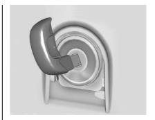
Remove any additional items attached to the key — such as keys, rings, or tags then fully insert the key into the manual release.
