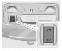
If equipped, the sunroof only operates when the ignition is on or in ACC/ACCESSORY, or when Retained Accessory Power (RAP) is active. See Retained Accessory Power (RAP) ⇒ 207.
