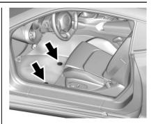
The driver side floor mat is held in place by two hook-type retainers.
