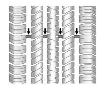
Treadwear indicators are one way to tell when it is time for new tires. Treadwear indicators appear when the tires have only 1.6 mm (1/16 in) or less of tread remaining. See *Tire Inspection* ⇒ 284 and *Tire Rotation* ⇒ 284 for additional information.
