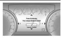
Auto Trans Only - Quickly apply full throttle. Release the brake pedal to launch the vehicle.
