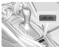
This optional handling mode can be selected by pressing the TCS/StabiliTrak/ESC button on the console two times. The appropriate message displays in the Driver Information Center (DIC).
