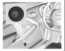
From inside the vehicle, press on the lower portion of the driver door.
