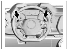
The system is activated and deactivated by pressing either of the paddles marked REV MATCH on the steering wheel. The system must be activated with each new ignition cycle.
