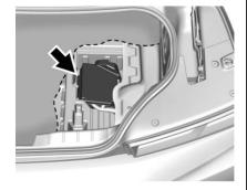
The rear compartment fuse block is on the right side under the trunk load floor.
