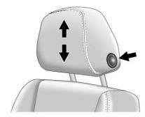
To raise or lower the head restraint, press the button located on the side of the head restraint, and pull up or push the head restraint down, and release the button. Pull and push on the head restraint after the button is released to make sure that it is locked in place.
