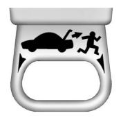
There is a glow-in-the-dark emergency trunk release handle on the trunk lid. This handle will glow following exposure to light. Pull the release handle to open the trunk from the inside.
