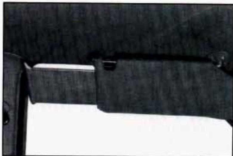
To block out glare, you can swing down the visors. You can also swing them from side to side. Your visors have an extension that can be pulled out for additional glare protection and a strap for holding small items, such as maps.
