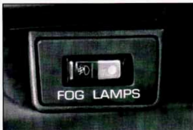
Press the right side of the switch to turn the fog lamps on, and the left side of the switch to turn them off. A light will glow in the right side of the switch when they are on.
