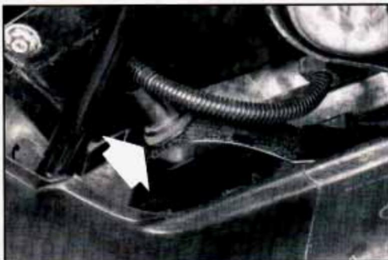
2. Turn the socket to the left and pull it out.
