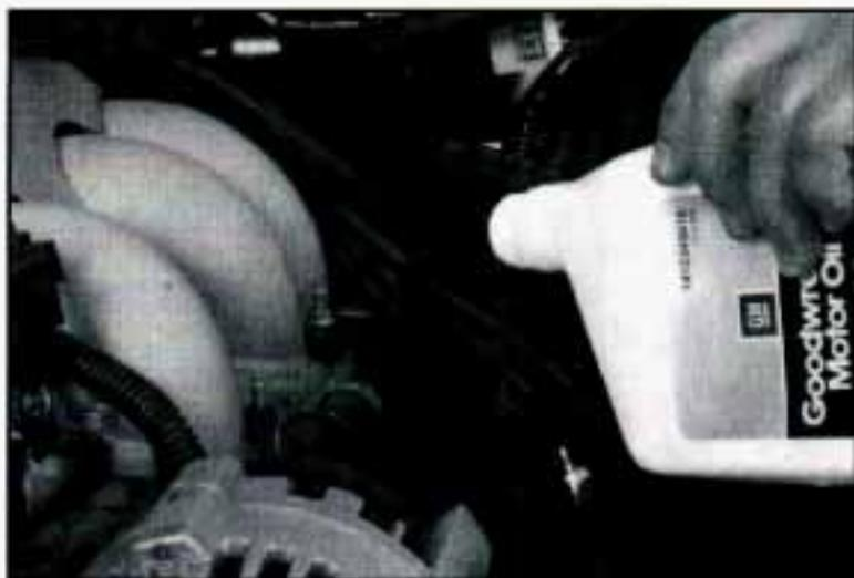
Just fill it enough to put the level somewhere in the proper operating range. Push the dipstick all the way back in when you're through.
