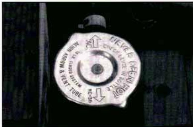
When you replace your radiator pressure cap, an AC<sup>®</sup> cap is recommended. See “Service Replacement Part and Filter Recommendations” in the Index.
