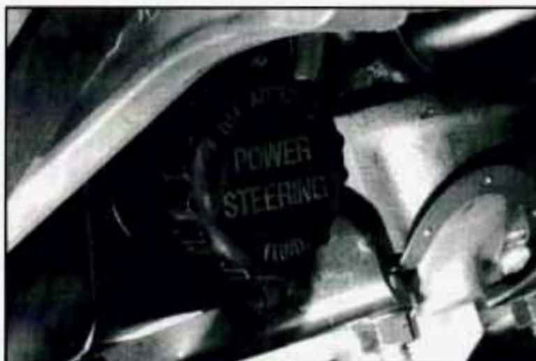
Unscrew the cap and wipe the dipstick with a clean rag. Replace the cap and completely tighten it.
