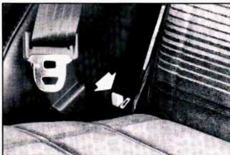
Push back on the seatback as you pull forward on the latch at the righthand side of the seat cushion. Then fold the seatback forward.
