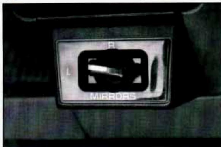
Move the switch to the right or left to choose the mirror, then move the switch from side to side or up and down as needed.
