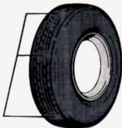
One way to tell when it's time for new tires is to check the treadwear indicators, which will appear when your tires have only  $\frac{2}{32}$  inch (1.6 mm) or less of tread remaining.
