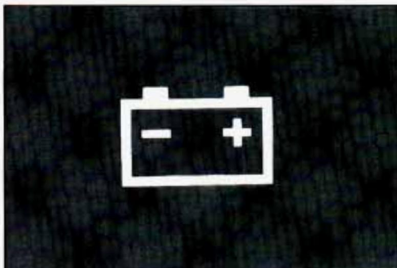
The charging system light is on your instrument cluster and will come on briefly when you turn on the ignition, but the engine is not running, as a check to show you it is working.
