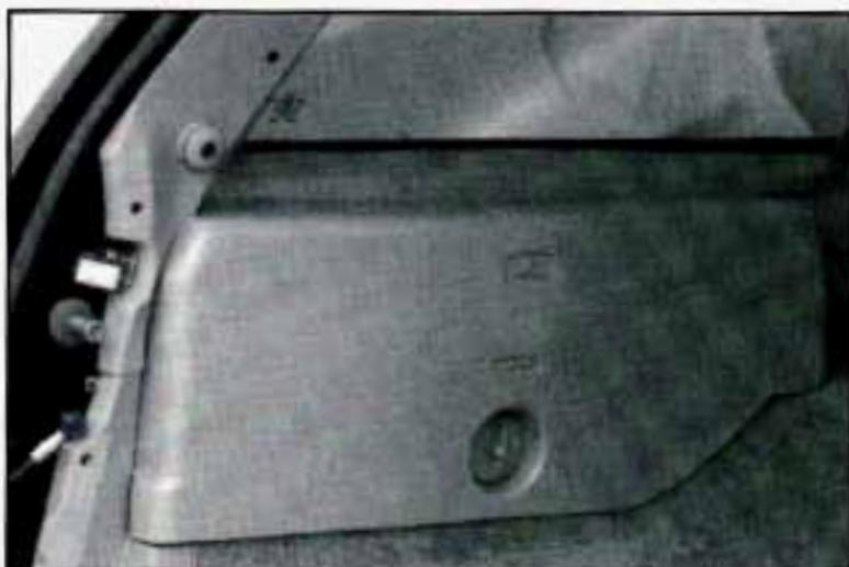
To remove your jack cover on two-door models, turn the plastic wing nut to the left until you can pull it out. Remove the jack cover.
