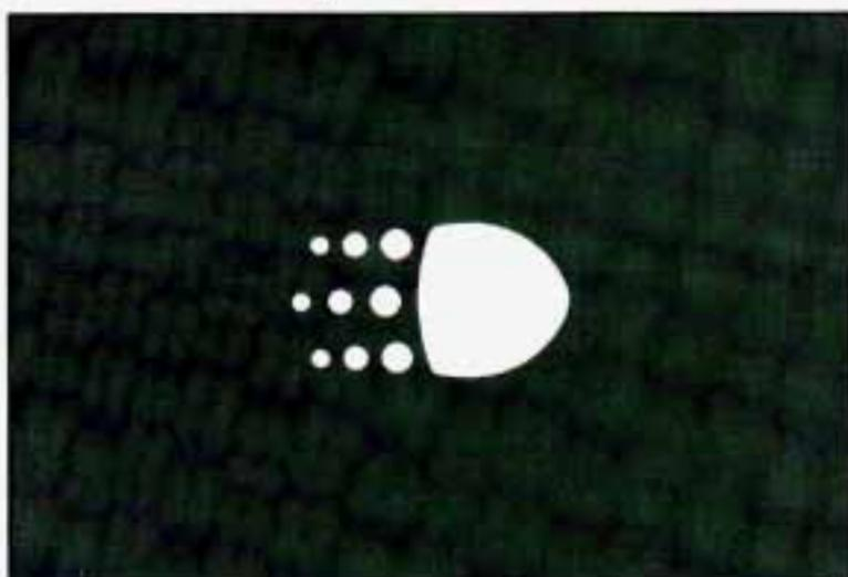
This green DRL indicator light is on the instrument cluster. The DRL indicator light is on whenever the ignition is on and the headlight switch and parking brake are off. For more details about DRL, see “Lights” in this section.
