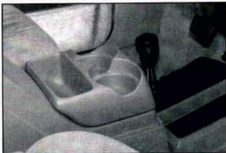
Your vehicle may have a console compartment between the bucket seats. To open it, just lift the top of the console while pressing the button on the driver's side.
