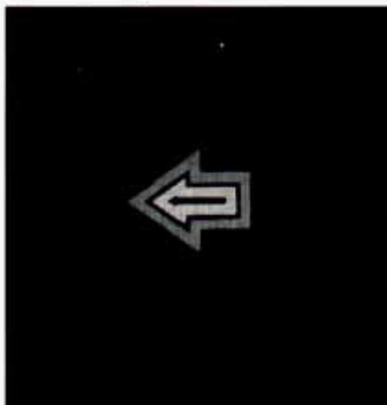
This light with the green arrows is on the instrument cluster. The turn signal indicator will come on whenever you signal a turn or lane change. See “Turn and Lane Change Signal” in this section.
