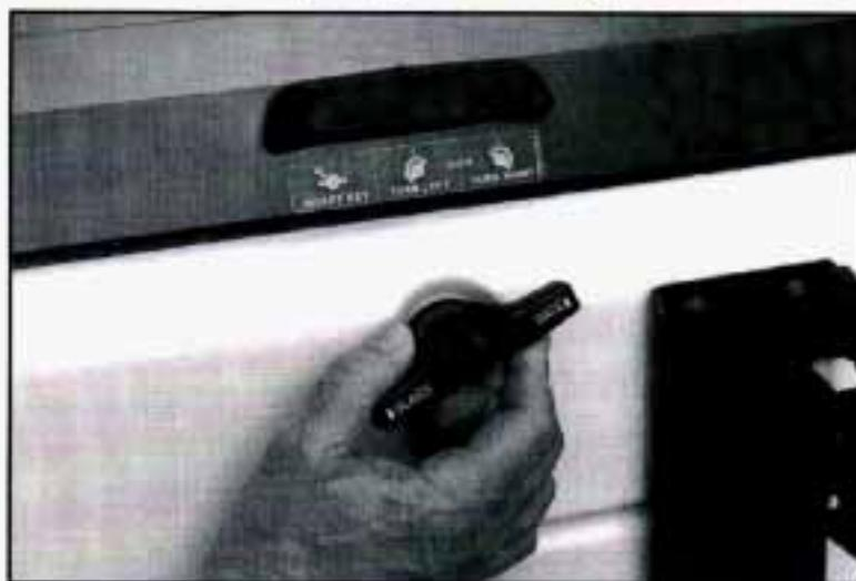
With the key in the lock, turn the lock handle to the left to unlock the glass. The endgate cannot be opened without first opening the endgate glass.
