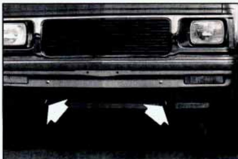
If you ever get stuck in sand, mud, ice or snow, your vehicle may be equipped with recovery hooks. The recovery hooks are provided at the front of your vehicle. You may need to use them if you’re stuck off-road and need to be pulled to some place where you can continue driving.
