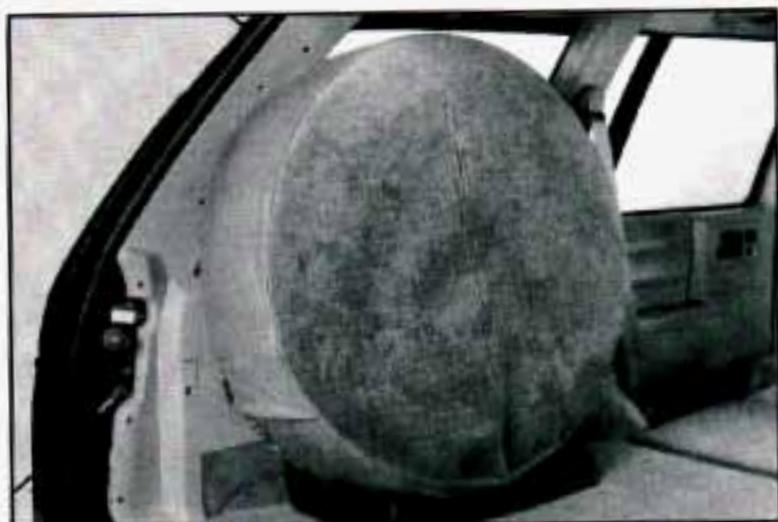
Your spare tire is in your vehicle's rear area, either mounted to the left wall, the floor, or the endgate.
