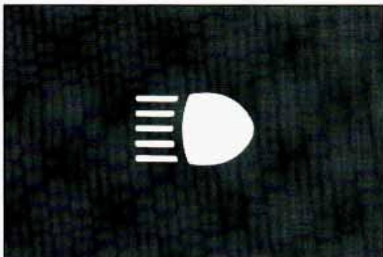
This blue high beam indicator light is on the instrument cluster and is on whenever you use your high beam headlights. For more details about high beams, see “Headlight High–Low Beam Changer” in this section.
