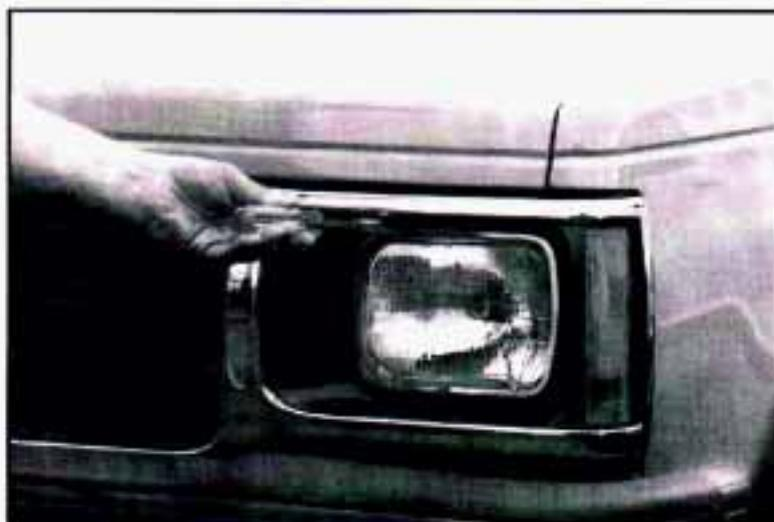
1. Remove the four screws from the headlight retainer.
