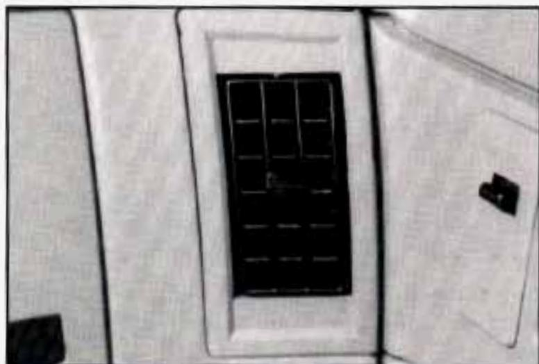
You will find air vents in the center and on the sides of your instrument panel. You can move the vents to direct the flow of air, or close the vents altogether. When you close a vent, it will increase the flow of air coming out of any vents that are open.
