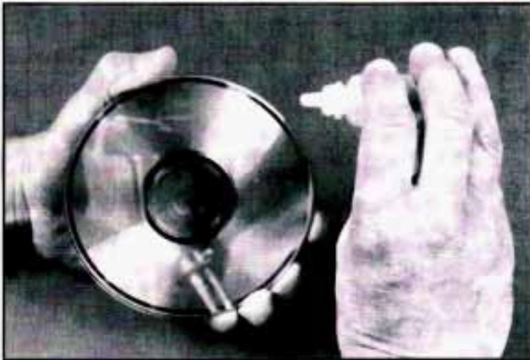
Be sure never to touch the signal surface when handling discs. Pick up discs by grasping the outer edges or the edge of the hole and the outer edge.
