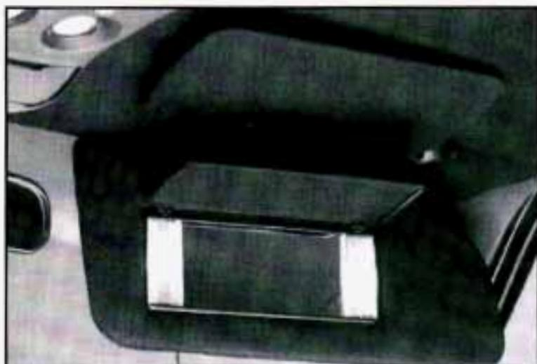
Some visors have mirrors built in, with and without lights. Just lift the mirror cover on each visor to turn the lights on if you have them.
