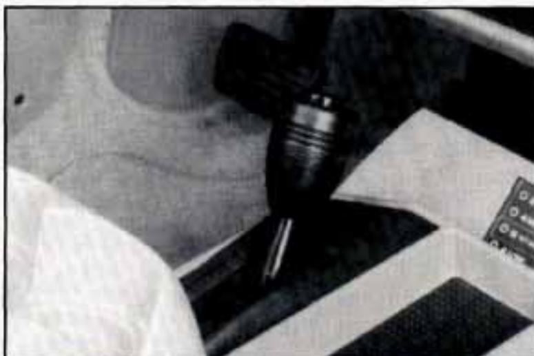
If your four-wheel drive vehicle has the manual transfer case, the transfer case shift lever is on the floor to the right of the driver. Use this lever to shift into and out of four-wheel drive.
