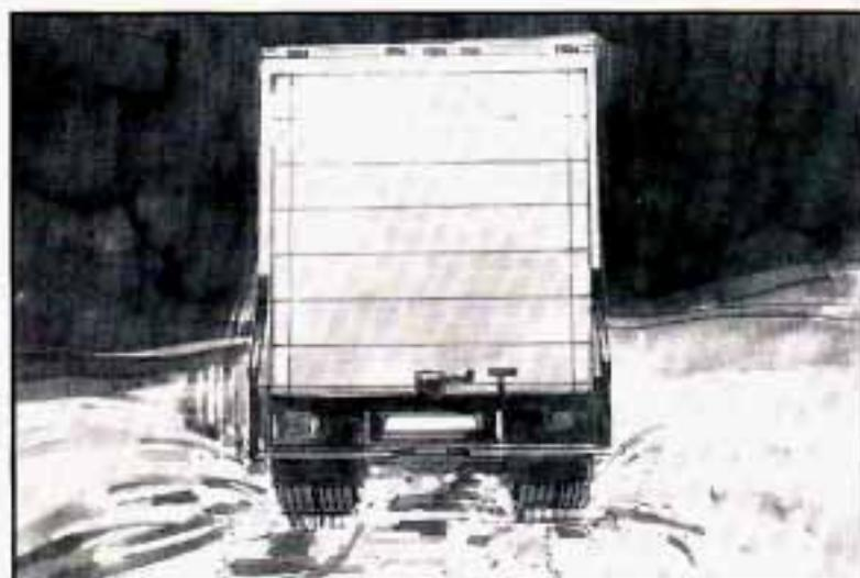
What's the worst time for this? "Wet ice." Very cold snow or ice can be slick and hard to drive on. But wet ice can be even more trouble because it may offer the least traction of all. You can get "wet ice" when it's about freezing (32°F; 0°C) and freezing rain begins to fall. Try to avoid driving on wet ice until salt and sand crews can get there.
