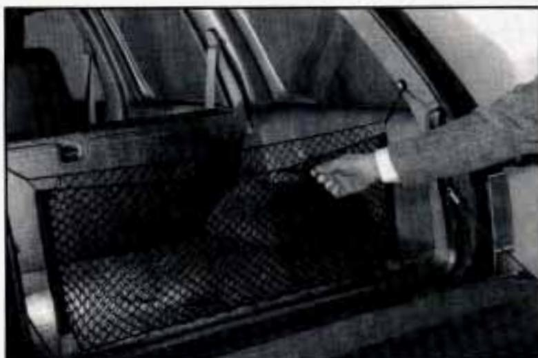
A convenience net may be provided for the rear of your vehicle to help keep small items, like gloves and light clothing in place during sharp turns or quick stops and starts.
