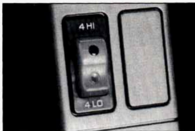
If your four-wheel drive vehicle has the electronic transfer case, the transfer case switch is on the left side of your instrument panel above the light switches. Use this switch to shift into and out of four-wheel drive. You can choose among three driving settings:
