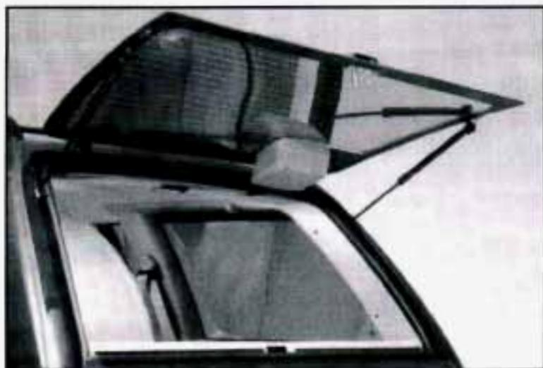
If your vehicle has a endgate-mounted spare tire carrier, you must move the carrier arm out of the way to open the glass.
