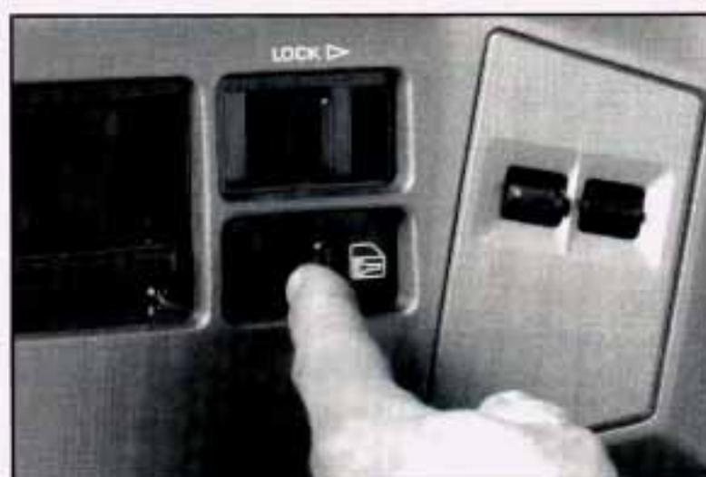
If your vehicle has power door locks, push the power door lock switch on either front door toward the key symbol. This switch will lock all the doors at once.
