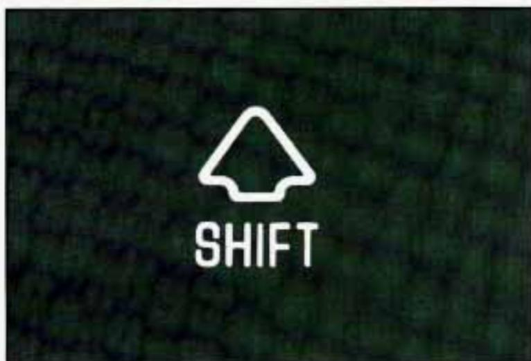
This amber **SHIFT** indicator light is on the instrument cluster of vehicles with manual transmissions. The **SHIFT** indicator light will help you get the best fuel economy. See “Shift Indicator Light” in this section.
