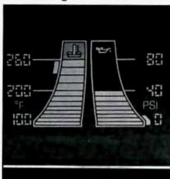
If you have a standard cluster, this gage shows the engine coolant temperature. If the gage pointer moves into the red area, your engine is too hot!
