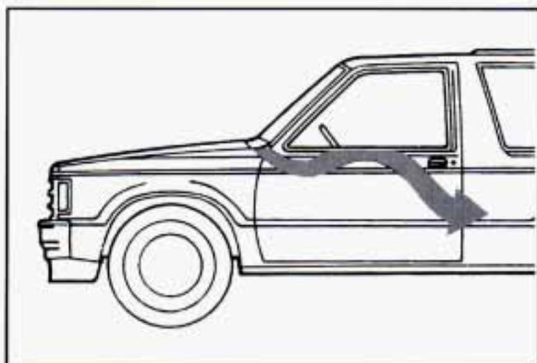
Your vehicle's flow-through ventilation system supplies outside air to the inside of your vehicle when it is moving. With the side windows closed, air will flow into the front air inlet grilles, through the vehicle, and out the rear air exhaust valve. Outside air will also enter the vehicle when the heater or the air conditioning fan is running.
