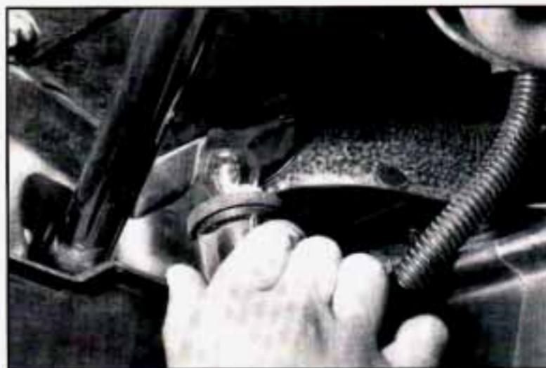
3. Turn the bulb to the left and pull it out of the socket.
