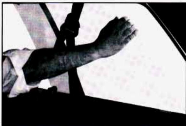
Your vehicle may have a sliding rear quarter window. Pull the latch in the center of the window and slide the glass to open it. When you close the window, be sure the latch catches.
