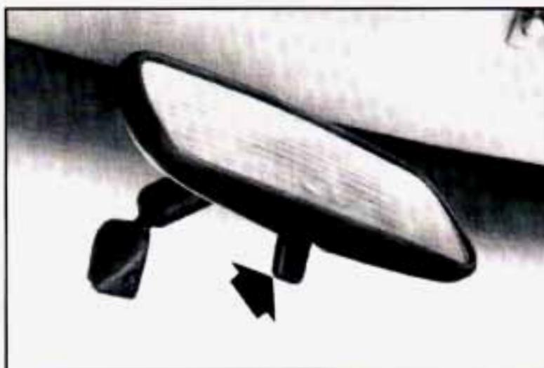
Press the tab under the mirror to reduce glare from headlights behind you.
