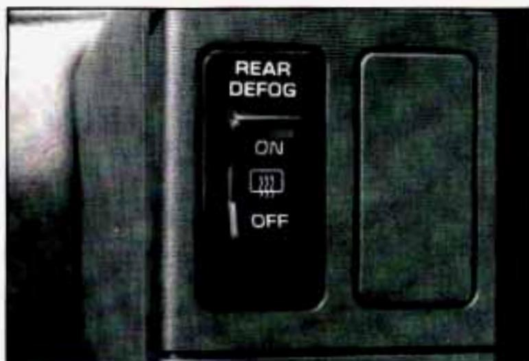
To turn on the rear window defogger, find the switch marked **REAR DEFOG** on your instrument panel. Press **“ON”** until the light in the switch comes on, then release it. The rear window defogger will only work if the ignition switch is turned to **RUN**.
