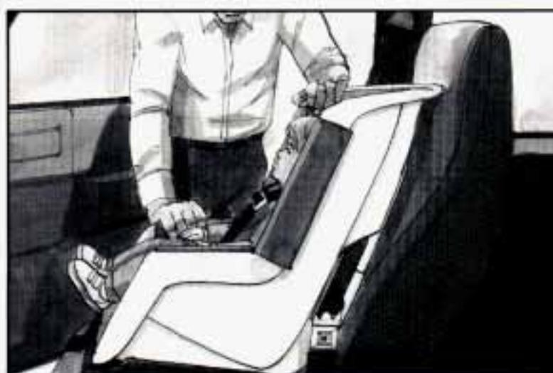
7. Push and pull the child restraint in different directions to be sure it is secure. If you're using a bucket seat, adjust the seat forward until the lap portion of the safety belt holds the restraint firmly. But don't move it any more than needed to tighten the lap belt.
