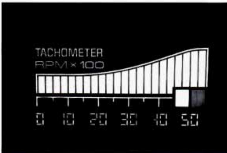
The tachometer displays the engine speed in revolutions per minute (rpm). It is available only with the digital speedometer.
