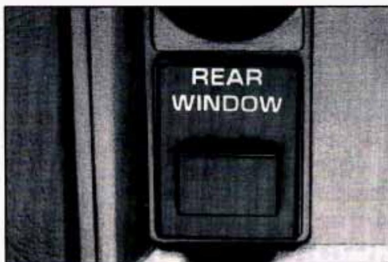
The electric endgate glass release lets you open your endgate glass by just pressing a button. The button is to the left of your radio.
