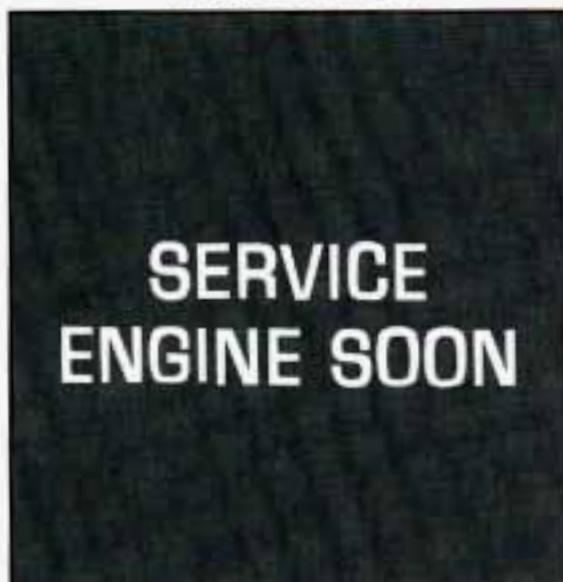
A computer monitors operation of your fuel, ignition and emission control systems. This light should come on when the ignition is on, but the engine is not running, as a check to show you it is working. If it does not come on at all, have it fixed right away. If it stays on, or it comes on while you are driving, the computer is indicating that you have a problem. You should take your vehicle in for service soon.
