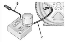
Attach the sealant/air hose (2) to the tire valve stem by turning it clockwise until tight.
