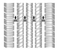
Treadwear indicators are one way to tell when it is time for new tires. Treadwear indicators appear when the tires have only 1.6 mm (1/16 in) or less of tread remaining. See *Tire Inspection*  $\Rightarrow$  310 and *Tire Rotation*  $\Rightarrow$  310.
