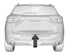
To unlock the liftgate, press on the power door lock switch or press on the Remote Keyless Entry (RKE) transmitter twice to unlock all doors. Press the touch pad in the liftgate handle and lift up. See Remote Keyless Entry (RKE) System Operation ⇒ 27.
