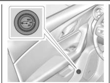
If equipped with a power liftgate, the switch is on the driver door. The vehicle must be in P (Park).
