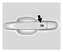
Press the button on the driver door handle when the RKE transmitter is within 1 m (3 ft) of the driver door handle. When unlocking from the driver door, the first press unlocks that door; press again within five seconds to unlock all passenger doors. See Remote Keyless Entry (RKE) System Operation
