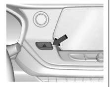
\( \begin{align\*} \tilde{\Delta} : Press to make the front and rear turn signal lamps flash on and off. This warns others that you are having trouble.
