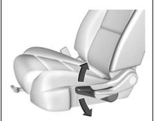
If equipped, move the lever up or down to manually raise or lower the seat.
