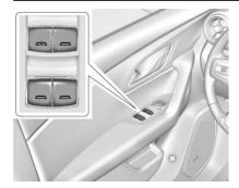
The power windows work when the ignition is on, in ACC/ACCESSORY, or when Retained Accessory Power (RAP) is active. See Retained Accessory Power (RAP) ⇒ 198.
