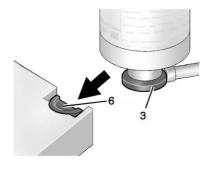
Slide the base of the tire sealant canister (3) into the slot on the top of the compressor (6) to hold it upright.
