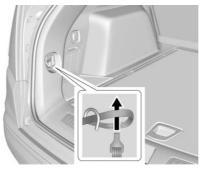
Place the loop end of the strap through the cargo tie-down. Place the hook end of the strap through the loop and pull it until the strap is fastened securely to the tie-down.
