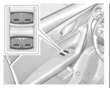
The power windows work when the ignition is on, in ACC/ACCESSORY, or when Retained Accessory Power (RAP) is active. See *Retained Accessory Power (RAP)* ⇔ *184*.
