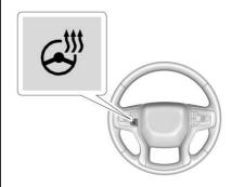
If equipped, press to turn the heated steering wheel on or off.
