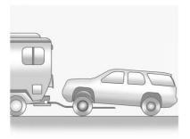
To tow a vehicle from the front with the rear wheels on the ground:
