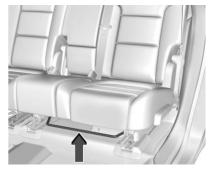
To adjust the seat position, lift the lever below the seat cushion and slide the seat forward or backward.
