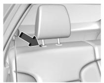
To lower the head restraint, press the button, located on the top of the seatback, and push the head restraint down. Try to move the
