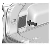
The rear compartment fuse block is behind a trim cover on the driver side of the rear storage compartment.
