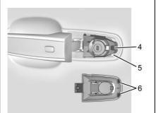
Insert the two tabs (6) at the back of the cap between the seal (5) and the metal base (4).
