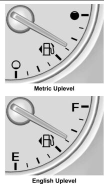
When the ignition is on, the fuel gauge indicates about how much fuel is left in the tank.
