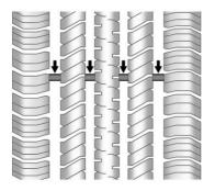
Treadwear indicators are one way to tell when it is time for new tires. Treadwear indicators appear when the tires have only 1.6 mm (1/16 in) or less of tread remaining. See *Tire Inspection*  $\Leftrightarrow$  298 and *Tire Rotation*  $\Leftrightarrow$  299.
