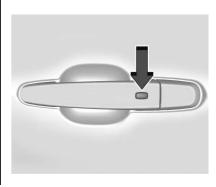
The RKE transmitter must be within 1 m (3 ft) of the liftgate or door being opened. Press the button on the door handle to unlock. See "Keyless Access Operation" in *Remote Keyless Entry (RKE) System Operation* ⇔ 8.
