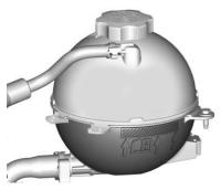
Check to see if coolant is visible in the coolant surge tank. If the coolant inside the coolant surge tank is boiling, do not do anything else until it cools down. See *Engine Overheating*  $\Rightarrow$  264.
