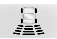
The instrument cluster may have a Park Assist display with bars that show "distance to object" and object location information for RPA. As the object gets closer, more bars light up and the bars change color from yellow to amber to red.
