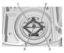
Turn the wing nut (4) counterclockwise to remove the jack (1), wheel wrench (2), and strap (3). Place the tool container near the tire being changed.
