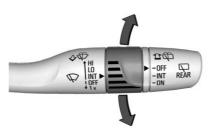
**INT :** Move the windshield wiper lever to INT. Turn the band up for more frequent wipes or down for less frequent wipes.
