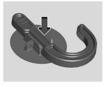
2. Push down on the other side of the load floor hook to lock into place.
