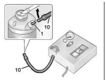
Attach the air only hose (10) to the sealant canister inlet valve (1) by turning it clockwise until tight.
