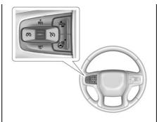
(c): Press to turn the system on or off. The indicator turns white on the instrument cluster when ACC is turned on.
