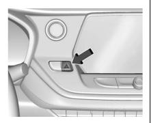
$\triangle$ : Press to make the front and rear turn signal lamps flash on and off. This warns others that you are having trouble.
