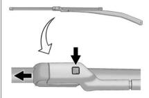
Press the button in the middle of the wiper arm connector, and pull the wiper blade away from the arm connector.
