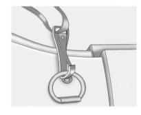
Attach the strap to the cargo tie-down in the rear of the vehicle.
