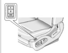
On vehicles with the memory feature, the "1" and "2" buttons on the outboard side of the driver
