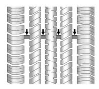
Treadwear indicators are one way to tell when it is time for new tires. Treadwear indicators appear when the tires have only 1.6 mm (1/16 in) or less of tread remaining. See *Tire Inspection on page 10-71* and *Tire Rotation on page 10-71* for more information.
