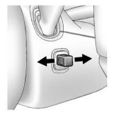
The switch used to adjust the pedals is located on the right side of the steering column, below the wiper stalk. Pull the switch toward you to move the pedals further from the floor, or push the switch away from you to move the pedals closer to the floor.
