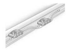
If the level of the shoulder is only slightly below the pavement, recovery should be fairly easy. Ease off the accelerator and then, if there is nothing in the way, steer so that the vehicle straddles the edge of the pavement. Turn the steering wheel 8 to 13 cm (3 to 5 in), about one-eighth turn, until the right front tire contacts the pavement edge. Then turn the steering wheel to go straight down the roadway.
