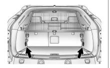
Mount the cargo net to the cargo tie-downs located on the lower side panels.
