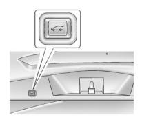
Press and release on the liftgate adjacent to the latch to close the liftgate.
