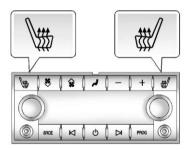
If available, the buttons are on the Rear Sear Audio (RSA) panel on the rear of the center console. With the ignition in ON/RUN/START, press # or # to heat the left or right outboard seat cushion and seatback. An indicator on the RSA display appears when this feature is on.
