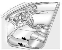
Pull up on the rear of the floor mat to unlock each retainer and remove.
