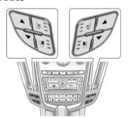
Heated and Ventilated Seat Buttons Shown, Heated Seat Buttons Similar
