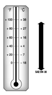
Cold Temperature Operation: In an area of extreme cold, where the temperature falls below -29°C (-20°F), an SAE 0W-30 oil should be used. An oil of this viscosity grade will provide easier cold starting for the engine at extremely low temperatures. When selecting an oil of the appropriate viscosity grade, be sure to always select an oil that meets the required specification, dexos. See "Specification" earlier in this section for more information.
