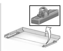
The loop of the D-ring slider must be facing inward toward the storage area and the ring must be in the up position for proper usage.
