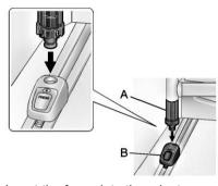
Insert the fence into the adapters and lock both latches (A) by turning to align • with the arrow on the adapter (B).
