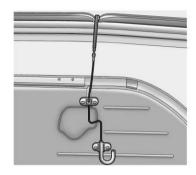
Store the cargo management system cover by hooking it onto the weatherstrip.
