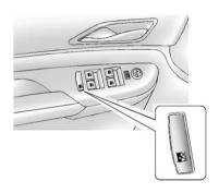
(Window Lockout): The window lockout switch is on the driver door This feature prevents the rear passenger windows from operating, except from the driver position. Press the switch to turn the lockout feature on or off. An indicator light shows the feature is on
