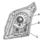
Up-Level Headlamp Assembly (Front View Driver Side)
