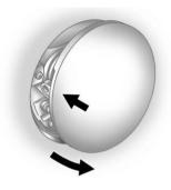
The tethered fuel cap is located behind a hinged fuel door on the passenger side of the vehicle.
