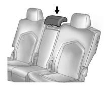
The center seating position has an integrated headrest that can be adjusted the same way as the head restraints.
