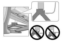
Raise the vehicle by turning the wheel wrench clockwise until the slots in the jack head fit into the metal flange located behind the triangle on the plastic moulding. Notice: Using a jack to raise the vehicle without positioning it correctly could damage your vehicle. When raising your vehicle on a jack, be sure to position it correctly under the frame and avoid contact with the plastic molding.
