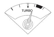
For vehicles with a turbo gauge, it indicates when the vehicle is using turbo power.
