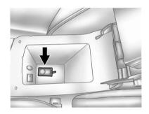
Place the new transmitter into the transmitter pocket. The transmitter pocket is inside the center console storage area located between the driver and front passenger seats. The storage area will need to be opened and the storage tray lifted up to access the transmitter pocket.
