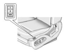
On vehicles with the memory feature, the "1" and "2" buttons on the outboard side of the driver seat are used to manually save and recall the positions of the driver seat, outside mirrors, and adjustable throttle and brake pedal positions, if available. These manually stored positions are referred to as Button Memory positions.
