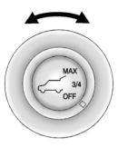
On vehicles with a power liftgate the switch is located on the driver door. The vehicle must be in P (Park) to use the power feature. The taillamps flash when the power liftgate moves.
