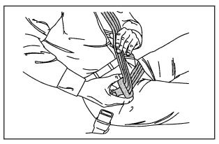
If the belt stops before it reaches the buckle, tilt the latch plate and keep pulling until you can buckle the belt.
