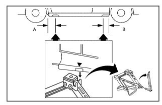
Find the jacking location using the diagram above and corresponding hoisting notches located in the plastic molding. The notches in the plastic molding are marked with a triangle shape to help you find them.
