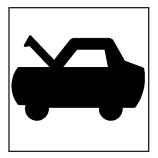
Pull the hood release lever with this symbol on it. It is located inside the vehicle on the lower left side of the instrument panel.
