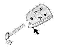
This key, inside the Remote Keyless Entry (RKE) transmitter, is used for the driver door, rear folding seats and rear seat pass-through door. To remove the key, press the button on the side of the transmitter near the bottom, and pull the key out. Never pull the key out without pressing the button.
