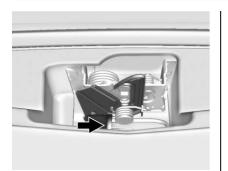
2. Go to the front of the vehicle to find the secondary hood release handle. The handle is under the front edge of the hood near the center. Push the handle to the right and at the same time raise the hood.
