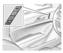
The SET, 1, 2, and D (Exit) buttons on the driver door are used to manually store and recall memory settings for the driver seat, outside mirrors, and power tilt and telescoping steering column (if equipped).
