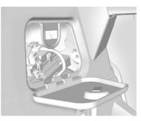
The rear compartment fuse block is behind a cover on the driver side of the rear compartment.
