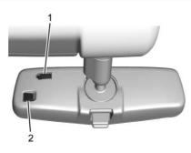
To adjust the brightness, press the button (1) on the back of the rearview mirror without covering the light sensor (2).
