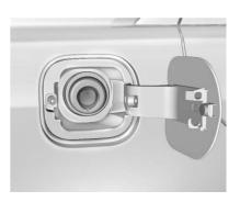
To open the fuel door, push and release the rearward center edge of the door. The fuel door is locked when the vehicle doors are locked. Press  $\overrightarrow{r}$  on the RKE transmitter to unlock. See *Remote Keyless Entry (RKE) System Operation*  $\Leftrightarrow$  29.
