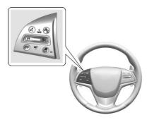
The Collision Alert control is on the steering wheel. Press  $\stackrel{\checkmark}{\longrightarrow}$  to set the FCA timing to Far, Medium, Near, or on some vehicles, Off. The first button press shows the current setting on the DIC. Additional button presses will change this setting. The chosen setting will remain until it is changed and will affect the timing of both the Collision Alert and the Tailgating Alert features. The timing of both
