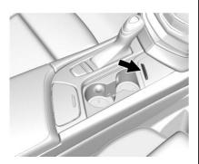
Cupholders in the front center console have a power retractable cover. Push the handle forward to express open. Pull the handle rearward to express close.
