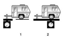
The trailer tongue (1) should weigh 10 to 15 percent of the total loaded trailer weight (2).
