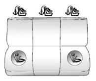
Rear Seat Seating positions with top tether anchors. Seating positions with two lower anchors.
