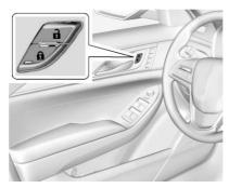
From inside, press  $\widehat{\mathbf{r}}$  or  $\widehat{\mathbf{n}}$ . The indicator light in the switch will illuminate when locked. See *Power Door Locks*  $\Rightarrow$  *39*.
