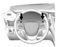
Vehicles with Tap Shift have controls on the back of the steering wheel to manually shift the automatic transmission.
