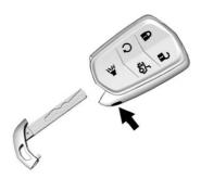
Press the button to remove the key. The key can be used for the driver door, rear folding seats and the rear seat pass-through door.
