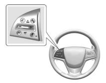
(5): Press to turn the system on or off. A white cruise control indicator comes on.
