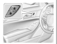
**a** : Press to lock the doors. The indicator light in the switch will illuminate when activated.
