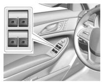
The windows work when the vehicle is in ON/RUN or ACC/ACCESSORY, or when Retained Accessory Power (RAP) is active. See *Retained Accessory Power* (RAP)  $\Rightarrow$  208.
