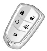
**\widehat{o}**: Press to lock all doors. The turn signal indicators may flash and/or the horn may sound on the second press to indicate locking. See *Vehicle Personalization*  $\Rightarrow$  *150*.
