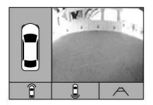
If equipped, a view of the area in front of the vehicle displays in the center stack. The view displays after shifting from R (Reverse) to a forward gear, or by pressing CAMERA in the center stack, and when the vehicle is moving forward slower than 8 km/h (5 mph). If equipped, the front view camera also displays when the Parking Assist system detects an object within 30 cm (12 in).
