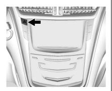
$\triangle$ : Press and hold this button for one second to make the front and rear turn signal lamps flash on and off. Release the button for at least one second and press again to turn the flashers off.
