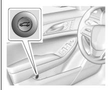
To open the trunk, press  $\iff$  on the driver door, press  $\approx$  twice quickly on the Remote Keyless Entry (RKE) transmitter, or press the touch pad on the rear of the vehicle after unlocking all doors.
