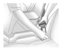
3. Push the latch plate into the buckle until it clicks. If the latch plate will not go fully into the buckle, check if the correct buckle is being used.
