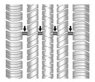
Treadwear indicators are one way to tell when it is time for new tires. Treadwear indicators appear when the tires have only 1.6 mm (1/16 in) or
