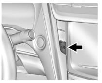
The automatic engine stop/start function can be disabled using the switch. The indicator on the switch will illuminate when the system is operational. When  $(\widehat{A})$  comes on green in the instrument cluster, the system is active. The system is not active when it comes on white with a slash through it.
