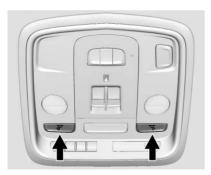
Press  $\overline{\mathscr{W}}$  or  $\overline{\mathscr{W}}$  next to each overhead console reading lamp.
