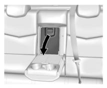
The vehicle has a rear seat pass-through door in the center of the rear seatback. Fold down the center armrest and pull the lever all the way down to release the door. The pass-through door can be locked or unlocked using the knob on the back of the door. Open the trunk to access the lock. Turn the knob toward to lock the door or away from to unlock the door.
