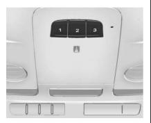
If equipped, this system provides a way to replace up to three remote control transmitters used to activate devices such as garage door openers, security systems, and home automation devices. Read the instructions completely before attempting to program the Universal Remote system. Because of the steps involved, it may be helpful to have another person available to assist you with programming the Universal Remote system.
