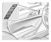
The SET, 1, 2, and D (Exit) buttons on the driver door are used to manually store and recall memory settings for the driver seat, outside mirrors, power tilt and telescoping steering column (if equipped).
