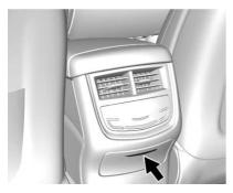
If equipped, press the top of the door to open the storage area on the rear of the center console. If equipped, there is a power outlet inside. Additional Storage Features
