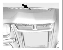
If equipped, the light sensor is on top of the instrument panel or on the windshield near the rearview mirror. Do not cover the sensor, otherwise the headlamps will come on when they are not needed.
