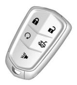
If the driver door is open when is pressed and Unlocked Door Anti-Lockout is enabled through the vehicle personalization, all doors will lock and then the driver door will immediately unlock. See *Vehicle Personalization*
