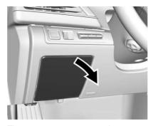
The storage compartment has a press to open latch. To access the fuses, open the compartment by pressing and releasing near the top center square.
