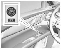
Move the selector switch to L (Left) or R (Right) to choose the driver or passenger mirror.
