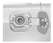
If equipped, the fuel door is locked when the vehicle doors are locked. Press on the RKE transmitter to unlock.
