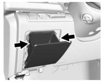
Apply pressure to the two retaining tabs on the sides of the compartment, until the two retaining tabs clear the sides of the instrument panel. Allow the compartment to move downward, and out of the way.
