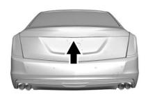
Press the touch pad on the rear of the trunk above the license plate when all doors are unlocked.
