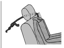
If the position you are using has an adjustable head restraint and you are using a single tether, route the tether around the inboard side of the head restraint.
