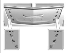
If equipped, the buttons are near the climate controls on the center stack. To operate, the ignition must be in ON/RUN.
