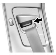
Press the release button and move the height adjuster to the desired position. The adjuster can be moved up by pushing the slide/trim up. After the adjuster is set to the desired position, try to move it down without pushing the release button to make sure it has locked into position.
