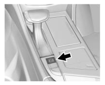
AVH can be turned on by pressing AVH with the driver safety belt fastened, the driver door closed, and the engine running. The AVH indicator will come on.
