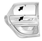
If equipped, use the handle to pull the sunshade up and attach to the holder at the top of the window.
