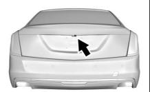
The camera that provides the Rear Camera Mirror (RCM) image is above the license plate, next to the Rear Vision Camera (RVC).
