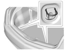
The cargo tie-downs can be used to secure small loads and the convenience net. See Convenience *Net*  $\Rightarrow$  108, if equipped.
