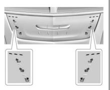
If equipped, the buttons are near the climate controls on the center stack. To operate, the ignition must be in ON/RUN.
