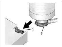
5. Slide the base of the tire sealant canister (3) into the slot on the top of the compressor (6) to hold it upright.
