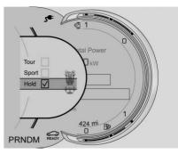
Use Hold Mode on a trip where it is expected that all of the electric charge will be depleted. Use Hold Mode mainly during highway or high speed driving to maximize both hybrid propulsion miles and fuel efficiency.
