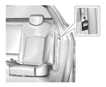
The handle is under the trim between the rear seat and the rear driver side door frame.
