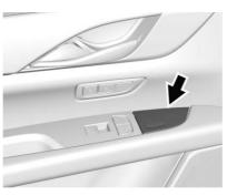
If equipped, press the lid to access the storage compartment in the rear doors.
