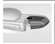
3. Move the cap inward and press to snap the cap in place.
