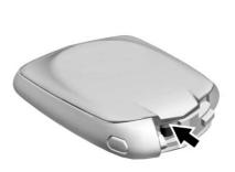
2. Separate the two halves of the transmitter using a flat tool inserted into the bottom center of the transmitter. Do not use the key slot.
