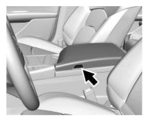
Press the button and lift to access the storage area. There is an auxiliary jack and USB port(s) inside. See the infotainment manual.
