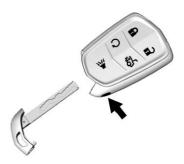
Press the button to remove the key. The key can be used for the driver door.
