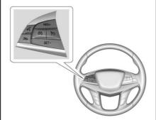
(5): Press to turn the system on and off. A white indicator appears in the instrument cluster when cruise is turned on.
