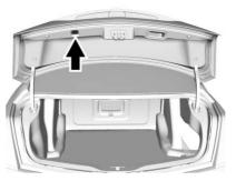
• Press the power trunk button on the trunk lid.
