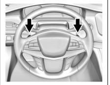
While using Regen on Demand, the vehicle will have increased coast deceleration. Use this to maximize regenerative braking, for sport driving, or when descending hills.
