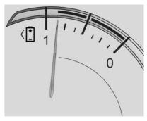
This gauge shows the high voltage battery charge level.
