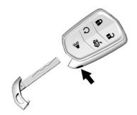
This key, inside the Remote Keyless Entry (RKE) transmitter, is used for the driver door. To remove the key, press the button on the side of the transmitter near the bottom, and pull the key out. Never pull the key out without pressing the button.
