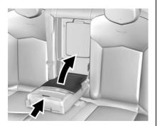
Press the latch to access the storage area in the rear armrest. Press the button to extend the cupholders.
