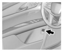
Press the fuel door button on the driver door for one second.
