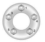
16. Tighten the wheel nuts firmly in a crisscross sequence, as shown.
