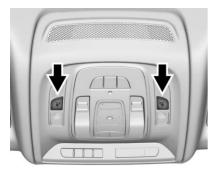
Press  $\overline{\mathscr{A}}$  or  $\overline{\mathscr{A}}$  next to each overhead console reading lamp.
