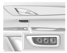
If equipped, press  $\stackrel{\frown}{=}$  to return the seat to the full rearward and full front of seat tilt down position. The seat will also move to this position when the rear door is opened.
