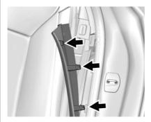
1. Remove the trim molding by pulling until the top three attachments are removed.
