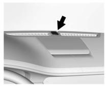
There is a light sensor on top of the instrument panel. Do not cover the sensor.
