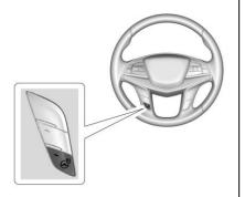
If equipped with a heated steering wheel, press to turn on or off. An indicator next to the button is lit when the feature is turned on.
