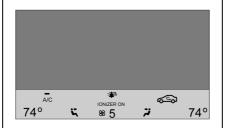
The climate control status screen appears briefly when the climate control buttons on the faceplate are adjusted.
