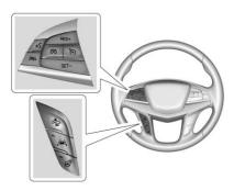
The Collision Alert control is on the steering wheel. Press Song to set the FCA timing to Far, Medium, or Near, or on some vehicles, Off. The first
