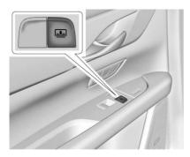
The rear door panels have controls for the rear sunroof sunshade. Press 主 to open or close.
