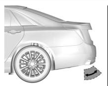
To operate, kick your foot straight up in one swift motion under the center of the rear bumper, then pull it back.
