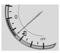
The power gauge shows the vehicle's total power consumption coming from the engine and/or battery.
