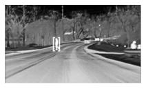
With the Front Pedestrian Braking system turned on, Night Vision provides a red Head-Up Display (HUD) alert when the system detects that the vehicle is approaching a pedestrian ahead much too quickly. In addition, an alert beeps or the Safety Alert Seat pulses, if equipped. See *Front Pedestrian Braking (FPB) System* ¢ 272.
