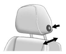
The fore and aft position of the head restraint can be adjusted.
