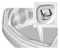
The cargo tie-downs can be used to secure small loads and the convenience net. See *Convenience Net* ⇔ *115*, if equipped.
