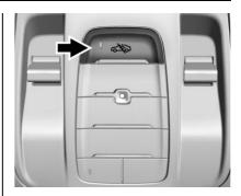
With the vehicle turned off, press in the front overhead console. The indicator light will come on momentarily, indicating that these sensors have been disabled for the next alarm system arming cycle.
