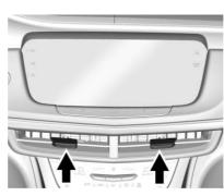
Adjustable air vents are in the center and on the sides of the instrument panel, on the rear of the center console storage, and in the headliner over the rear seats, if equipped.
