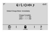
When the Programmable Charging system is disabled, the Default Charge Mode Status screen and the pop-up will display "- -:- -" for the Charge Complete Time. The Programmable Charging system will be disabled if the Charge Complete Time cannot be confidently estimated. If the Programmable Charging system is consistently disabled, see your dealer. A message displays if the vehicle is not able to charge.
