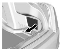
The rear compartment fuse block is behind a cover on the passenger side of the rear compartment.
