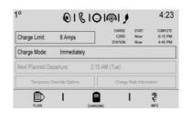
**Immediately :** The vehicle starts charging as soon as it is connected to an electrical outlet. See *Plug-In Charging (Hybrid Only)* \$ 282.
