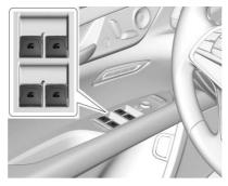
The windows work when the vehicle is in ON/RUN, ACC/ACCESSORY, or Retained Accessory Power (RAP). See *Retained Accessory Power* (*RAP*)  $\Rightarrow$  232.
