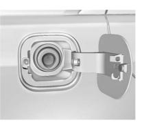
To open the fuel door, push and release the rearward center edge of the door. The fuel door is locked when the vehicle doors are locked. Press **a** on the RKE transmitter to unlock.
