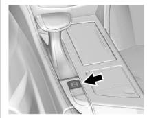
Automatic Vehicle Hold (AVH) can be turned on by pressing AUTO HOLD with the driver safety belt fastened, the driver door closed, and the engine running. The AVH indicator will come on.
