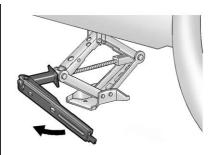
9. Raise the vehicle by turning the jack handle clockwise. Raise the vehicle far enough off the ground so there is enough room for the road tire to clear the ground.
