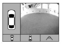
If equipped, a view of the area in front of the vehicle displays in the infotainment display. The view displays after shifting from R (Reverse) to a forward gear, or by pressing CAMERA in the center stack, and when the vehicle is moving forward slower than 8 km/h (5 mph). If equipped, the front view camera also displays when the Front Parking Assist system detects an object within 30 cm (12 in).
