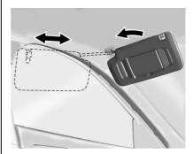
Pull the sun visor down to block glare. Detach the sun visor from the center mount to pivot to the side window, or to extend along the rod.
