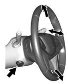
Press the control to move the tilt and telescoping steering wheel up and down or forward and rearward.
