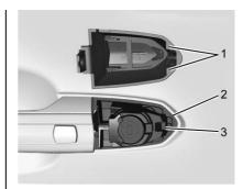
2. Insert the tabs (1) on the rear of the cap into the space between the seal (2) and the metal base (3).
