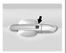
Press the lock/unlock button when the RKE transmitter is within 1 m (3 ft) of the driver door handle. When unlocking from the driver door, the first press unlocks that door; press again within five seconds to unlock all passenger doors. See *Remote Keyless Entry* (*RKE*) *System Operation*  $\Rightarrow$  35.
