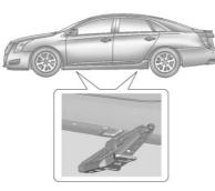
8. Position the jack lift head at the jack location nearest the flat tire within the depression of the jack pads, as shown. The jack must not be used in any other position.
