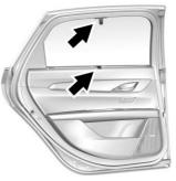
If equipped, use the handle to pull the sunshade up and attach to the holder at the top of the window.
