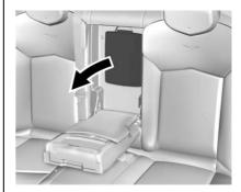
Some vehicles have a rear seat pass-through door in the center of the rear seatback. Fold down the center armrest and pull the latch to open the door.
