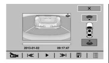
To Activate : Touch Video Recorder on the Home screen. Touch will have a red dot when the video recorder is on. It will remain on until it has been turned off. Recording will start after exiting the playback screen. Advise other drivers and occupants of the vehicle that video images are being recorded.
