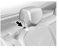
To lower the head restraint, press the button, located on the top of the seatback, and push the head restraint down. Try to move the head restraint after the button is released to make sure that it is locked in place. Always adjust the head restraint so that the top of the restraint is at the same height as the top of the occupant's head.
