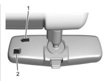
To adjust the brightness, press the button (1) on the back of the rearview mirror without covering the light sensor (2).
