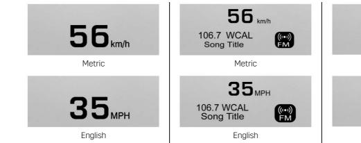
**Speed View :** This display gives the speedometer reading (in English or metric units), speed limit, Adaptive Cruise Control speed, Lane Departure Warning, and Vehicle Ahead indicator. Some information only appears on vehicles that have these features, and when they are active.
