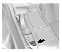
Press and release MODE on the center console to activate the mode menu in the instrument cluster. The first press of the button will show the current mode. Subsequent presses will scroll through the available modes. Select a new setting whenever driving conditions change. The following modes are available:
