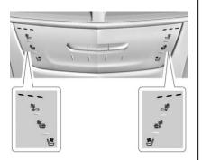
If equipped, the buttons are near the climate controls on the center stack. To operate, the ignition must be on.
