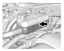
Check to see if coolant is visible in the reservoir. If coolant is visible but the coolant level is below the cold fill line, there could be a leak in the cooling system.
