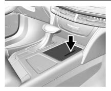
There are cupholders in the center console. Push and release on the passenger side of the cover to access the cupholders. Additional Storage Features
