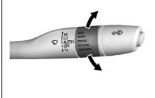
**AUTO :** Use this setting for intermittent wipes when Rainsense<sup>™</sup> is disabled, or for Rainsense wipes when it is enabled. For intermittent wipes, move the lever up to AUTO, then turn the band on the wiper lever up for more frequent wipes or down for less frequent wipes.
