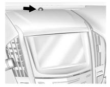
The solar sensor monitors the solar heat.
