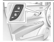
From the inside, press  $\widehat{\bullet}$  or  $\widehat{\bullet}$ . The indicator light in the switch will illuminate when locked. See *Power Door Locks*  $\Leftrightarrow$  41.
