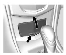
To access, press on the cover and release. There is an accessory power outlet inside. See *Power Outlets* ⇔ 114.
