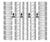
Treadwear indicators are one way to tell when it is time for new tires. Treadwear indicators appear when the tires have only 1.6 mm (1/16 in) or less of tread remaining. See *Tire Inspection*  $\Rightarrow$  303 and *Tire Rotation*  $\Rightarrow$  303.
