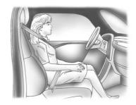
If a person of adult size is sitting in the front outboard passenger seat, but the off indicator is lit, it could be because that person is not sitting properly in the seat. Use the following steps to allow the system to detect that person and enable the front outboard passenger frontal airbag and knee airbag:
