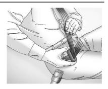
If the webbing locks in the latch plate before it reaches the buckle, tilt the latch plate flat to unlock.
