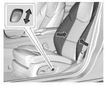
If equipped, to increase or decrease the back bolster support, press and hold the lumbar control up and down.
