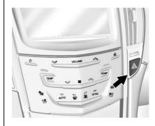
The hazard warning flashers turn on automatically if the airbags deploy.
