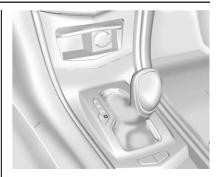
Vehicles with DSC may either use the shift lever or the tap shift controls on the back of the steering wheel (if equipped) to manually shift the automatic transmission.
