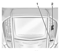
Use the thumbwheels (1) near the air vents to open or close off the airflow.
