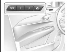
If equipped, memory seats allow two drivers to store and recall their unique seat positions for driving the vehicle, and a shared exit position for getting out of the vehicle. Other feature positions may also be set, such as power mirrors and power steering wheel, if equipped. Memory positions are linked to RKE transmitter 1 or 2 for automatic memory recalls.
