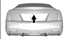
Press the touch pad on the rear of the trunk above the license plate when all doors are unlocked.
