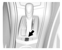
The automatic engine stop/start function can be disabled using the switch. The indicator on the switch will illuminate when the system is operational.
