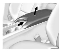
Press the button and lift to access the storage area. There is a USB Port and an auxiliary jack inside. See "USB Port" and "Auxiliary Jack" in the infotainment manual.
