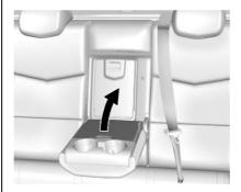
Pull the armrest down and lift the cover to access the storage area.
