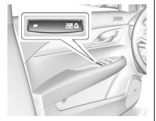
The rear door safety locks prevent passengers from opening the rear doors from inside the vehicle. Press a to activate the safety locks on the rear doors. The indicator light in the switch will illuminate when activated.
