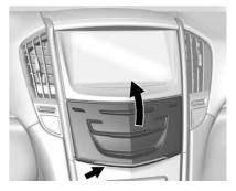
If equipped with storage behind the climate control system, touch the bottom of the climate control panel until the door starts to open. Touch the bottom of the climate control panel again until the door automatically starts to close.
