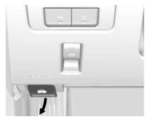
Pull the hood release handle inside the vehicle. It is on the lower left side of the instrument panel.
