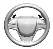
The system is activated and deactivated by pressing either of the paddles on the steering wheel. The system must be activated with each new ignition cycle.
