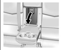
This vehicle may have a rear seat pass-through door in the center of the rear seatback. Fold down the center armrest and pull the latch to open the door.
