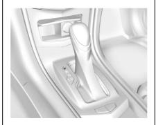
**P**: This position locks the drive wheels. Use P (Park) when starting the engine because the vehicle cannot move easily.
