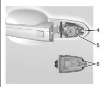
Insert the two tabs (6) at the back of the cap between the seal (5) and the metal base (4).
