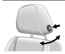
To adjust the head restraint forward and rearward, press the button located on the side facing of the head restraint and move it forward or rearward until the desired locking position is reached. Try to move the head restraint after the button is released to make sure that it is locked in place.
