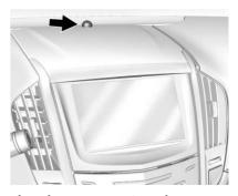
The solar sensor monitors the solar heat.
