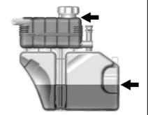
If coolant is visible but the coolant level is not at or above the cold fill line, add a 50/50 mixture of clean drinkable water and DEX-COOL coolant.
