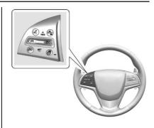
(5): Press to turn the system on and off. A white cruise control indicator appears in the instrument cluster when cruise is turned on.
