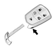
This key, inside the Remote Keyless Entry (RKE) transmitter, is used for the driver door and glove box. To remove the key, press the button near the bottom of the transmitter, and pull the key out. Never pull the key out without pressing the button.
