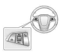
(On/Off): Press to turn the cruise control system on or off. A white indicator comes in the instrument cluster when cruise is turned on.
