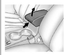
The armrest must be in the rearward position to open it. Lift the lever and then lift up on the armrest to access the storage area.
