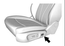
If available, press and hold the front of the switch to increase lumbar support, or the rear of the switch to decrease lumbar support. Release the switch when the seatback reaches the desired level of lumbar support.
