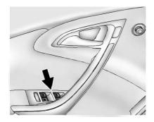
The power window switches are located on the driver door. Each passenger door has a switch that controls only that window.
