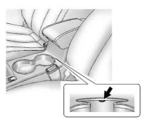
There are two cupholders in the center console with a removable liner. To remove the liner, lift up on the notch on the underside of the rear of the cupholder.
