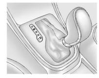
Move the shift lever from D (Drive) to the left into the (+) or (-) manual position.
