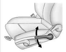
If available, move the lever up or down to manually raise or lower the seat.
