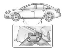
Position the jack lift head at the jack location nearest the flat tire. The location is indicated by a notch in the flange. The jack must not be used in any other position.
