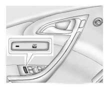
This feature prevents the rear passenger windows from operating, except from the driver position. This feature only works when the ignition is in ACC/ACCESSORY or ON/RUN, or in RAP.
