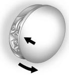
The fuel cap is behind a hinged fuel door on the passenger side of the vehicle. To open the fuel door, push and release the rearward center edge of the door.
