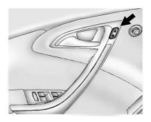
(Unlock): Press to unlock the doors.
