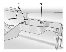
To reinstall the shelf, slide it into the side guides (1) and push back until it engages into the rear panel (2).
