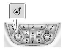
(Heated Steering Wheel): For vehicles with a heated steering wheel, press to turn it on or off. A light on the button displays when the feature is turned on.
