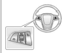
h: Press to turn the cruise control system on or off. A white indicator comes in the instrument cluster when cruise is turned on.
