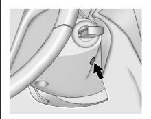
If charging or jump starting the battery does not work, locate the hole below the ignition lock. Insert a flat bladed tool or another key from the key chain into the opening. When the lever can be felt, actuate the lever toward the driver, and remove the key from the ignition.
