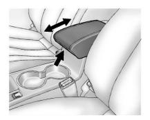
The armrest is adjustable. Lift the lever to move it forward or rearward.
