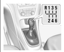
This is the shift pattern for the 6-speed manual transmission.
