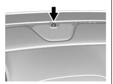
The indicator light, on the instrument panel near the windshield, indicates the status of the system:
