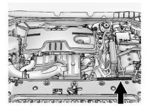
Lift the hood and pull the prop rod by the sleeve from the retainer, located above the radiator.
