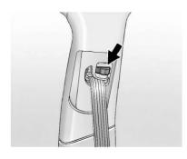
Press the release button and move the height adjuster to the desired position. The adjuster can be moved up by pushing the slide/trim up. After the adjuster is set to the desired position, try to move it down without pressing the release button to make sure it has locked into position.
