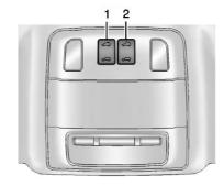
If equipped, the sunroof operates when the ignition is in ON/RUN or ACC/ACCESSORY, or in Retained Accessory Power (RAP). See Retained Accessory Power (RAP) \$ 192.
