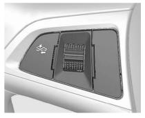
The Collision Alert control is on the steering wheel. Press to set the alert timing. The first button press shows the current control setting on the DIC. Additional button presses will change this setting and turn the system off.
