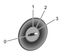
The ignition switch has four different positions.
