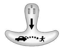
There is an emergency trunk release handle inside the trunk on the trunk lid. The release handle can be accessed by folding the rear seatback. See *Rear Seats* ⇔ *54*. Pull the release handle to open the trunk from the inside. After use, return to the stored position.
