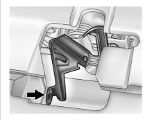
Go to the front of the vehicle and with hand palm side down, slide the secondary hood release handle toward the driver side of the vehicle.
