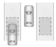
The SBZA sensor covers a zone of approximately one lane over from both sides of the vehicle, or 3.5 m (11 ft). The height of the zone is approximately between 0.5 m (1.5 ft) and 2 m (6 ft) off the ground. This zone starts at approximately the middle of the vehicle and goes back 5 m (16 ft).
