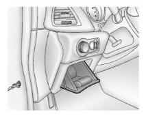
The instrument panel fuse block is on the driver side of the instrument panel. To access:
