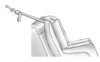
If you are using a single tether in the rear center seating position, route the single tether over the headrest.
