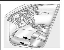
Reinstall by lining up the floor mat retainer openings over the carpet retainers and snap into position.
