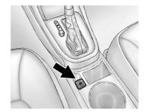
The Electric Parking Brake (EPB) switch is on the center console. The EPB can always be activated, even if the ignition is off. To prevent draining the battery, avoid repeated cycles of the EPB when the engine is not running.
