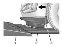
Ramps (2) are required for the front fascia (3) to clear the flatbed (1). The ramp height should be approximately 102 mm (4 in). Lower the flatbed onto the set of ramps.
