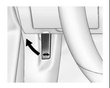
Pull up on the hood release handle. It is located inside the vehicle to the left of the steering column.
