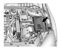
To open the fuse block cover, press the clips at the front and back and rotate the cover up to the side.
