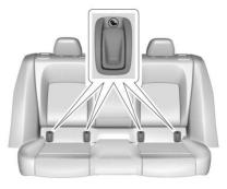
The lower anchors are located under the labeled covers on the seatback near the crease between the seatback and the seat cushion.
