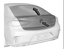
To unlock the liftgate, press on the power door lock switch or press on the Remote Keyless Entry (RKE) transmitter twice to unlock all doors and the liftgate. Press the emblem on the end of the liftgate to open the liftgate. See Remote Keyless Entry (RKE) System Operation ⇒ 29.
