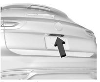
To open the liftgate, press the touch pad on the bottom of the liftgate.
