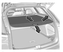
To use the cargo cover, pull the handle toward the rear and up until it engages in the side retainers.
