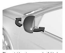
The outside mirrors can be folded inward to prevent damage when going through an automatic car wash. Push the mirror outward to return it to the original position.
