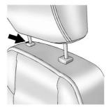
To lower the head restraint, press the button, located on the top of the seatback, and push the head restraint down. Try to move the head restraint after the button is released to make sure that it is locked in place.
