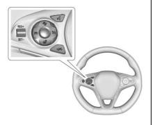
: Press to turn cruise control on or off. A white indicator comes on in the instrument cluster.
