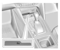
Place the new RKF transmitter into the storage bin with the buttons facing up.
