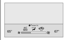
The climate control status display appears briefly when the center stack climate controls are adjusted. The air delivery mode can be adjusted on the climate control display.
