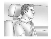
If equipped with base seats, adjust the head restraint so that the top of the restraint is at the same height as the top of the occupant's head. This position reduces the chance of a neck injury in a crash.
