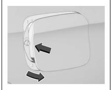
The fuel door is locked when the vehicle doors are locked. Press on the RKE transmitter to unlock.
