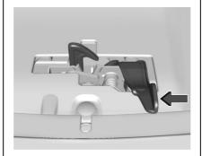
Go to the front of the vehicle to find the secondary hood release handle. The handle is under the front edge of the hood near the center. Push the handle to the right and at the same time raise the hood.
