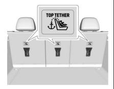
The top tether anchors are on the back of the rear seatbacks. Remove the cargo cover before installing the top tether. The cargo cover should remain off while the top tether is in use. Be sure to use an anchor on
