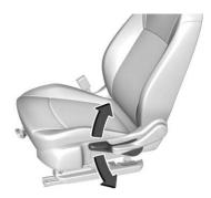
If available, move the lever up or down to manually raise or lower the seat.
