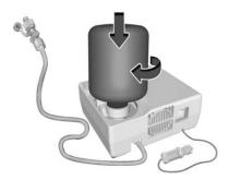
Remove the plug from the sealant canister inlet valve (2) and from the sealant canister (1).
