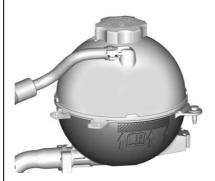
Check to see if coolant is visible in the coolant surge tank. If the coolant inside the coolant surge tank is boiling, do not do anything else until it cools down.
