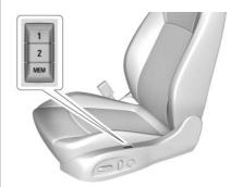
If equipped, memory seats allow two drivers to save and recall their unique seat positions for driving the vehicle. The driver seat may also be moved rearward to an exit position for getting out of the vehicle. Other feature positions may also be saved, such as power mirrors and power steering wheel, if equipped. Memory positions are linked to RKE transmitter 1 or 2 for automatic memory recalls.
