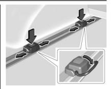
Press the button on a tie-down and slide it to the required position. Fold up the tie-downs to use them.
