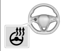
: If equipped, press to turn on or off. A light near the button displays when the feature is turned on. The steering wheel takes about three minutes to start heating.
