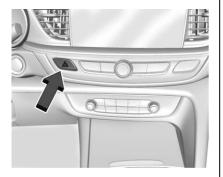
: Press to make the front and rear turn signal lamps flash on and off. Press again to turn the flashers off.
