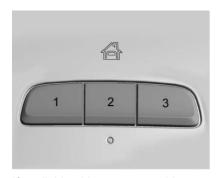
If available, this system provides a way to replace up to three remote control transmitters used to activate devices such as garage door openers, security systems, and home automation devices.
