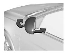
The mirrors can be folded inward toward the vehicle to prevent damage when going through an automatic car wash. Push the mirror outward to return it to the original position.
