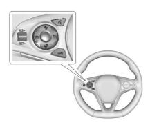
(iii): Press to turn the system on or off. The indicator turns white on the instrument cluster when ACC is turned on.
