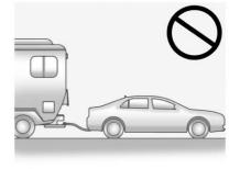
The vehicle was not designed to be towed from the rear with all four wheels on the ground.
