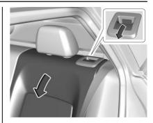
Pull on the lever on the top of the seatback to unlock it and fold the seatback forward.
