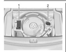
Remove the compressor (1) and the tire sealant canister (2).
