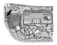
The electrical cord is located on the passenger side of the engine compartment, between the fender and the air cleaner.
