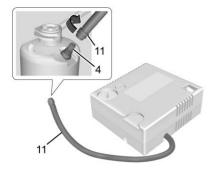
Attach the air only hose (11) to the sealant canister inlet valve (4) by turning it clockwise until tight.
