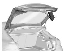
Use the handle to lower and close the liftgate. If equipped, do not press the touch pad while closing the liftgate. This will cause the liftgate to be unlatched.
