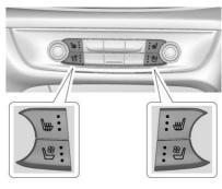
If equipped, the buttons are near the climate controls on the center stack. To operate, the engine must be running.
