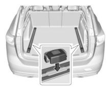
Insert the tie-downs into the rails and press the button while inserting it.
