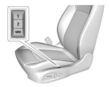
If equipped, memory seats allow two drivers to save and recall their unique seat positions for driving the vehicle. Other feature positions may also be saved, such as power mirrors and power steering wheel, if equipped. Memory positions are linked to RKE transmitter 1 or 2 for automatic memory recalls.
