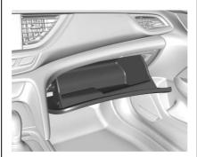
Lift up the handle to open the glove box.
