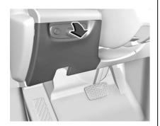
The instrument panel fuse block is in the instrument panel, on the driver side of the vehicle. To access the fuses, press in on the sides of the cover and pull to release it from the instrument panel.
