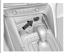
The 12-volt power outlets can be used to plug in electrical equipment, such as a cell phone or MP3 player.
