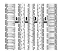
Treadwear indicators are one way to tell when it is time for new tires. Treadwear indicators appear when the tires have only 1.6 mm (1/16 in) or less of tread remaining. See *Tire Inspection* ♀ 289 and *Tire Rotation* ♀ 289.
