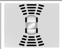
The instrument cluster may have a Park Assist display with bars that show "distance to object" and object location information for RPA, and on some vehicles, FPA. As the object gets closer, more bars light up and the bars change color from yellow to amber to red
