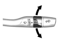
**INT:** Use for intermittent wipes. To adjust wipe frequency, turn the band up for more frequent wipes or down for less frequent wipes.
