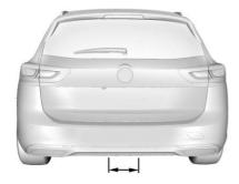
If equipped, the liftgate may be operated with a kicking motion under the rear bumper at the location of the projected logo.
