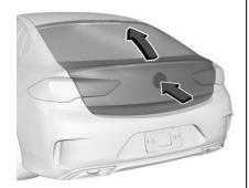
To open the liftgate, press the emblem on the end of the liftgate. Unlocking all doors will also unlock the liftgate.
