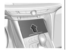
To open the front storage compartment, slide the cover forward.
