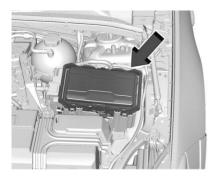
To remove the fuse block cover, squeeze the three retaining clips on the cover and lift it straight up.
