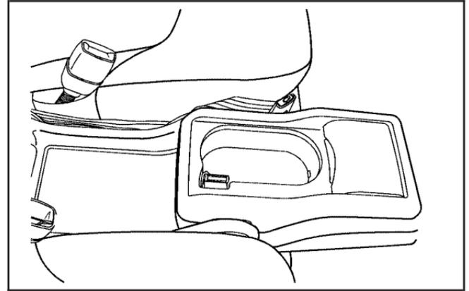
If your vehicle is the six-passenger model, there is a cupholder located underneath the seat. To access, pull the center seat forward. The cupholder has a support that adjusts to two positions to fit either a large cup or two smaller cups.
