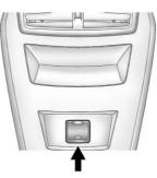
The power outlet is on the rear of the center console.
