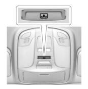
If equipped, the rear window sunshade button is on the overhead console. To open the sunshade, press and release. The sunshade will fully extend. To close the sunshade, press and release the switch again. The sunshade will fully close.
