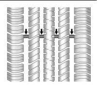
Treadwear indicators are one way to tell when it is time for new tires. Treadwear indicators appear when the tires have only 1.6 mm (1/16 in) or less of tread remaining. See *Tire Inspection*  $\Rightarrow$  277 and *Tire Rotation*  $\Rightarrow$  277.
