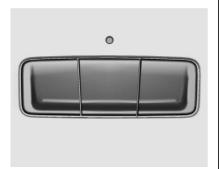
If equipped, these buttons in the overhead console provide a way to replace up to three remote control transmitters used to activate devices such as garage door openers, security systems, and home automation devices.
