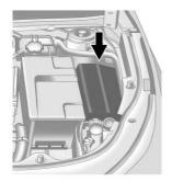
To remove the fuse block cover, squeeze the three retaining clips on the cover and lift it straight up.
