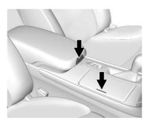
There is storage in the center console armrest. Press the button to access. Depending on the options, there may be an accessory power outlet, auxiliary jack, USB port(s), and a transmitter pocket inside. See *Power Outlets*  $\Rightarrow$  *103* and the infotainment manual.
