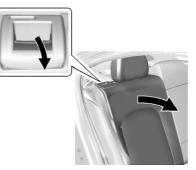
1. Pull on the lever on the top of the seatback to unlock it.
