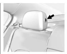
The head restraint can be folded rearward to allow for better visibility when the rear seat is unoccupied. To fold the head restraint, press the button on the side of the head restraint.
