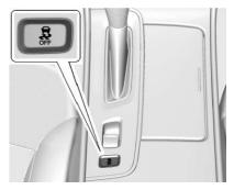
The TCS/StabiliTrak button is on the center console.
