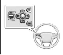
**(On/Off) :** Press to turn the system on or off. The indicator turns white on the instrument cluster when ACC is turned on.
