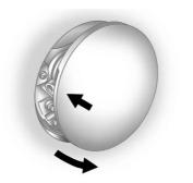
The fuel cap is behind a hinged fuel door on the passenger side of the vehicle. To open the fuel door, push and release the rearward center edge of the door. If equipped, the fuel door is locked when the vehicle doors are locked. Press an on the RKE transmitter to unlock.
