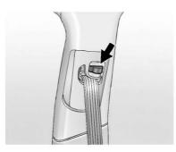
Press the release button and move the height adjuster to the desired position. The adjuster can be moved up by pushing the slide/trim up. After the adjuster is set to the desired position, try to move it down without pushing the release button to make sure it has locked into position.
