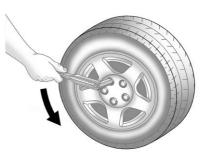
Turn the wheel wrench counterclockwise to loosen all of the wheel nuts, but do not remove them yet.
