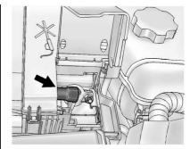
The vehicle has a remote positive (+) terminal under a trim cover. It is under the battery cover on the driver side of the engine compartment. See *Engine Compartment Overview*  $\Leftrightarrow$  231. You should always use this remote positive terminal.
