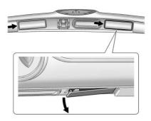
2. Push the end on either of the lamp assemblies (passenger side shown) and then move the lamp assembly down to remove it from the trunk lid.
