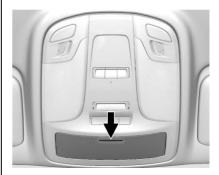
If equipped, press the cover and release to access.
