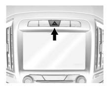
(Hazard Warning Flashers) : Press this button on the center stack above the audio system, to make the front and rear turn signal lamps flash on and off. Press again to turn the flashers off.
