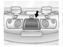
The cold air intake for the battery is located behind the rear seat, on the filler panel. Do not cover the intake. See *Battery* - *North America*  $\Rightarrow$  250.
