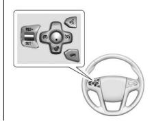
O (On/Off) : Press to turn cruise control on or off. A white indicator comes on in the instrument cluster.
