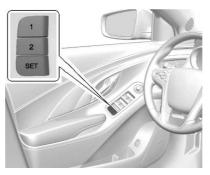
If memory equipped, the 1, 2. and SET buttons on the driver door are used to manually store and recall the driver seat and outside mirror positions.
