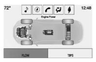
Engine Power – Engine is active with energy flowing to the wheels.
