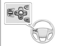
S : Press to turn cruise control on or off. A white indicator comes on in the instrument cluster.
