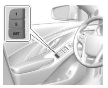
If equipped, the 1, 2, and SET buttons on the driver door are used to manually store and recall the driver seat, and outside mirror positions.
