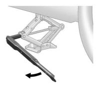
6. Turn the jack handle clockwise to raise the vehicle far enough off the ground for the compact spare to fit under the vehicle.
