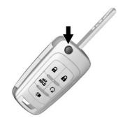
Press the button on the RKE transmitter to extend the key. Press the button and the key blade to retract the key.
