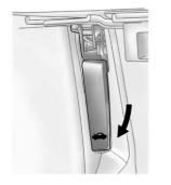
1. Pull the interior hood release handle located to the left of the steering column below the instrument panel.
