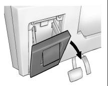
Pull up on the handle and pull the cover down to open.
