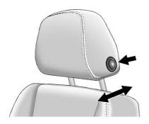
To adjust the head restraint forward or rearward, press the button located on the side facing of the head restraint and move it forward or rearward until the desired locking position is reached. Try to move the head restraint after the button is released to make sure that it is locked in place.
