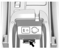
3. Place the new transmitter into the transmitter pocket inside the armrest storage area.
