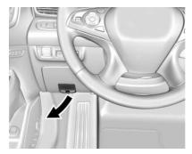
1. Pull the interior hood release handle located to the left of the steering column below the instrument panel.
