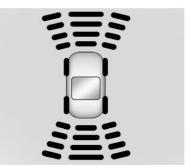
The instrument cluster may have a Park Assist display with bars that show "distance to object" and object location information for RPA, and on some vehicles, FPA. As the object gets closer, more bars light up and the bars change color from yellow to amber to red.
