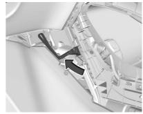
11. Pull the manual park release lever 90° to its latching position.
