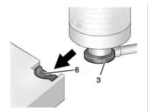
Slide the base of the tire sealant canister (3) into the slot on the top of the compressor (6) to hold it upright.
