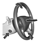
To adjust the steering wheel, if equipped:
