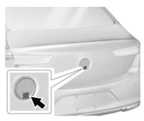
• Press the bottom of the emblem above the license plate when all doors are unlocked or when the transmitter is within 1 m (3 ft) of the rear of the vehicle.
