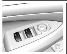
Power windows work when the ignition is on, in ACC/ACCESSORY, or when Retained Accessory Power (RAP) is active. See *Retained Accessory Power (RAP)* ⇔ *183*.
