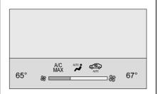
The climate control status display appears briefly when the center stack climate controls are adjusted.
