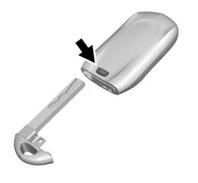
Press the button on back of the RKE transmitter to pull out the key. Never pull the key out without pressing the button.
