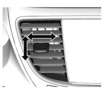
Use the slider knob on the air vent louvers to change the amount and direction of the airflow.
