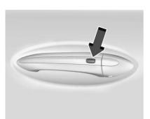
Press the lock/unlock button when the RKE transmitter is within 1 m (3 ft) of the driver door handle. When unlocking from the driver door, the first press unlocks that door; press again within five seconds to unlock all passenger doors. See *Remote Keyless Entry* (*RKE*) System Operation ⇔ 30. Driver Door Key Lock Cylinder Access (In Case of Dead Battery)
