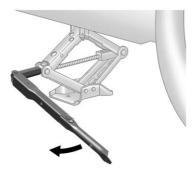
Raise the vehicle by turning the jack handle clockwise. Raise the vehicle far enough off the ground so there is enough room for the road tire to clear the ground.
