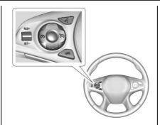
S: Press to turn cruise control on or off. A white indicator comes on in the instrument cluster.
