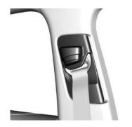
Press the release button and move the height adjuster to the desired position. The adjuster can be moved up by pushing the slide/trim up. After the adjuster is set to the desired position, try to move it down without pushing the release button to make sure it has locked into position.
