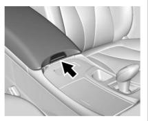
Push the storage compartment lid backward and pull up to open the storage compartment lid. Two USB ports and an auxiliary jack are inside.
