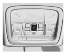
If equipped, the rear window sunshade switch is on the overhead console. To open the sunshade, press and release the switch. The sunshade will fully extend. To close the sunshade, press and release the switch again. The sunshade will fully close. The sunshade only operates when the ignition is on or in ACC/ ACCESSORY.
