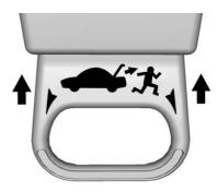
After pulling the emergency trunk release handle, push the handle back into the bezel.
