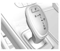
The shift pattern is displayed in the top of the shift lever. The selected gear position will illuminate red on the shift lever, while all others will be displayed in white. If the shift is not immediate, as in very cold conditions, the indicator on the shift lever may blink until it is fully engaged. The shift lever always starts from a center position, represented by an amber dot on the shift pattern. After releasing the shift lever, it will return to the center position.
