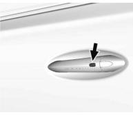
The RKE transmitter must be within 1 m (3 ft) of the door being opened.
