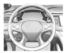
Vehicles with Tap Shift have controls on the back of the steering wheel to manually shift the automatic transmission. To enter Permanent Tap Shift Mode:
