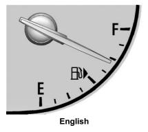
When the ignition is on, the fuel gauge indicates about how much fuel is left in the tank.
