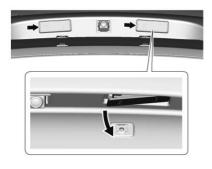
Push the lamp assembly toward the center of the vehicle, then move the lamp downward, and remove it from the vehicle body.
