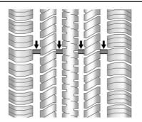
Treadwear indicators are one way to tell when it is time for new tires. Treadwear indicators appear when the tires have only 1.6 mm (1/16 in) or less of tread remaining. See *Tire Inspection*  $\Rightarrow$  282 and *Tire Rotation*  $\Rightarrow$  283.
