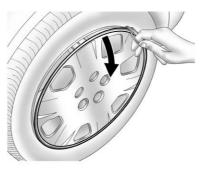
Take off the wheel cover or center cap, if the vehicle has one, to reach the wheel bolts.
