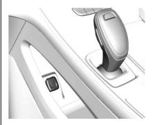
The 12-volt power outlets can be used to plug in electrical equipment, such as a cell phone or MP3 player.
