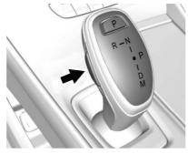
This vehicle is equipped with an electronic transmission. The shift lock release button is designed to prevent shifting out of P (Park), unless the ignition is on, the brake pedal is applied, and the shift lock release button is pressed.
