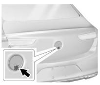
Press the bottom of the emblem above the license plate when all doors are unlocked.
