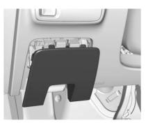
The instrument panel fuse block is in the instrument panel, on the driver side of the vehicle. To operate the fuses, open the fuse panel by pulling down at the top.
