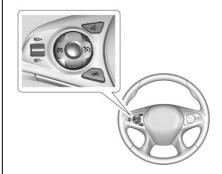
$\mathfrak{G}$ : Press to turn cruise control on or off. A white indicator comes on in the instrument cluster.
