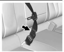
2. Disconnect the rear seat belt mini-latch, using a key in the slot on the mini-buckle.
