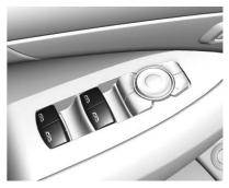
All windows can be opened without holding the window switch. Press the switch down fully and quickly release to express open the window.
