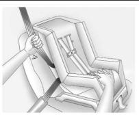
6. To tighten the belt, push down on the child restraint, pull the shoulder portion of the belt to tighten the lap portion of the belt, and feed the shoulder belt back into the retractor. When installing a forward-facing child restraint, it may be helpful to use your knee to push down on the child restraint as you tighten the belt.
