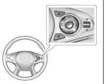
Use the right steering wheel control to open and scroll through the different items and displays.
