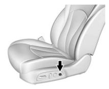
If equipped, press the massage button to use the massage feature. To stop massage, press this button again.
