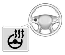
If equipped, press to turn on or off. A light near the button displays when the feature is turned on.
