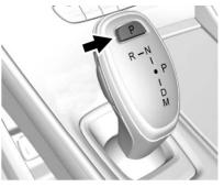
2. Press the P button on the shift lever.
