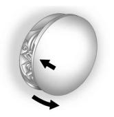
To open the fuel door, push and release the rearward center edge of the door.
