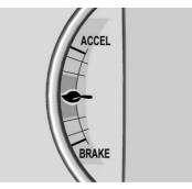
This gauge is a guide to driving in an efficient manner and will vary based on driver input. To maximize efficiency, keep the leaf in the solid green zone in the center of the gauge. The leaf moves down when braking and up when accelerating. When either is done aggressively, the vehicle is being driven less efficiently and the gauge will move further from the center.
