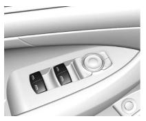
Power windows work when the ignition is on, in ACC/ACCESSORY, or when Retained Accessory Power (RAP) is active. See *Retained Accessory Power (RAP)* \$\dots\$ 183.
