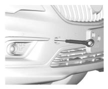
Install the tow eye into the socket by turning it clockwise until it stops in a horizontal position.
