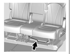
To adjust the seat position, lift the lever below the seat cushion and slide the seat forward or backward.
