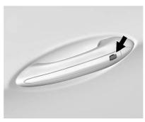
If equipped with Keyless Access, the RKE transmitter must be within 1 m (3 ft) of the door being opened. Press the button on the door handle to open. The liftgate is also unlocked when the RKE transmitter is within range of the liftgate handle. Press the touch pad underneath the handle and lift.
