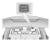
Press on the bottom of the liftgate next to the pull cup to close. Press any liftgate button or the touch pad while the liftgate is moving to stop it. Pressing again restarts the operation in the reverse direction. The touch pad on the liftgate handle cannot be used to close the liftgate.
