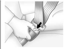
To unlatch the belt, push the button on the buckle. The belt should return to its stowed position. Slide the latch plate up the safety belt webbing when the safety belt is not in use. The latch plate should rest on the stitching on the safety belt, near the guide loop on the side wall.
