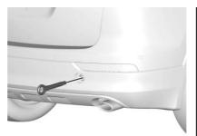
Install the tow eye into the socket by turning it clockwise until it stops in a horizontal position.
