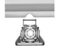
Locate the notch on the sheet metal weld flange. Place the center of the jack lift head on the center of the sheet metal notch.
