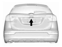
To open the liftgate, press on the power door lock switch or press on the Remote Keyless Entry (RKE) transmitter twice to unlock all doors. Press the touch pad on the underside of the liftgate handle and lift up. See Remote Keyless Entry (RKE) System Operation ⇒ 26.
