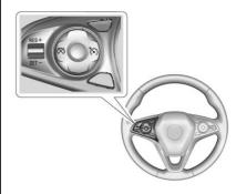
(S): Press to turn cruise control on or off. A white indicator comes on in the instrument cluster when the cruise is turned on.
