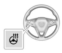
**3**: If equipped with a heated steering wheel, press to turn on or off. A light near the button displays when the feature is turned on.
