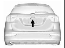
To open the liftgate, press on the power door lock switch or press on the RKE transmitter twice to unlock all doors. Press the touch pad on the underside of the liftgate handle and lift up.
