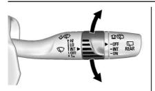
**INT :** Use for intermittent wipes. To adjust wipe frequency, turn the band up for more frequent wipes or down for less frequent wipes. If the vehicle has Rainsense, see the following Rainsense information.
