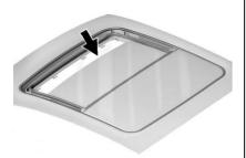
Dirt and debris may collect on the sunroof seal or in the track. This could cause an issue with sunroof operation or noise. It could also plug the water drainage system. Periodically open the sunroof and remove any obstacles or loose debris. Wipe the sunroof seal and roof sealing area using a clean cloth, mild soap, and water. Do not remove grease from the sunroof. If water is seen dripping into the water drainage system, this is normal.
