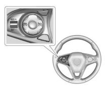
(C): Press to turn cruise control on or off. A white indicator comes on in the instrument cluster when the cruise is turned on.
