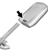
Press this button to remove the key. The key can be used to open the driver door.
