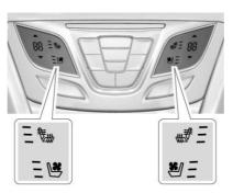
If equipped, the buttons are near the climate controls. To operate, the engine must be running.
