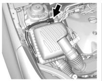
Open the hood and unwrap the electrical cord. The cord is in the passenger side of the engine compartment, near the air filter. It is shipped from the factory with a tie holding it in place. Use care in removing the tie so that the cord is not damaged.
