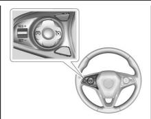
• Press to turn cruise control on or off. A white indicator comes on in the instrument cluster when cruise control is turned on.
