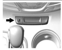
To turn off only TCS, press and release  $\frac{1}{64}$ . The traction off light  $\frac{1}{62}$  illuminates in the instrument cluster.
