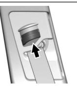
Move the height adjuster up to the desired position by pushing up on the height adjuster.
