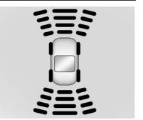
The instrument cluster may have a park assist display with bars that show "distance to object" and object location information for RPA, and on some vehicles, FPA. As the object gets closer, more bars light up and the bars change color from yellow to amber to red.
