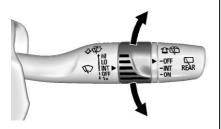
**INT :** Use for intermittent wipes or Rainsense, if equipped and enabled. To adjust wipe frequency, turn the band up for more frequent wipes or down for less frequent wipes. If Rainsense is enabled, see "Rainsense" later in this section.
