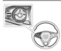
$\overline{85}$ : Press to turn the system on or off. A white cruise control indicator comes on in the instrument cluster.
