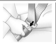
To unlatch the belt, push the button on the buckle. The belt should return to its stowed position. Slide the latch plate up the seat belt webbing when the seat belt is not in use. The latch plate should rest on the stitching on the seat belt, near the guide loop on the side wall.
