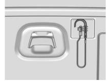
Use the hook underneath to hold open the cargo floor cover.
