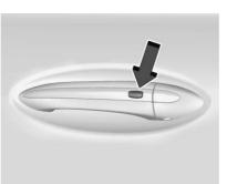
The RKE transmitter must be within 1 m (3 ft) of the liftgate or door being opened. Press the button on the door handle to unlock. See "Keyless Access Operation" in *Remote Keyless Entry (RKE) System Operation* ⇔ 28. Driver Door Key Lock Cylinder Access (In Case of Dead Battery)
