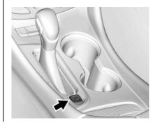
The Electric Parking Brake (EPB) switch is on the center console. The EPB can always be activated, even if the ignition is off. To prevent draining the battery, avoid repeated cycles of the EPB when the engine is not running.
