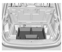
The cargo management system is used to store items in the cargo area under the load cover.
