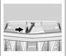
Go to the front of the vehicle to find the secondary release handle. The handle is under the front edge of the hood near the center. Push the handle to the right and at the same time raise the hood.
