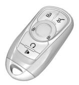
**\widehat{\mathbf{O}}**: Press to lock all doors. The turn signal indicators may flash and/or the horn may sound on the second press to indicate locking. See *Vehicle Personalization*  $\Rightarrow$  150. If a passenger door is open when  $\widehat{\mathbf{O}}$  is pressed, all doors lock. If the driver door is open when  $\widehat{\mathbf{O}}$  is pressed, all doors lock except the driver door. These settings can be modified. See *Vehicle Personalization*  $\Rightarrow$  150.
