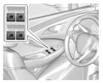
Power windows work when the ignition is on, in ACC/ACCESSORY, or when Retained Accessory Power (RAP) is active. See *Retained Accessory Power (RAP)* ⇔ 194.
