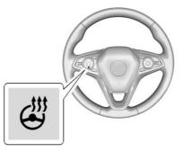
If equipped with a heated steering wheel, press to turn on or off. A light near the button displays when the feature is turned on. The steering wheel takes about three minutes to start heating.
