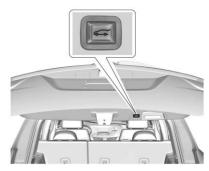
Press any liftgate button or the touch pad while the liftgate is moving to stop it. Pressing again restarts the operation in the reverse direction. The touch pad on the liftgate handle cannot be used to close the liftgate.
