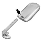
1. Press the button on the transmitter to access the key.
