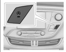
The automatic engine stop/start feature can be disabled and enabled by pressing the switch with the (A) symbol. Auto Stop is enabled each time you start the vehicle.
