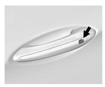
The RKE transmitter must be within 1 m (3 ft) of the door being opened. Press the button on the door handle to unlock. The liftgate is also unlocked when the RKE transmitter
