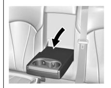
If equipped, the rear seat has an armrest in the center of the seatback. Lower the armrest to access the cupholders.
