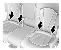
The lower anchors are behind the horizontal openings in the seat cushion trim located below the anchor label. Seating positions with top tether anchors.
