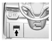
There is storage next to the steering wheel. Lift the handle to access.
