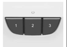
If equipped, this system provides a way to replace up to three remote control transmitters used to activate devices such as garage door openers, security systems, and home automation devices.
