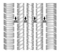
Treadwear indicators are one way to tell when it is time for new tires. Treadwear indicators appear when the tires have only 1.6 mm (1/16 in) or less of tread remaining. See *Tire Inspection*  $\Rightarrow$  291 and *Tire Rotation*  $\Rightarrow$  291.
