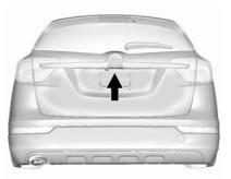
To open the liftgate, press a on the power door lock switch or press a on the RKE transmitter twice to unlock all doors. Press the touch pad on the underside of the liftgate handle and lift up.
