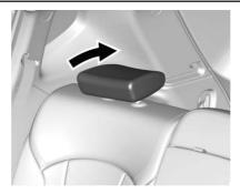
The rear outboard head restraints are designed to be folded. The head restraint can be folded backward to allow for better visibility when the rear seat is unoccupied. To fold the head restraint, press the button on the side of the head restraint. Seats and Restraints 55
