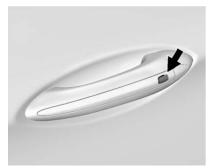
Driver Side Shown, Passenger Side Similar Pressing the lock/unlock button will cause all doors to lock if any of the following occur:
