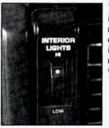
You can brighten or dim the instrument panel lamps by rotating the control up or down. To turn on the interior courtesy lamps, rotate the control all the way up to HI.
