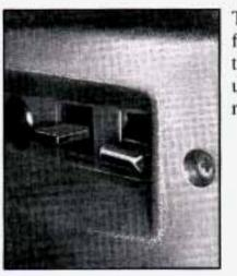
The switch is located on the front of the seat. To recline the seatback hold the switch up. Hold the switch down to raise the seatback.
