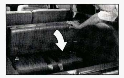
Pull the seatback toward the rear of the vehicle, then push it down to the locked position.
