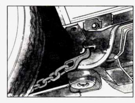
Attach T-hook chains behind the front wheels into the bottom of the floor pan on both sides.
