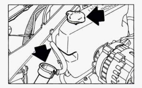
Put the cap back on the coolant recovery tank, but leave the radiator pressure cap off.
