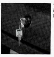
To unlock the trunk from the outside, insert the door key and turn it clockwise.
