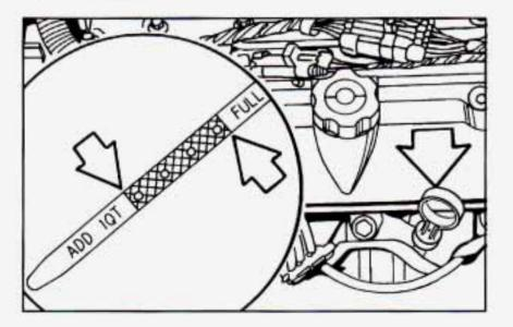
The 3100 V6 engine oil dipstick is located near the front and center of the engine compartment. 2.2L L4 Engine
