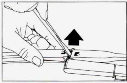
Replacement blades come in different types and are removed in different ways. Here's how to remove the type with a spring release:
