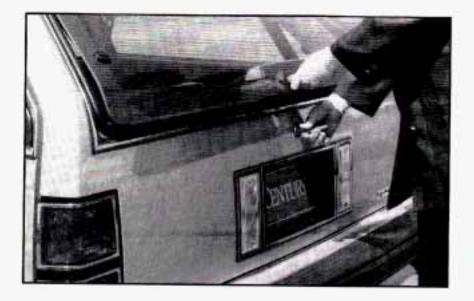
Turn the key to the left to release the liftgate glass. Then, pull the glass up by the handle. To close, lower the glass until the latch catches.
