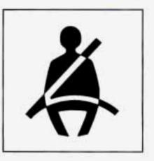
When the key is turned to RUN or START a chime will come on for about eight seconds to remind people to fasten their safety belts, unless the driver's safety belt is already buckled. The safety belt light will also come on and stay on for about 20 seconds, then it will flash for about 55 seconds. If the driver's belt is already buckled, neither the chime nor the light will come on.
