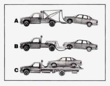
Try to have a GM dealer or a professional towing service tow your Buick. The usual towing equipment is a sling-type (A) or a wheel-lift (B) or car carrier (C) tow truck. If your vehicle has been changed or modified since it was factory-new by adding aftermarket items like fog lamps, aero skirting, or special tires and wheels, these instructions and illustrations may not be correct.
