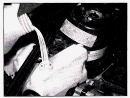
Then fill the coolant recovery tank to the FULL HOT mark.
