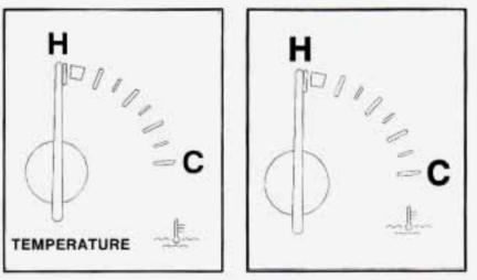
This gage shows the engine coolant temperature. If the gage pointer moves into the red area, your engine is too hot!
