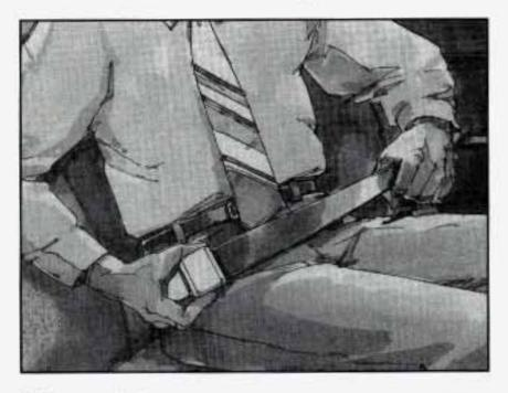
When you sit in a center seating position or in a station wagon third seat, you have a lap safety belt, which has no retractor. To make the belt longer, tilt the latch plate and pull it along the belt.
