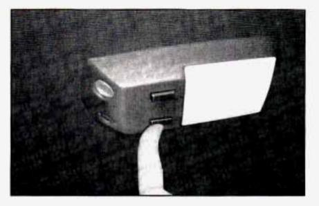
Press the switch to turn the front seat reading lamps on or off.
