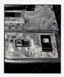
Press the power door lock switch on either front door to lock or unlock all the doors at once.
