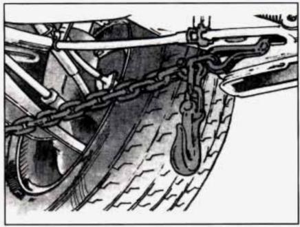
Attach T-hook chains on both sides in the slotted holes in the floor pan just ahead of the rear wheels.
