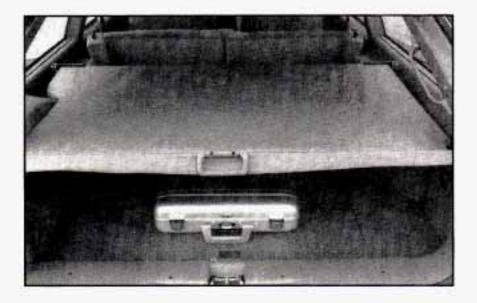
To Use the Cover: Grasp the handle and pull the cover over the rear storage area. Insert the ends of the support rod into the slots in the trim panel near the liftgate.
