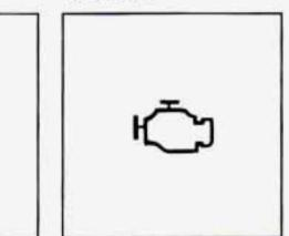
Your vehicle is equipped with either an amber SERVICE ENGINE SOON light or an amber engine symbol light.
