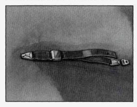
To use a child restraint here, you will need a special infant/child seat attaching belt and the hardware that goes with it. See the earlier part about the top strap if the child restraint has one. Your dealer can order the belt and attaching hardware and install the hardware for you. It's free. The special belt is GM Part No. 12340286. Your dealer can find the part number for the correct attaching hardware in the accessory section of the GM Parts Catalog.
