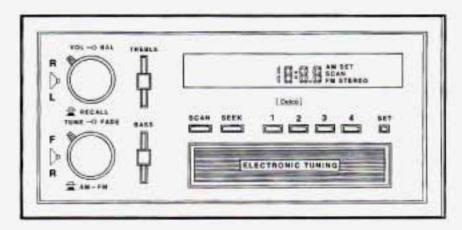
The digital display indicates information on time or radio station frequency, the AM or FM radio band, whether the station is in stereo, and other radio functions.
