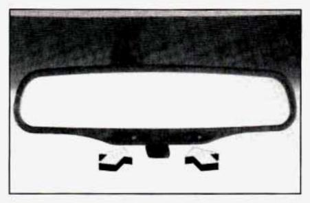
Press the switches on the front of the mirror to turn on the reading lamps.
