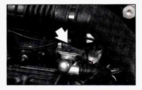
The 2.2L (VIN Code 4) has one bleed valve located at the thermostat housing.
