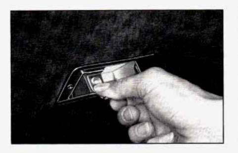
To clean the rear ashtrays, fully open the ashtray. Press down on the snuffer as you pull the ashtray down and out.
