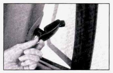
To open, pull the latch forward, then push on the center of the latch to swing the window out into the open position.
