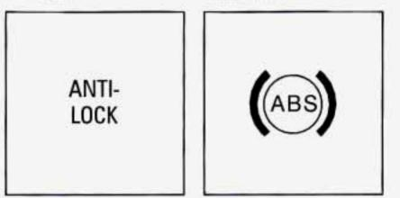
With the anti-lock brake system, this light will come on when you start your engine and it will stay on for three seconds. That's normal. If the light doesn't come on, have it fixed so it will be ready to warn you if there is a problem.
