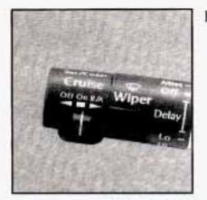
Move the cruise control switch to ON.
