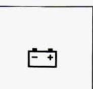
The red battery warning light is designed to come on briefly when you turn on the ignition, but the engine is not running, as a check to show you it is working.
