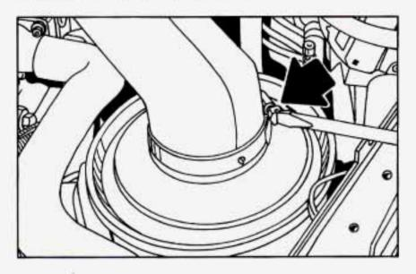
Use a screwdriver to loosen the hose clamp, then lift the rubber duct.
