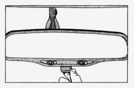
When you are sitting in a comfortable driving position, adjust the mirror so you can see clearly behind you car. The day-night adjustment allows you to reduce glare from lights behind you, pull the lever toward you to the night position.
