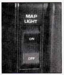
Press the switch to turn the map lamp on and off.
