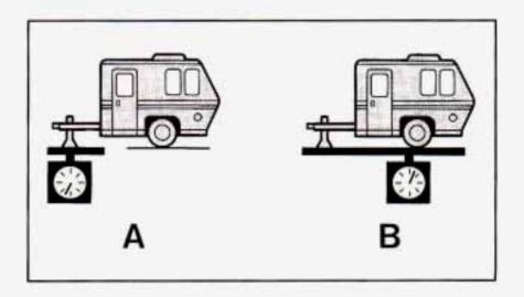
If you're using a "dead-weight" hitch, the trailer tongue (A) should weigh 10% of the total loaded trailer weight (B). If you have a "weight-distributing" hitch, the trailer tongue (A) should weigh 12% of the total loaded trailer weight (B).
