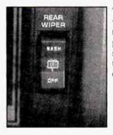
The rear window washer/wiper switch is at the center of the instrument panel. Press the top of the switch labeled WASH and the rear wiper will run at a constant speed.
