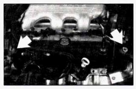
3.1L V6 (VIN Code M): There are two bleed valves. One is located on the thermostat housing. The other is located on the thermostat bypass tube.
