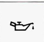
If you have a problem with your oil, this red oil pressure warning light may stay on after you start your engine, or come on when you are driving. Stop your vehicle and shut off the engine if this light stays on.
