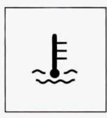
This red warning light is designed to tell you that your engine coolant has overheated or your radiator cooling fan is not working.
