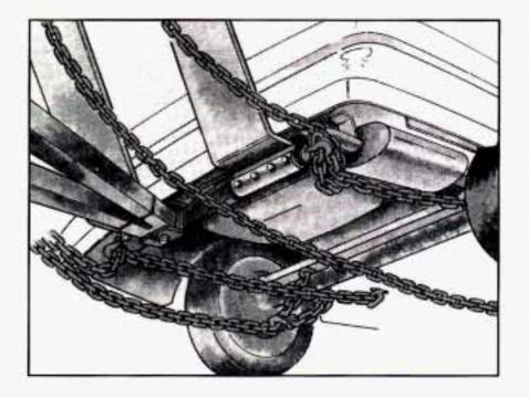
Position the lower sling crossbar directly under the rear bumper.
