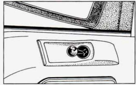
Use the remote control knob on the driver's door to adjust the driver's outside mirror. Adjust the passenger's outside mirror by hand.
