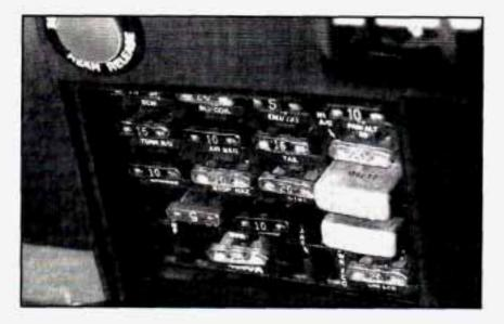
The wiring circuits in your vehicle are protected from short circuits by a combination of fuses, circuit breakers, and fusible thermal links in the wiring itself. This greatly reduces the chance of damage caused by electrical problems. The fuse panel is located inside the glove box, on the left side.
