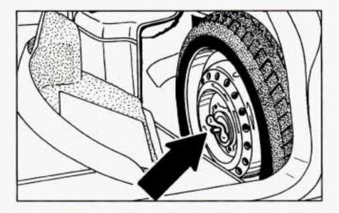
Remove the wing nut from the center of the spare tire and remove the adapter.
