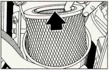
Remove and replace the filter. Replace the cover, wing nut and rubber duct. Tighten the hose clamp.
