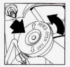
Then keep turning the pressure cap, but now push down as you turn it. Remove the pressure cap.
