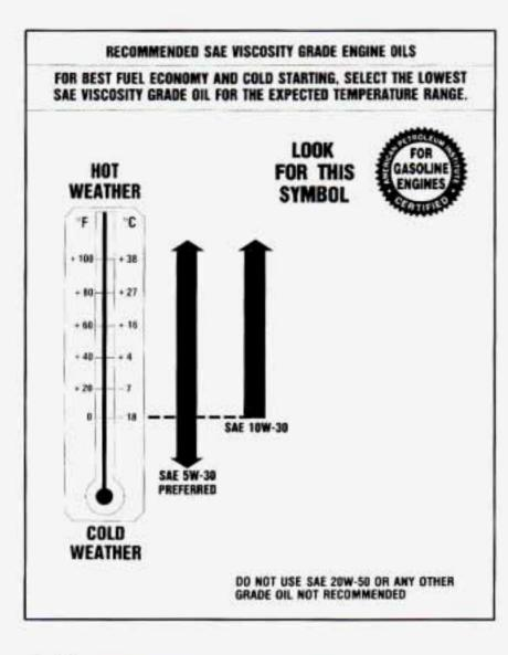
As shown in the chart, SAE 5W-30 is best for your vehicle. However, you can use SAE 10W-30 if it's going to be 0°F (-18°C) or above. These numbers on an oil container show its viscosity, or thickness. Do not use other viscosity oils, such as SAE 20W-50.
