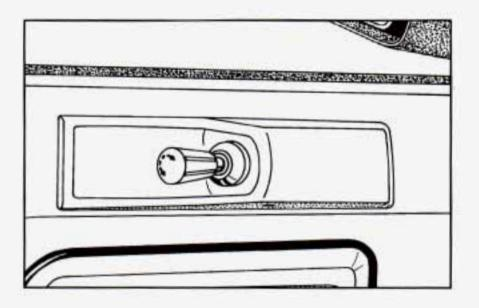
Turn the knob left or right to select the driver's or passenger's mirror. Rotate the knob to adjust the mirror.
