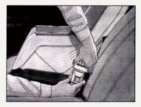
To tighten the belt, pull the shoulder belt while you push down on the child restraint.
