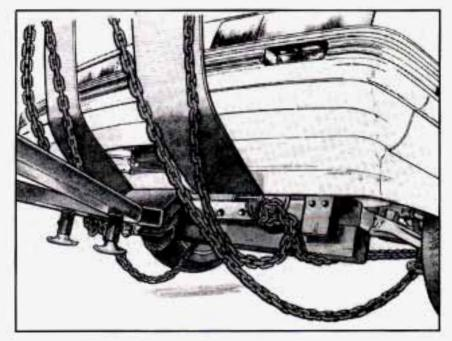
Position the lower sling crossbar halfway between the timber and the lower edge of the fascia.
