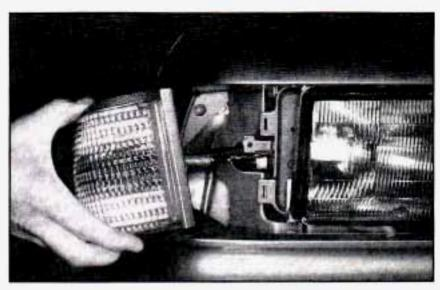
The bulb assembly is now loose. Pull it forward until the bulb assembly can be reached. To replace the turn/park bulb:
