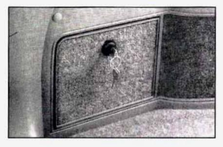
Use your door key to unlock the storage bin on the driver's side near the liftgate.
