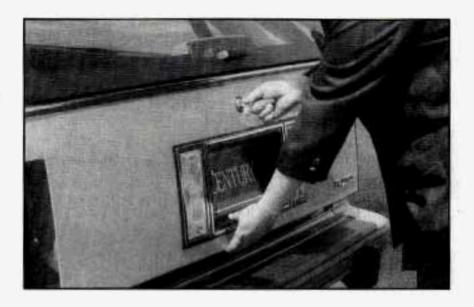
Turn the key to the right to unlatch the liftgate, then pull up on the bottom of the liftgate. To close, pull down on the handle inside the liftgate, then firmly shut the liftgate.
