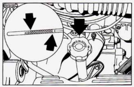
The 2.2L L4 engine oil dipstick is located in the fill cap near the front and center of the engine compartment.
