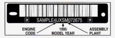
This is the legal identifier for your Buick. It appears on a plate in the front corner of the instrument panel, on the driver's side. You can see it if you look through the windshield from outside your vehicle. The VIN also appears on the Vehicle Certification and Service Parts labels and the certificates of title and registration.
