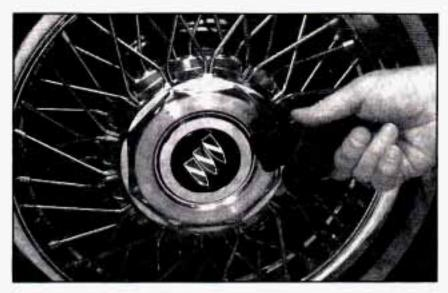
Removing the wire wheel cover requires this wire wheel key wrench.
