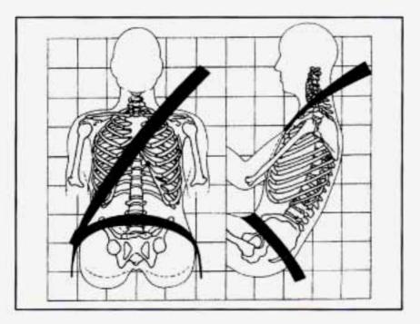
The lap belt should be worn as low on the hips as possible. In a crash, this applies force to the strong pelvic bones. And you'd be less likely to slide under the lap belt. If you slid under it, the belt would apply force at your abdomen. This could cause serious or even fatal injuries. The shoulder belt should go over the shoulder and across the chest. These parts of the body are best able to take belt restraining forces. The safety belt locks if there's a sudden stop or a crash.
