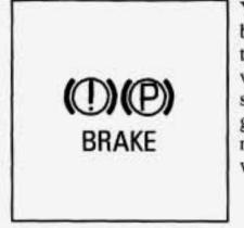
Your Buick's hydraulic brake system is divided into two parts. If one part isn't working, the other part can still work and stop you. For good braking, though, you need both parts working well.
