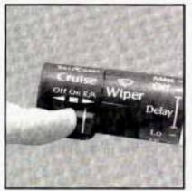
Once you're going about 25 mph (40 km/h) or more, you can move the cruise control switch from ON to R/A (Resume/Accelerate) for about half a second. You'll go right back up to your chosen speed and stay there.
