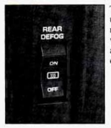
The rear window defogger uses a warming grid to remove fog from the rear window. In winter, it can also keep ice from forming on the rear window.
