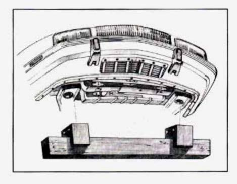
Position a 4" x 4" wood beam across sling chains with spacer blocks contacting the forward extensions of the engine cradle.
