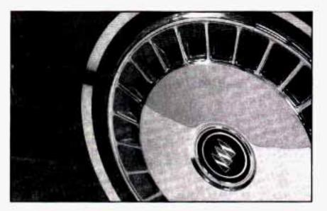
You will be using the flat end of the wheel wrench to remove the wheel cover. Pry along the edge of the wheel cover until it comes off.
