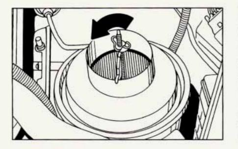
2. Remove the wing nut and pull off the cover.
