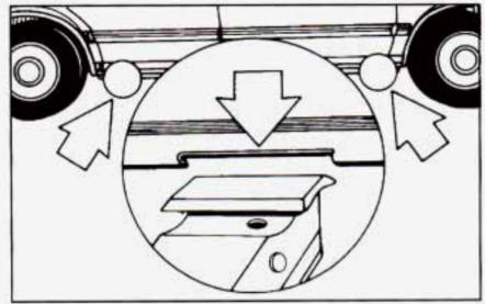
Position the jack under the vehicle nearest the tire to be changed. The jack location should be approximately five inches (12.7 cm) from the wheel well.
