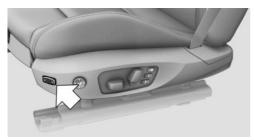
The width of the backrest can be changed with the side wings to adjust the side support to your own needs.
