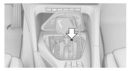
4. Using the screwdriver from the tool kit, refer to page 247, press the red lever while moving the selector lever to the desired position with the button pressed.
