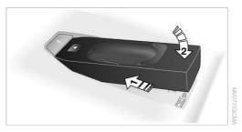
3. To remove the snap-in adapter: press button 1.
