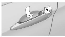
Grasp the handle on the driver's or front passenger door completely, arrow 1.
