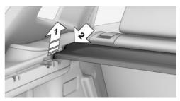
2. Pull the cover back, up and out of the lateral brackets on both sides, arrow 2.
