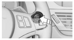
Pressing the Start/Stop button switches the ignition on or off and starts the engine.
