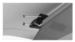
4. Attach the hooks 1 at the bottom of the retaining straps into the eyelets on the rear seat backrest, arrow, on both sides.
