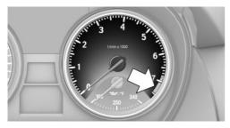
Never force the engine speed up into the red warning field, see arrow. In this range, the fuel supply is interrupted to protect the engine.
