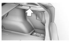
Hooks designed for hanging shopping bags and totes, for example, are located on the left and right sides of the cargo cover support, arrow.
