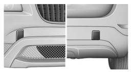
Press on the lower part of the cover. The cover is pushed out at the top edge and can be pulled out.
