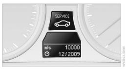
The remaining driving distance and the date of the next scheduled service are displayed briefly immediately after you start the engine or switch on the ignition. The current service requirements can be read out from the remote control by the service specialist.
