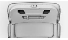
Recessed grips on the inside trim of the tailgate can be used to conveniently pull down the tailgate.
