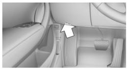
On the driver's side is an OBD socket for checking the primary components in the vehicle emissions.
