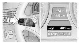
Press the computer button on the turn signal lever.
