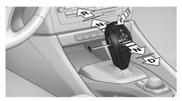
Briefly push the selector lever in the desired direction, beyond a resistance point if necessary. When shifting out of P or into R, simultaneously push the unlock button 1.
