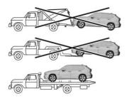
Towing a vehicle with xDrive Do not tow a vehicle with xDrive with just the front or rear axle raised; otherwise, the wheels could lock up and the transfer case could be damaged.
