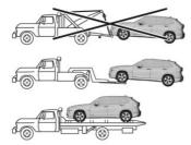
Have your vehicle transported with a tow truck with a so-called lift bar or on a flat bed.
