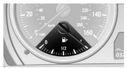
The vehicle inclination may cause the display to vary.
