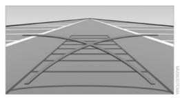
2. Turn the steering wheel to the point where the pathway line covers the corresponding turning circle line.
