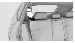
1. Reach into the recess and pull the lever toward the front. 2. Engage the backrest in the desired position or fold it down.
