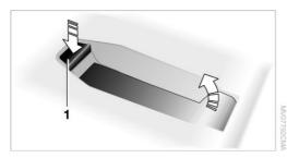
2. Insert the snap-in adapter at the front, arrow 1, and press down, arrow 2, until it engages.
