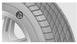
RSC label on the tire sidewall.
