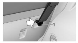
Lash the partition net tightly. To do this, tighten the retaining straps using the tensioning buckles.
