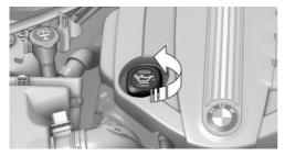
Add a maximum quantity of 1 US quart/1 liter of oil only after a corresponding message appears on the Control Display.
