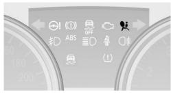
When the ignition is switched on,, refer to page 58, the warning lamp comes on briefly to indicate that the entire airbag
