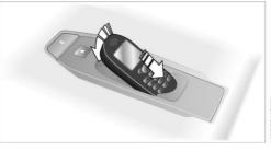
The battery is charged beginning with the radio ready state of the vehicle.
