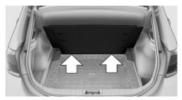
Reach under the cargo floor panel on the left, right and at the rear. Fold the panel up and forward, pressing it into the gap between the cargo area floor and the rear seat backrest.
