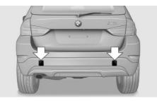
The anchorage points are under the covers in the bumper. Remove the covers, refer to page 260.
