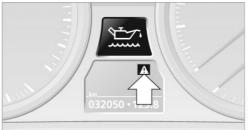
▲ The symbol indicates that Check Control messages have been stored. The Check Control messages can be displayed later.
