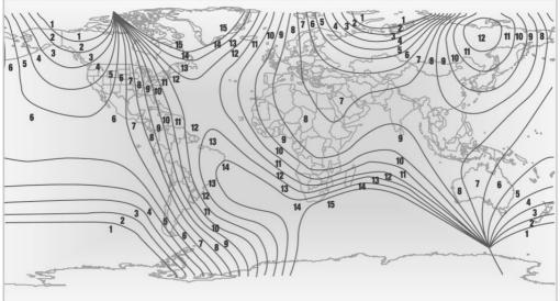
Press the adjustment button for 3-4 seconds. The number of the compass zone set is shown in the display.
