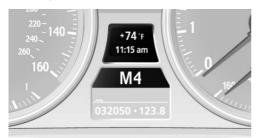
The transmission position is displayed and the engaged gear, such as M4, is displayed in manual mode.
