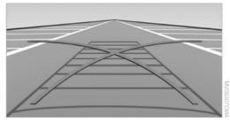
2. Turn the steering wheel to the point where the pathway line covers the corresponding turning circle line.
