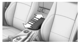
Slide the center armrest into the desired position.
