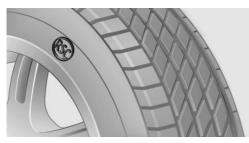
RSC label on the tire sidewall.
