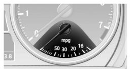
Displays the current fuel consumption. You can check whether you are currently driving in an efficient and environmentally-friendly manner.
