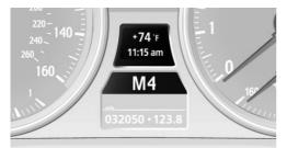
The selector lever position is displayed and the engaged gear, such as M4, is displayed in manual mode.
