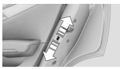
Push the locking lever on the rear doors down. The door can now be opened from the outside only.
