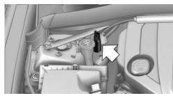
The so-called starting aid terminal in the engine compartment acts as the battery's positive terminal. Pull the cover up and off.
