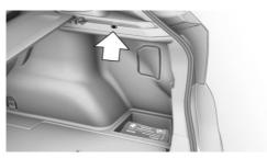
A multi-function hook is located on each side of the cargo area, arrow.
