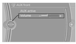
5. Turn the controller until the desired volume is set and press the controller.
