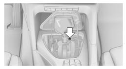
Using the screwdriver from the tool kit, refer to page 249, press the red lever while moving the selector lever to the desired position with the button pressed.
