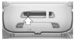
On the inside of the tailgate. To remove, press on the tab, arrow.
