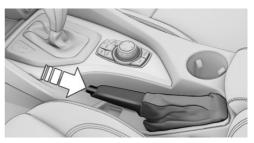
Pull up slightly, press the button, and lower the lever.
