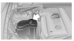
3. The filling level indicator 1 in the filler neck indicates the coolant level. The coolant level is correct if it is between the arrows of the respective reservoir label 2.
