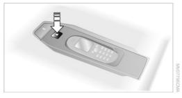
Press the button and remove the mobile phone.
