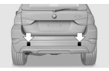
The anchorage points are under the covers in the bumper. Remove the covers, refer to page 262.
