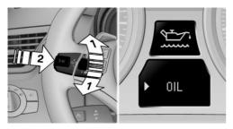
Press button 2 in the turn indicator lever. The oil level is checked and the reading displayed.
