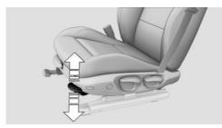
Pull the lever and apply your weight to the seat or lift it off, as necessary.
