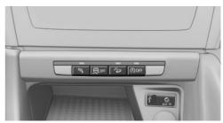
Press and hold the button, but not longer than approx. 10 seconds, until the indicator lamp for DSC lights up in the instrument cluster and DSC OFF is displayed. DTC Dynamic Traction Control and DSC are deactivated together.
