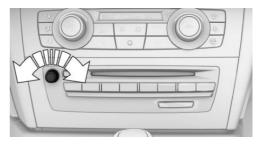
Turn the knob until the desired volume is selected. The setting is stored for the remote control currently in use.
