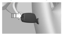
Press and hold button on signal lever.
