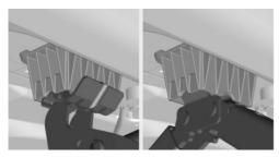
3. Extend the vehicle jack by turning the crank or lever clockwise.
