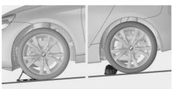
If you need to change a wheel on a slight downhill gradient, place chocks and other suitable objects, for example a rock, under the wheels of both the front and rear axles against the rolling direction.
