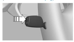
Press and hold button on signal lever. Information is displayed in the CID (central information display) of the instrument cluster.
