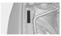
The vehicle identification number can be found in the engine compartment.
