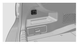
The socket is located on the left side in the cargo area.
