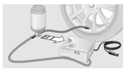
Screw the filling hose of the sealant container onto the tire valve of the nonworking wheel.
