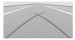
Turning radius lines can only be superimposed on the rearview camera image together with pathway lines.
