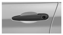
Unlock or lock the driver's door via the door lock using the integrated key.
