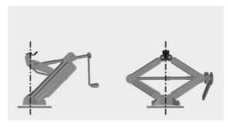
Make sure that the vehicle jack foot stands vertically and perpendicularly beneath the jacking point after extending the vehicle jack.
