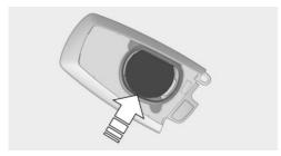
4. Insert a type CR 2450 battery with the positive side facing up.
