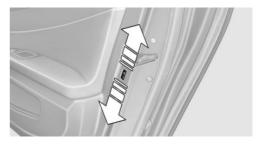
Push the locking lever on the rear doors down.
