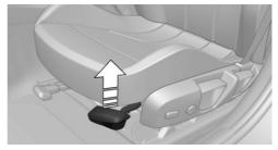
Pull the lever and move the seat to the desired tilt. After releasing the lever, apply your weight to the seat or lift it off to make sure the seat engages properly.
