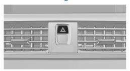
The button is located in the center console. The red light in the button flashes when the hazard warning flashers are activated.
