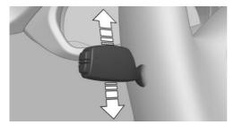
With the ignition switched off, press the lever either up or down past the resistance point for approx. 2 seconds.
