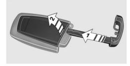
Push battery in the direction of the arrow using a pointed object and lift it out.
