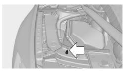
The body ground or a special nut acts as the battery negative terminal.
