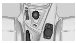
Press button repeatedly until the desired program is displayed in the instrument cluster.
