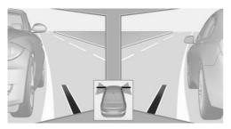
Guidelines at the bottom of the image show the position of the front of the vehicle.
