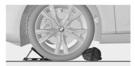
Place chocks or other suitable objects, for example a rock, in front of and behind the wheel that is diagonally opposite to the wheel that you wish to change.
