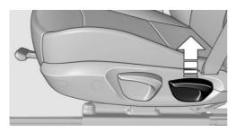
Pull the lever and apply your weight to the backrest or lift it off, as necessary.
