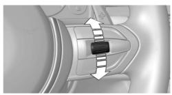
On the right side of the steering wheel, turn the thumbwheel to activate the corresponding list.
