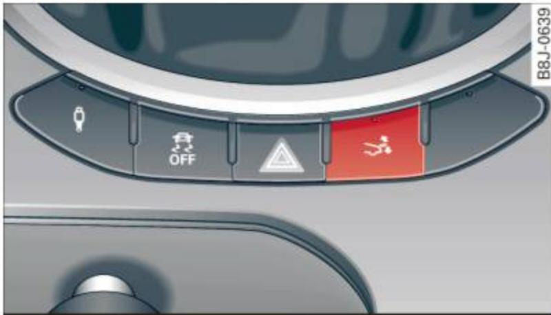
Fig. 128 Switch for rear spoiler
