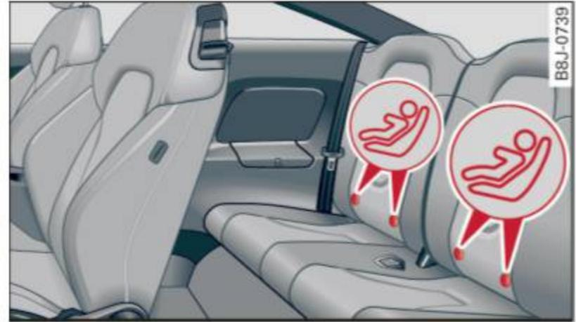
**Fig. 118** Rear seatbacks: locator buttons for lower anchorages
