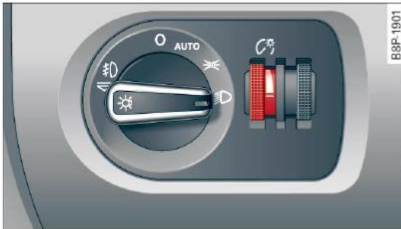
Fig. 46 Instrument panel illumination
