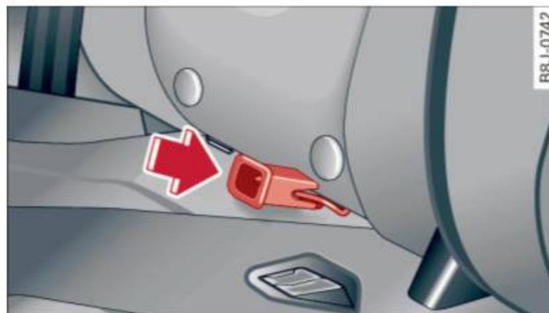
**Fig. 121** Close-up: fitting the guidance fixture over the lower anchorage bracket
