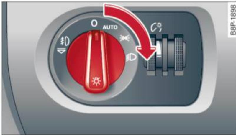
Fig. 39 Instrument panel: light switch
