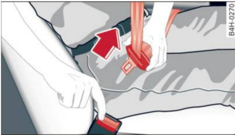
Fig. 103 Releasing the tongue from the buckle
