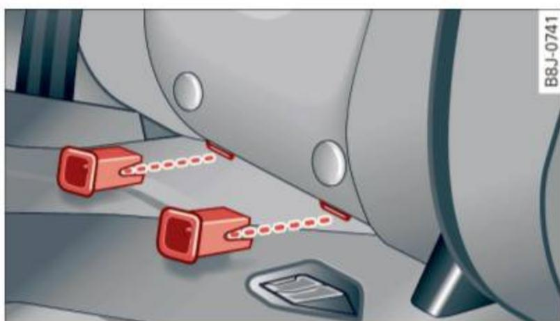
**Fig. 120** Rear seats: installing the guidance fixtures
