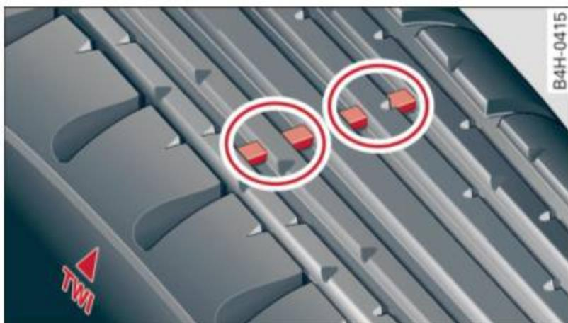
Fig. 144 Tire tread: tread wear indicators (TWI)
