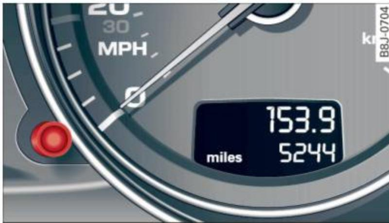
Fig. 5 Speedometer close-up: odometer display
