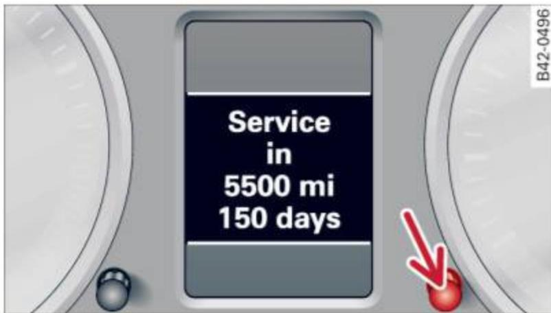
Fig. 19 Section of instrument cluster: Service interval display
