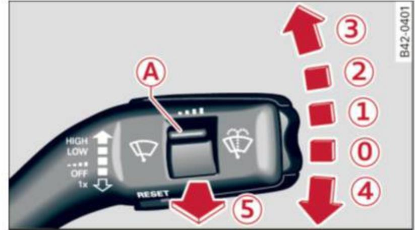
Fig. 50 Wiper lever: windshield wiper lever positions
