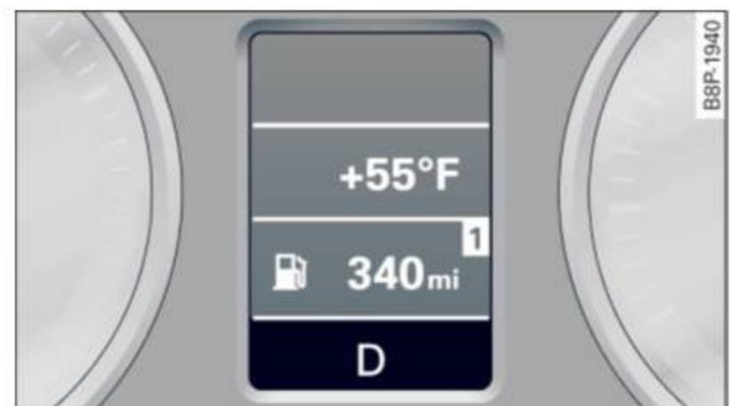
Fig. 80 Display: Selector lever position
