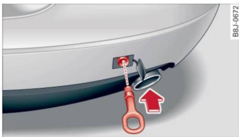
Fig. 175 Rear bumper: screwing in the towing loop
