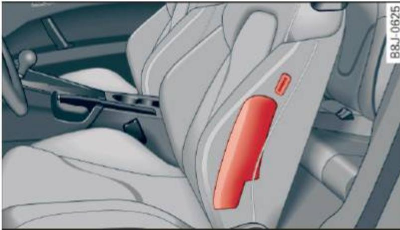
**Fig. 110** Side airbag location in the driver's seat
