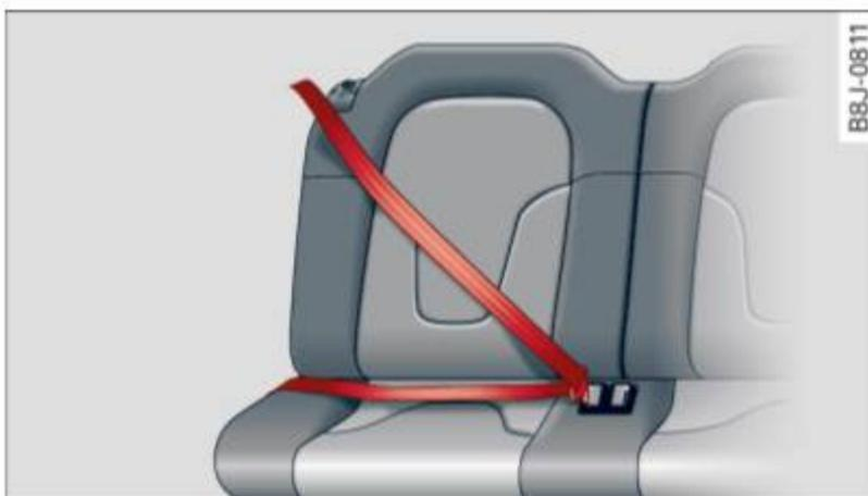
**Fig. 112** Schematic overview: keep unused safety belts away from children in child safety seats. - outer rear safety belt,
