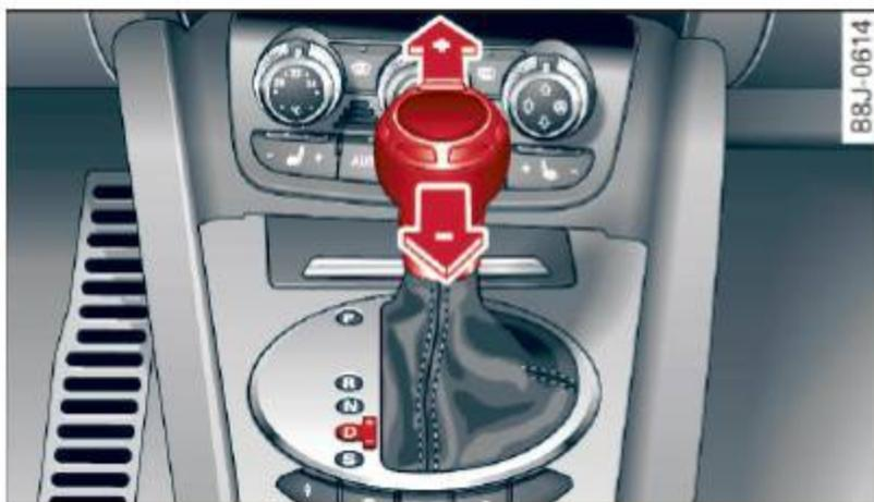
Fig. 83 Center console: Manual shifting (tiptronic)
