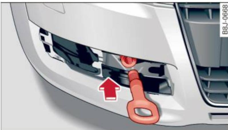
Fig. 171 Front bumper: screwing in the towing loop
