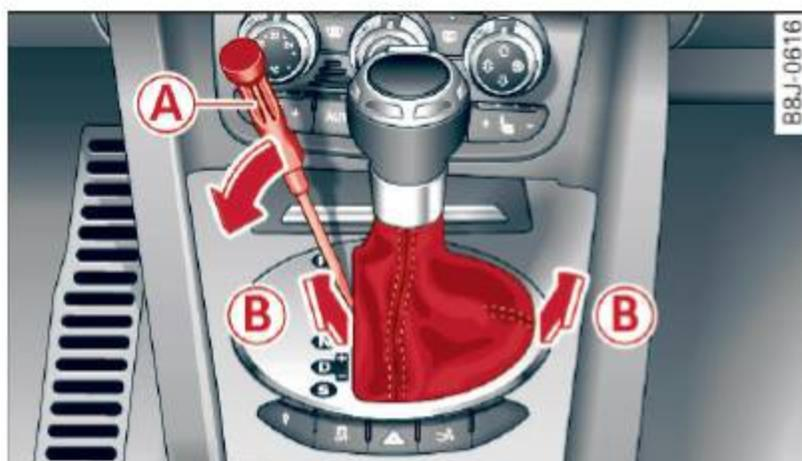
Fig. 86 Selector lever: Removing the selector lever boot
