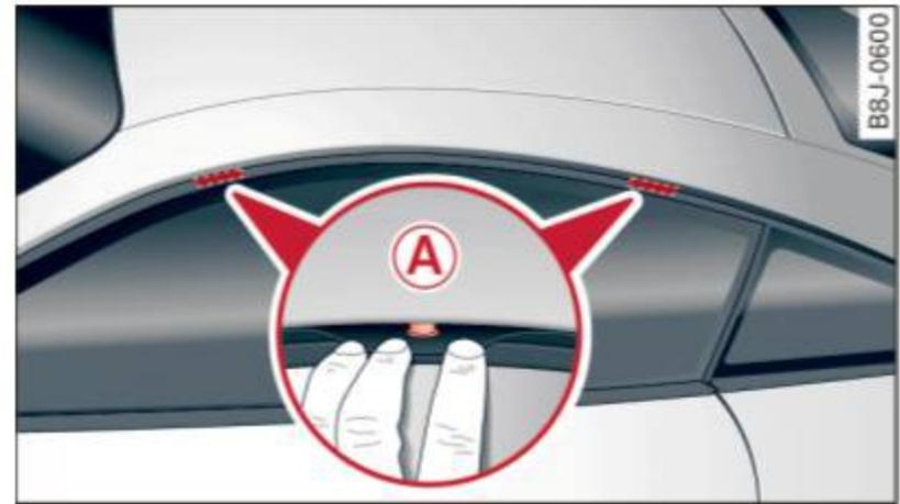
Fig. 62 Mounting locations for roof rack
