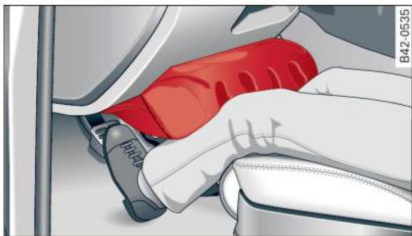
**Fig. 109** Inflated airbags protecting in a frontal collision
