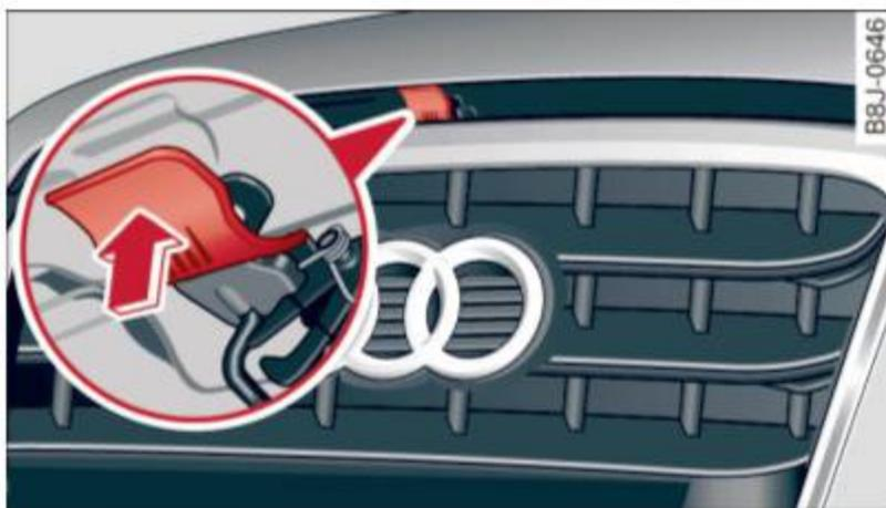
Fig. 133 Release lever under the engine hood
