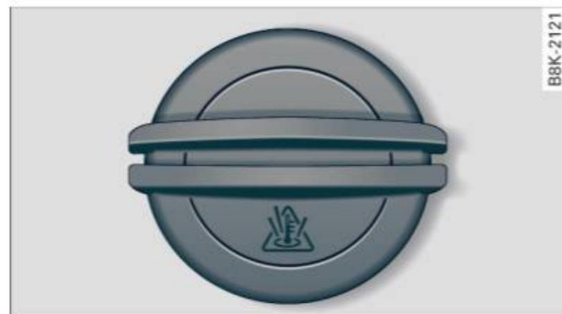
**Fig. 138** Engine compartment: cover on the coolant expansion tank
