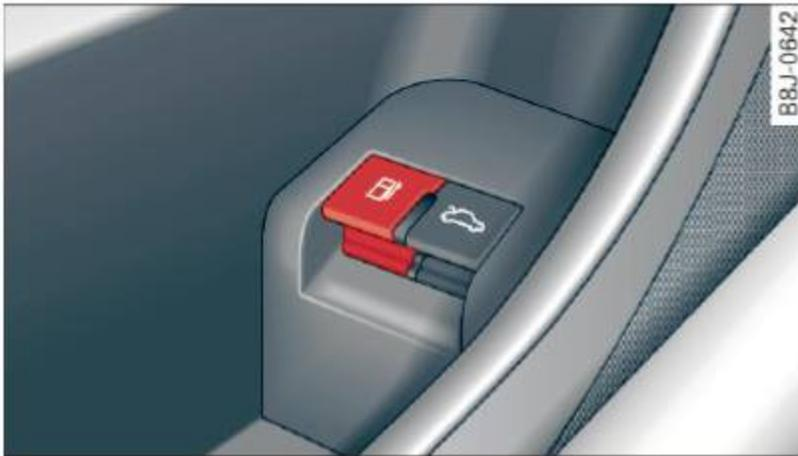
Fig. 129 Driver's door: Unlocking fuel filler flap
