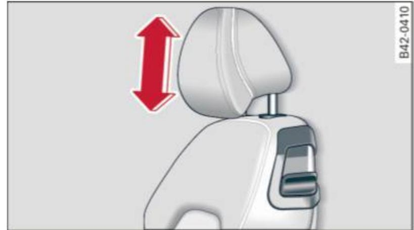
Fig. 57 Driver's seat head restraint: adjusting the height
