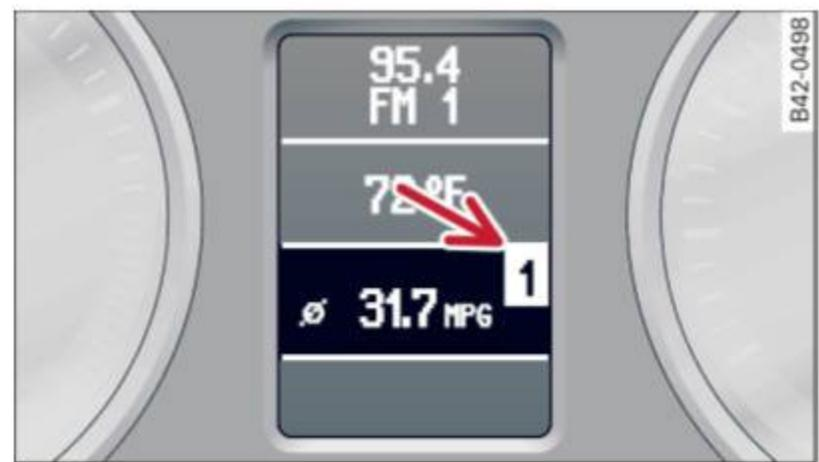
Fig. 9 Trip computer display: memory level 1
