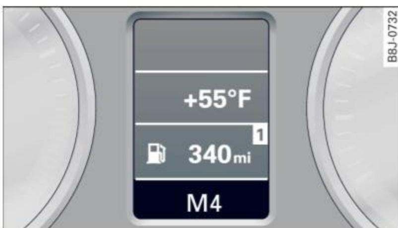
Fig. 84 Display: Manual shifting (tiptronic)
