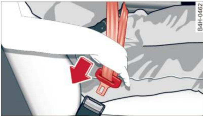
**Fig. 100** Belt buckle and tongue on the driver's seat
