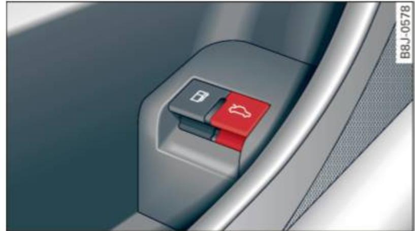
Fig. 32 Driver's door: remote rear lid release
