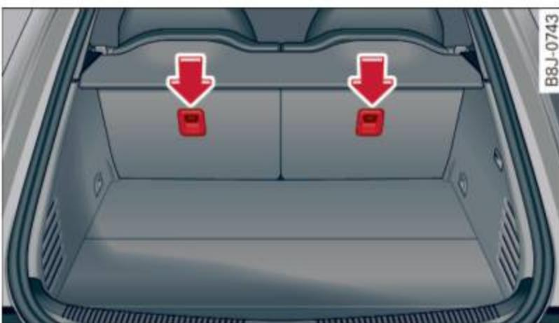
**Fig. 123** Tether anchors: attachment hook locations behind the rear seatbacks
