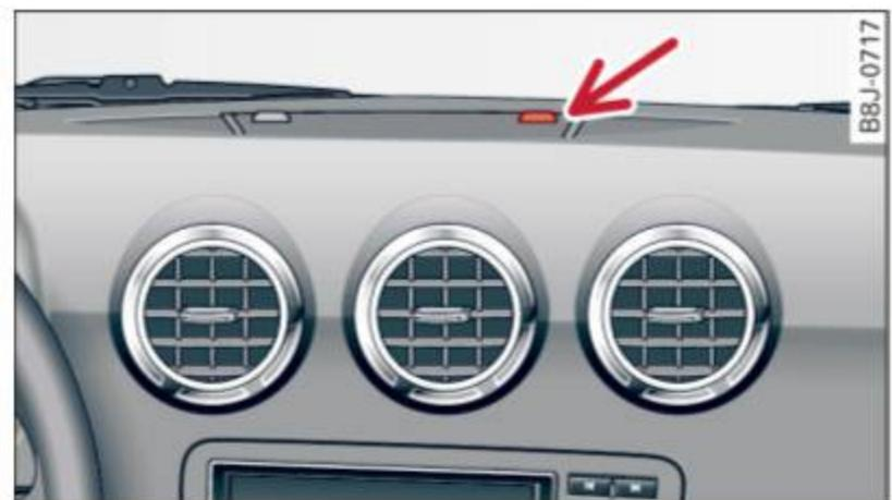
**Fig. 36** Diode position in the instrument panel
