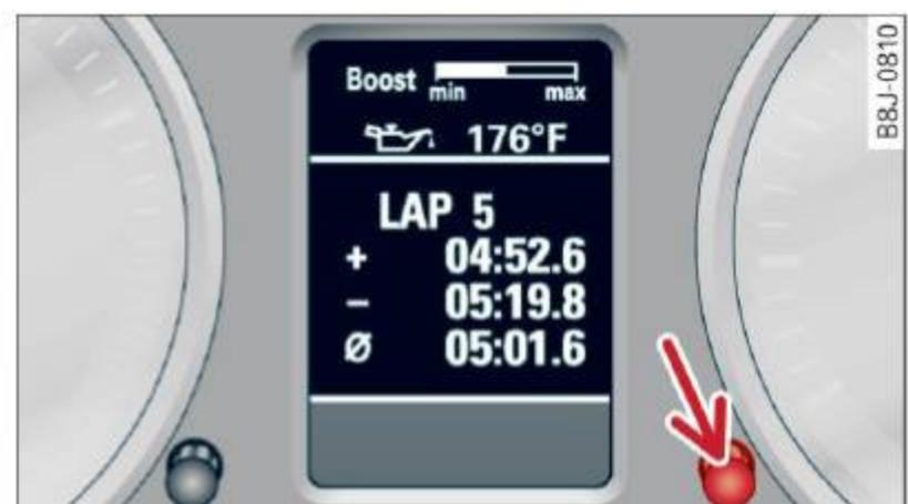
Fig. 20 Display: boost and engine oil temperature indicator
