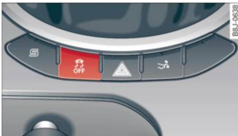
Fig. 127 Center console: ESC OFF button
