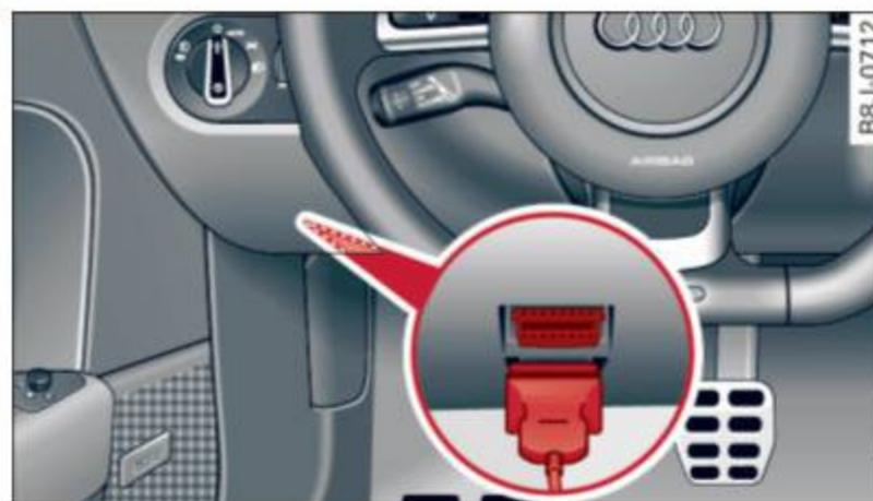
Fig. 24 Location of Data Link Connector (DLC)
