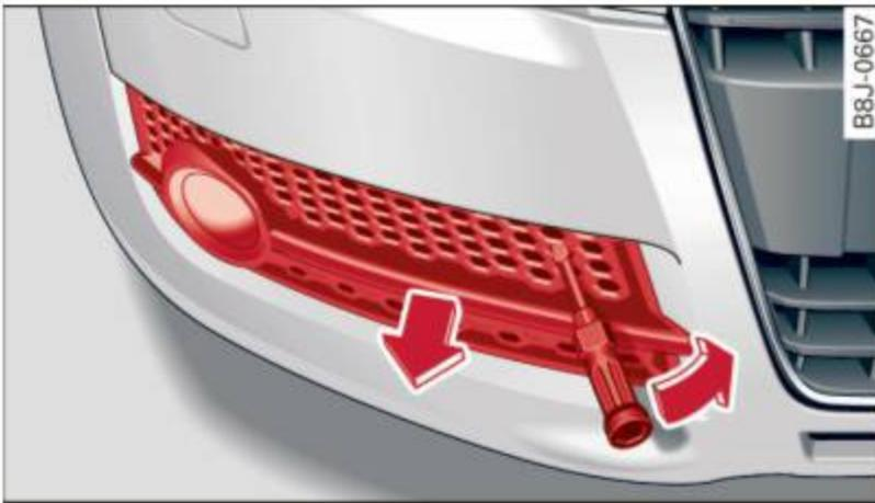
Fig. 170 Front bumper: removing the grill
