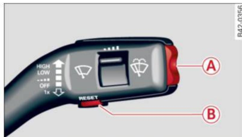
Fig. 148 Wiper lever: Controls for the menu display
