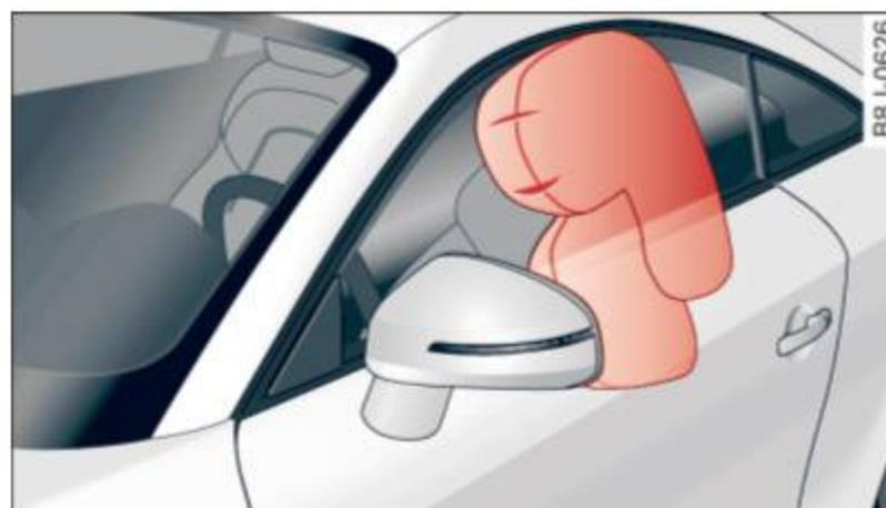
Fig. 111 Inflated side airbags on left side of vehicle
