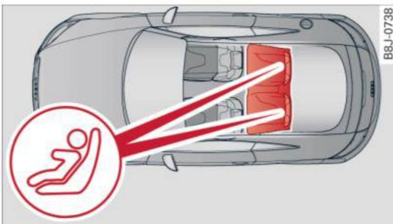
**Fig. 117** Schematic overview: LATCH anchorage point locations
