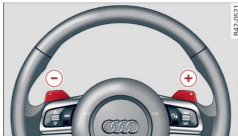
Fig. 85 Sport steering wheel with selector paddles
