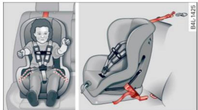
**Fig. 114** Schematic overview: installation of the attachments applicable to a LATCH seat
