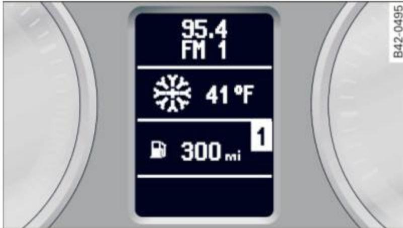
Fig. 6 Instrument cluster: center display
