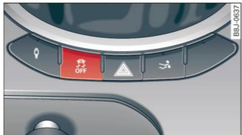
Fig. 126 Center console: ESC OFF button
