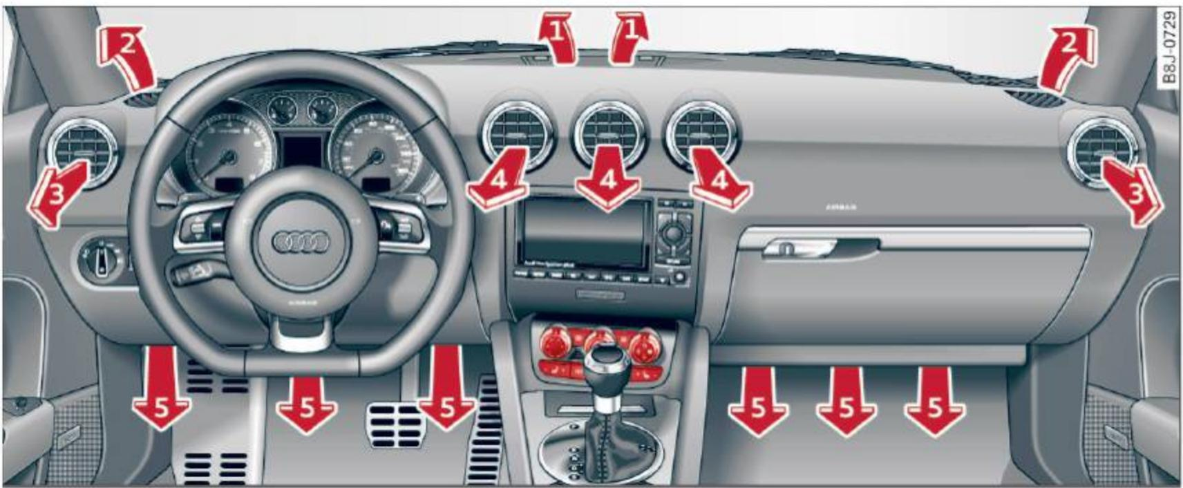
Fig. 69 Instrument panel: Location of air vents
