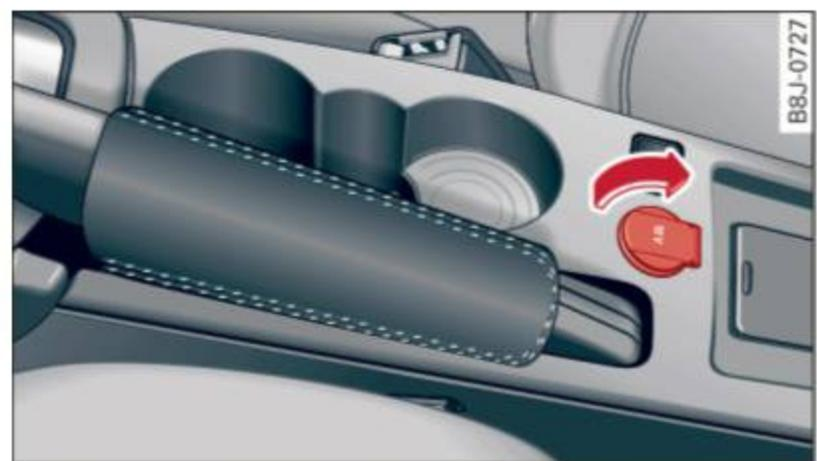
Fig. 66 Center console, front: 12-volt outlet
