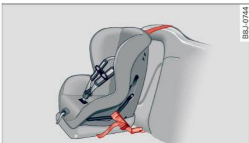
Fig. 124 Tether strap: proper routing and mounting
