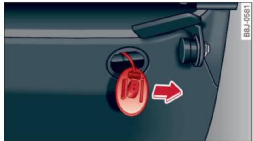
**Fig. 35** Section: Interior luggage compartment: Emergency release
