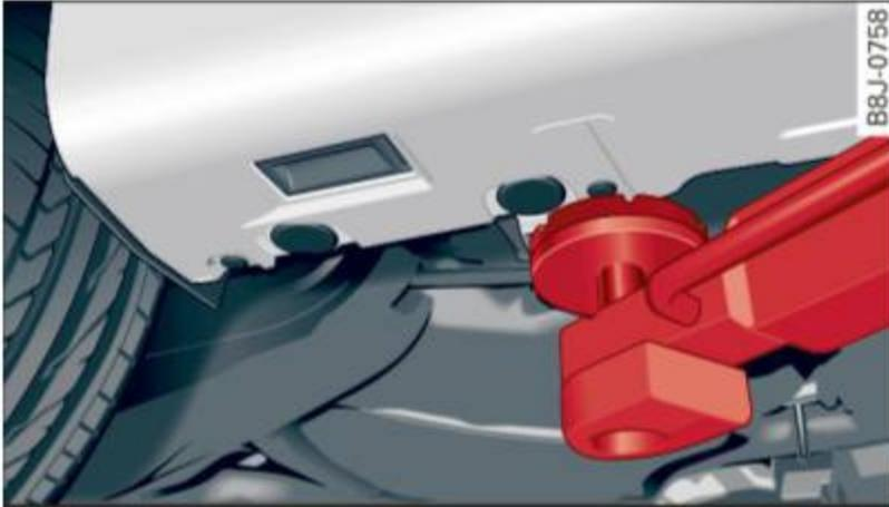
Fig. 177 Rear lifting point (right side)
