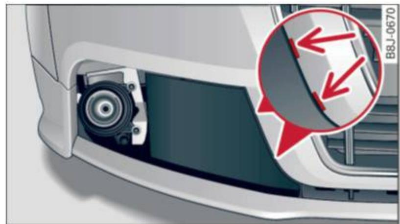
Fig. 173 Right front section with plastic cover
