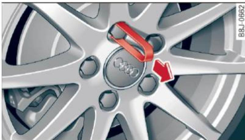
Fig. 157 Wheel change: removing the wheel bolt caps
