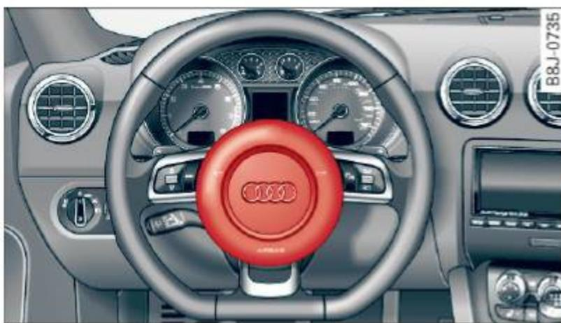
Fig. 104 Location of driver airbag: in steering wheel
