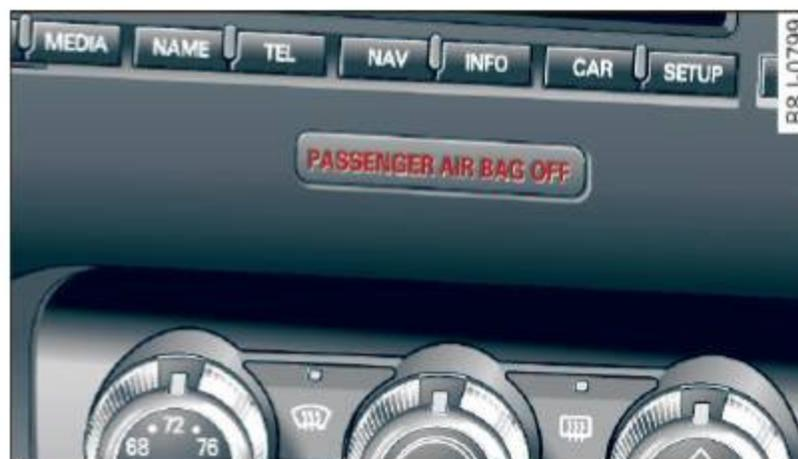
**Fig. 107** Section from the instrument panel: **PASSENGER AIR BAG OFF** light
