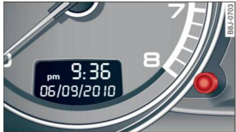
Fig. 73 Section of instrument cluster: Set/Check button
