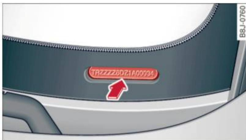
Fig. 179 Vehicle Identification Number (VIN) plate: location on driver's side dash panel
