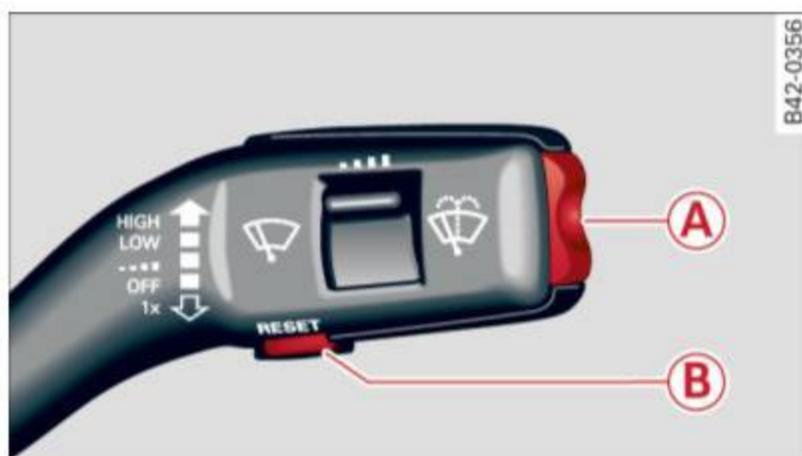
Fig. 12 Wiper lever: Controls for the menu display
