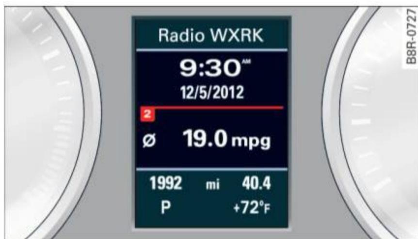
Fig. 9 Instrument cluster: center display
