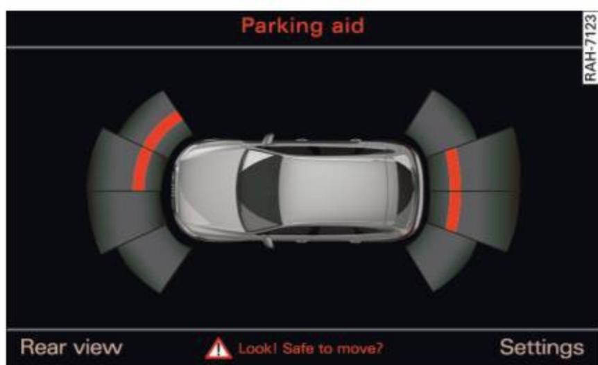
Fig. 146 MMI display: visual distance display
