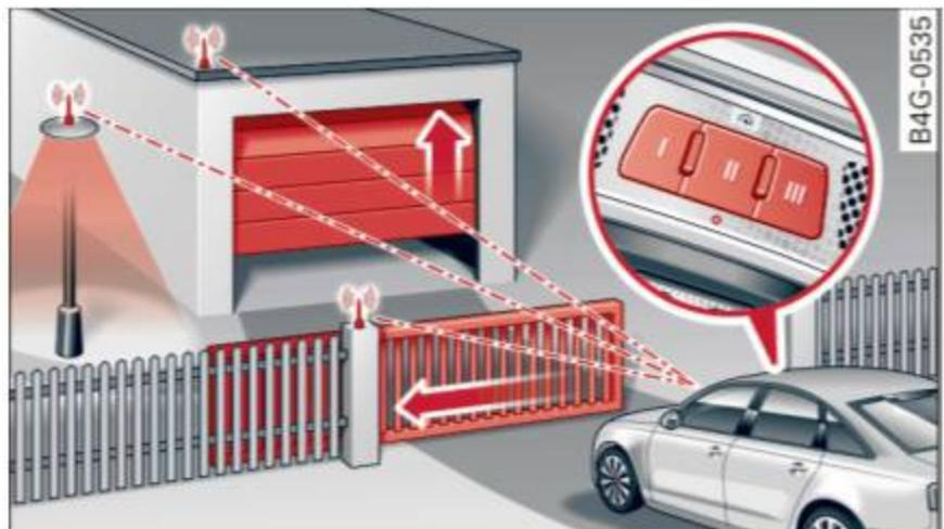
**Fig. 43** Garage door opener: examples of using with different systems
