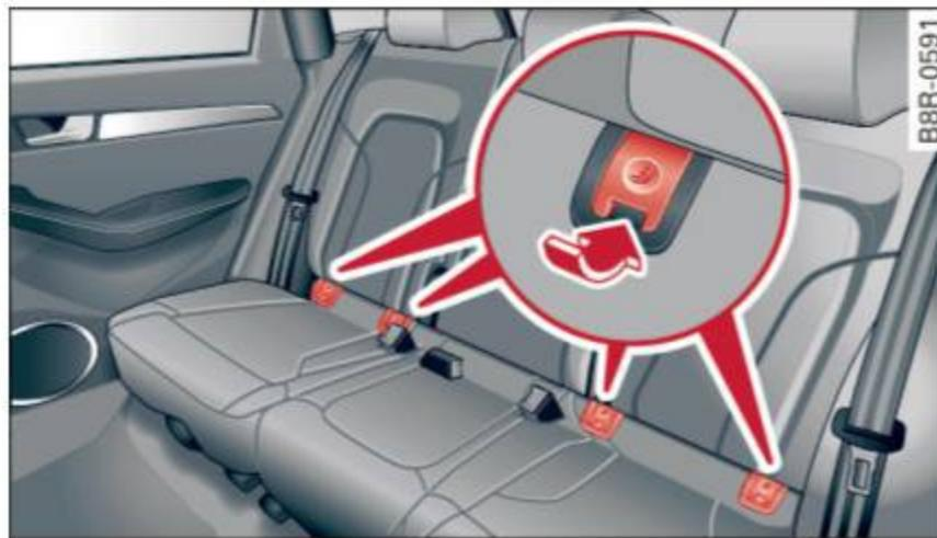
**Fig. 179** Lower anchorages, covers marked
