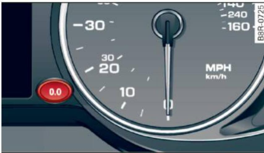
Fig. 7 Instrument cluster: reset button
