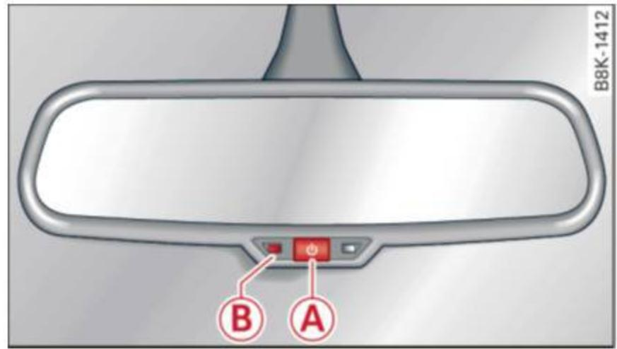
Fig. 61 Automatic dimming rearview mirror\*
