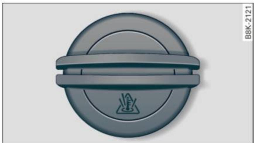
**Fig. 200** Engine compartment: cover on the coolant expansion tank
