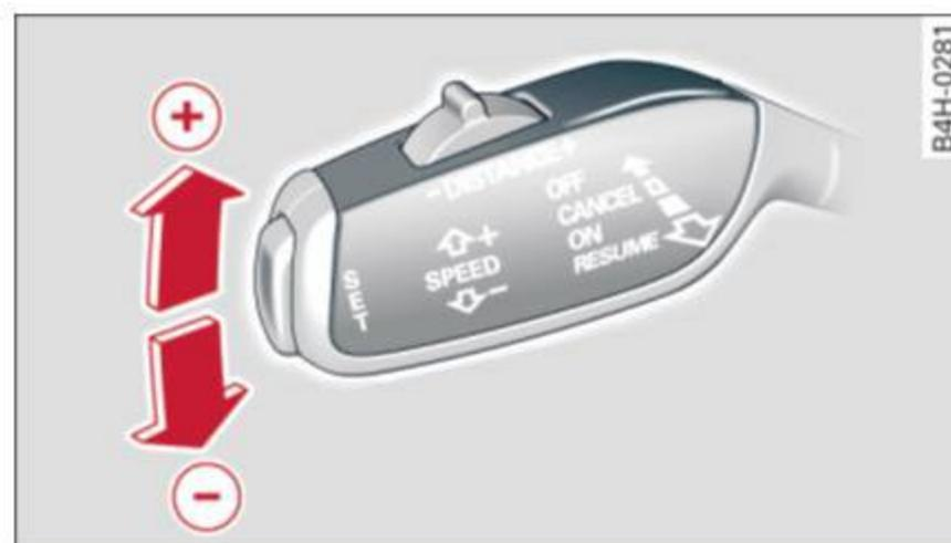
Fig. 122 Selector lever: changing the speed
