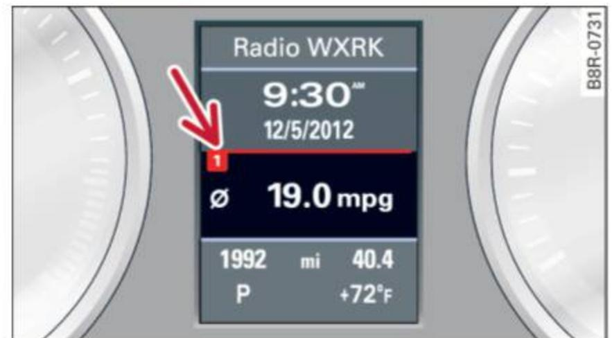
Fig. 16 Trip computer display: memory level 1
