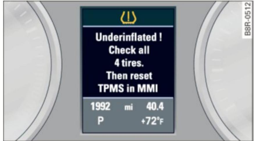
Fig. 208 Instrument cluster: indicator light with message
