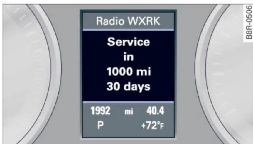
Fig. 14 Instrument cluster: Service interval display
