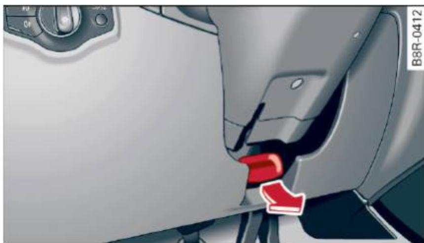
Fig. 98 Lever under the steering column
