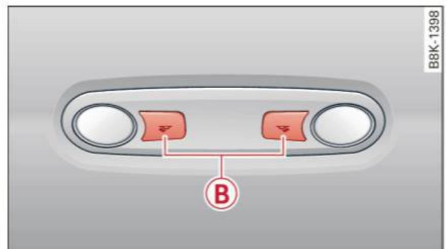
Fig. 52 Rear headliner: rear reading lights
