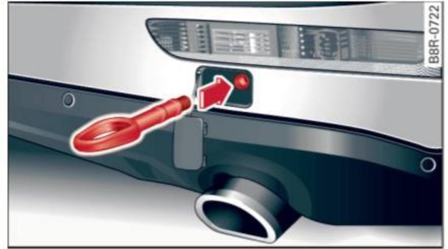
Fig. 232 Rear bumper: Screwing in towing loop
