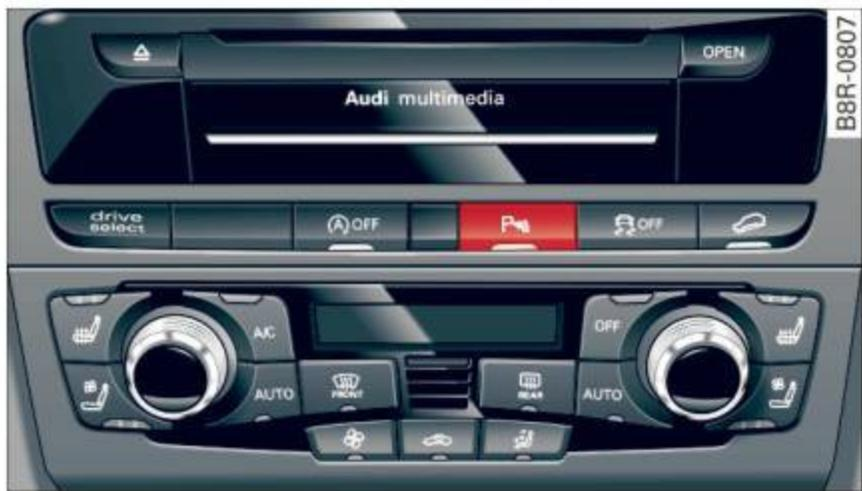
Fig. 145 Center console: Parking system switch
