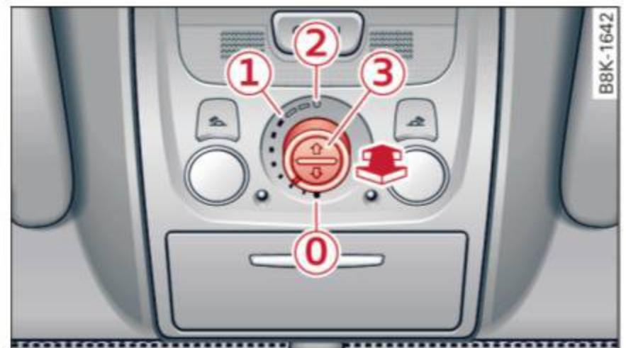
Fig. 42 Section from headliner: Knob for Panoramic sliding sunroof
