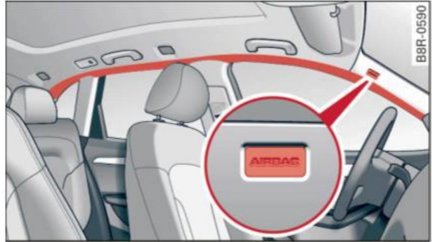
**Fig. 171** Side curtain system, driver's side: side curtain airbag location
