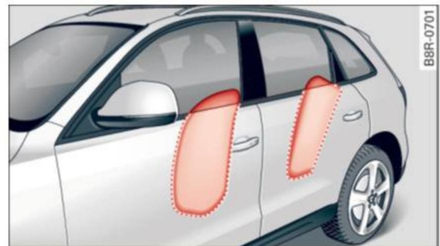
**Fig. 170** Inflated side airbags on left side of vehicle
