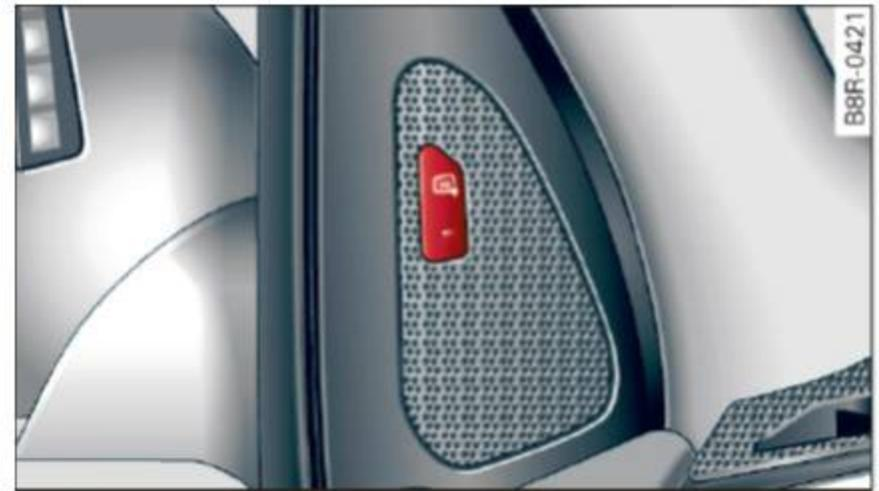
Fig. 131 Driver's door: Side assist button
