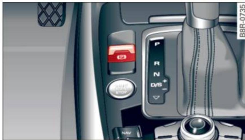
Fig. 103 Center console: Parking brake
