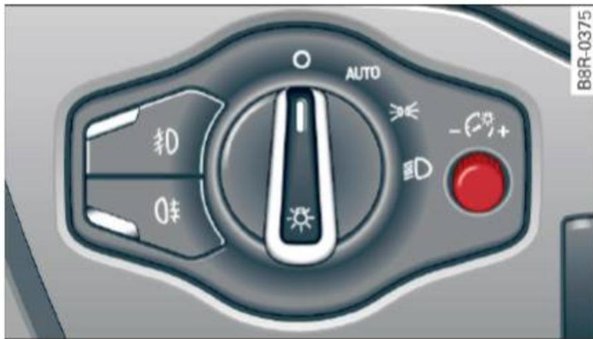
Fig. 53 Instrument illumination
