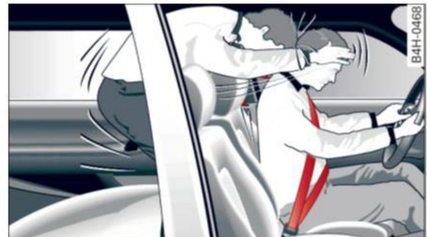
**Fig. 158** A rear passenger not wearing a safety belt will fly forward and strike the driver
