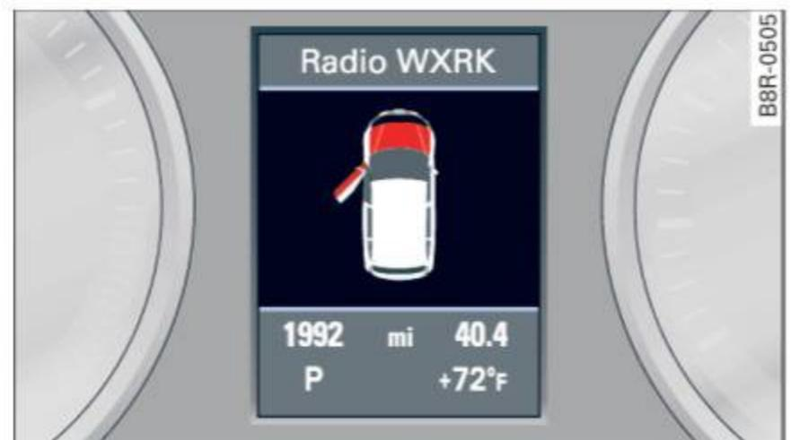
Fig. 13 Display: Open door- and trunk lid warning
