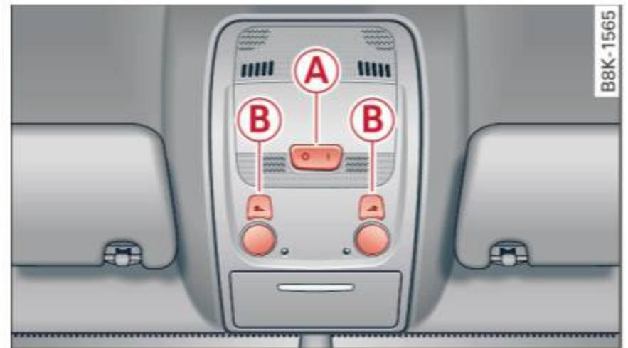
Fig. 51 Front headliner: interior lighting controls
