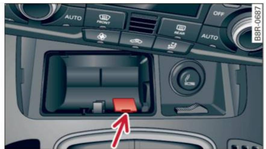
Fig. 140 Selector lever emergency release
