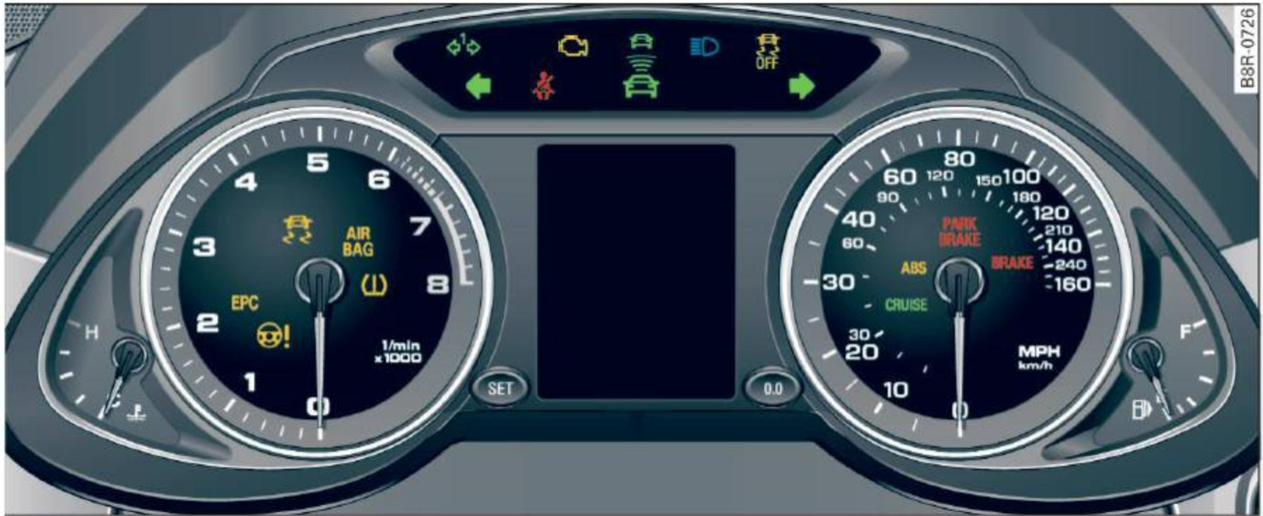
Fig. 8 Instrument cluster with warning/indicator lights
