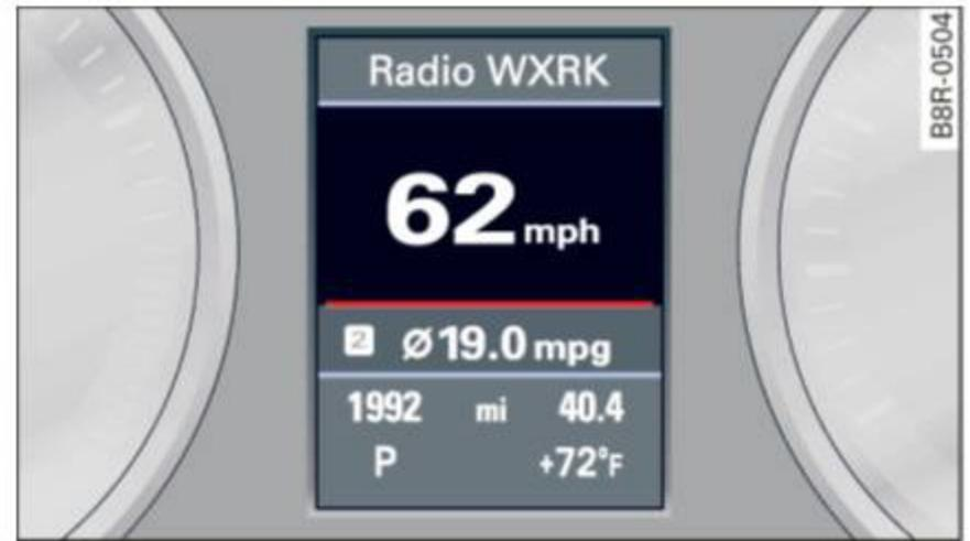
Fig. 12 Display: Digital speedometer
