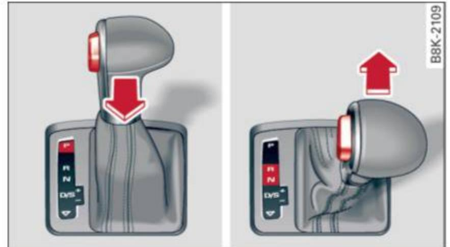
**Fig. 135** Shift gate: selector lever lock positions and release button highlighted
