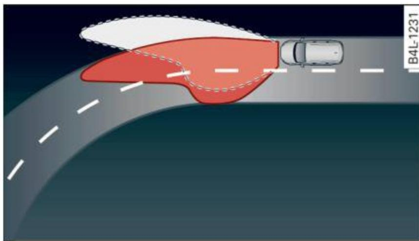
Fig. 48 Adaptive light when driving
