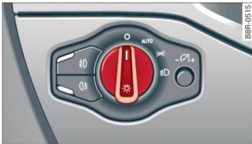
Fig. 46 Instrument panel: light switch
