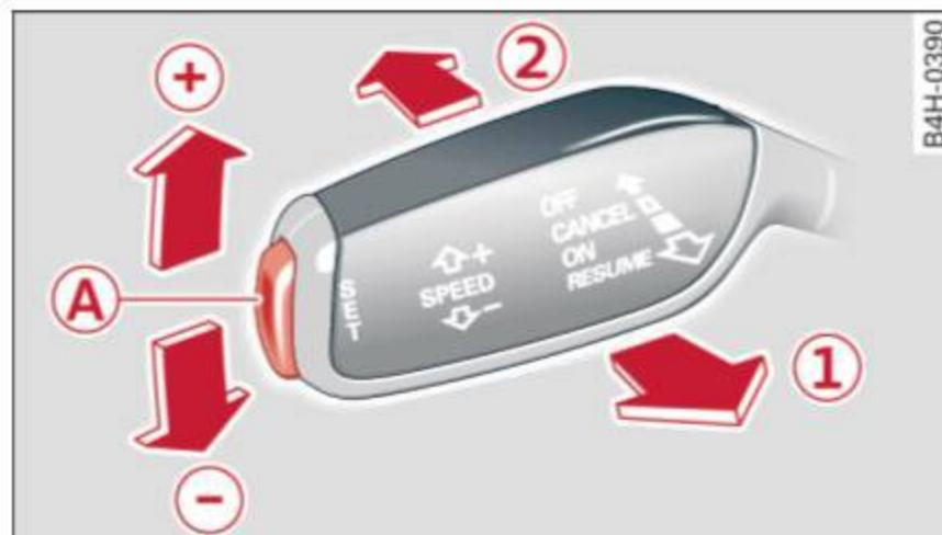
Fig. 108 Control lever with push-button
