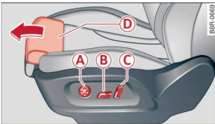
Fig. 64 Front seat: Controls for seat adjustment
