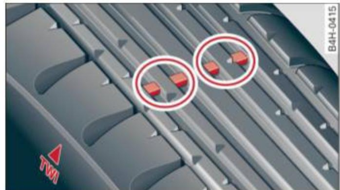
**Fig. 205** Tire profile: tread wear indicator
