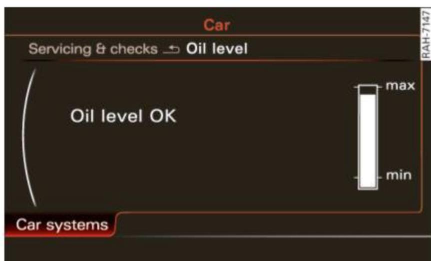
Fig. 198 Display: Oil level indicator
