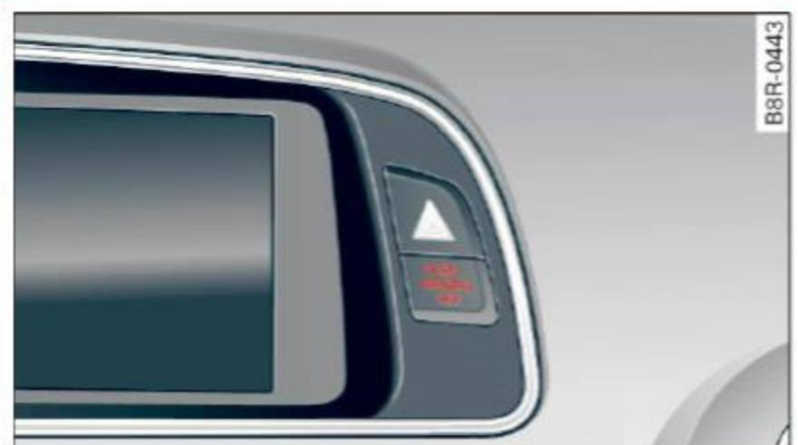
Fig. 168 Section from the instrument panel: PASSENGER AIR BAG OFF light
