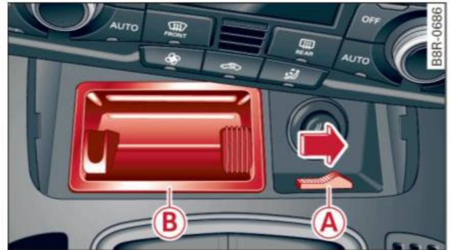
Fig. 139 Front center console: Removing the ashtray insert
