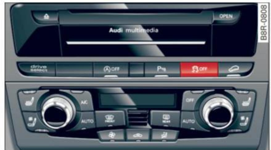
Fig. 186 Version B: Upper center console, OFF button
