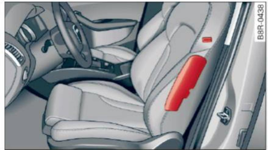
**Fig. 169** Side airbag location in the driver's seat
