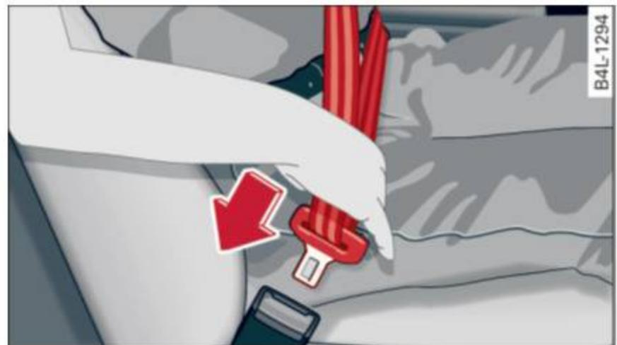
Fig. 160 Belt buckle and tongue on the driver's seat
