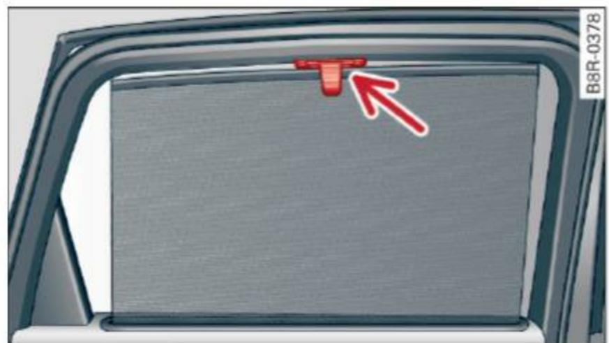
Fig. 55 Sun shade pulled up on a rear window
