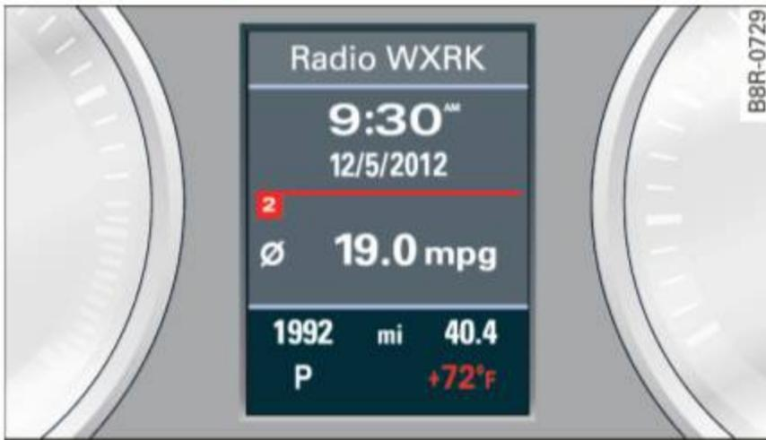
Fig. 11 Display: outside temperature
