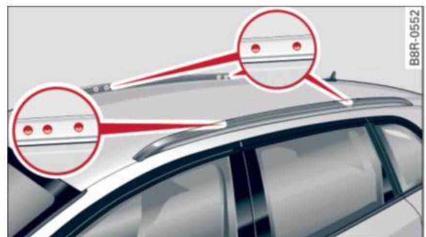
Fig. 81 Roof rack attachment points
