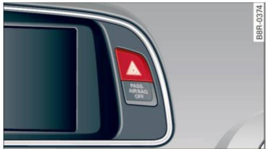
Fig. 49 Emergency flasher switch
