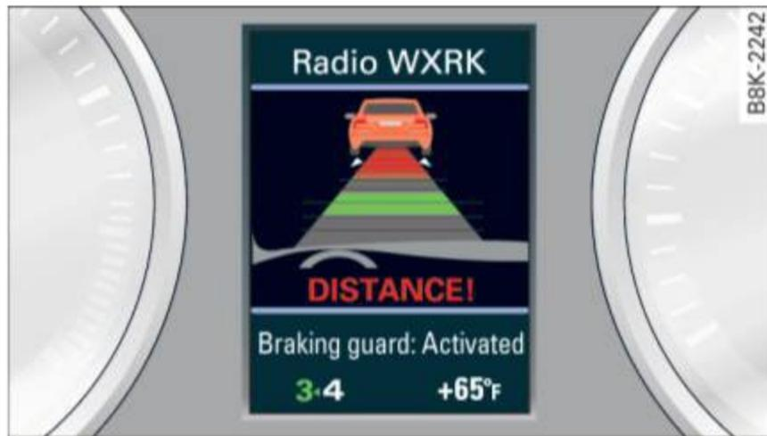
Fig. 126 Instrument cluster: approach warning
