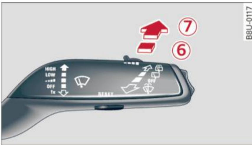
Fig. 57 Rear wiper actuation
