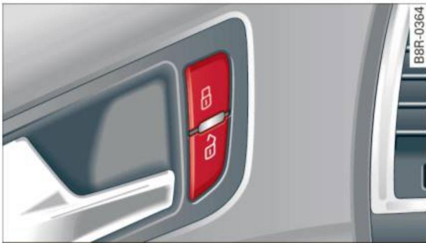
Fig. 32 Driver's door: power locking switch
