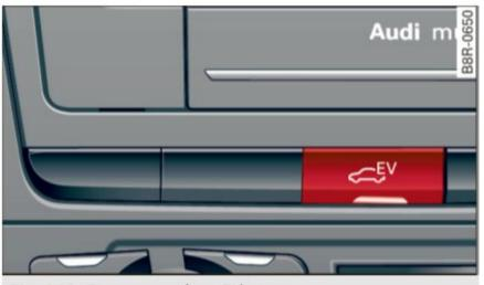
► To turn on EV mode, press the <a> button</a>. The indicator light in the button will turn on. The indicator light also turns on in the instrument cluster display.
