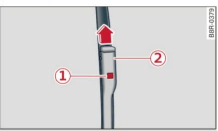
Fig. 58 Removing the wiper blade
