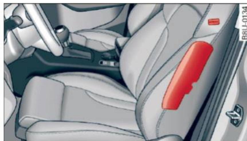
Fig. 119 Side airbag location in the driver's seat
