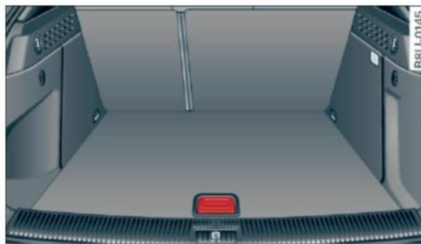
Fig. 64 Luggage compartment: reversible cargo area floor with the decorative side facing up
