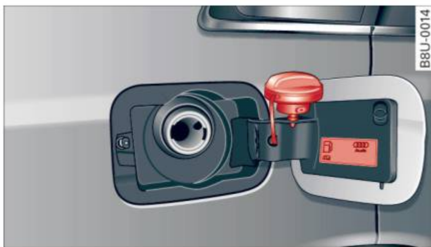
Fig. 136 Fuel filler door with attached fuel cap
