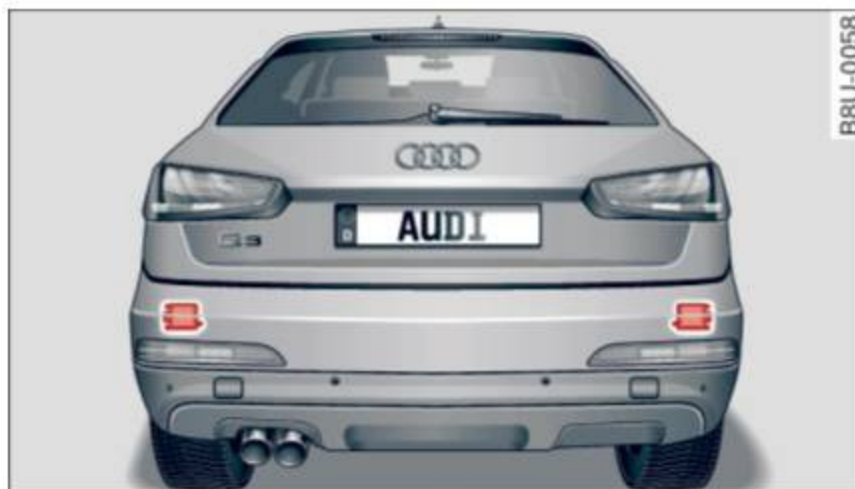
Fig. 84 Rear of the vehicle: position of the sensors
