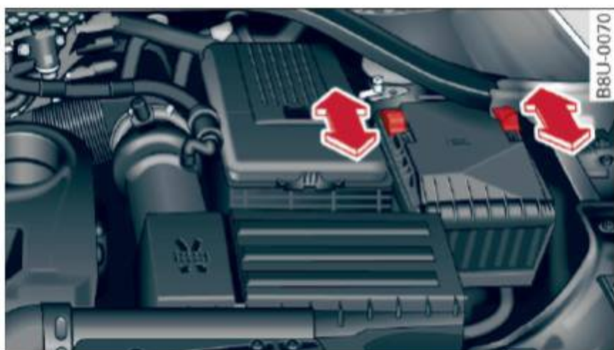
Fig. 163 Engine compartment: removing the fuse panel cover
