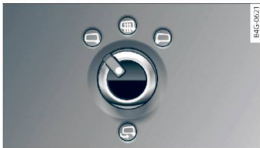
Fig. 38 Driver's door: knob for the exterior mirrors
