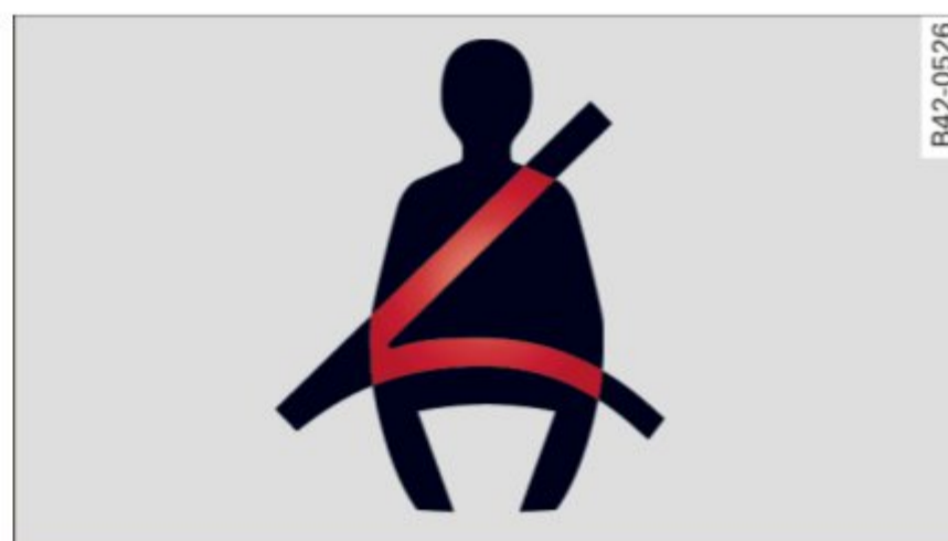
Fig. 104 Safety belt warning light in the instrument cluster - enlarged
