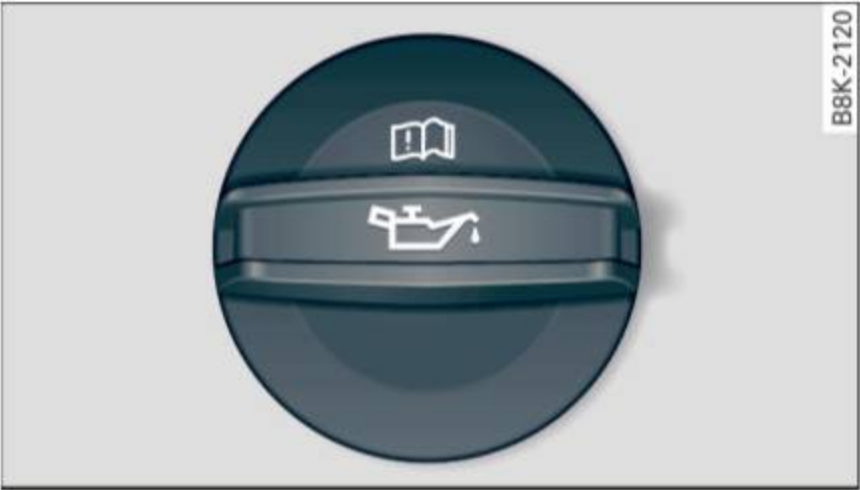
Fig. 142 Engine compartment: engine oil filler opening cover
