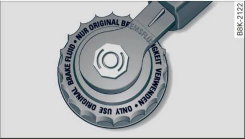
Fig. 144 Engine compartment: cap on brake fluid reservoir
