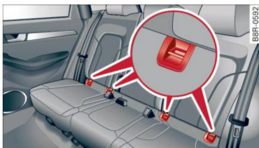
Fig. 130 Rear seats: lower anchorage bracket locations
