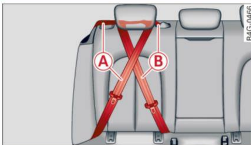
Fig. 123 Schematic overview: keep unused safety belts away from children in child safety seats. (A) - outer rear safety belt, (B) - center rear safety belt
