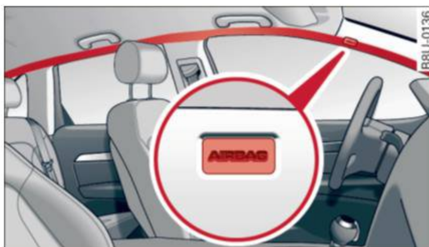
Fig. 121 Side curtain system, driver's side: side curtain airbag location
