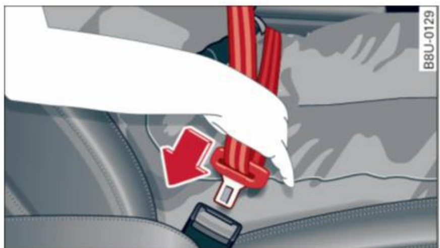
Fig. 110 Belt buckle and tongue on the driver's seat
