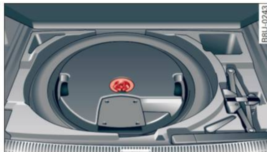
Fig. 160 Luggage compartment: space-saving spare tire (compact spare tire)
