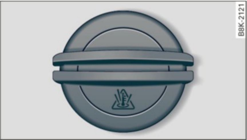
Fig. 143 Engine compartment: coolant expansion tank cover
