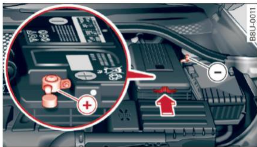
Fig. 164 Engine compartment: Connectors for jumper cables and charger
