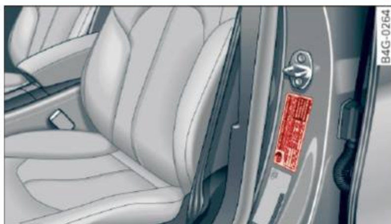
Fig. 149 Driver's side B-pillar: tire pressure label
