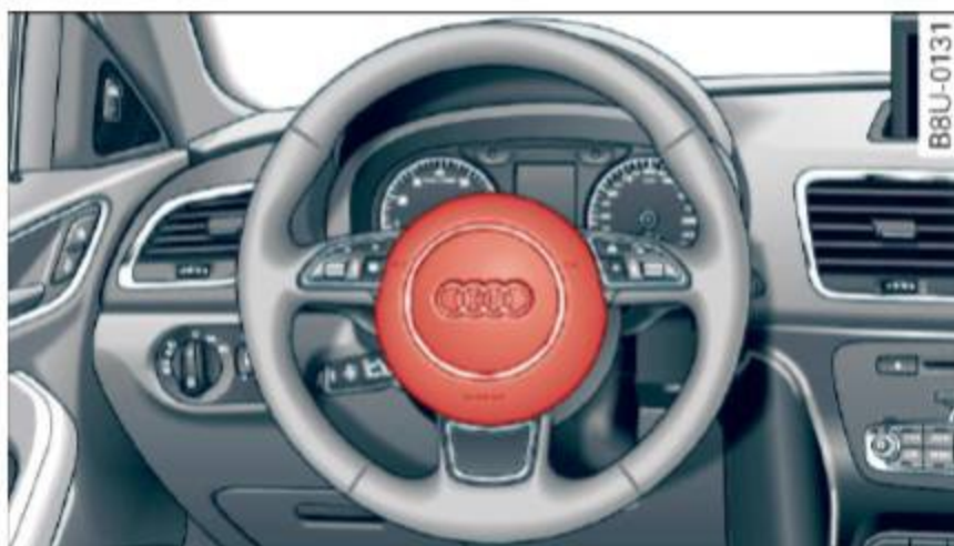
Fig. 115 Location of driver airbag: in steering wheel
