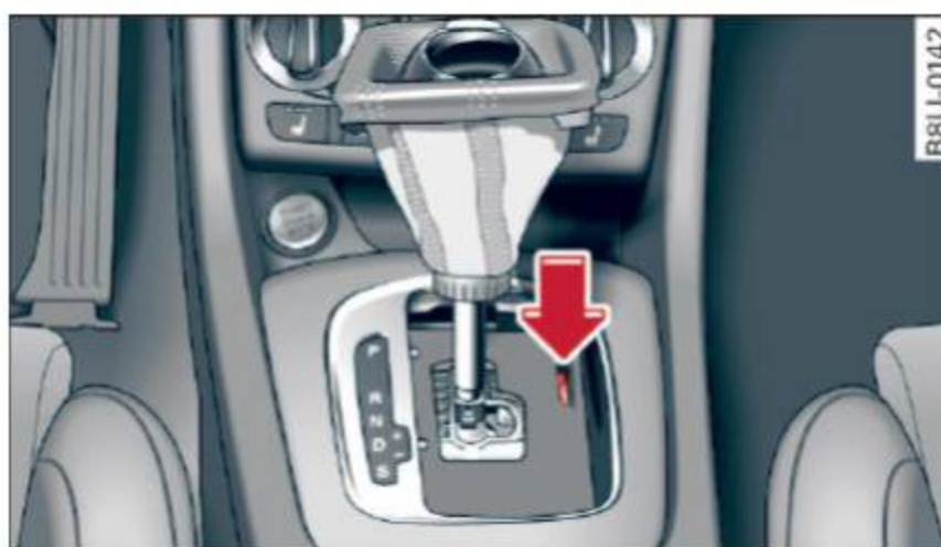
Fig. 78 Selector lever: emergency release
