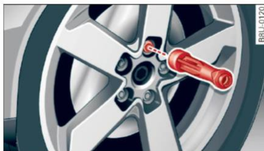
Fig. 158 Changing a wheel: using the hexagonal socket (with the blade removed) to turn the bolts
