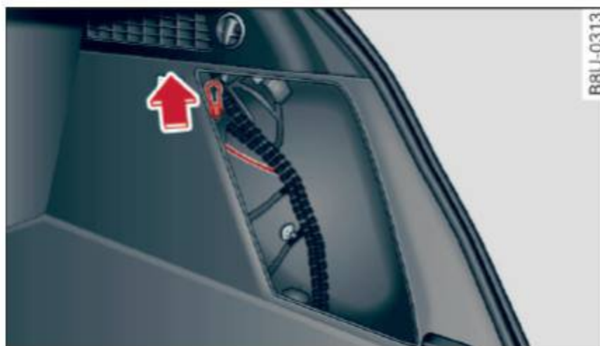
Fig. 137 Right side trim panel in the luggage compartment: emergency release mechanism
