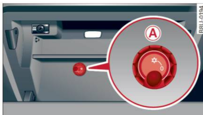
Fig. 56 Glove compartment: switching cooling mode* on/off
