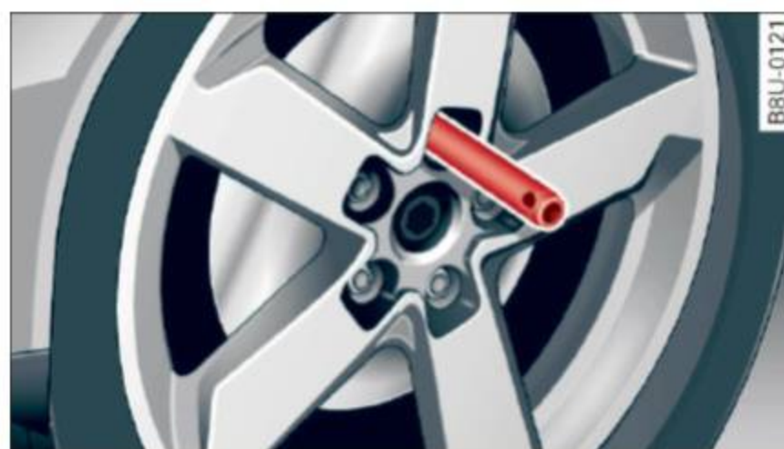
Fig. 159 Changing a wheel: alignment pin inside the top hole
