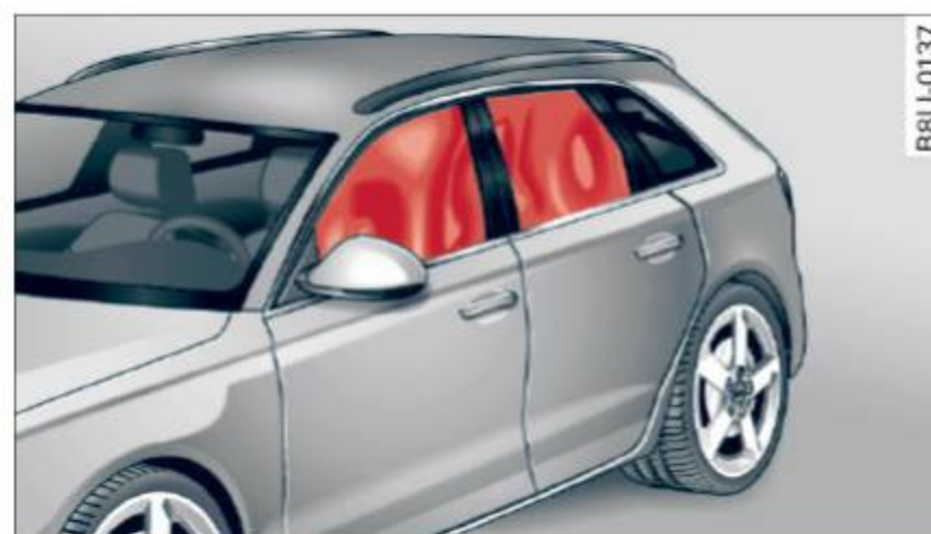
Fig. 122 Illustration of principle: Inflated side curtain airbags on the left side
