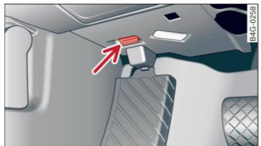
Fig. 14 Location of Data Link Connector (DLC)
