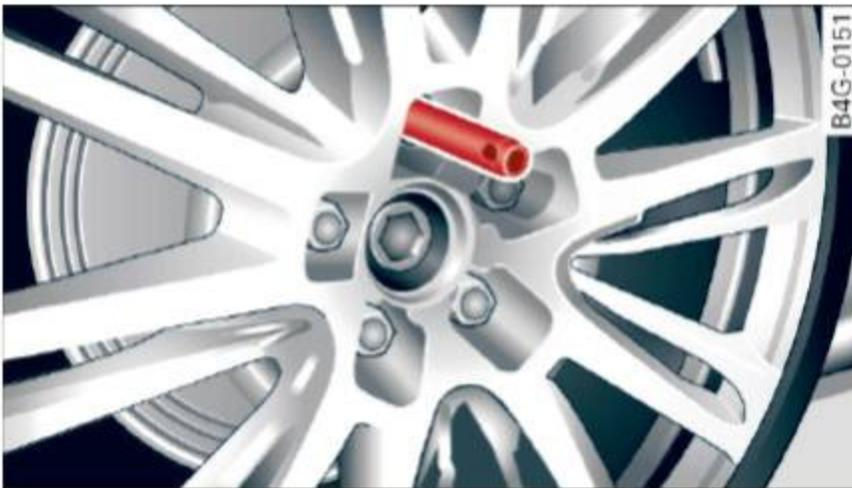
Fig. 208 Changing a wheel: alignment pin inside the top hole
