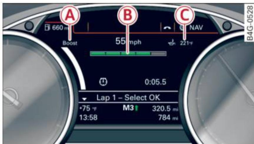
Fig. 87 Instrument cluster: boost, shifting and engine oil temperature indicators
