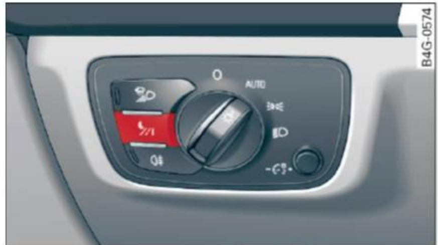
**Fig. 115** Area around the light switch: night vision assistant button
