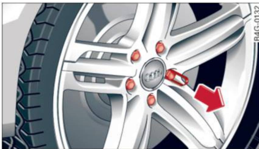
**Fig. 202** Changing a wheel: removing the wheel bolt caps
