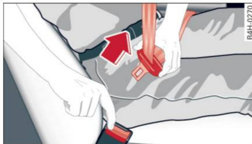
Fig. 153 Releasing the tongue from the buckle
