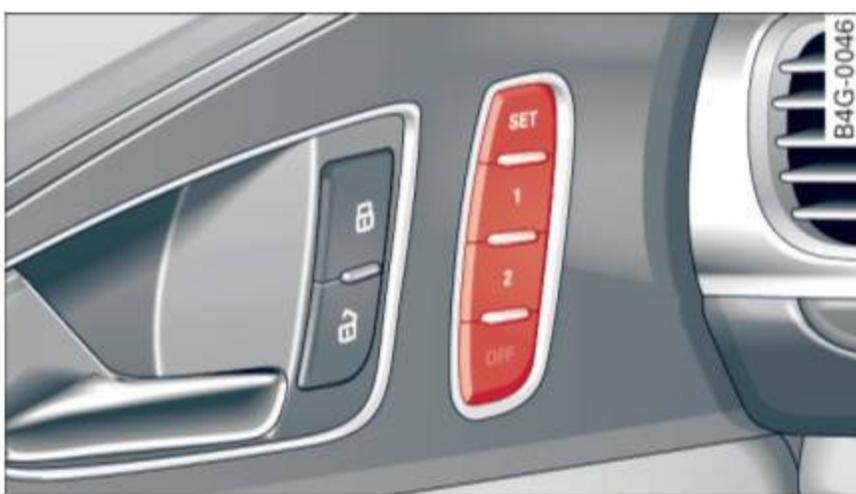
Fig. 51 Driver's door: memory function buttons
