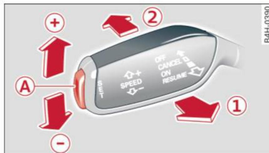
Fig. 86 Operating lever: cruise control system
