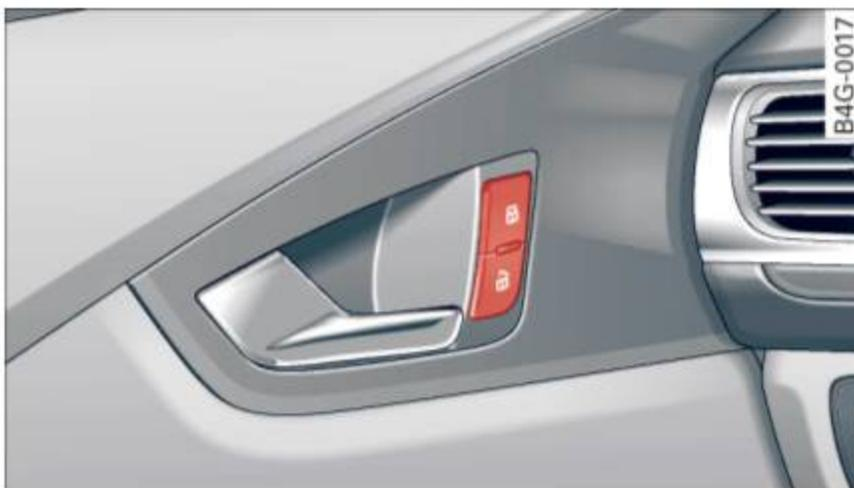
Fig. 20 Driver's door: central locking switch
