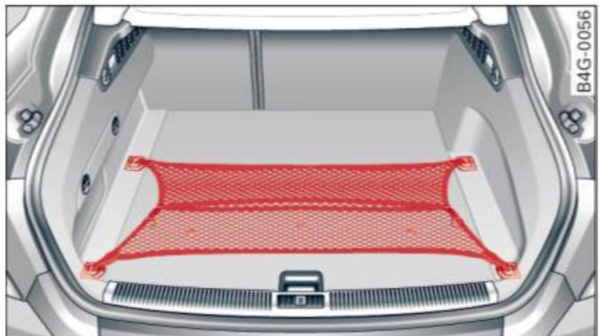
**Fig. 63** Luggage compartment: cargo net stretched out
