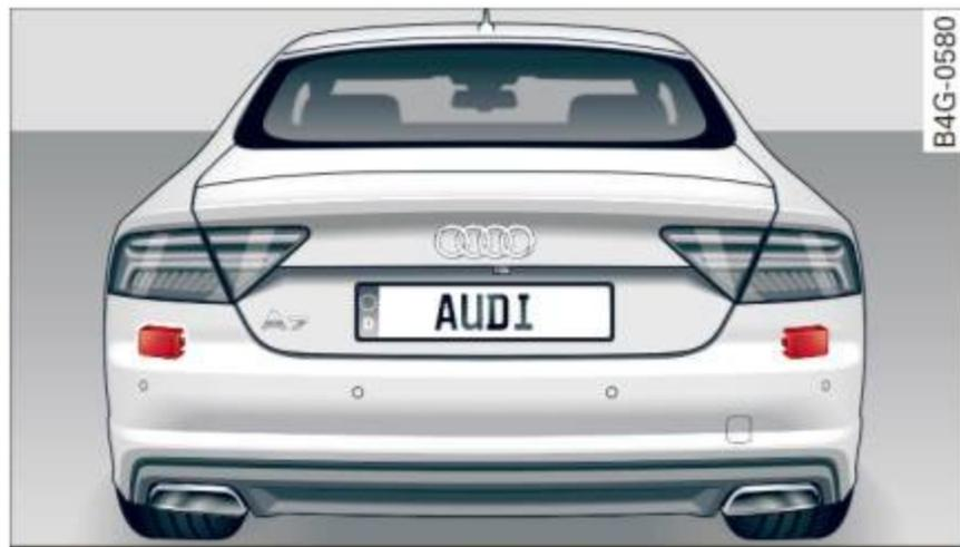
Fig. 108 Rear of the vehicle: position of the sensors
