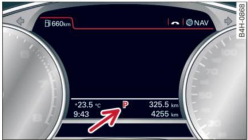
Fig. 81 Instrument cluster: selector lever positions
