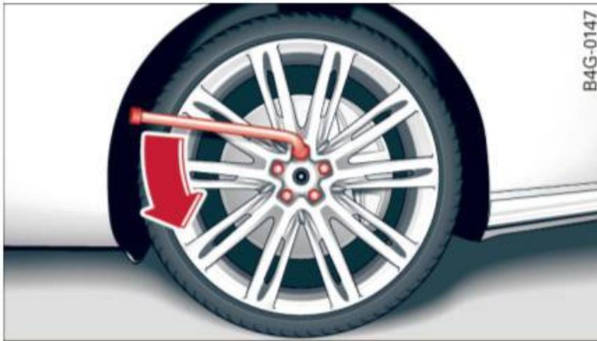
Fig. 203 Changing a wheel: loosening the wheel bolts
