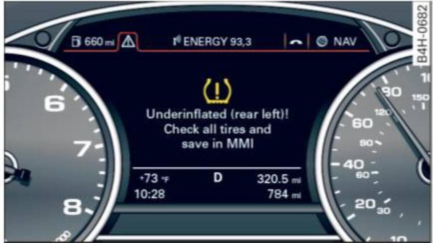
Fig. 194 Instrument cluster: indicator light with message
