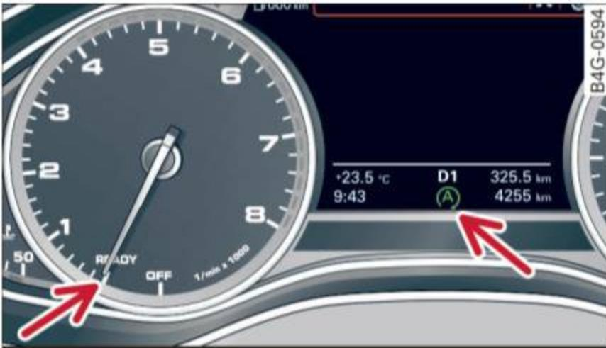
Fig. 78 Instrument cluster: engine switched off (stop phase)
