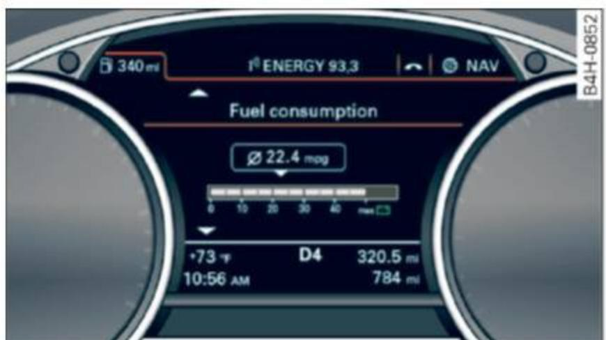
Fig. 8 Instrument cluster: fuel consumption display
