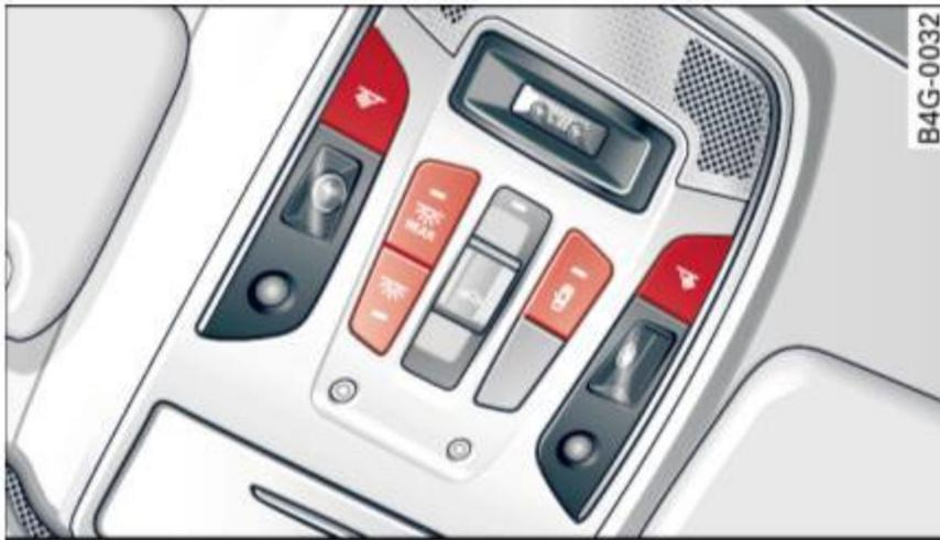
Fig. 36 Front headliner: interior lighting controls
