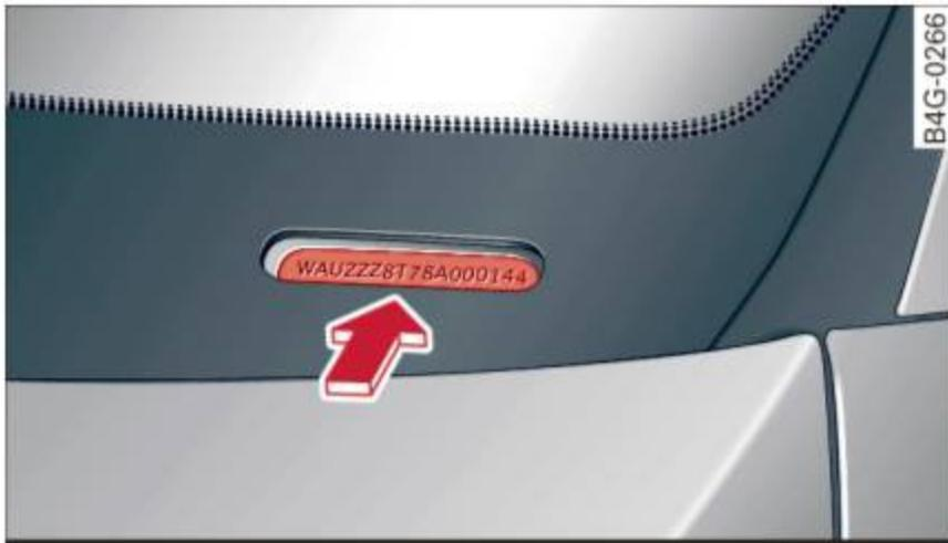
Fig. 223 Windshield (front left): Vehicle Identification Number (VIN)
