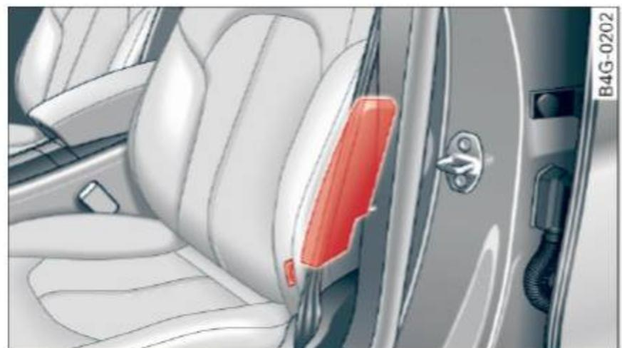
Fig. 161 Side airbag location in the driver's seat
