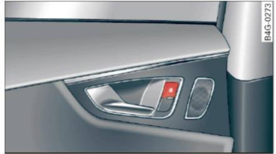
Fig. 21 Rear door: central locking switch
