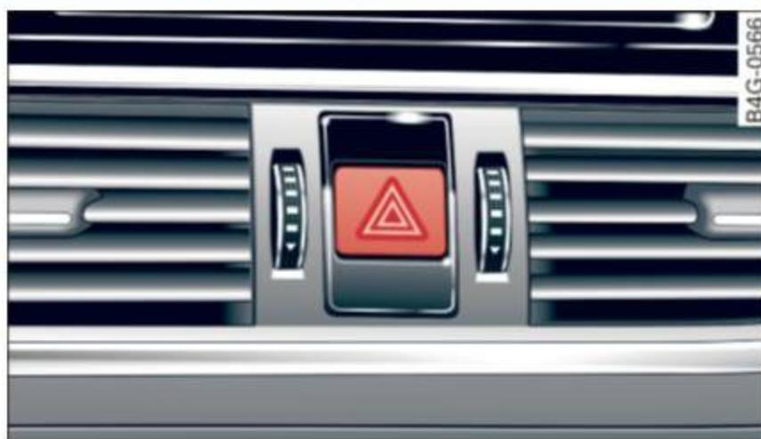
Fig. 35 Center console: emergency flasher button
