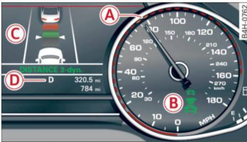
Fig. 95 Instrument cluster: adaptive cruise control
