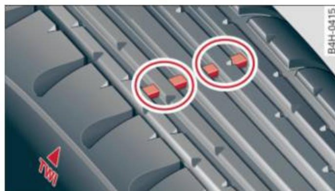
**Fig. 191** Tire profile: treadwear indicator
