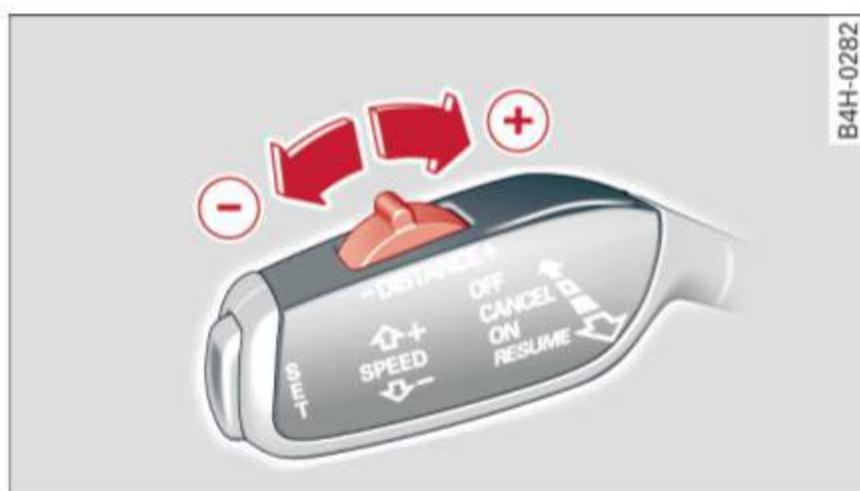
Fig. 98 Operating lever: setting the distance
