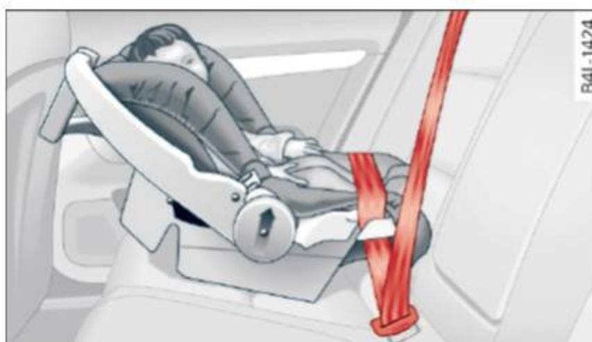
**Fig. 166** Schematic overview: rearward-facing infant seat, properly installed on the rear seat
