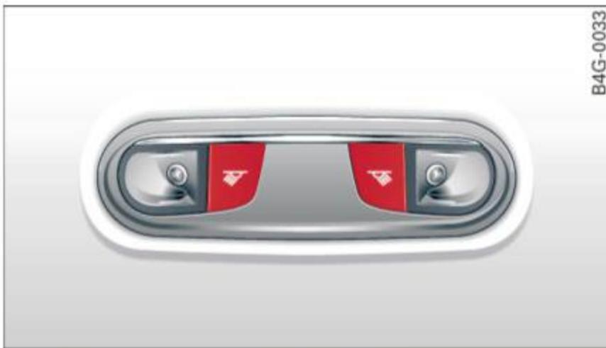
Fig. 37 Rear headliner: Reading light
