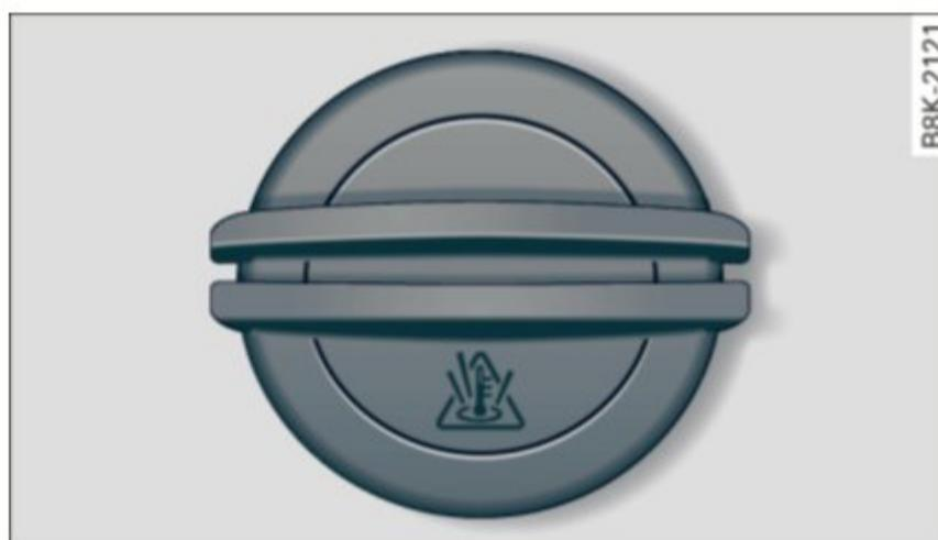
**Fig. 186** Engine compartment: coolant expansion tank cover
