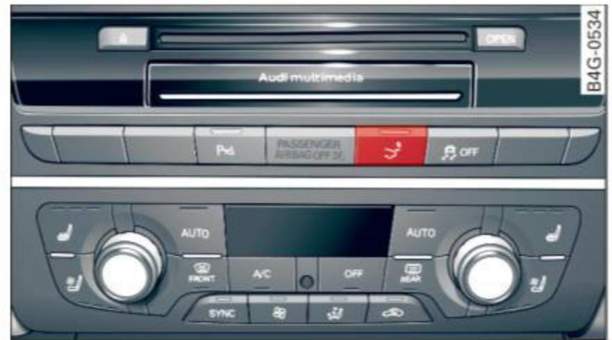
**Fig. 141** Center console: button for the rear spoiler
