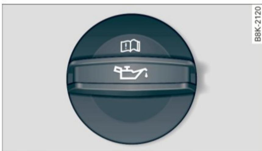
Fig. 185 Engine compartment: engine oil filler opening cover
