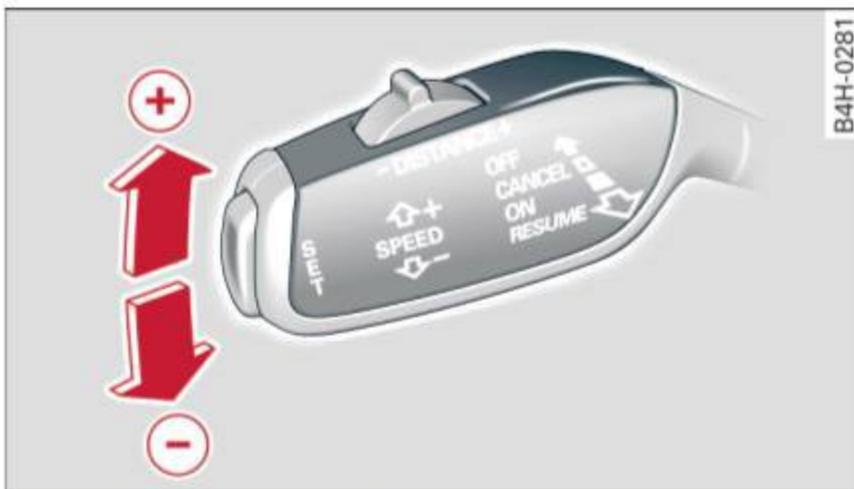
Fig. 96 Operating lever: changing the speed
