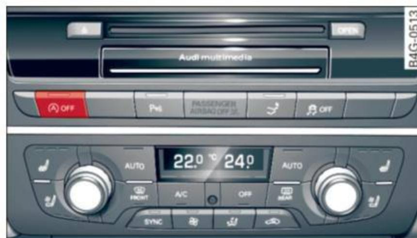
Fig. 79 Center console: Start/Stop system button
