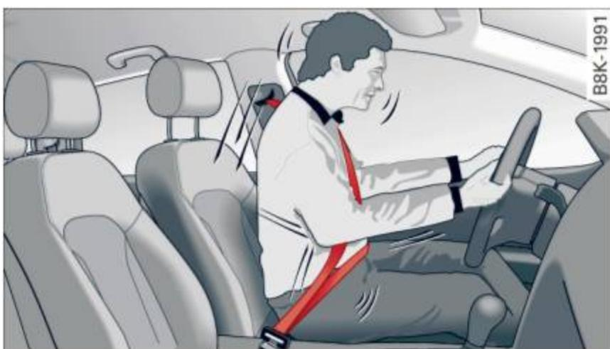
**Fig. 149** Driver is correctly restrained in a sudden braking maneuver
