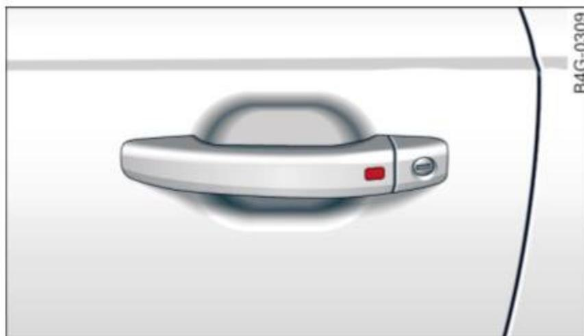
Fig. 19 Door handle: locking the vehicle
