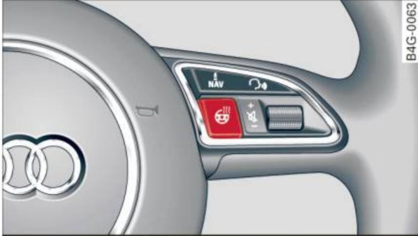
Fig. 73 Steering wheel: steering wheel heating button
