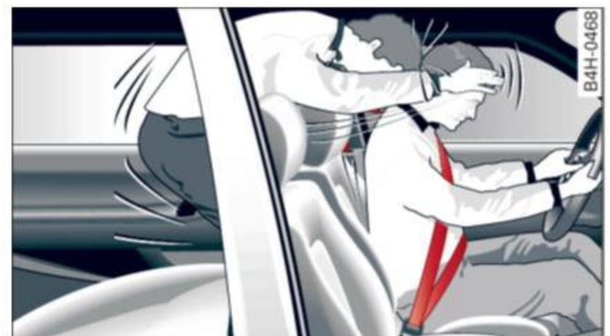
Fig. 148 A rear passenger not wearing a safety belt will fly forward and strike the driver
