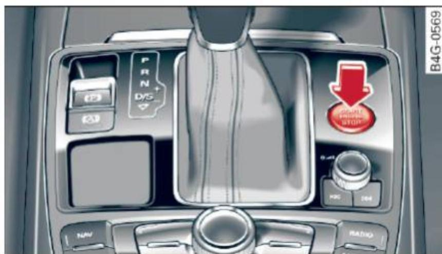
Fig. 76 Center console: START ENGINE STOP button
