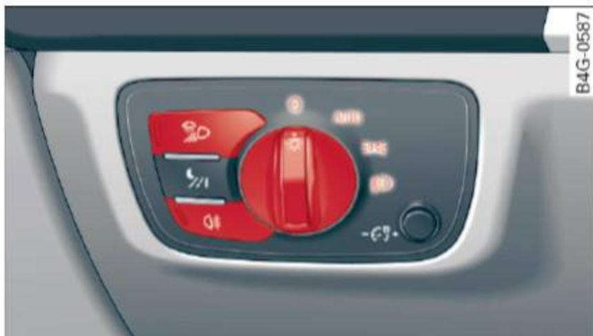
Fig. 33 Instrument panel: light switch with all weather lights
