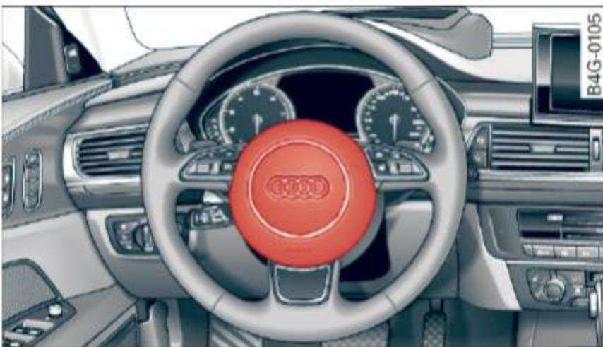
**Fig. 155** Location of driver airbag: in steering wheel
