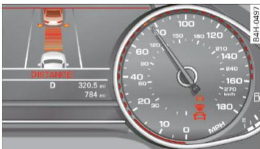
Fig. 100 Instrument cluster: approach warning
