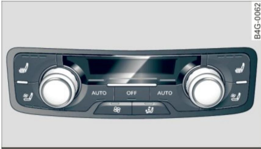
Fig. 72 4-zone deluxe automatic climate control system: rear controls
