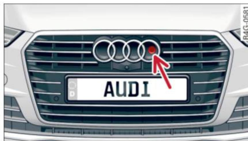
Fig. 114 Front of the vehicle: night vision assistant camera
