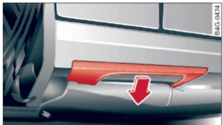
Fig. 206 Sill: removing the cover
