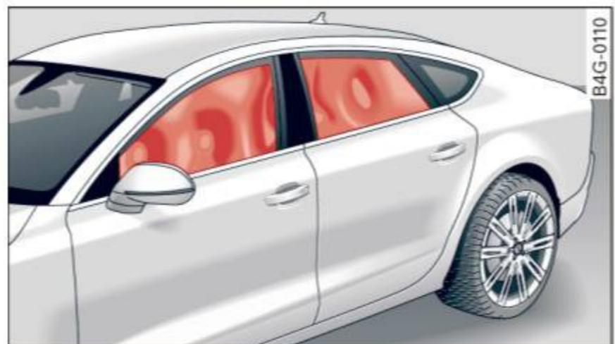
**Fig. 164** Illustration of principle: Inflated side curtain airbags on the left side
