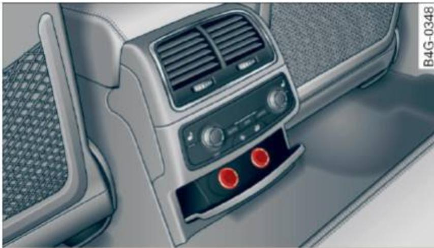
Fig. 56 Example of a rear center console: sockets\*
