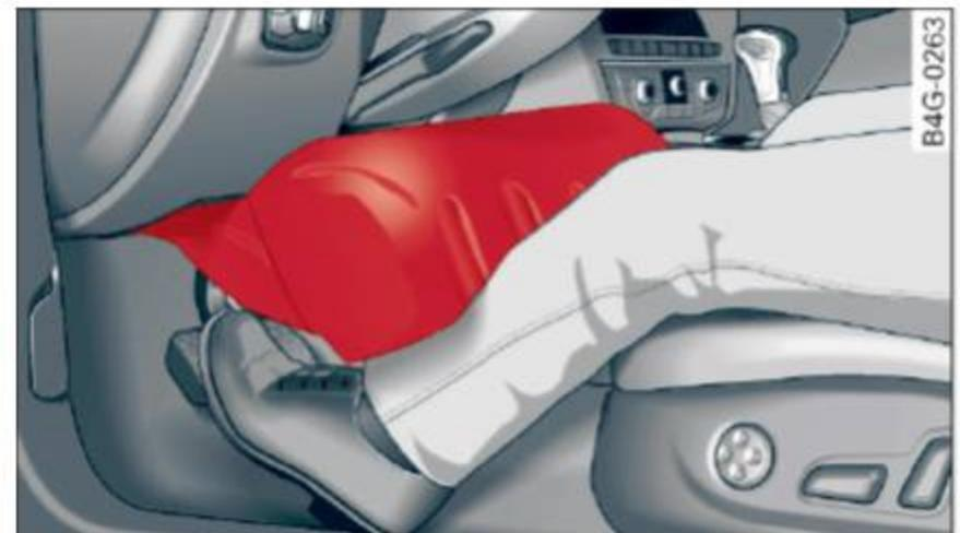
**Fig. 160** Inflated airbags protecting in a frontal collision
