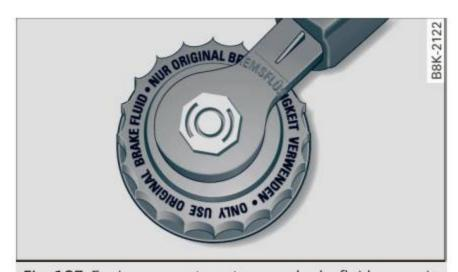
Fig. 187 Engine compartment: cap on brake fluid reservoir
