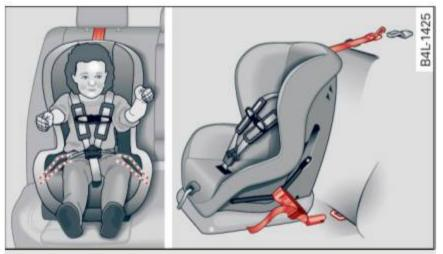
Fig. 167 Schematic overview: installation of the attachments applicable to a LATCH seat
