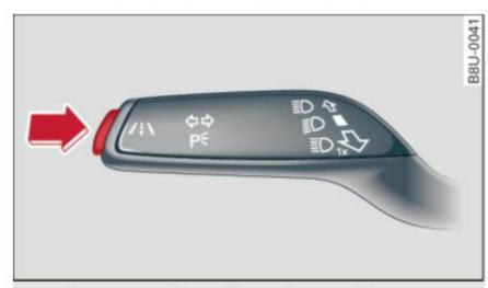
Fig. 101 Turn signal lever: button for active lane assist
