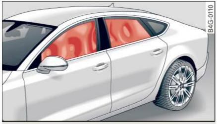
Fig. 164 Illustration of principle: Inflated side curtain airbags on the left side
