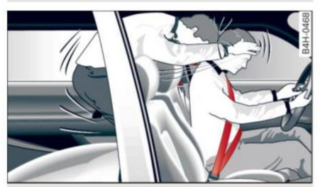
Fig. 148 A rear passenger not wearing a safety belt will fly forward and strike the driver
