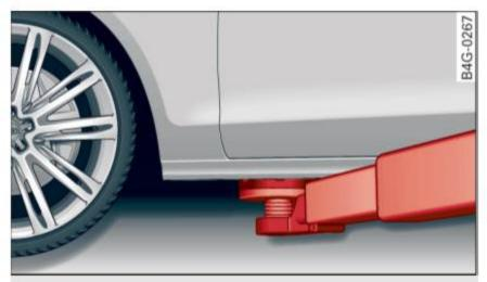
Fig. 221 Front lifting point
