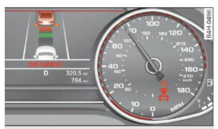
Fig. 99 Instrument cluster: request for driver intervention
