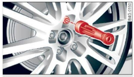
Fig. 207 Changing a wheel: using the screwdriver handle (with the blade removed) to turn the bolts
