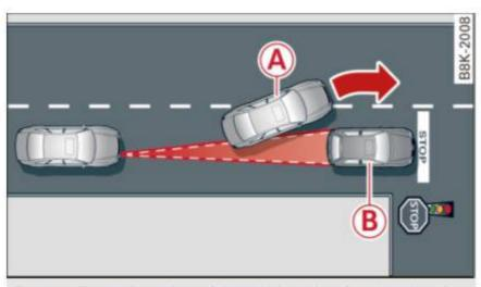
Fig. 93 Example: object changing lanes and stationary object
