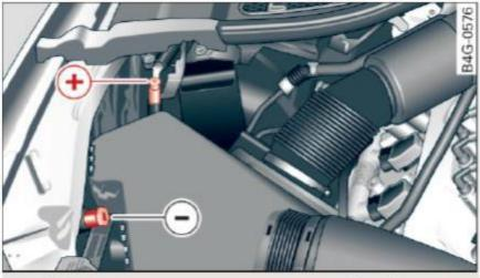
Fig. 188 Engine compartment: connectors for a charger and jump start cables
