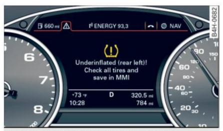
Fig. 195 Display: indicator light with a message
