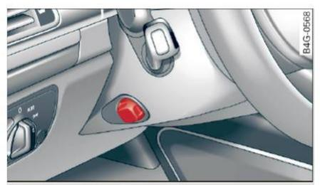
Fig. 75 Switch for adjusting the steering wheel position
