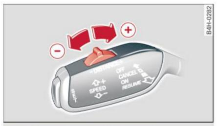
Fig. 98 Operating lever: setting the distance
