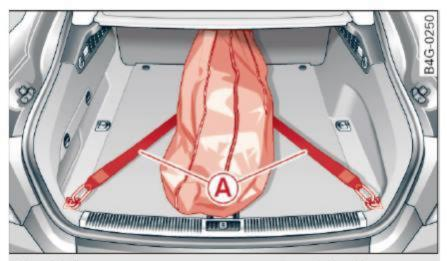
Fig. 68 Luggage compartment: securing the bag\*
