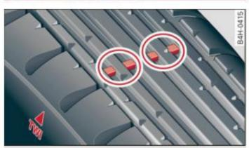
Fig. 191 Tire profile: treadwear indicator
