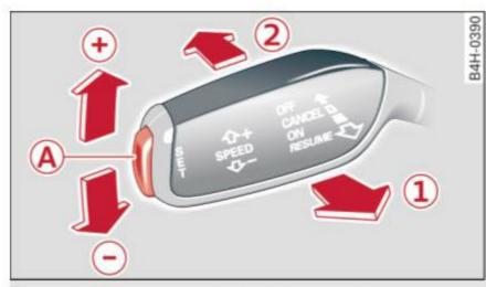
Fig. 86 Operating lever: cruise control system
