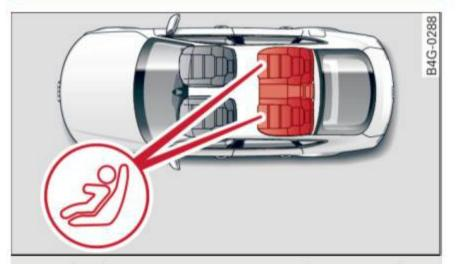
Fig. 170 Schematic overview: LATCH anchorage point locations
