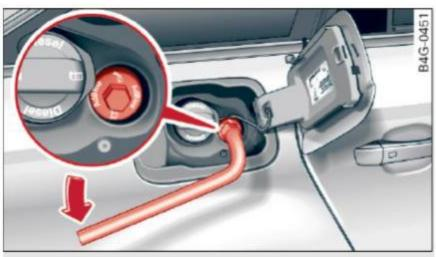
Fig. 180 Right rear side of the vehicle: removing the AdBlue cap
