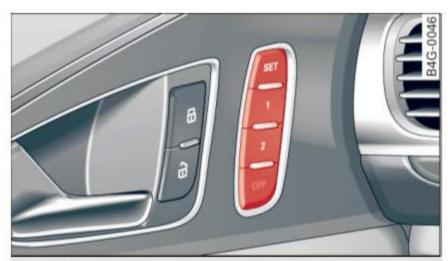
Fig. 51 Driver's door: memory function buttons
