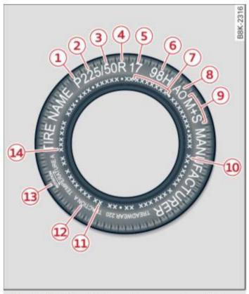
Fig. 190 Tire designations on the sidewall
