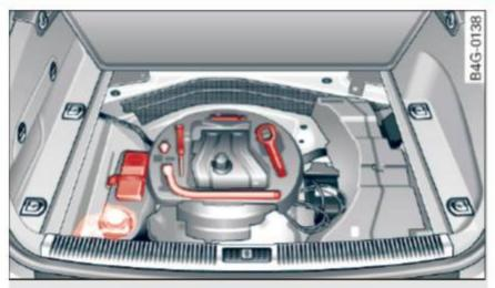
Fig. 197 Luggage compartment: vehicle tool kit, tire mobility kit and compressor
