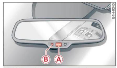
Fig. 40 Automatic dimming rearview mirror\*
