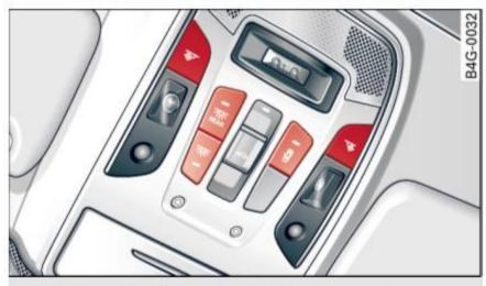
Fig. 36 Front headliner: interior lighting controls
