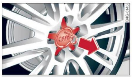
Fig. 201 Changing a wheel: Removing the wheel cover
