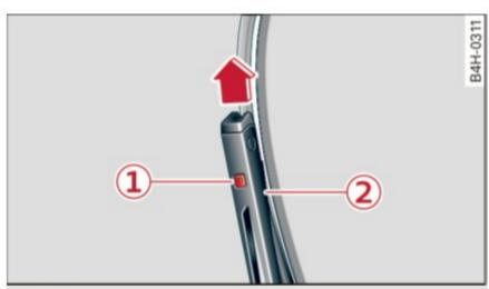
Fig. 44 Removing windshield wiper blades
