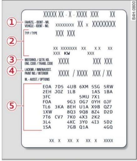
Fig. 224 Vehicle identification label
