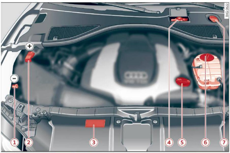
Fig. 184 Typical location of the reservoir and the engine oil filler opening
