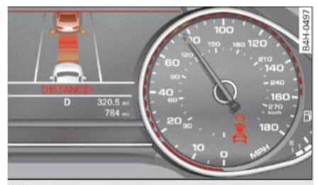
Fig. 100 Instrument cluster: approach warning
