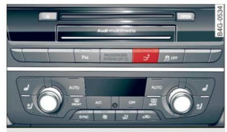
Fig. 141 Center console: button for the rear spoiler
