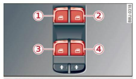
Fig. 29 Driver's door: power window controls
