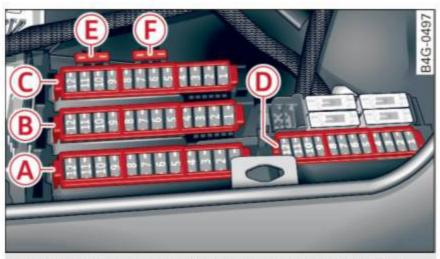
Fig. 213 Luggage compartment: fuse panel with plastic bracket
