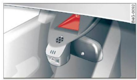
Fig. 102 Windshield: camera window for active lane assist
