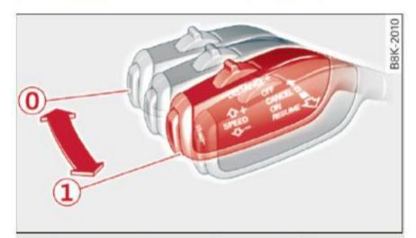
Fig. 94 Operating lever: switching on and off
