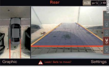
Fig. 136 Infotainment system: aligning the vehicle
