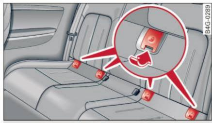
Fig. 171 Lower anchorages, covers marked
