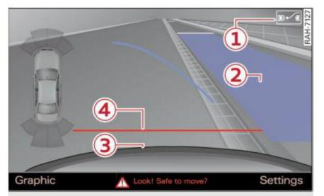
Fig. 125 Infotainment: blue surfaces aligned in the parking space
