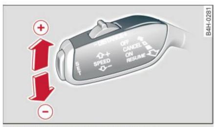
Fig. 96 Operating lever: changing the speed
