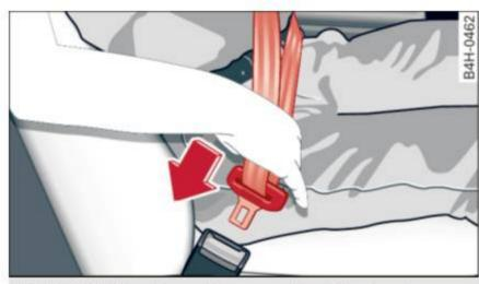
Fig. 150 Belt buckle and tongue on the driver's seat
