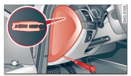
Fig. 210 Driver's side cockpit: cover
