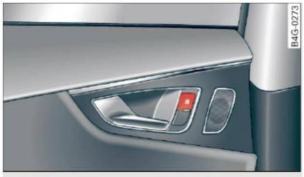
Fig. 21 Rear door: central locking switch
