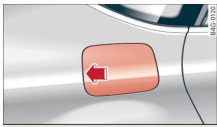
Fig. 176 Right rear side of the vehicle: opening the fuel filler door
