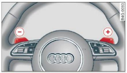
Fig. 84 Steering wheel: manual shifting with the shift paddles\*
