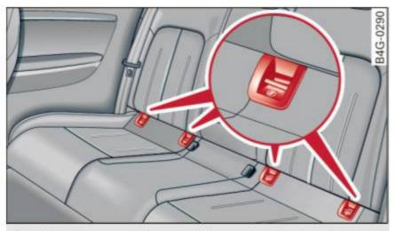
Fig. 172 Rear seats: lower anchorage bracket locations
