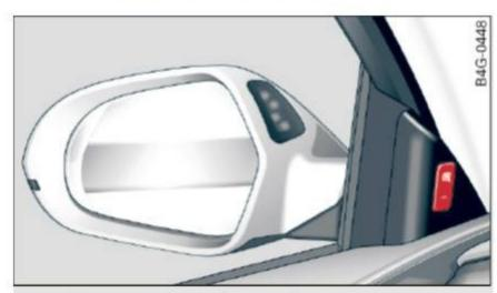
Fig. 109 Driver's door: side assist button
