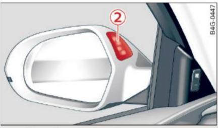
Fig. 106 Display on the exterior mirror
