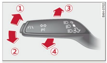
Fig. 34 Turn signal and high beam lever
