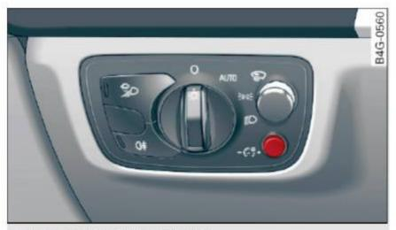
Fig. 38 Instrument illumination
