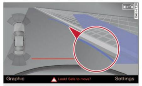
Fig. 126 Infotainment: contact of the blue curved line with the curb
