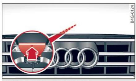
Fig. 183 Rocker switch under the hood
