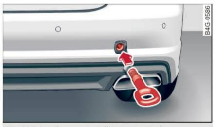
Fig. 219 Rear bumper: installing the towing loop
