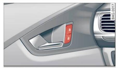
Fig. 20 Driver's door: central locking switch
