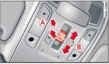
Fig. 30 Section of headliner: sunroof button
