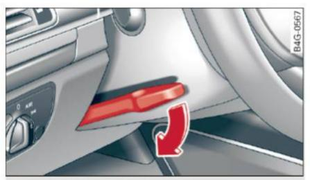
Fig. 74 Lever on the steering column
