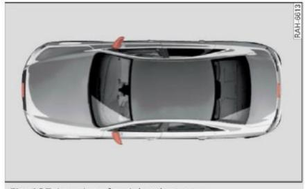
Fig. 127 Location of peripheral cameras
