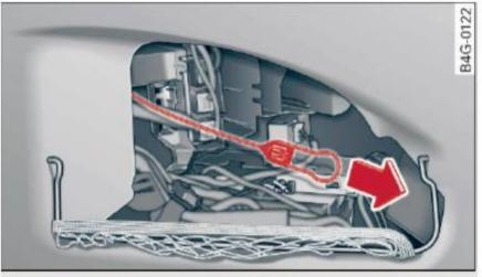
Fig. 179 Luggage compartment: fuel filler door emergency release
