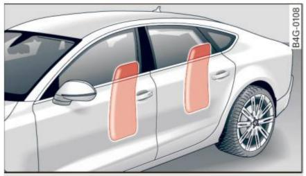
Fig. 162 Inflated side airbags on left side of vehicle, rear side airbag
