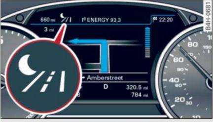
Fig. 111 Instrument cluster: symbol when the infrared image is not visible
