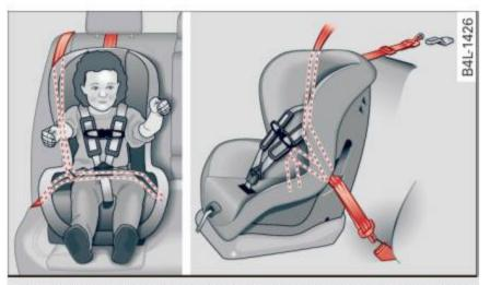
Fig. 168 Schematic overview: installation of the seat using the vehicle's safety belt system
