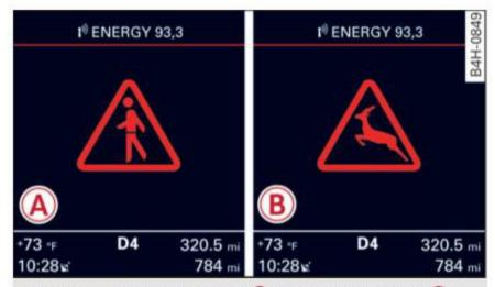
Fig. 113 Instrument cluster: (A) pedestrian warning/(B) wild animal warning, when the night vision assist image is not selected in the instrument cluster display
