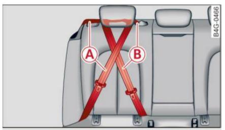
Fig. 165 Schematic overview: keep unused safety belts away from children in child safety seats. (A) - outer rear safety belt, (B) - center rear safety belt\*
