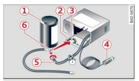
Fig. 199 Components of the tire mobility kit
