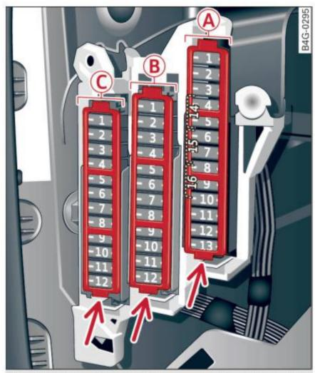
Fig. 211 Driver side cockpit: fuse panel with plastic bracket
