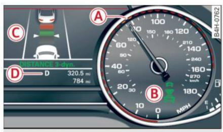
Fig. 95 Instrument cluster: adaptive cruise control
