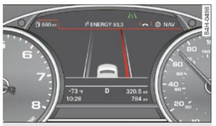
Fig. 103 Instrument cluster: active lane assist is switched on and providing warnings
