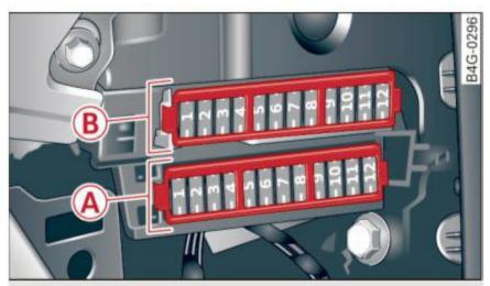
**Fig. 212** Front passenger side cockpit: fuse panel with plastic bracket
