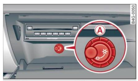
Fig. 59 Glove compartment: switching cooling mode on/
