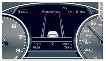
Fig. 104 Instrument cluster: active lane assist is switched on but not ready to provide warnings
