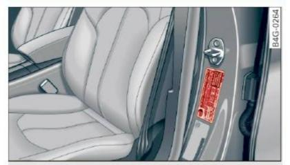
Fig. 192 Driver's side B-pillar: tire pressure label
