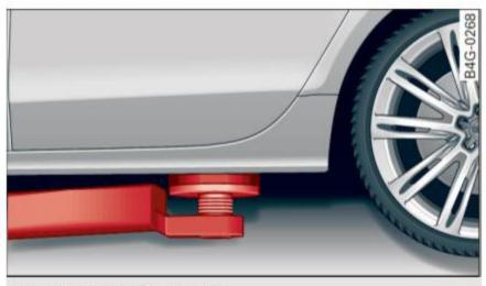
Fig. 222 Rear lifting point
