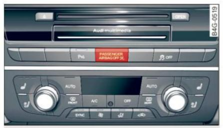
Fig. 158 Section from the instrument panel: PASSENGER AIR BAG OFF light
