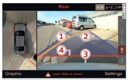
Fig. 135 Infotainment system: aiming at a parking space
