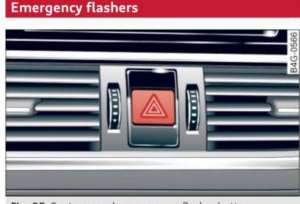
Fig. 35 Center console: emergency flasher button
