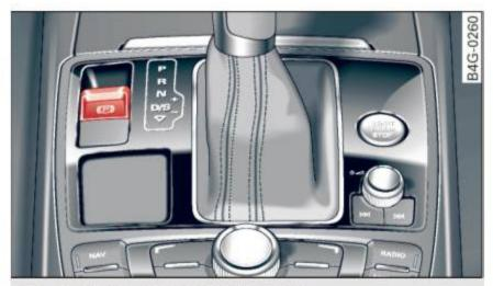
Fig. 80 Center console: parking brake
