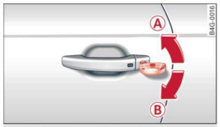
Fig. 22 Driver's door: door lock cylinder
