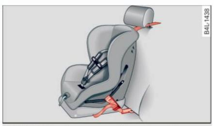
Fig. 175 Tether strap: proper routing and mounting
