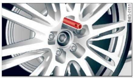
Fig. 208 Changing a wheel: alignment pin inside the top
