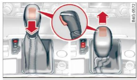
Fig. 82 Selector lever lock
