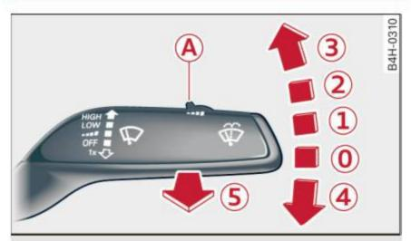
Fig. 43 Windshield wiper lever
