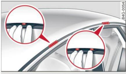
Fig. 60 Attachment points for the roof rack
