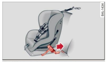
Fig. 173 Lower anchorages: proper mounting
