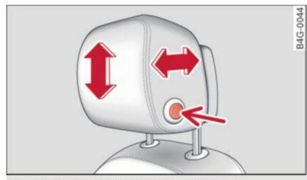
Fig. 48 Front seat: adjusting the head restraint
