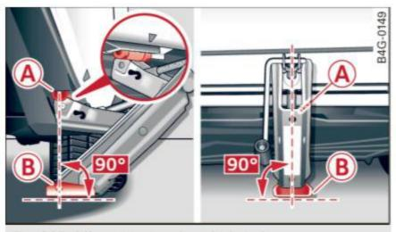
Fig. 205 Sill: positioning the vehicle jack
