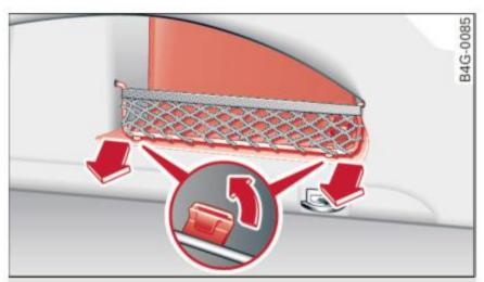
Fig. 178 Right side trim in the luggage compartment: removing the trim
