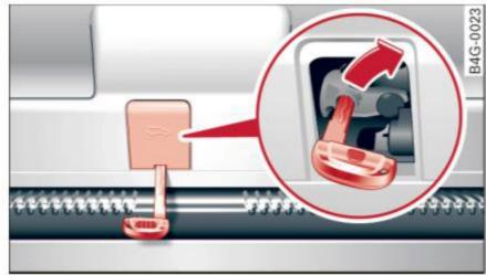
Fig. 27 Inner luggage compartment lid: access to the emergency release
