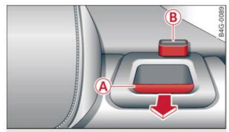
Fig. 61 Backrest: release lever and securing knob
