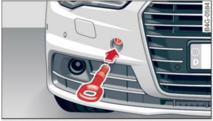
Fig. 217 Front bumper: installing the towing loop
