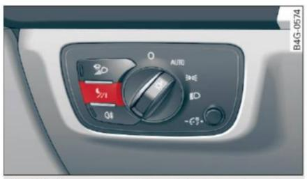
Fig. 115 Area around the light switch: night vision assistant button
