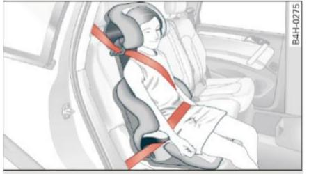
Fig. 169 Rear seat: child properly restrained in a booster seat
