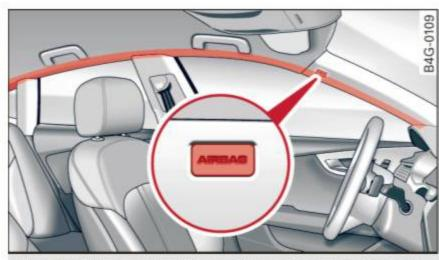
Fig. 163 Side curtain airbags, driver's side: side curtain airbag location
