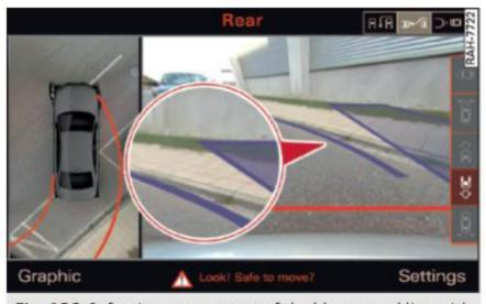
Fig. 138 Infotainment: contact of the blue curved line with the curb
