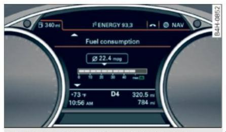
Fig. 8 Instrument cluster: fuel consumption display
