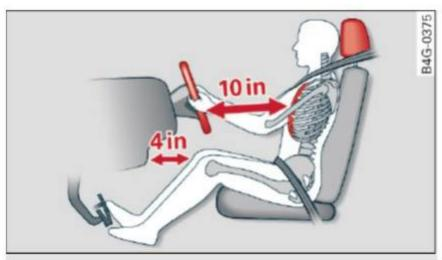
Fig. 142 Correct seating position
