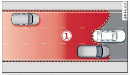
Fig. 105 Sensor detection range
