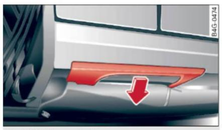
Fig. 206 Sill: removing the cover
