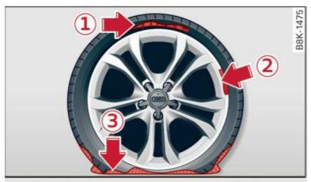
Fig. 198 Tire: tire damage that cannot be repaired
