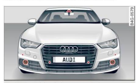
Fig. 91 Front of the vehicle: sensors and video camera
