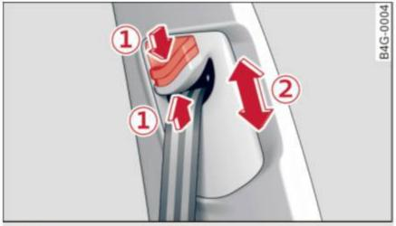
Fig. 154 Safety belt height adjustment for the front seats – loop-around fittings
