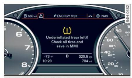
Fig. 194 Instrument cluster: indicator light with message
