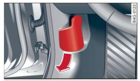
Fig. 182 Driver footwell: release lever
