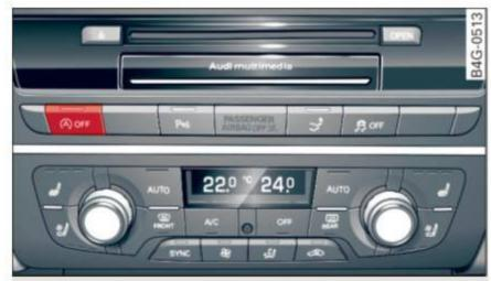
Fig. 79 Center console: Start/Stop system button
