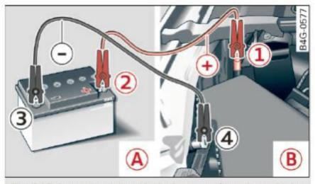
Fig. 215 Jump starting with the battery of another vehicle:
