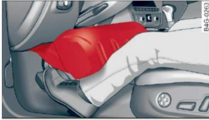
Fig. 160 Inflated airbags protecting in a frontal collision
