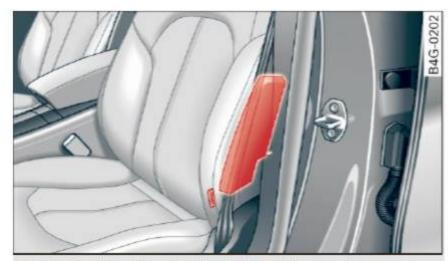
Fig. 161 Side airbag location in the driver's seat
