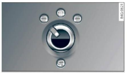
Fig. 39 Driver's door: knob for the exterior mirrors
