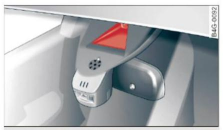
Fig. 101 Windshield: camera window for active lane assist
