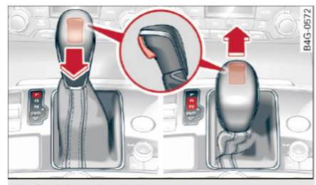
Fig. 84 Selector lever lock
