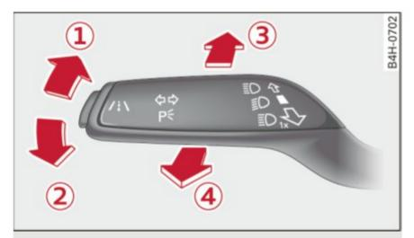
Fig. 38 Turn signal and high beam lever
