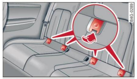
Fig. 169 Lower anchorages, covers marked
