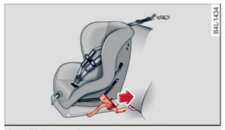
Fig. 171 Lower anchorages: proper mounting
