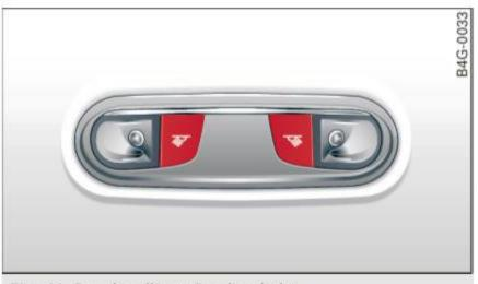
Fig. 41 Rear headliner: Reading light
