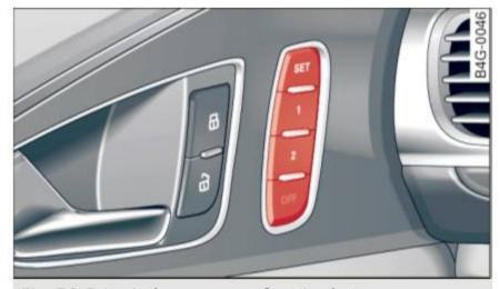
Fig. 56 Driver's door: memory function buttons
