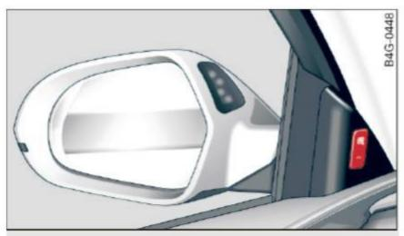
Fig. 108 Driver's door: side assist button
