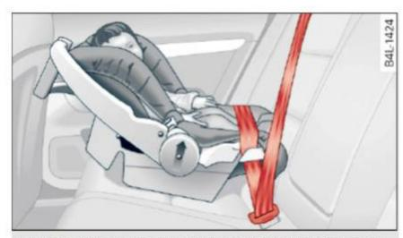
**Fig. 164** Schematic overview: rearward-facing infant seat, properly installed on the rear seat
