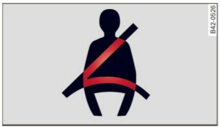
Fig. 142 Safety belt warning light in the instrument cluster - enlarged
