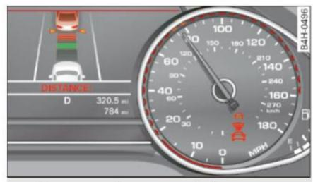
Fig. 98 Instrument cluster: request for driver intervention
