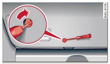
Fig. 29 Inner luggage compartment lid: access to the emergency release
