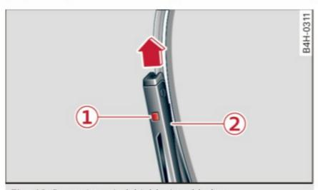
Fig. 49 Removing windshield wiper blades
