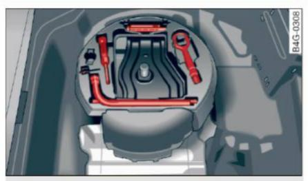
Fig. 194 Luggage compartment: vehicle tool kit
