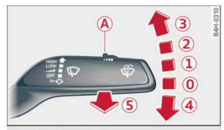
Fig. 48 Windshield wiper lever
