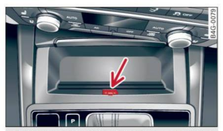
Fig. 87 Front center console: emergency release for the selector lever
