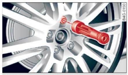
Fig. 201 Changing a wheel: using the screwdriver handle (with the blade removed) to turn the bolts
