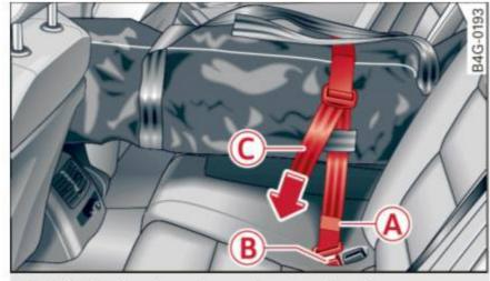
Fig. 71 Rear bench seat: securing the ski sack
