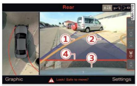
Fig. 134 Infotainment system: aiming at a parking space
