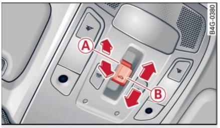
Fig. 33 Section of headliner: sunroof button
