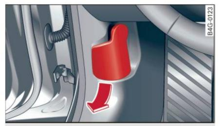
Fig. 180 Driver footwell: release lever
