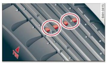
Fig. 189 Tire profile: treadwear indicator
