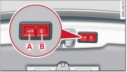
Fig. 27 Luggage compartment lid: (A) closing button, (B) lock button (vehicles with convenience key\*)
