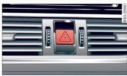
Fig. 39 Center console: emergency flasher button
