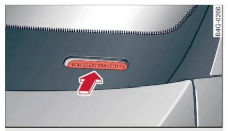
Fig. 217 Windshield (front left): Vehicle Identification Number (VIN)
