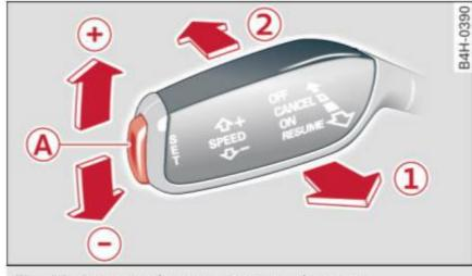
Fig. 88 Operating lever: cruise control system
