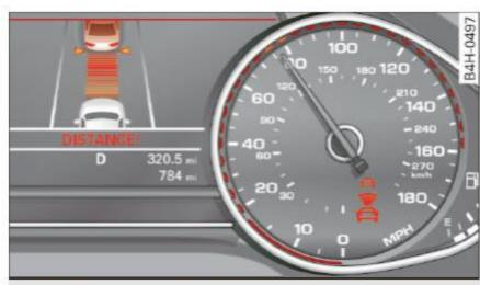
Fig. 99 Instrument cluster: approach warning
