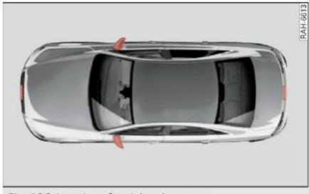
Fig. 126 Location of peripheral cameras
