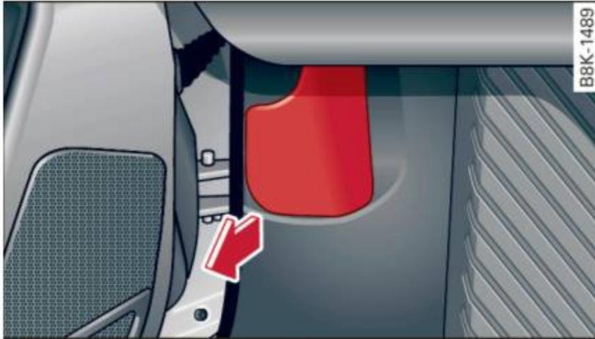
Fig. 159 Driver's side footwell: engine hood release lever
