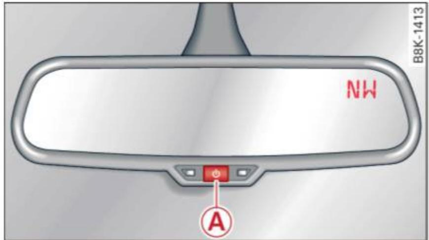
Fig. 50 Rearview mirror: Digital compass activated
