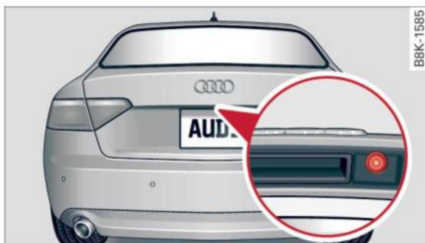
**Fig. 114** Trunk lid: Location of the rear view camera
