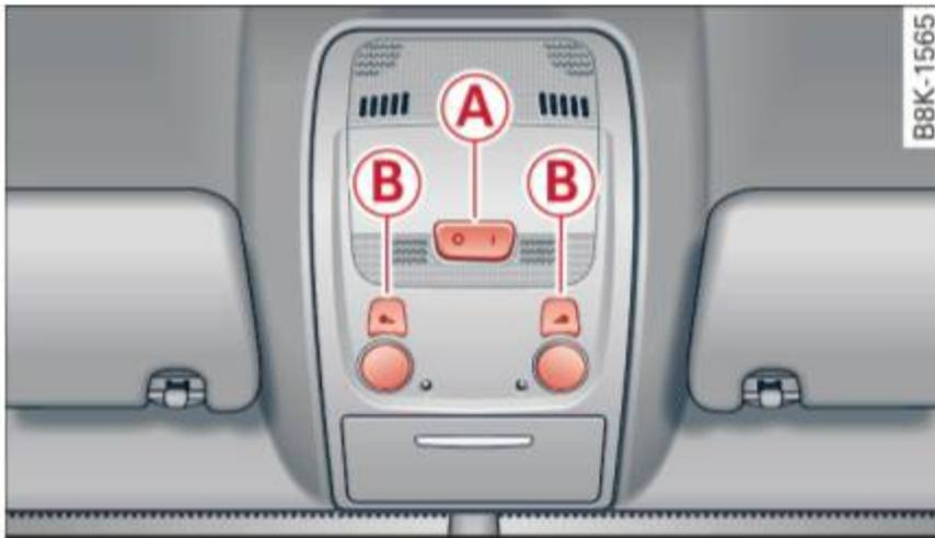
Fig. 40 Front headliner: interior lighting controls
