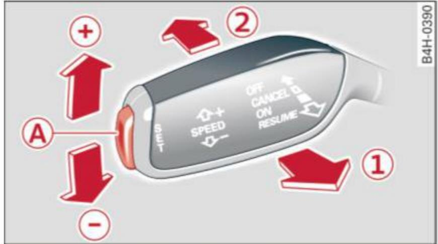
Fig. 83 Control lever with push-button
