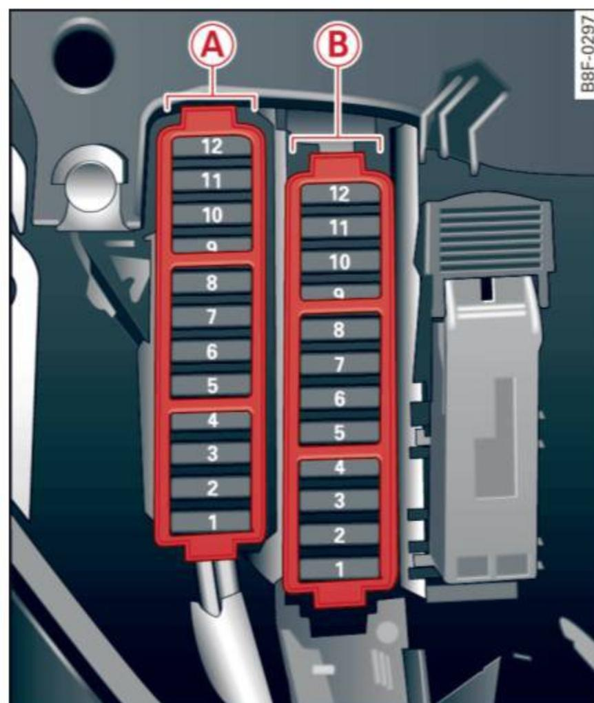
Fig. 184 Right cockpit: fuse panel with plastic clip
