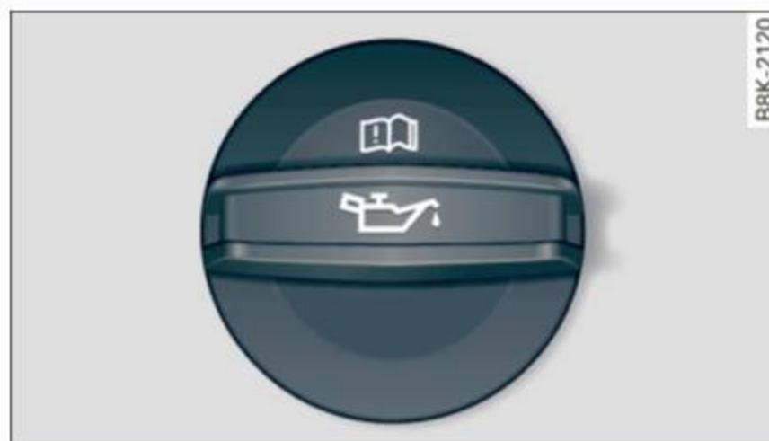
Fig. 163 Engine compartment: Cover on the oil filler neck
