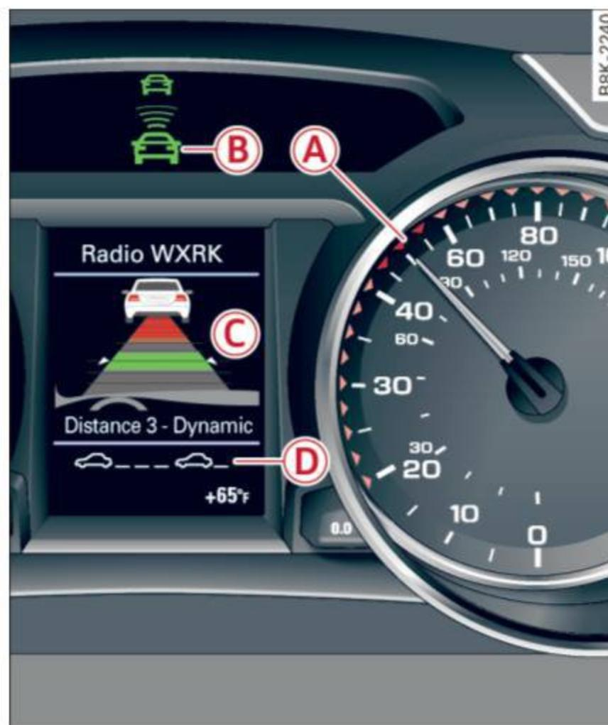
Fig. 98 Instrument cluster: Audi adaptive cruise control
