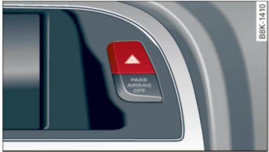
Fig. 39 Center console: emergency flasher switch
