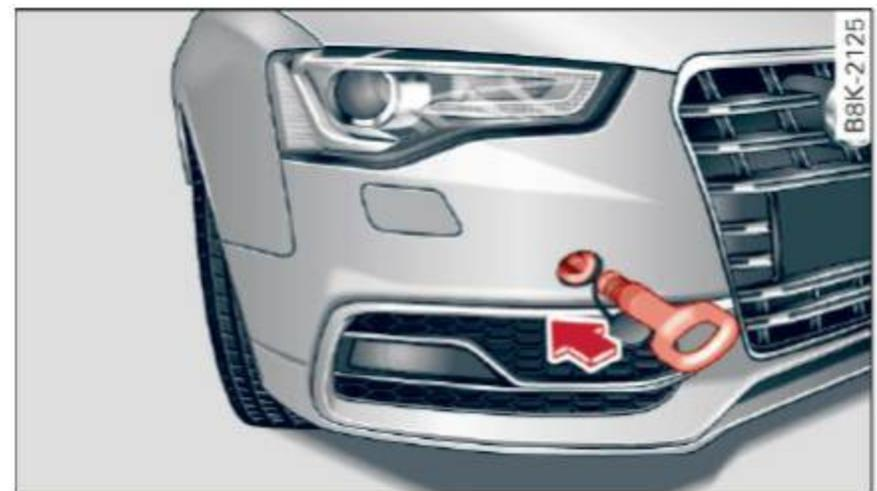
Fig. 189 Front bumper: screwing in the towing loop
