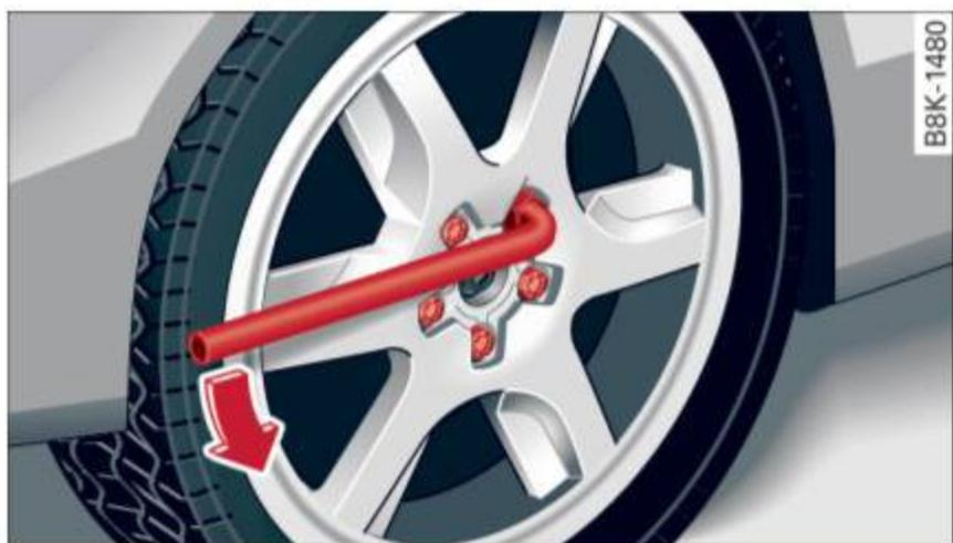
Fig. 177 Changing a wheel: loosening the wheel bolts
