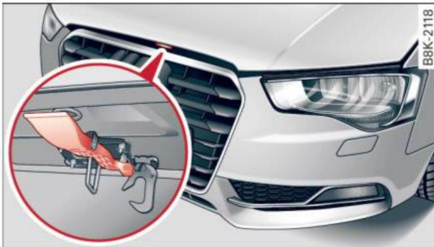
Fig. 160 Release lever under the engine hood
