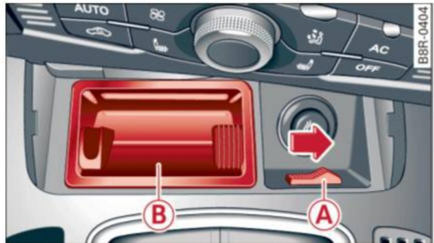
Fig. 91 Front center console: Removing the ashtray insert
