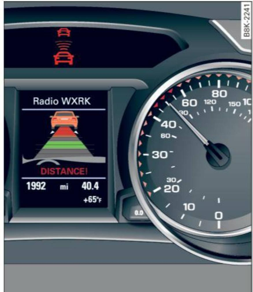
**Fig. 102** Instrument cluster: request for driver intervention
