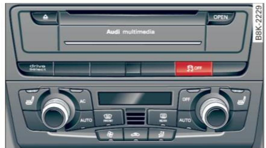
Fig. 154 Version B: upper center console,
