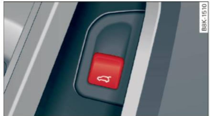
Fig. 27 Driver's door: remote rear lid release
