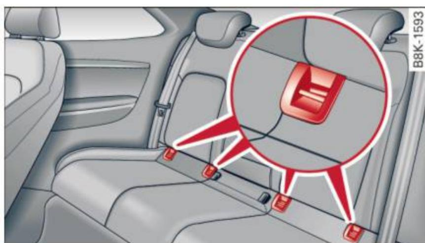
Fig. 149 Rear seats: lower anchorage bracket locations
