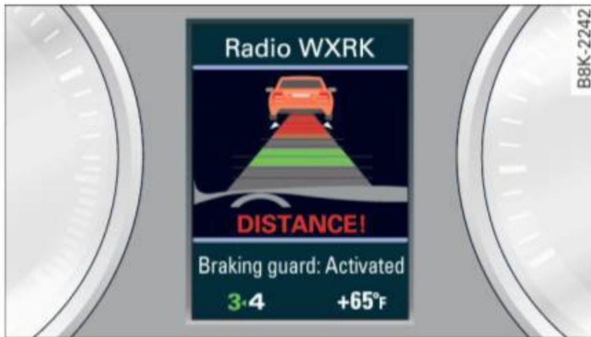
Fig. 103 Instrument cluster: approach warning
