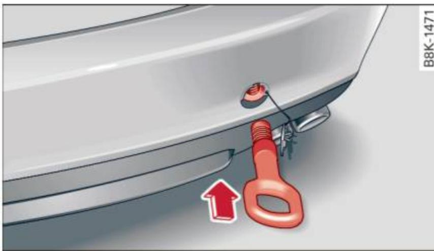
Fig. 191 Rear bumper: Screwing in towing loop
