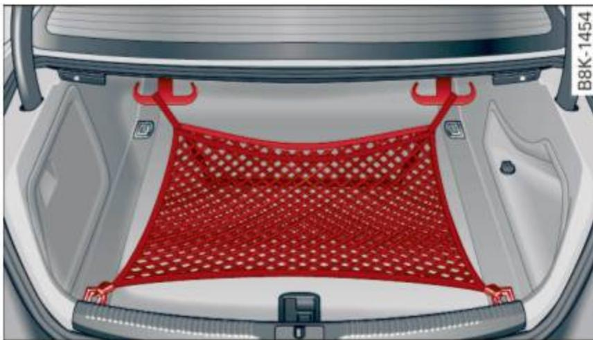
Fig. 70 Luggage compartment: cargo net at the top of the luggage compartment
