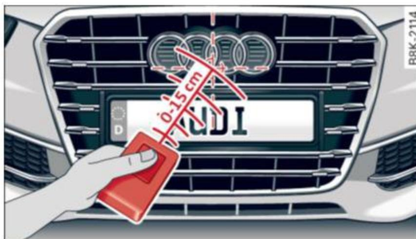
**Fig. 36** Distance between the radiator grille and the hand transmitter
