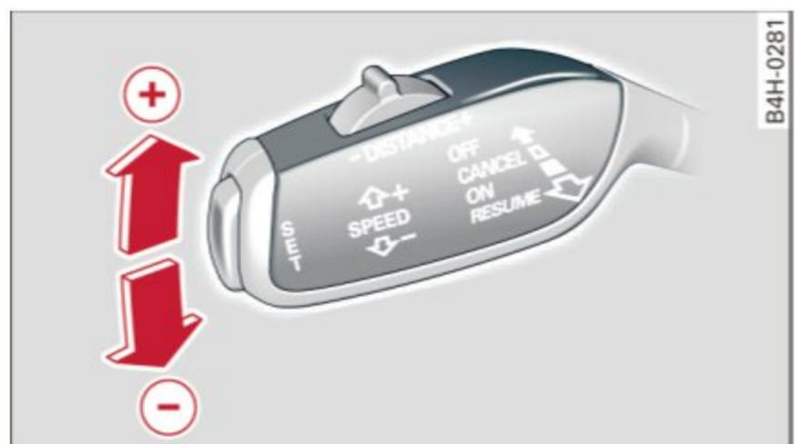
**Fig. 99** Selector lever: changing the speed
