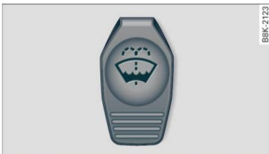
**Fig. 167** Engine compartment: Cover on the windshield and headlight\* washer fluid container
