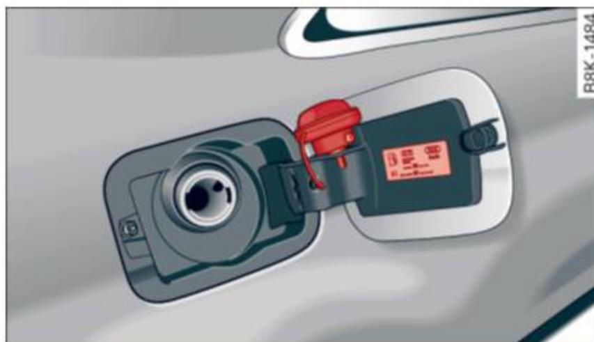
Fig. 156 Fuel filler flap with attached fuel cap
