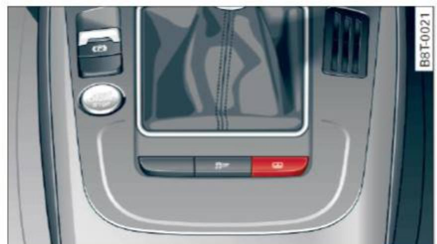
Fig. 47 Without MMI: Button for rear window sun shade
