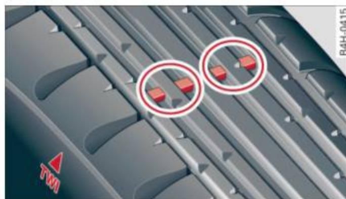
**Fig. 169** Tire profile: Treadwear indicator
