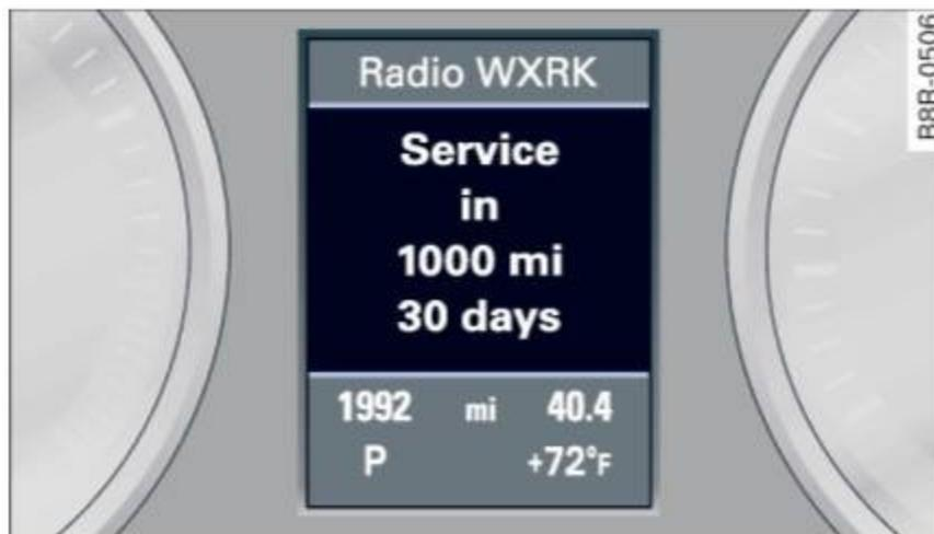
Fig. 17 Display: Service interval display
