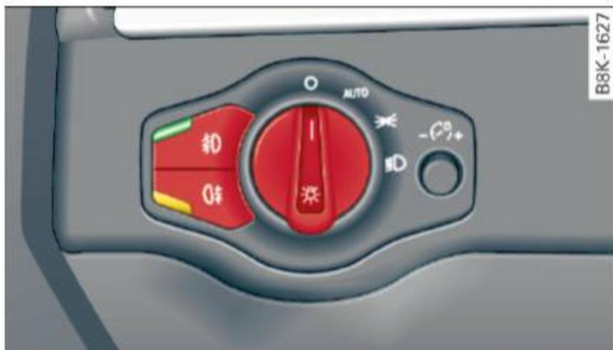
Fig. 37 Instrument panel: headlight control switch
