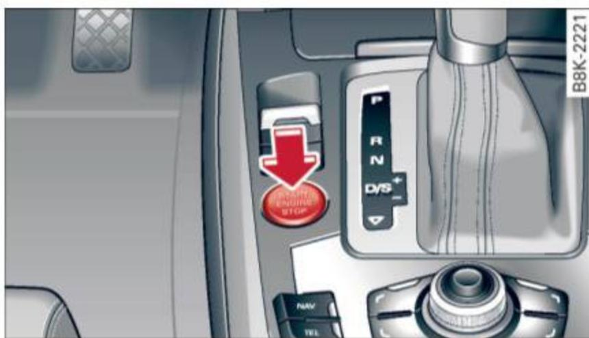
Fig. 80 Center console: START ENGINE STOP button
