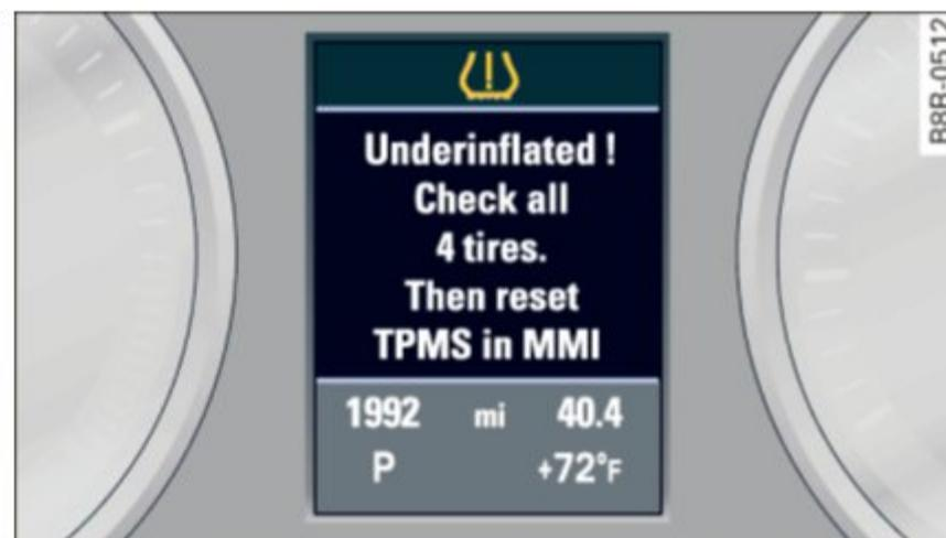
Fig. 172 Instrument cluster: indicator light with message
