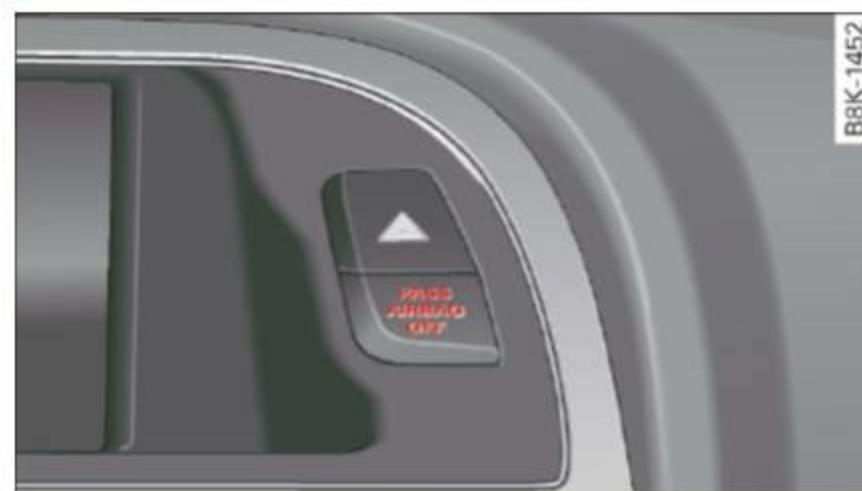
**Fig. 135** Section from the instrument panel: PASSENGER AIR BAG OFF light
