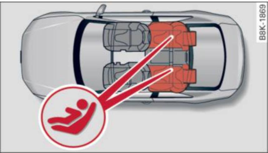
Fig. 147 Schematic overview: LATCH anchorage point locations
