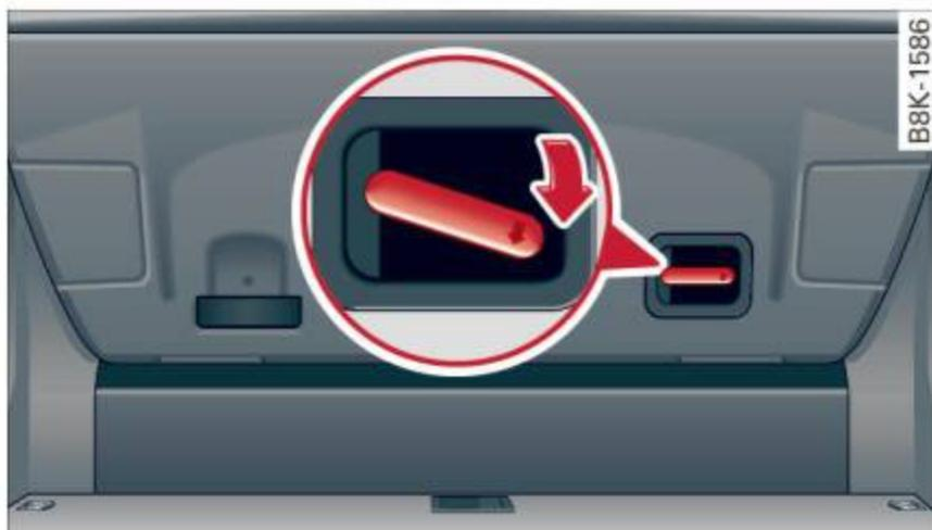
Fig. 29 Trunk escape handle: view from inside the closed rear lid
