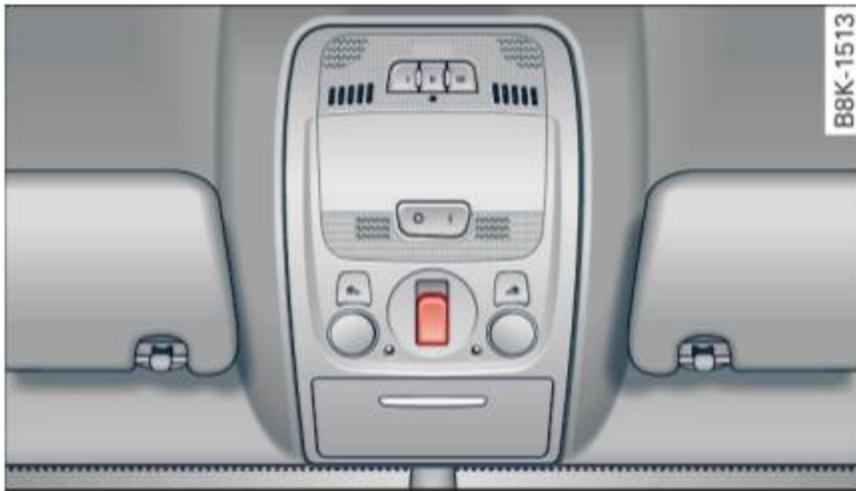
Fig. 32 Section of headliner: switch for sunroof
