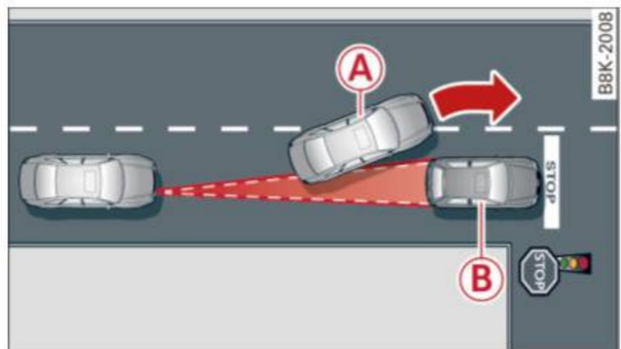
Fig. 95 Example: object changing lanes and stationary object
