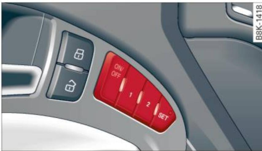
Fig. 60 Driver's door: memory function buttons
