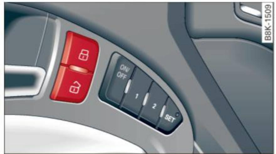
Fig. 24 Driver's door: power locking switch
