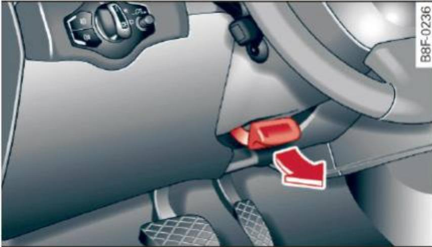
Fig. 76 Lever under the steering column
