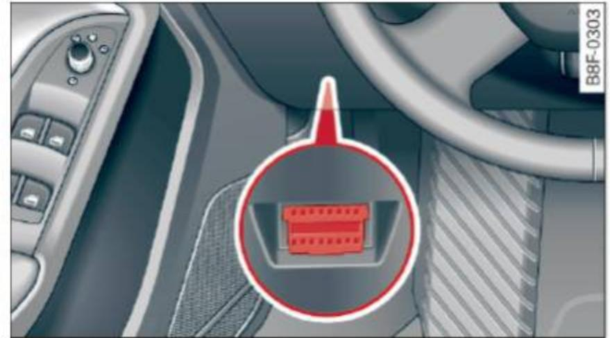
Fig. 18 Location of Data Link Connector (DLC)
