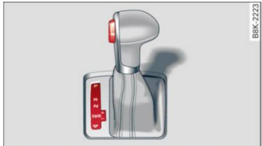
Fig. 88 Shift gate on the center console: selector lever with release button
