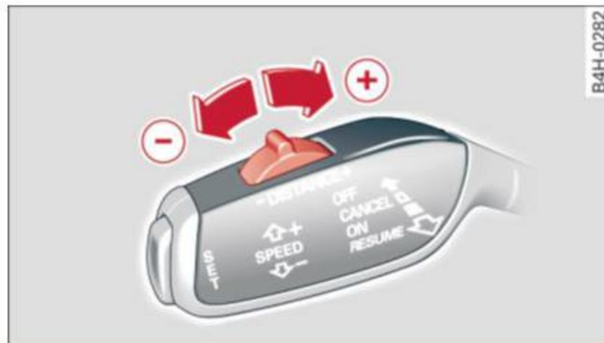
Fig. 101 Selector lever: setting the distance
