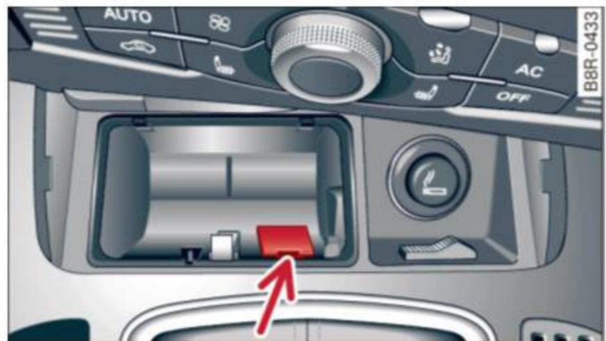
Fig. 92 Selector lever emergency release
