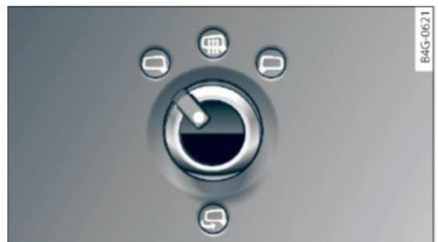
Fig. 43 Driver's door: knob for the exterior mirrors
