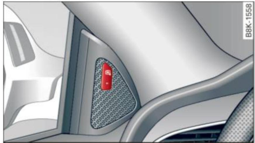
Fig. 108 Driver's door: Side assist button
