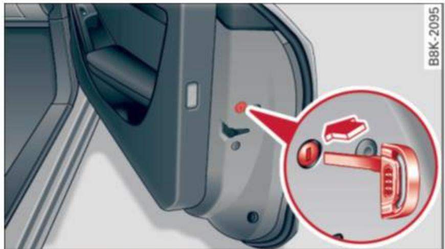
Fig. 26 Front passenger's door: emergency lock
