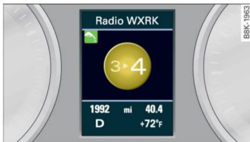
Fig. 14 Display: enhanced shift indicator
