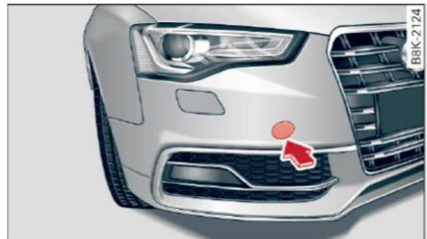
Fig. 188 Front bumper: removing the cover cap
