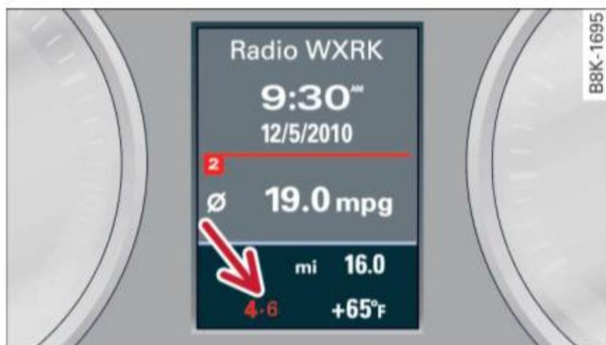
Fig. 12 Display: Gearshift indicator
