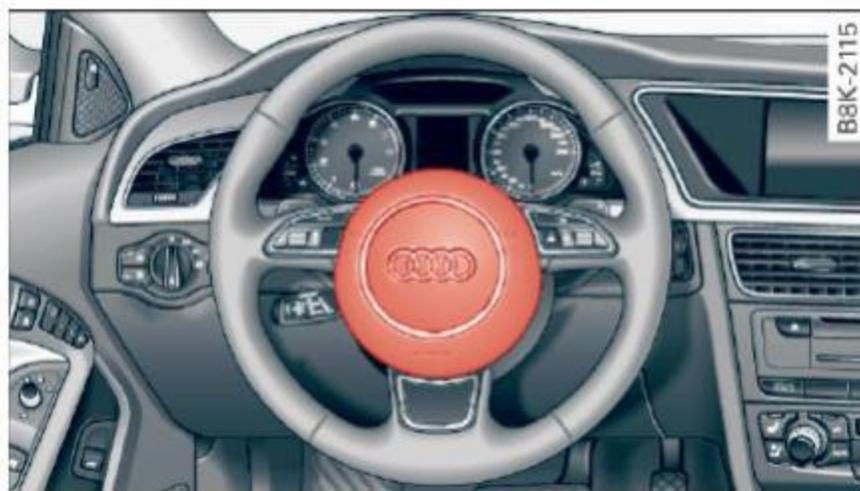
Fig. 132 Location of driver airbag: in steering wheel
