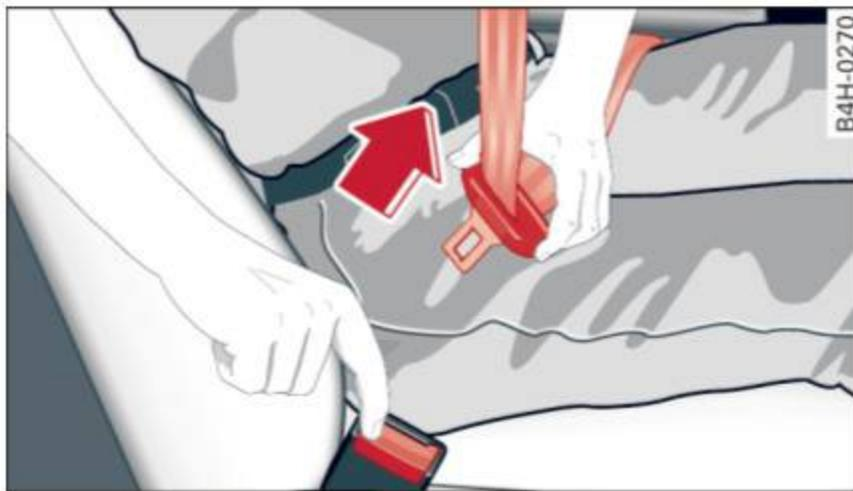
Fig. 131 Releasing the tongue from the buckle
