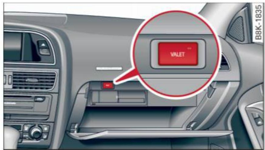
Fig. 33 Glove compartment: valet parking button
