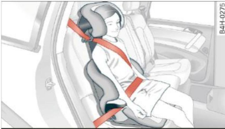
**Fig. 146** Rear seat: child properly restrained in a booster seat
