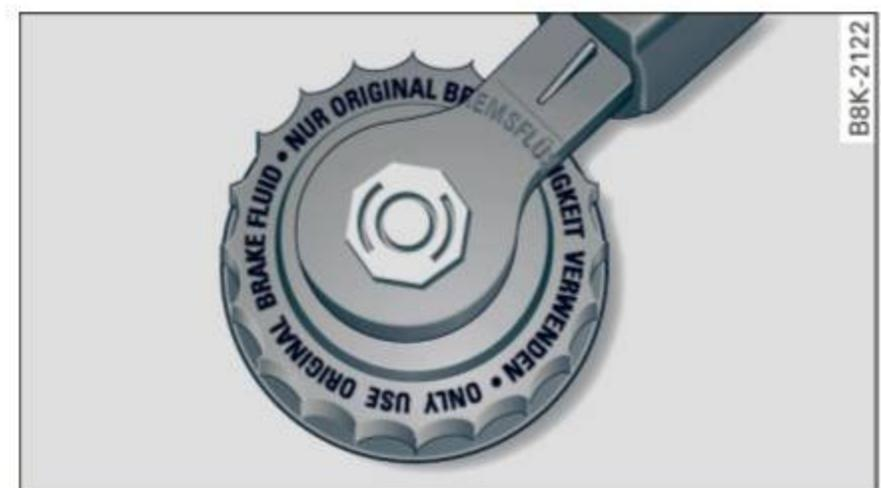
**Fig. 165** Engine compartment: Cover on the brake fluid reservoir
