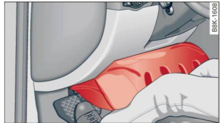
Fig. 137 Inflated airbags protecting in a frontal collision
