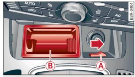
Fig. 91 Front center console: Removing the ashtray insert
