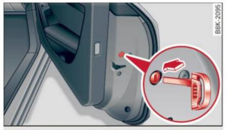
Fig. 26 Front passenger's door: emergency lock
