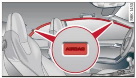
Fig. 140 Side curtain system, driver's side: side curtain airbag location
