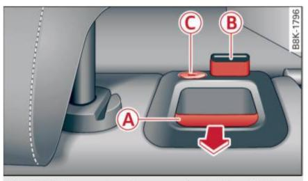
Fig. 68 Backrest: release lever, securing knob and latch
