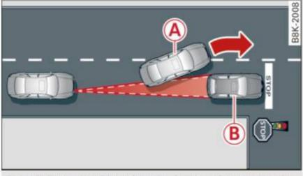
**Fig. 95** Example: object changing lanes and stationary object
