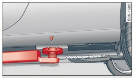
Fig. 194 Rear lifting point
