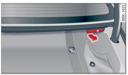
Fig. 67 Luggage compartment: release lever
