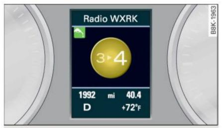
Fig. 14 Display: enhanced shift indicator
