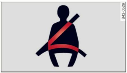
Fig. 122 Safety belt warning light in the instrument cluster - enlarged
