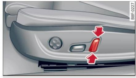
Fig. 57 Front seat: adjusting the power head restraint
