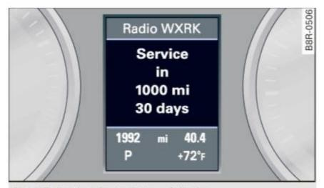
Fig. 17 Display: Service interval display
