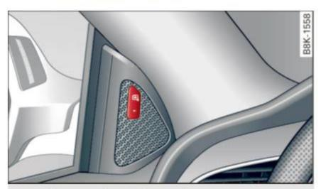
Fig. 108 Driver's door: Side assist button
