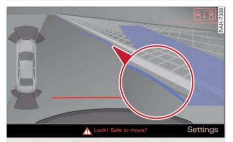
Fig. 118 MMI Display: Blue curve on the curb
