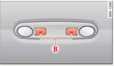
Fig. 41 Rear headliner: rear reading lights
