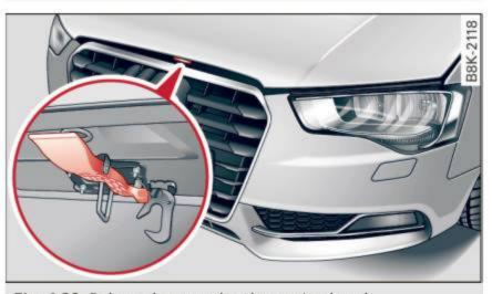
Fig. 160 Release lever under the engine hood
