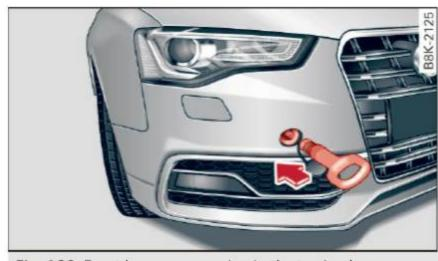
Fig. 189 Front bumper: screwing in the towing loop
