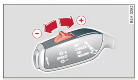
Fig. 101 Selector lever: setting the distance
