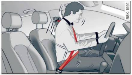
Fig. 127 Driver is correctly restrained in a sudden braking maneuver
