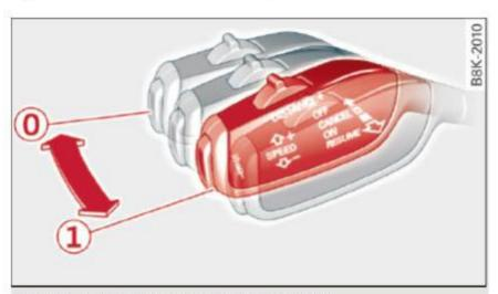
Fig. 97 Selector lever: switching on/off
