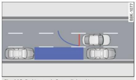
Fig. 112 Parking mode 2: parallel parking
