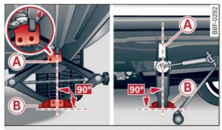
Fig. 179 Sill: positioning the vehicle jack
