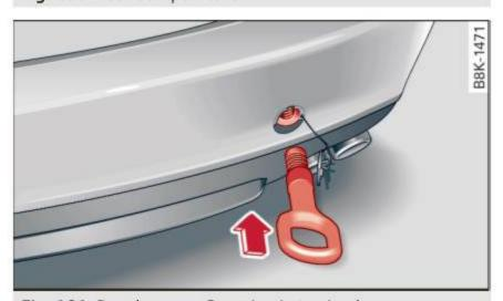
Fig. 191 Rear bumper: Screwing in towing loop
