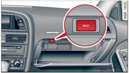
Fig. 33 Glove compartment: valet parking button
