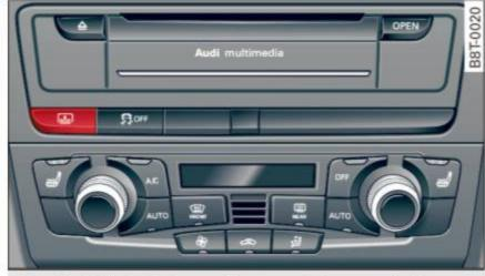
Fig. 46 With MMI: Button for rear window sun shade
