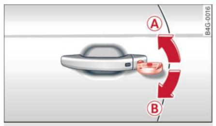
Fig. 25 Driver's door: lock cylinder
