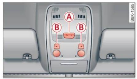
Fig. 40 Front headliner: interior lighting controls
