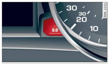
Fig. 6 Instrument cluster: reset button
