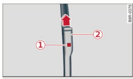
Fig. 49 Removing windshield wiper blade
