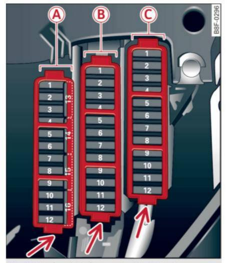
Fig. 183 Left cockpit: fuse panel with plastic clip
