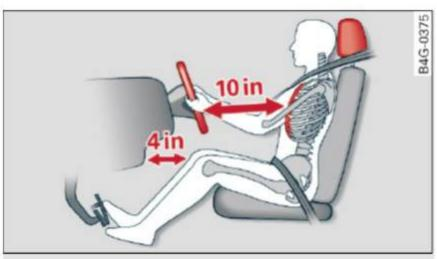
Fig. 119 Correct seating position
