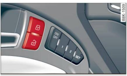
Fig. 24 Driver's door: power locking switch
