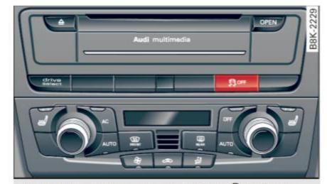
Fig. 154 Version B: upper center console, 🕏 OFF button
