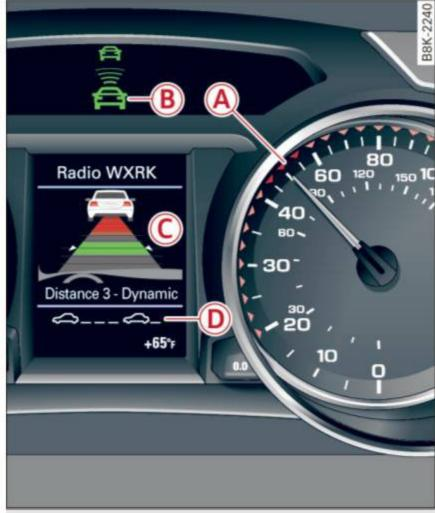
Fig. 98 Instrument cluster: Audi adaptive cruise control
