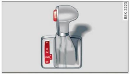
Fig. 88 Shift gate on the center console: selector lever with release button
