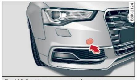
Fig. 188 Front bumper: removing the cover cap
