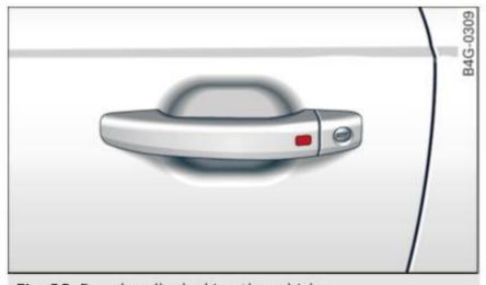
Fig. 23 Door handle: locking the vehicle
