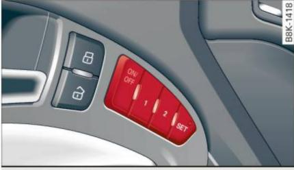
Fig. 60 Driver's door: memory function buttons
