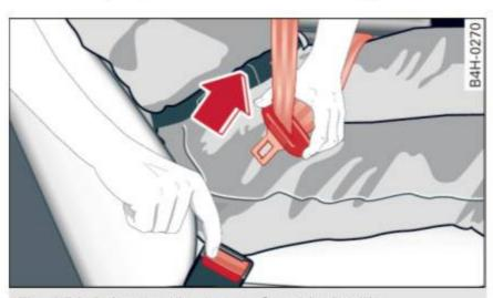
Fig. 131 Releasing the tongue from the buckle
