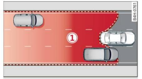
Fig. 104 Sensor detection range
