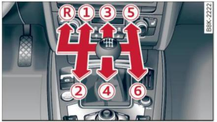
Fig. 85 Gearshift pattern: 6-speed manual transmission
