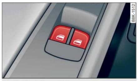
Fig. 30 Driver's door: controls
