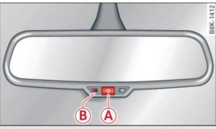
Fig. 44 Automatic dimming rearview mirror\*
