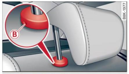
Fig. 59 Rear head restraints: release
