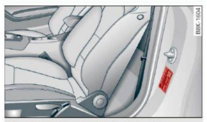
Fig. 170 Driver's side B-pillar: tire pressure label
