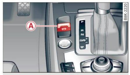
Fig. 81 Center console: Parking brake
