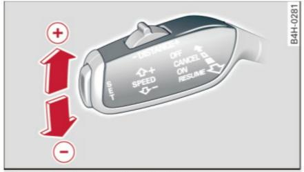
Fig. 99 Selector lever: changing the speed
