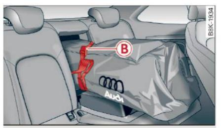
Fig. 73 Rear bench seat: securing the ski sack
