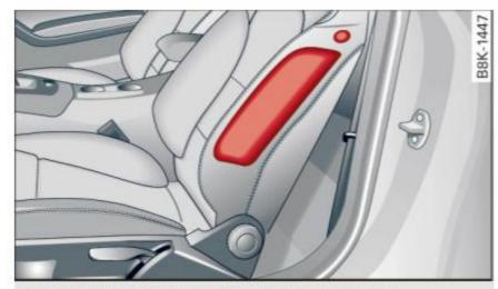
Fig. 138 Side airbag location in the driver's seat
