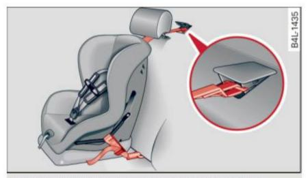
Fig. 152 Tether strap: proper routing and mounting
