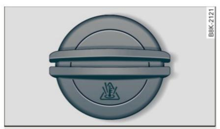
**Fig. 164** Engine compartment: Cover on the coolant expansion tank
