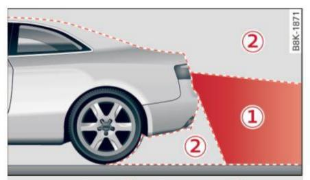
Fig. 113 Covered area 1 and uncovered area 2 of the rear view camera
