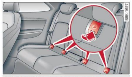
Fig. 148 Lower anchorages, covers marked
