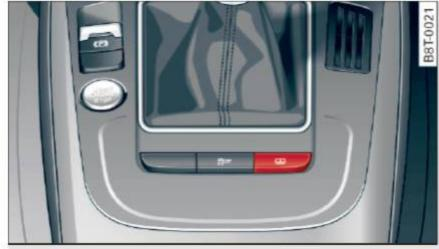
Fig. 47 Without MMI: Button for rear window sun shade
