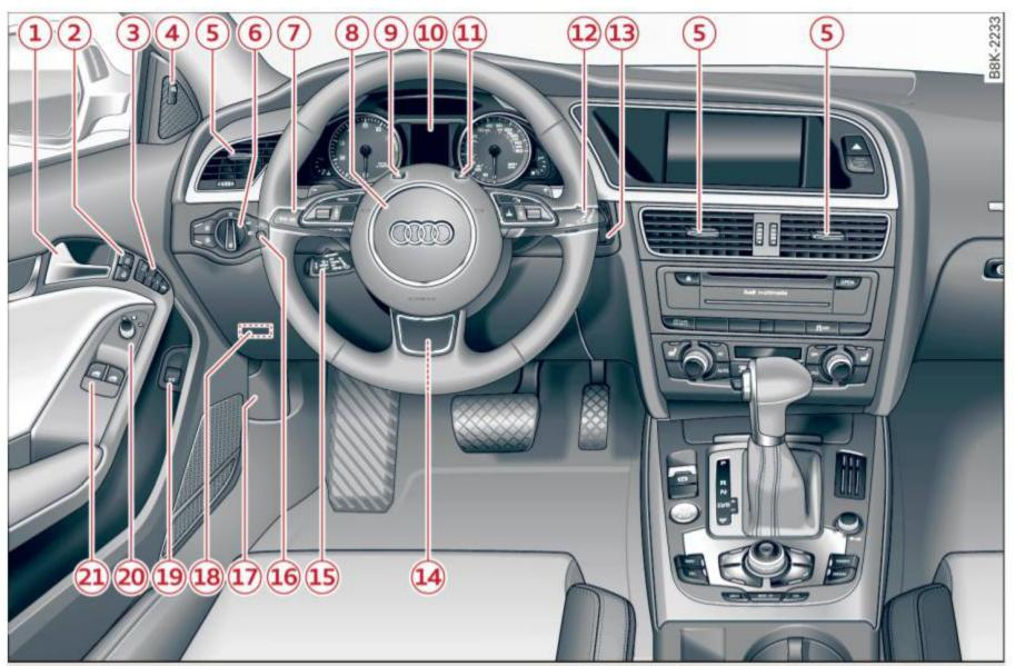
Fig. 1 Cockpit: left section
