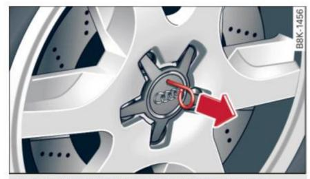
Fig. 175 Changing a wheel: removing the wheel cover
