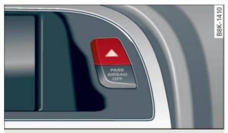
Fig. 39 Center console: emergency flasher switch
