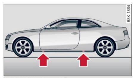
Fig. 178 Sill panels: markings
