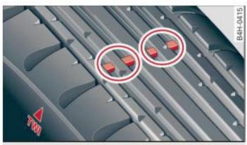
Fig. 169 Tire profile: Treadwear indicator
