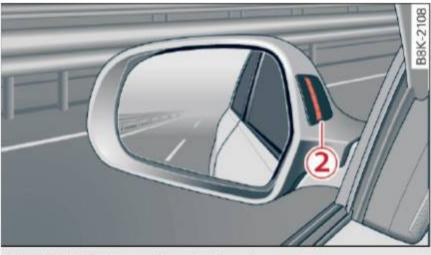
Fig. 105 Display on the exterior mirror
