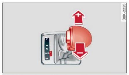
Fig. 89 Center console: shifting the gears manually
