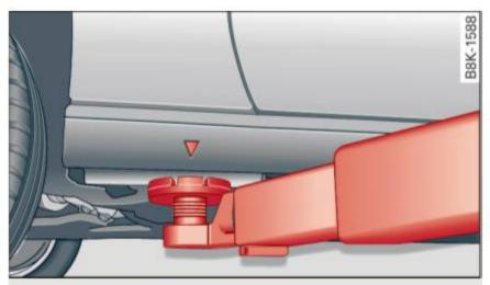
Fig. 193 Front lifting point
