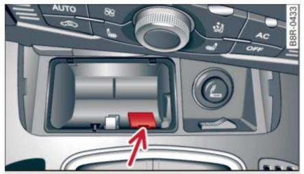
Fig. 92 Selector lever emergency release
