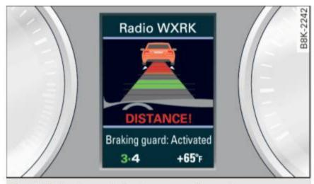
Fig. 103 Instrument cluster: approach warning
