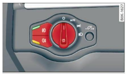
Fig. 37 Instrument panel: headlight control switch
