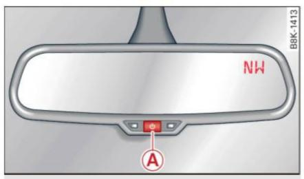
Fig. 50 Rearview mirror: Digital compass activated
