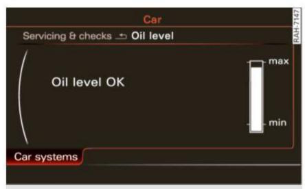
Fig. 162 MMI Display: Oil level indicator
