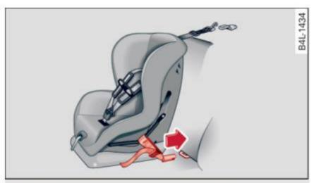
Fig. 150 Lower anchorages: proper mounting
