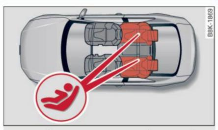
Fig. 147 Schematic overview: LATCH anchorage point locations
