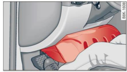
Fig. 137 Inflated airbags protecting in a frontal collision
