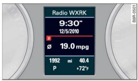
Fig. 7 Instrument cluster: center display
