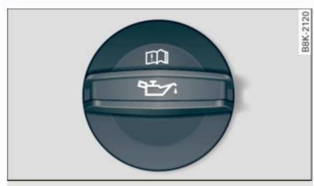
Fig. 163 Engine compartment: Cover on the oil filler neck
