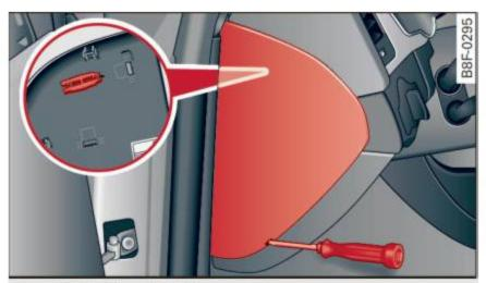
Fig. 182 Left cockpit: fuse panel cover
