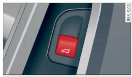
Fig. 27 Driver's door: remote rear lid release
