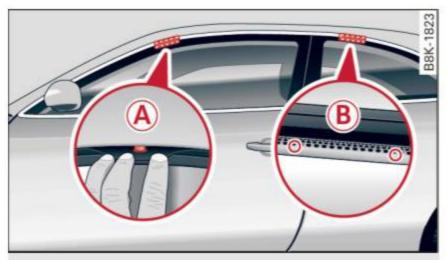
Fig. 66 Roof rack attachment points
