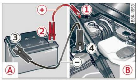
Fig. 187 Jump starting with the battery of another vehicle:
