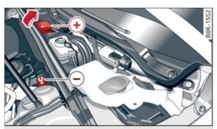
Fig. 186 Engine compartment: Connectors for jumper cables and charger
