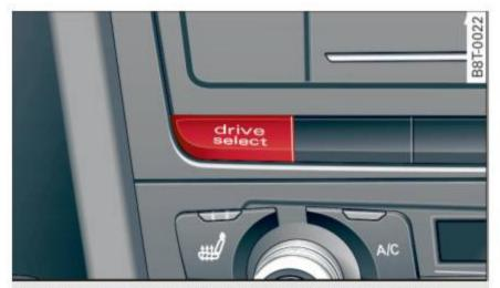
Fig. 109 Center console: Control for Audi drive select
