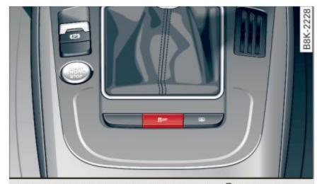
Fig. 153 Version A: lower center console, \$ OFF button
