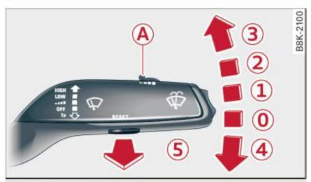
Fig. 48 Windshield wiper lever
