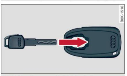
Fig. 79 Insert emergency key into the adapter
