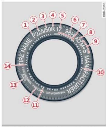
Fig. 168 Tire designations on the sidewall
