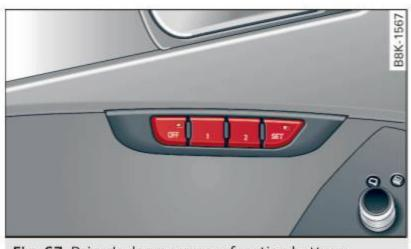
Fig. 67 Driver's door: memory function buttons
