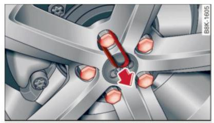
Fig. 201 Changing a wheel: removing the wheel bolt caps
