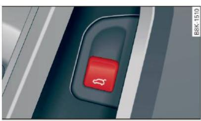
Fig. 29 Driver's door: Unlocking the rear lid
