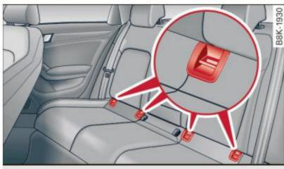
Fig. 168 Rear seats: lower anchorage bracket locations
