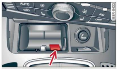
Fig. 112 Selector lever emergency release
