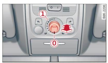
Fig. 37 Section of headliner: knob for sunroof
