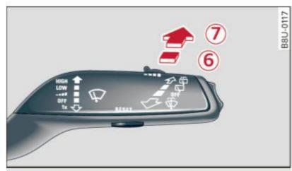
Fig. 56 allroad: Rear wiper actuation
