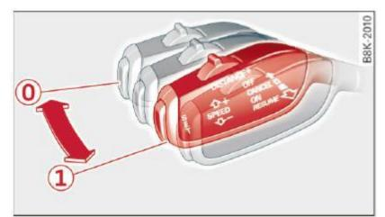
Fig. 117 Selector lever: switching on/off
