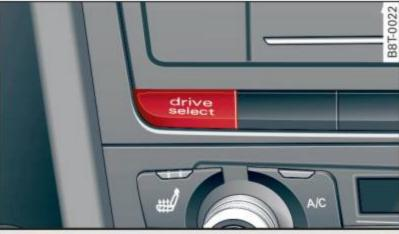
Fig. 129 Center console: Control for Audi drive select
