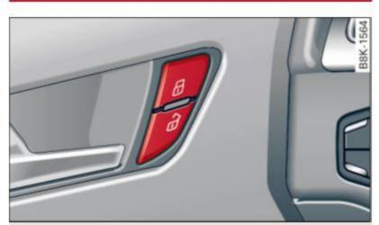
Fig. 24 Driver's door: power locking switch
