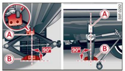
Fig. 204 Sill: positioning the vehicle jack
