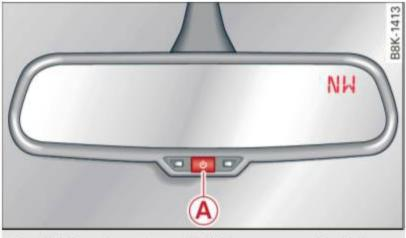
Fig. 59 Rearview mirror: Digital compass activated
