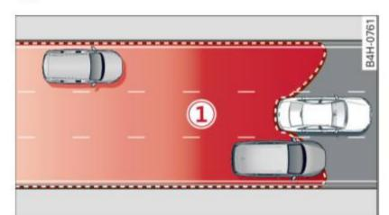
Fig. 124 Sensor detection range
