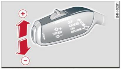
Fig. 119 Selector lever: changing the speed
