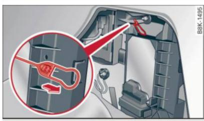
**Fig. 179** Luggage compartment: Emergency opening of fuel filler flap
