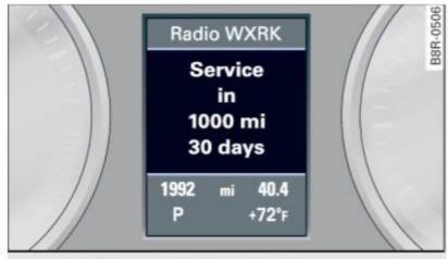
Fig. 17 Display: Service interval display
