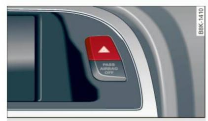
Fig. 45 Center console: emergency flasher switch
