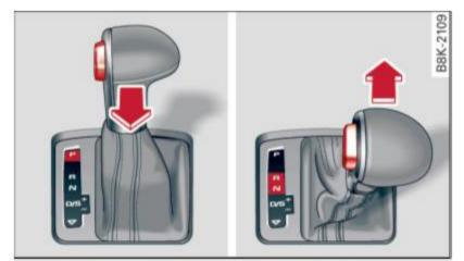
Fig. 107 Shift gate: selector lever lock positions and release button highlighted
