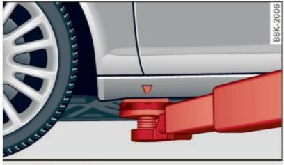
Fig. 218 Front lifting point
