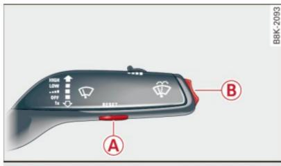
Fig. 11 Windshield wiper lever: controls for the trip computer
