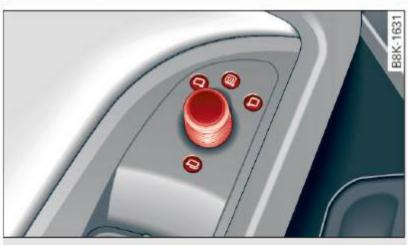
Fig. 49 Forward section of driver's armrest: power mirror controls
