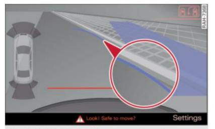
Fig. 138 MMI Display: Blue curve on the curb
