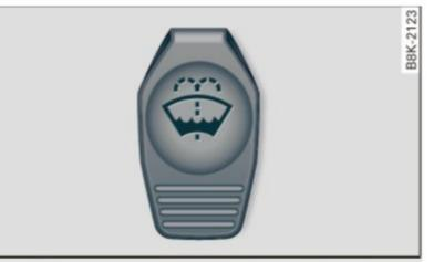
**Fig. 188** Engine compartment: Cover on the windshield and headlight\* washer fluid container
