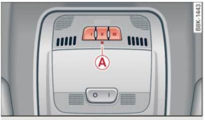
Fig. 41 Headliner: control unit
