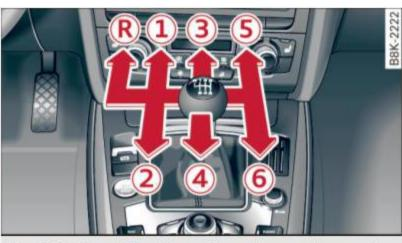
Fig. 105 Gearshift pattern: 6-speed manual transmission
