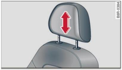
Fig. 64 Front seat: adjusting the head restraints
