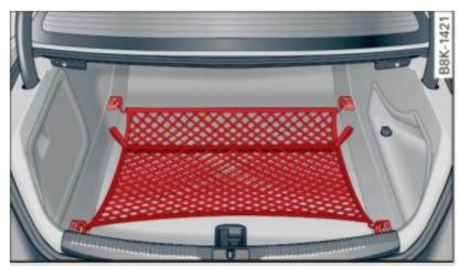
Fig. 84 Luggage compartment: cargo net stretched out
