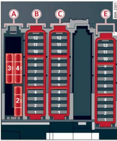
Fig. 210 Right luggage compartment: fuse panel with plastic clip
