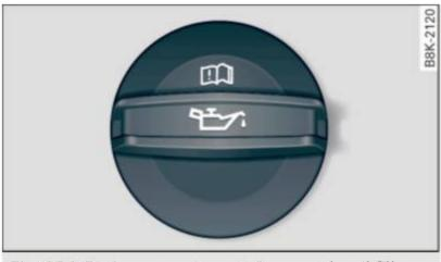
Fig. 184 Engine compartment: Cover on the oil filler neck
