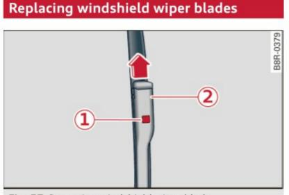
Fig. 57 Removing windshield wiper blade
