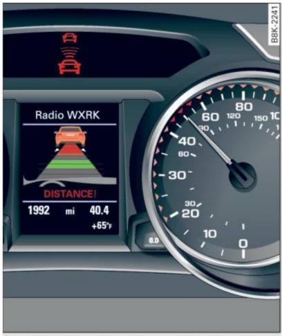
Fig. 122 Instrument cluster: request for driver intervention
