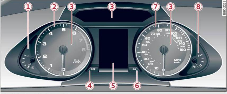
Fig. 3 Overview of the instrument cluster
