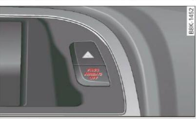
Fig. 156 Section from the instrument panel: PASSEN-GER AIR BAG OFF light
