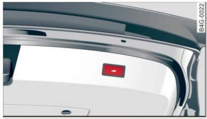
Fig. 30 Locking switch in the rear lid
