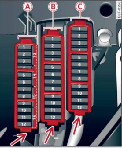
Fig. 208 Left cockpit: fuse panel with plastic clip
