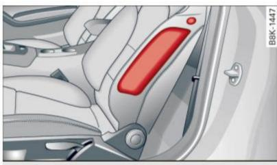
Fig. 157 Side airbag location in the driver's seat
