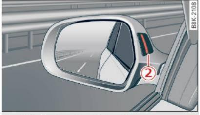
Fig. 125 Display on the exterior mirror
