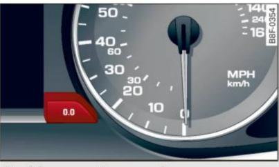
Fig. 6 Instrument cluster: reset button
