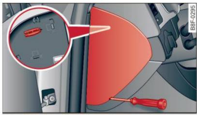
Fig. 207 Left cockpit: fuse panel cover
