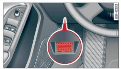
Fig. 18 Location of Data Link Connector (DLC)
