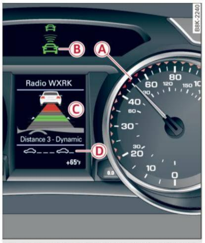
Fig. 118 Instrument cluster: Audi adaptive cruise control
