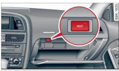
Fig. 39 Glove compartment: valet parking button
