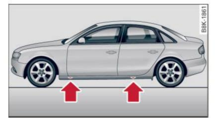
Fig. 203 Sill panels: markings
