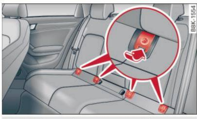
Fig. 167 Lower anchorages, covers marked
