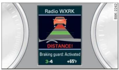
Fig. 123 Instrument cluster: approach warning
