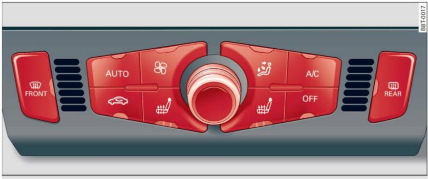
Fig. 94 Automatic climate control system: control
