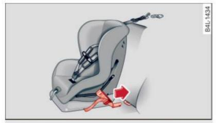
Fig. 169 Lower anchorages: proper mounting
