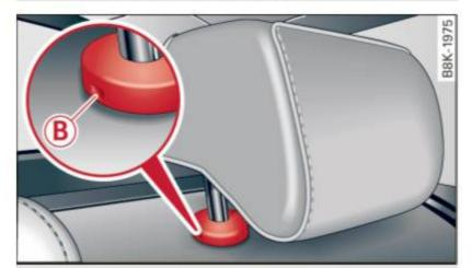
Fig. 66 Rear head restraints: release
