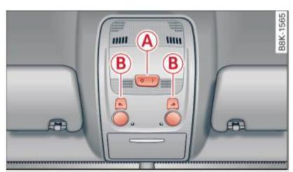
Fig. 46 Front headliner: interior lighting controls
