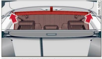
Fig. 80 Behind the backrest: hanging the partition net
