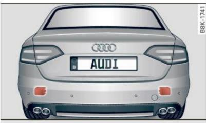
Fig. 127 Rear of the vehicle: position of the sensors
