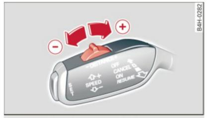
Fig. 121 Selector lever: setting the distance
