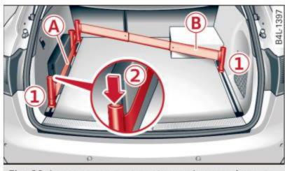
Fig. 89 Luggage compartment: securing attachments
