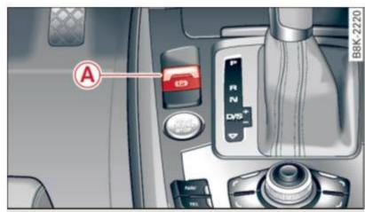
Fig. 101 Center console: Parking brake
