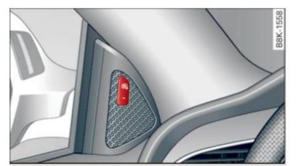
Fig. 128 Driver's door: Side assist button
