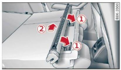
Fig. 82 Folded backrest: installing the partition net
