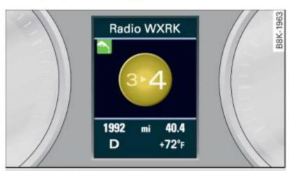
Fig. 14 Display: enhanced shift indicator
