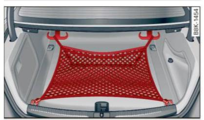
Fig. 85 Luggage compartment: cargo net at the top of the luggage compartment
