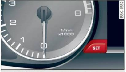
Fig. 102 SET button in the instrument cluster
