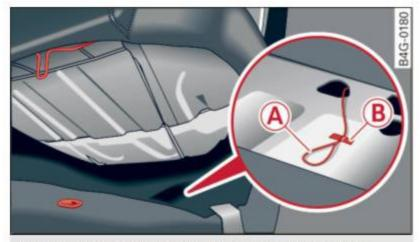
Fig. 31 Rear bench seat: emergency release cable
