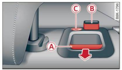
**Fig. 79** Backrest: release lever, securing knob and latch\*
