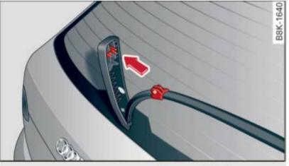
Fig. 58 Rear wiper: Removing the wiper blade
