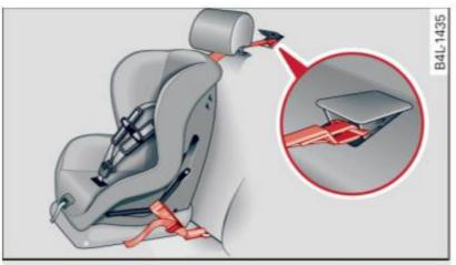
Fig. 172 Sedan Tether strap: proper routing and mounting
