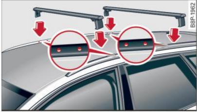
Fig. 76 allroad: Roof rack attachment points
