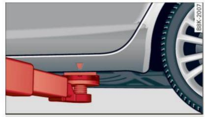
Fig. 219 Rear lifting point
