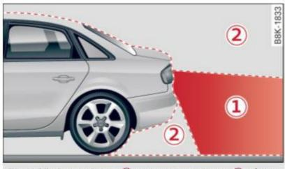
Fig. 133 Covered area (1) and uncovered area (2) of the rear view camera
