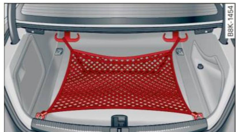
Fig. 85 Luggage compartment: cargo net at the top of the luggage compartment
