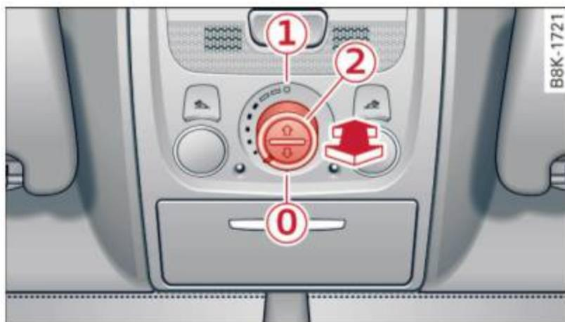
Fig. 38 Section from headliner: knob for sunroof.
