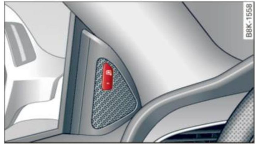
Fig. 128 Driver's door: Side assist button
