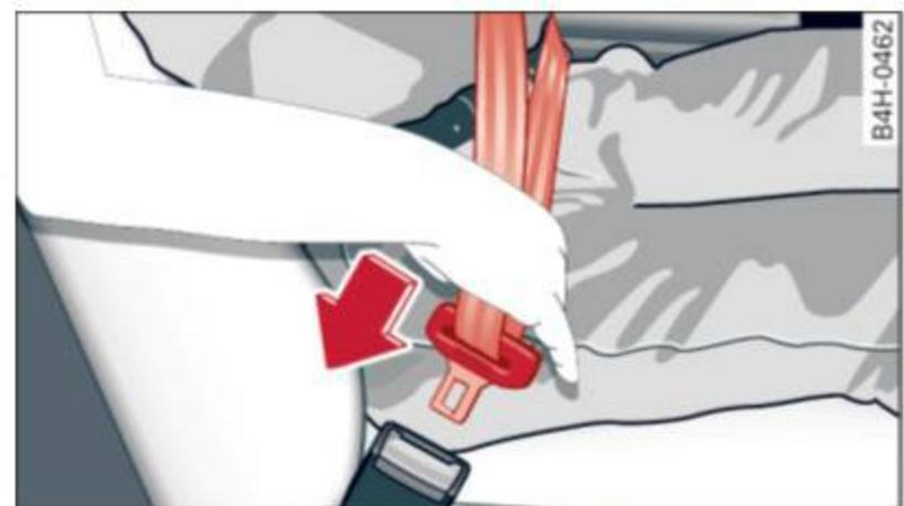
**Fig. 148** Belt buckle and tongue on the driver's seat
