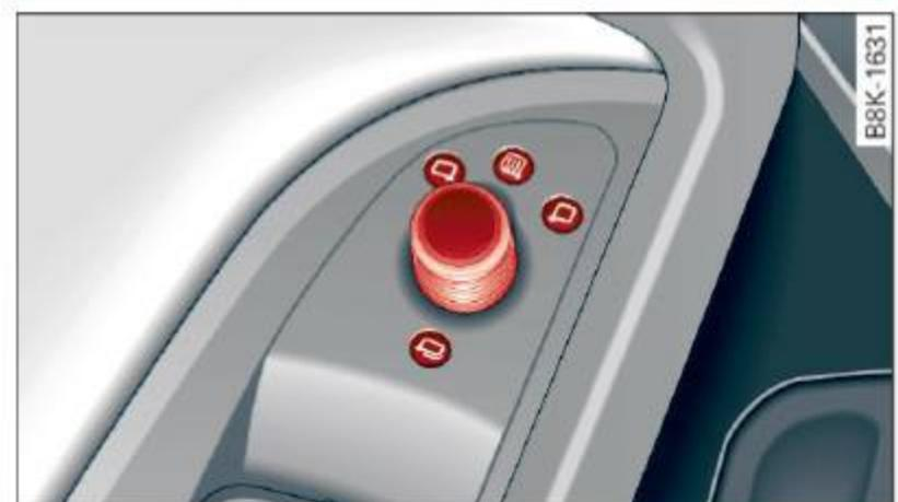
Fig. 49 Forward section of driver's armrest: power mirror controls
