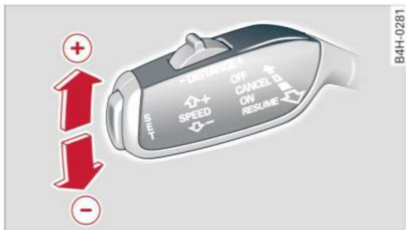
Fig. 119 Selector lever: changing the speed
