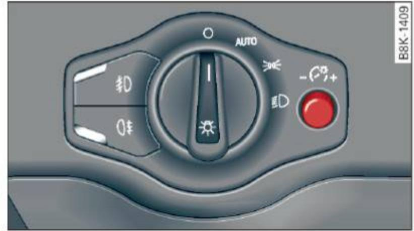
Fig. 48 Instrument illumination
