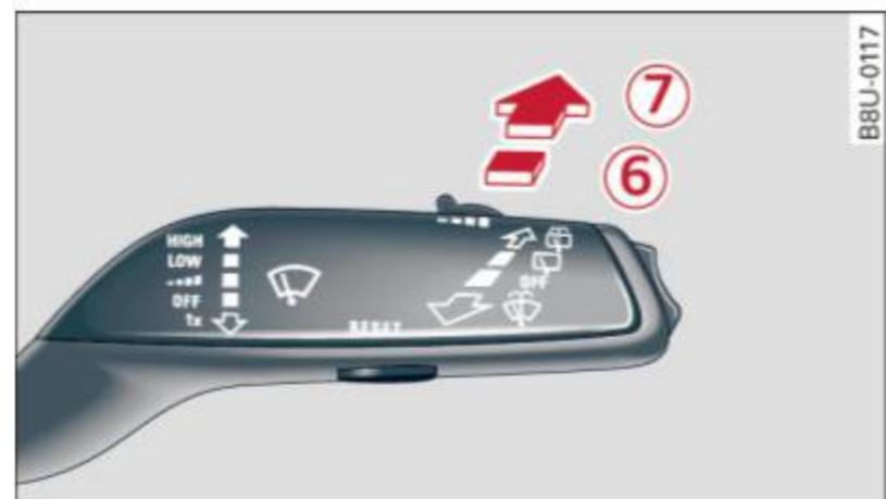
Fig. 56 allroad: Rear wiper actuation
