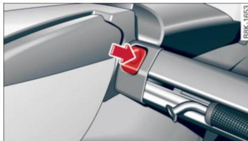
Fig. 81 Behind the backrest: removing the partition net
