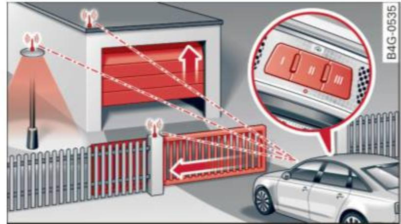
Fig. 40 Garage door opener: examples of using with different systems
