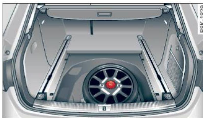
Fig. 198 Inflatable spare tire with compressor
