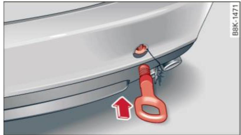
Fig. 216 Rear bumper: Screwing in towing loop
