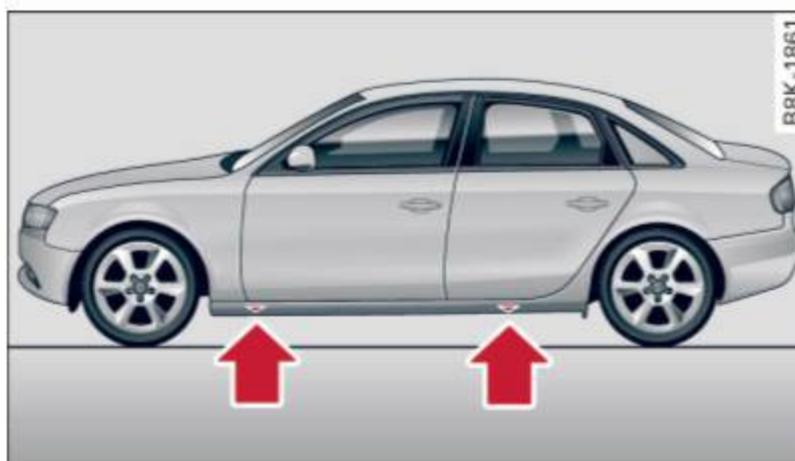
Fig. 203 Sill panels: markings
