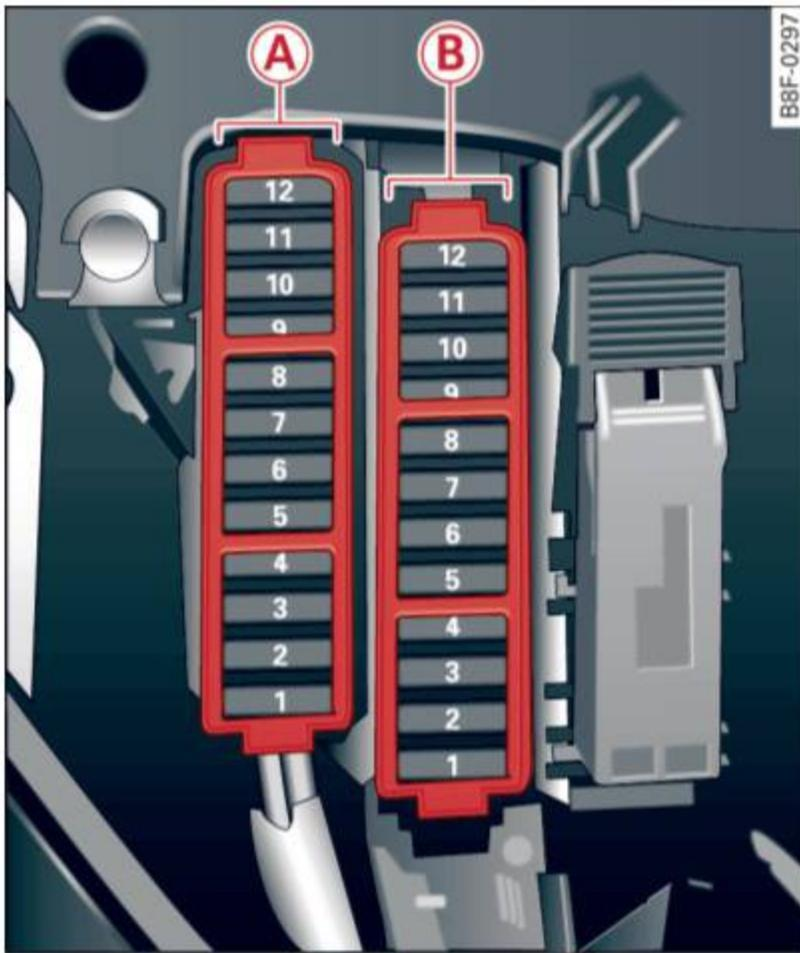
Fig. 209 Right cockpit: fuse panel with plastic clip
