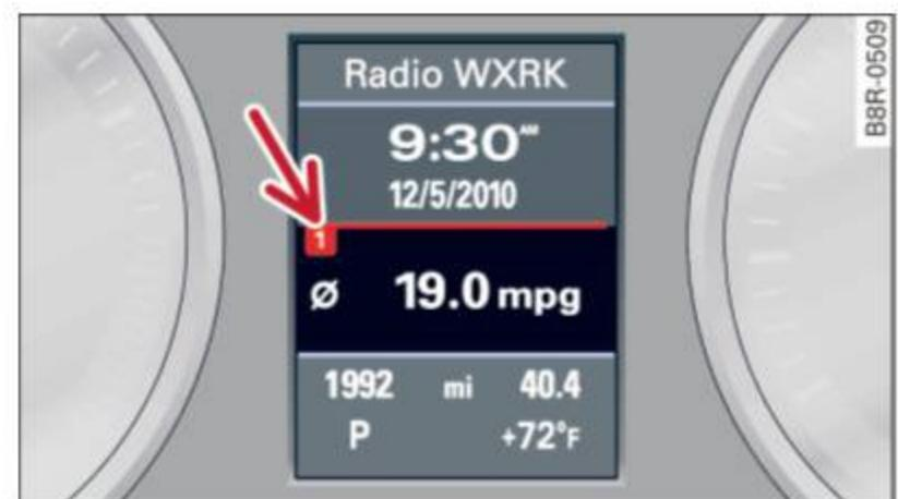
Fig. 10 Trip computer display: memory level 1
