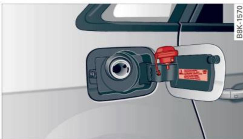
**Fig. 177** Fuel filler flap with attached fuel cap
