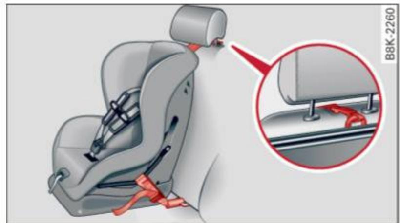
**Fig. 173** allroad Tether strap: proper routing and mounting
