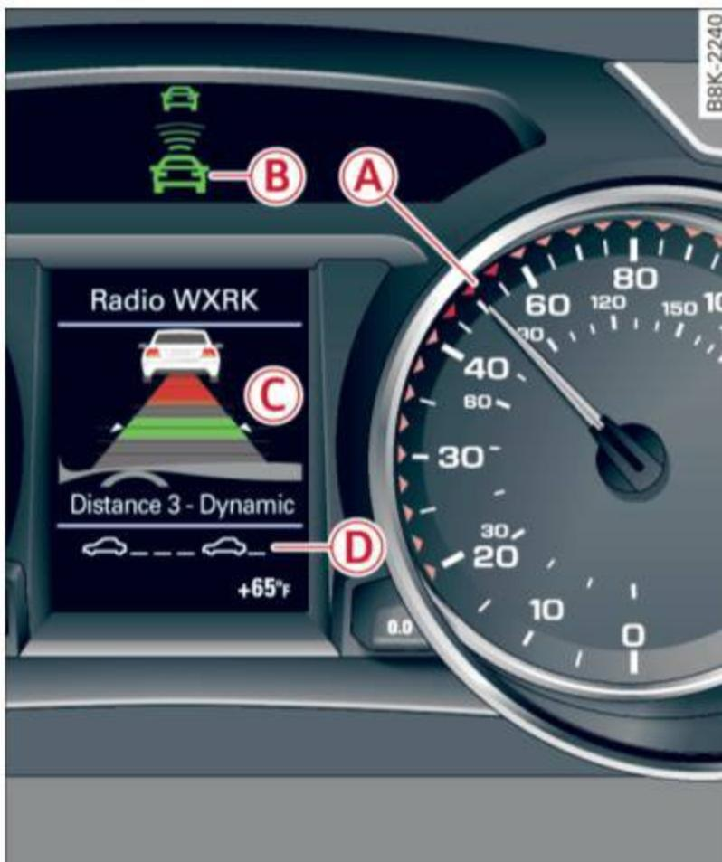
Fig. 118 Instrument cluster: Audi adaptive cruise control
