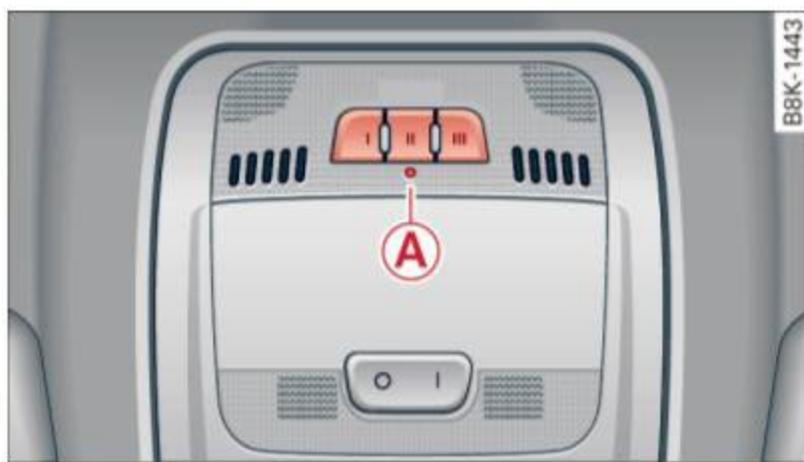
Fig. 41 Headliner: control unit
