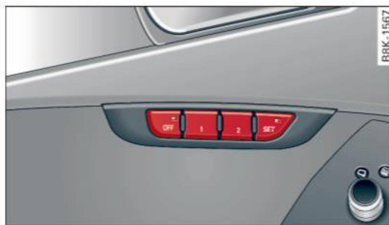
**Fig. 67** Driver's door: memory function buttons
