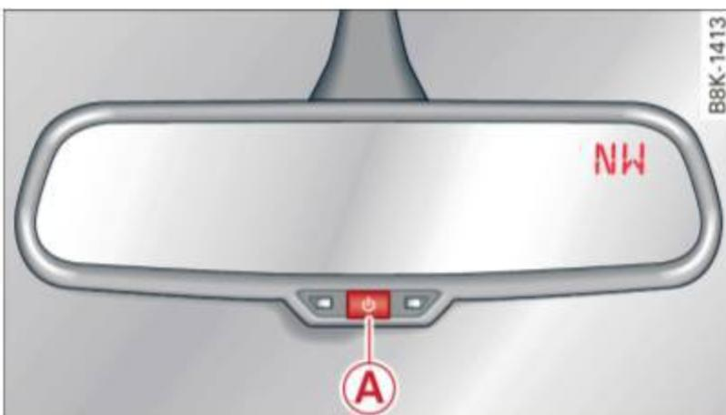
Fig. 59 Rearview mirror: Digital compass activated
