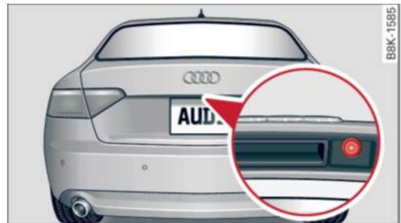
Fig. 134 Trunk lid: Location of the rear view camera
