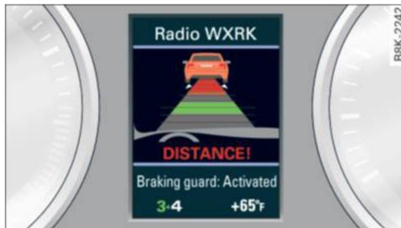
Fig. 123 Instrument cluster: approach warning
