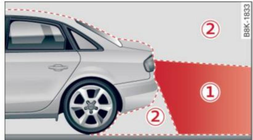
Fig. 133 Covered area ① and uncovered area ② of the rear view camera
