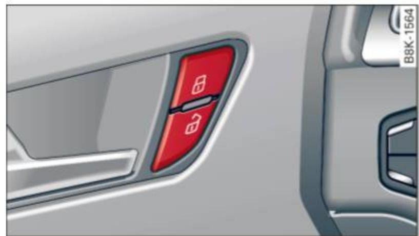
Fig. 24 Driver's door: power locking switch
