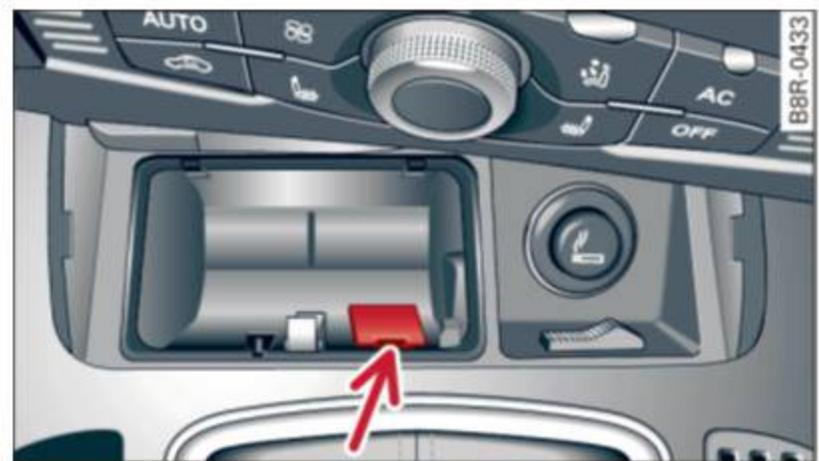
Fig. 112 Selector lever emergency release
