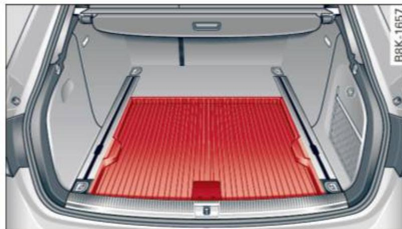
Fig. 93 Luggage compartment: cargo area floor reversed
