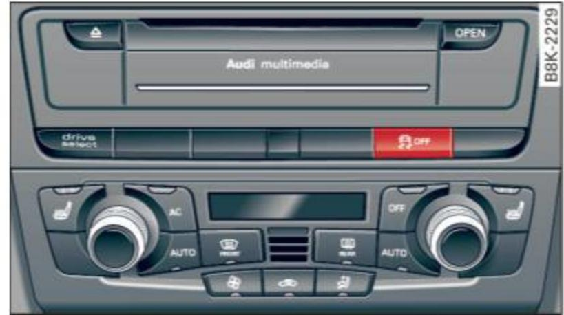
Fig. 175 Version B: upper center console, ESC OFF button
