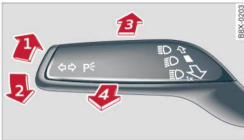
Fig. 44 Turn signal and high beam lever
