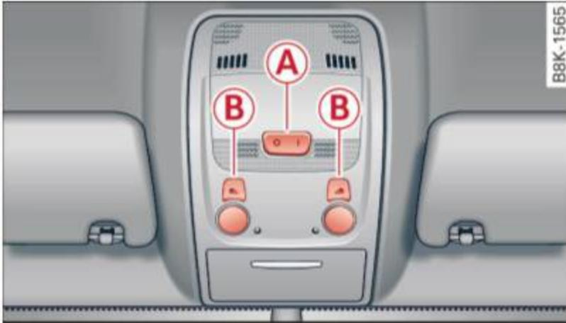
Fig. 46 Front headliner: interior lighting controls
