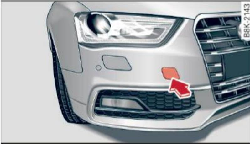
Fig. 213 Front bumper: removing the cover cap
