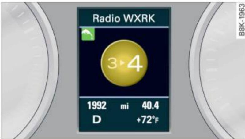
Fig. 14 Display: enhanced shift indicator
