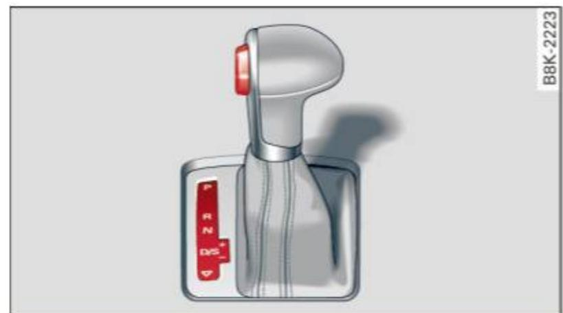
**Fig. 108** Shift gate on the center console: selector lever with release button
