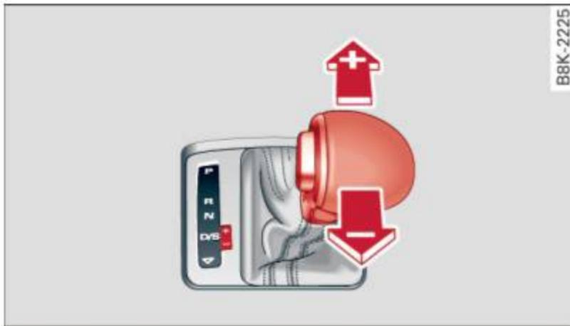
Fig. 109 Center console: shifting the gears manually
