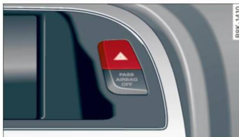
Fig. 45 Center console: emergency flasher switch
