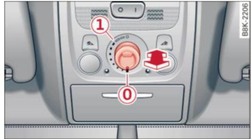
**Fig. 37** Section of headliner: knob for sunroof
