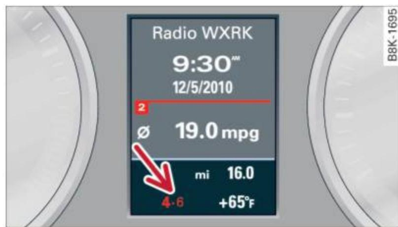
Fig. 12 Display: Gearshift indicator
