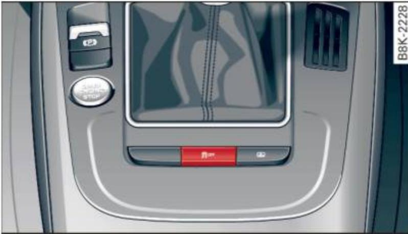
Fig. 174 Version A: lower center console, ESC OFF button
