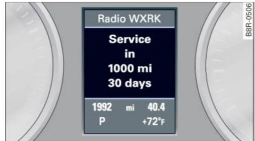
Fig. 17 Display: Service interval display
