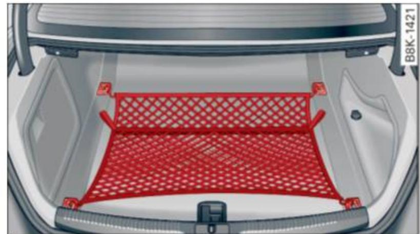
Fig. 84 Luggage compartment: cargo net stretched out
