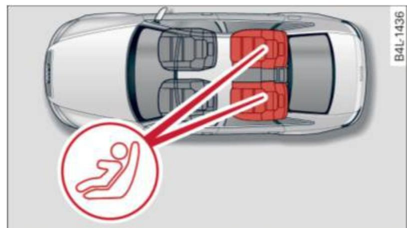
**Fig. 166** Schematic overview: LATCH anchorage point locations
