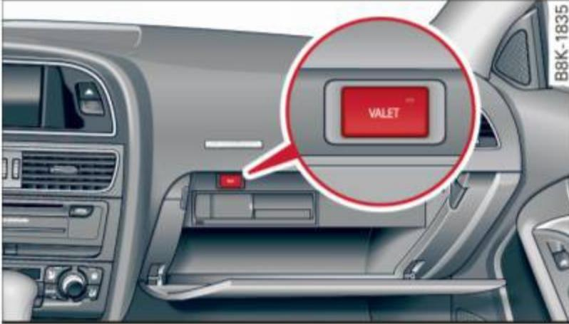
Fig. 39 Glove compartment: valet parking button
