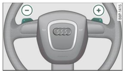
Fig. 125 Sport steering wheel with selector paddles
