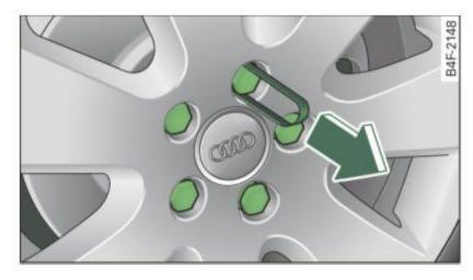
Fig. 192 Wheel change: removing the wheel bolt caps
