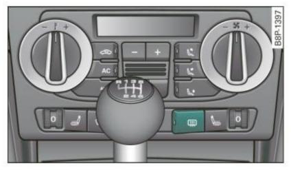
Fig. 110 Switch for rear window defogger with air-conditioning
