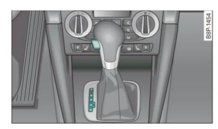
Fig. 122 Section from center console: Selector lever with release button
