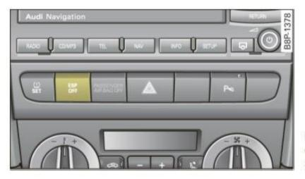
Fig. 163 Center console with ESP switch
