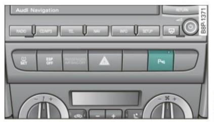
Fig. 115 Center console: Switch for parking aid
