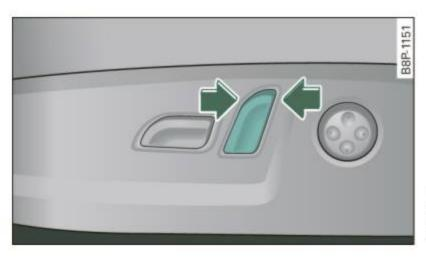
Fig. 76 Driver's seat: switch for seatback adjustment
