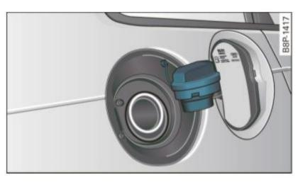
Fig. 165 Fuel cap hooked on the opened fuel filler flap
