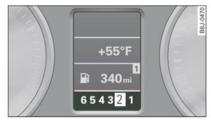
Fig. 124 Display: Manual shifting (tiptronic)
