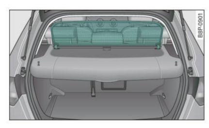
Fig. 63 Sun blind in extended position
