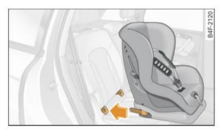
Fig. 157 LATCH-type seat with both latch bars extended
