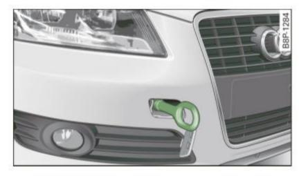
Fig. 207 Front bumper: screwing in the towing loop
