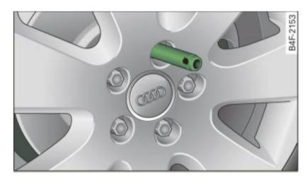
Fig. 198 Wheel change: alignment pin inside the top hole
