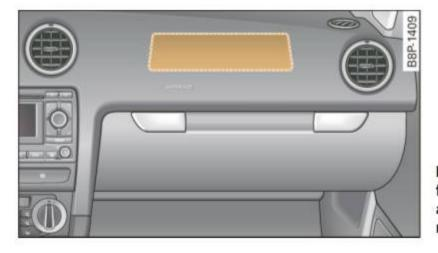
Fig. 144 Location of front passenger's airbag: in the instrument panel
