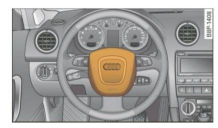
Fig. 143 Location of driver airbag: in steering wheel
