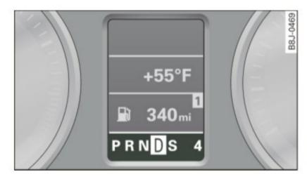
Fig. 120 Display: Selector lever positions
