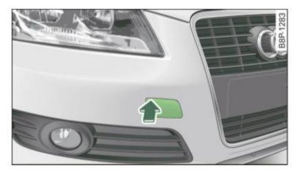
Fig. 206 Front bumper: removing the cover cap
