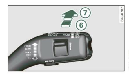
Fig. 65 Wiper lever: activating the rear window wiper and washer
