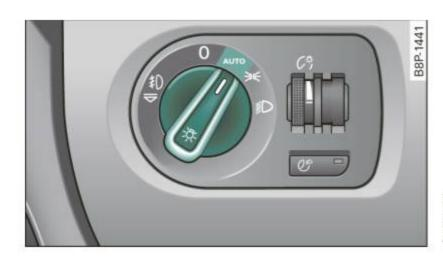
Fig. 48 Instrument panel: light switch in AUTO position
