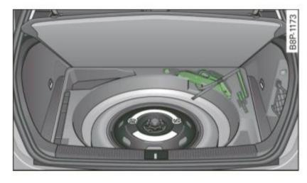
Fig. 189 Vehicle tool kit and jack
