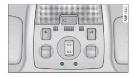
Fig. 58 Control panel above windshield: position of ambient light bulbs
