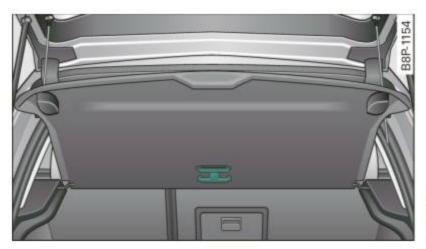
Fig. 88 Mounting hooks under the rear parcel shelf
