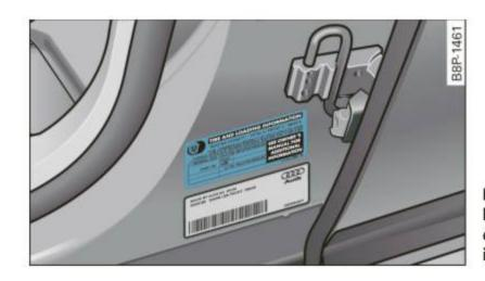
Fig. 180 Tire pressure label: located either on driver's side B-pillar or inside the fuel filler flap
