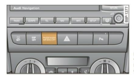
Fig. 146 Section from the center console: PASSENGER AIR BAG OFF light
