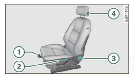
Fig. 73 Adjustment controls: locations on driver's seat
