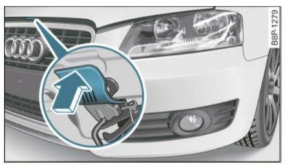
Fig. 168 Engine hood release lever
