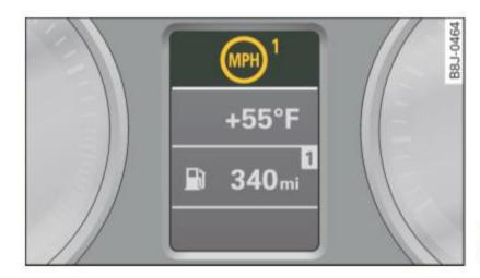
Fig. 18 Display: speed warning system
