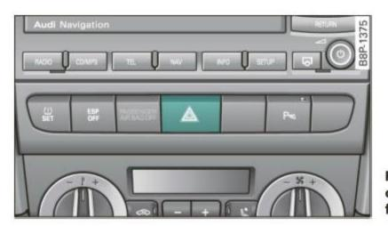
Fig. 54 Center console: emergency flasher switch
