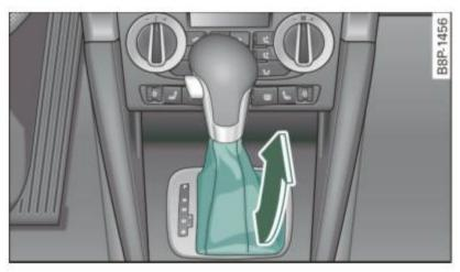
Fig. 126 Selector lever: Remove selector lever sleeve
