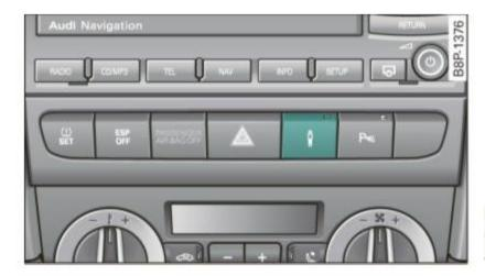
Fig. 118 Center console: Switch for Audi magnetic ride
