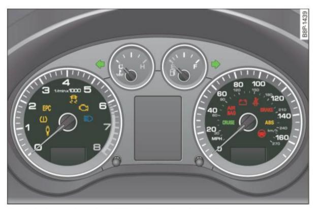
Fig. 5 Instrument cluster with warning/indicator lights
