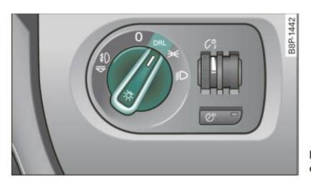
Fig. 49 Switch for daytime running lights
