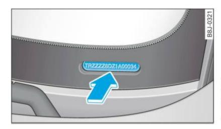
Fig. 213 Vehicle Identification Number (VIN) plate: location on driver's side dash panel
