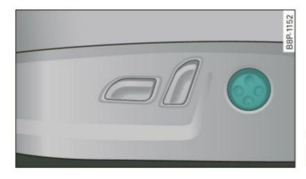
Fig. 77 Driver seat: switch for lumbar adjustment
