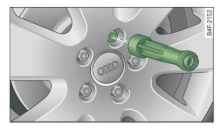
Fig. 197 Wheel change: using the screwdriver handle (with the blade removed) to turn the bolts
