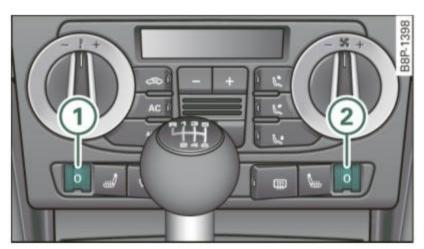
Fig. 111 Center console: thumbwheels for front seat heating
