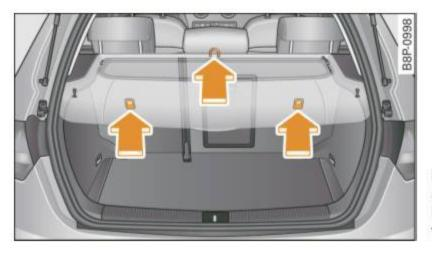
Fig. 159 Tether anchors: attachment hook locations behind the rear seatbacks
