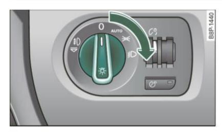
Fig. 46 Instrument panel: light switch
