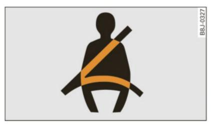
Fig. 132 Safety belt warning light in the instrument cluster enlarged
