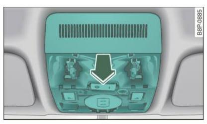
Fig. 43 Removing the light unit
