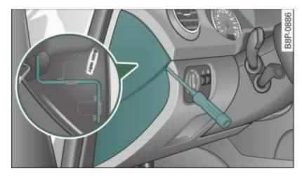
Fig. 44 Left end face of the instrument panel: fuse cover with hand crank
