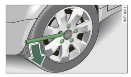
Fig. 187 Wheel change: loosening the wheel bolts
