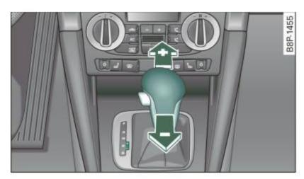
Fig. 117 Center console: Manual shifting (tiptronic)
