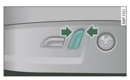
Fig. 73 Driver's seat: switch for seatback adjustment
