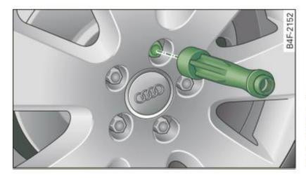
Fig. 190 Wheel change: using the screwdriver handle (with the blade removed) to turn the bolts
