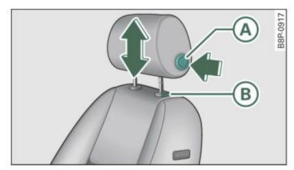
Fig. 75 Driver's seat head restraint: adjusting the height
