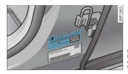
Fig. 173 Tire pressure label: located either on driver's side B-pillar or inside the fuel filler flap
