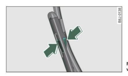
Fig. 63 Unlatching wiper blades
