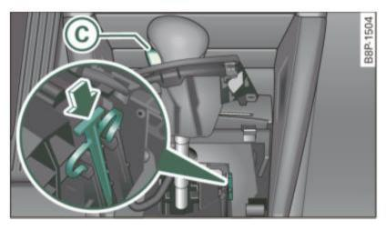
Fig. 123 Selector lever: emergency release from the Park position
