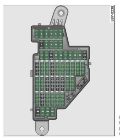
Fig. 194 Fuse carrier behind the instrument panel end face, cover removed
