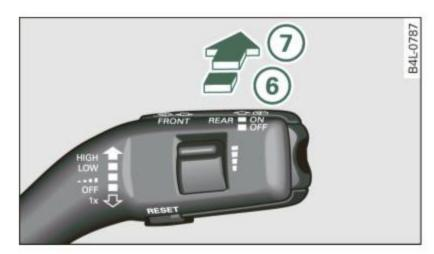
Fig. 62 Wiper lever: activating the rear window wiper and washer
