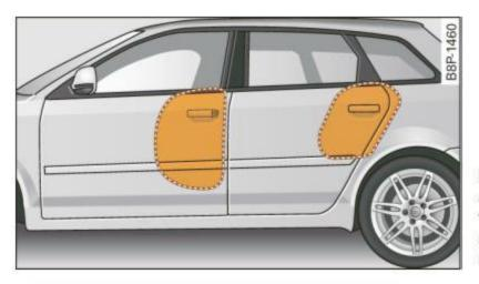
Fig. 144 Inflated side airbags on left side of vehicle, rear side airbag optional equipment
