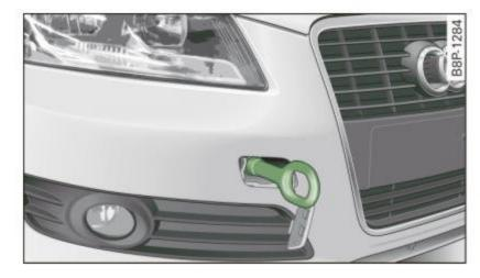
Fig. 198 Front bumper: screwing in the towing loop
