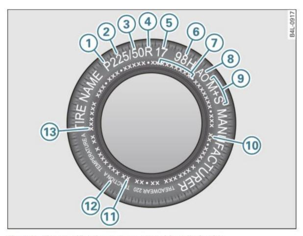
Fig. 177 Tire specification codes on the sidewall of a tire
