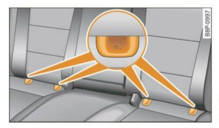
Fig. 153 Rear seats: lower anchorage bracket locations
