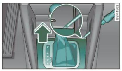
Fig. 122 Selector lever: Remove selector lever sleeve
