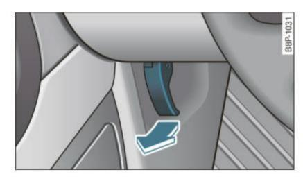
Fig. 162 Driver's side footwell: engine hood release lever
