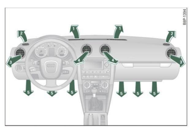
Fig. 104 Instrument panel: air outlet locations and airflow directions
