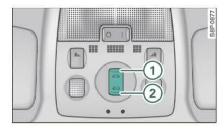
Fig. 39 Section of the roof liner Toggle switch for the panoramic sliding sunroof
