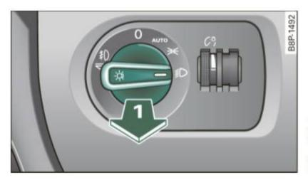
Fig. 49 Fog light activation: light switch position on vehicles WITHOUT sensor light
