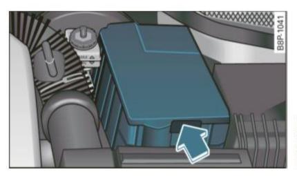
Fig. 171 Engine compartment (4-cylinder engine): Battery with cover\*
