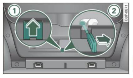
Fig. 33 Rear lid interior section: Emergency release
