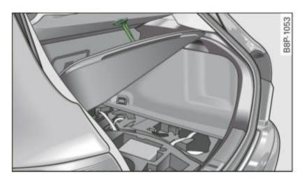
Fig. 181 Floor panel hung on the bottom of the luggage compartment cover
