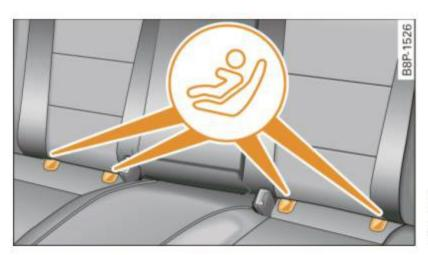
Fig. 152 Rear seatbacks: locator buttons for lower anchorages
