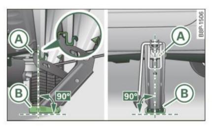
Fig. 189 Close-up: proper positioning of lifting jack
