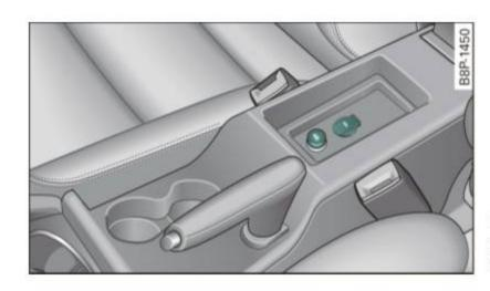
Fig. 94 Center console, front: 12-volt outlet
