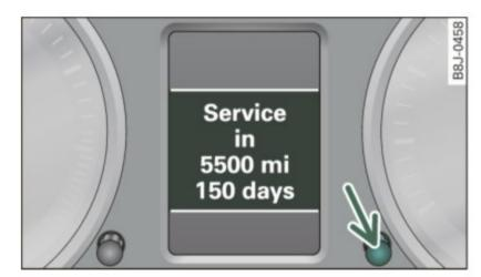
Fig. 9 Section of instrument cluster: Service interval display
