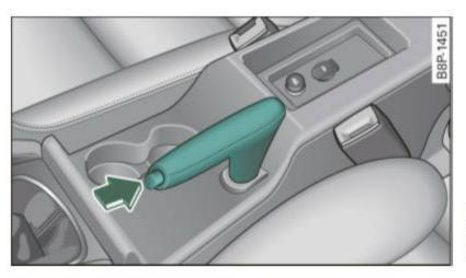
Fig. 110 Center console: Parking brake
