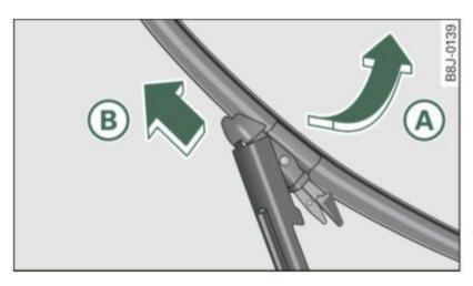
Fig. 64 Removing wiper blades
