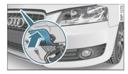
Fig. 163 Engine hood release lever
