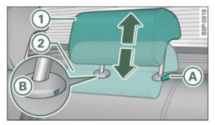
Fig. 77 Center rear head restraint: adjusting the height
