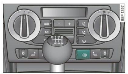
Fig. 105 Switch for rear window defogger with air-conditioning
