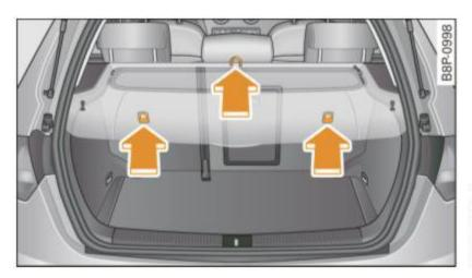
Fig. 155 Tether anchors: attachment hook locations behind the rear seatbacks
