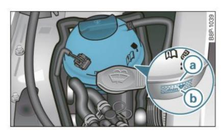
Fig. 169 Engine compartment: coolant expansion tank
