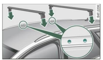
Fig. 90 Roof rails: front and rear mounting locations
