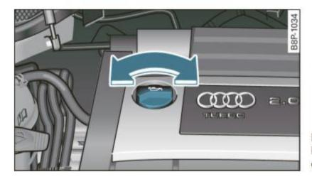
Fig. 168 Oil filler cap location: 2.0 liter, 4cylinder turbo engine
