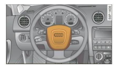
Fig. 139 Location of driver airbag: in steering wheel
