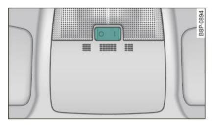
Fig. 53 Control panel above windshield: interior light switches
