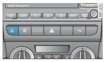
Fig. 179 Car: Tire pressure monitoring system
