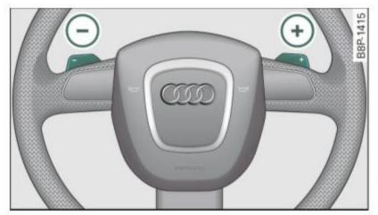
Fig. 119 Sport steering wheel with selector paddles
