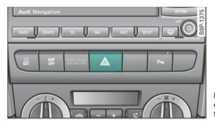
Fig. 51 Center console: emergency flasher switch
