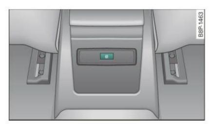
Fig. 29 Rear power locking switch
