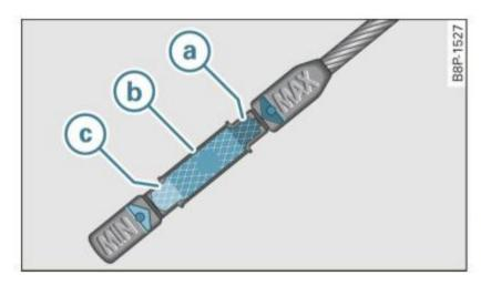
Fig. 166 Dipstick (Version A): Oil level ranges
