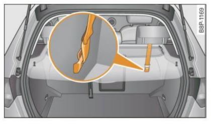
Fig. 157 Tether strap: proper routing and mounting
