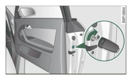
Fig. 34 Emergency locking device in the doors
