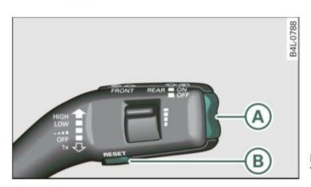
Fig. 20 Wiper lever: Trip computer controls
