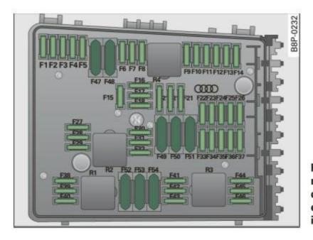
Fig. 195 Fuse assignment in the engine compartment in the example with 54 plugin fuses
