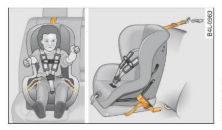
Fig. 148 Schematic overview: installation of the attachments applicable to a LATCH seat
