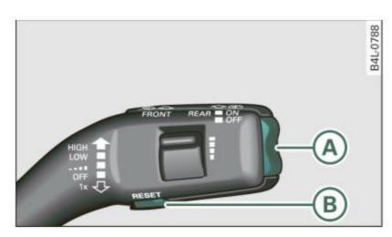
Fig. 12 Wiper arm/wiper lever: controls for the trip computer
