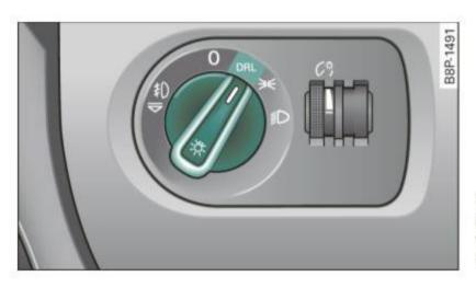
Fig. 47 Instrument panel: Light switch with daytime running lights (DRL)
