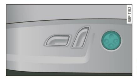
Fig. 74 Driver seat: switch for lumbar adjustment
