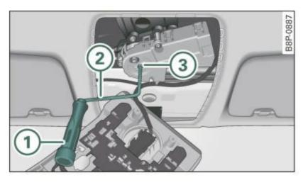
Fig. 45 Light unit in the headliner: crank for emergency operation
