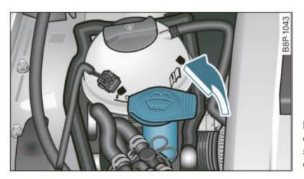
Fig. 172 Engine compartment: windshield washer fluid container
