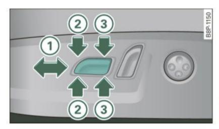
Fig. 72 Seat cushion adjustment: switch motions
