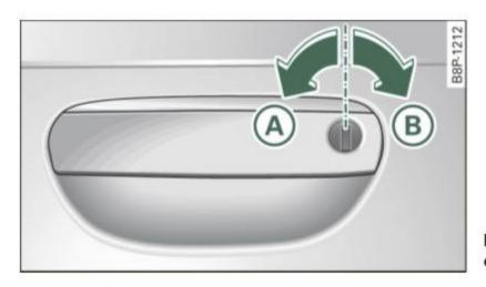
Fig. 27 Key turns for opening and closing.
