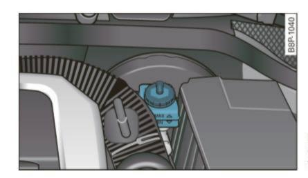
Fig. 170 Engine compartment: brake fluid reservoir
