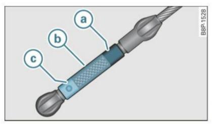
Fig. 167 Dipstick (Version B): Oil level ranges
