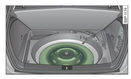
Fig. 183 Compact spare wheel in the wheel well
