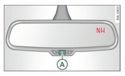
Fig. 68 Inside rear view mirror: digital compass activated
