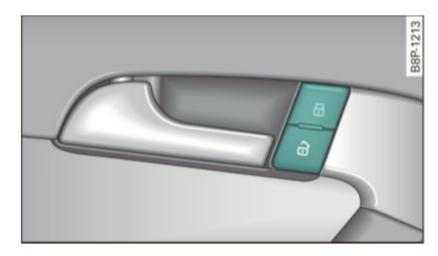
Fig. 28 Driver's door: power locking switch
