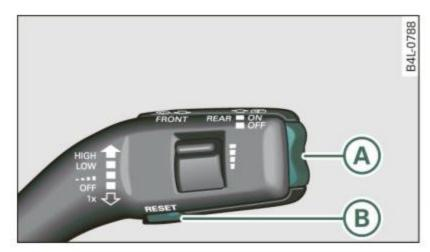
Fig. 15 Wiper lever: Controls for the menu display
