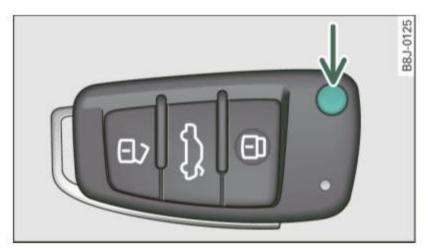
Fig. 23 Fold-up master key with remote control
