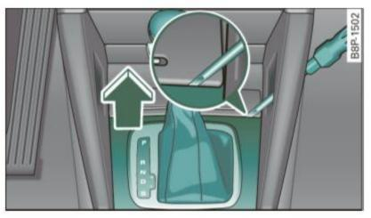
Fig. 120 Selector lever: Remove selector lever sleeve
