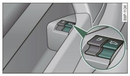
Fig. 30 Driver's door, rear bottom: remote rear lid release
