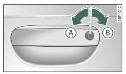
Fig. 38 Key turns for opening and closing
