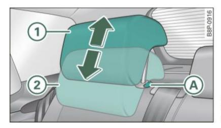
Fig. 76 Outer rear head restraints: adjusting the height
