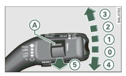
Fig. 61 Wiper lever: windshield wiper lever positions
