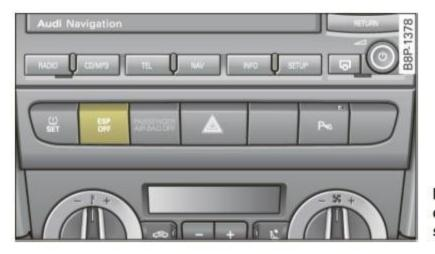
Fig. 158 Center console with ESP switch
