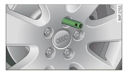
Fig. 191 Wheel change: alignment pin inside the top hole
