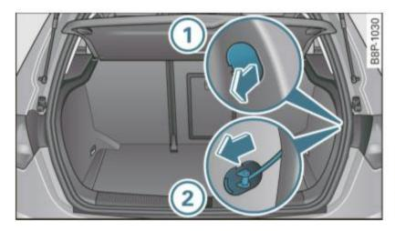
Fig. 161 Inside the luggage compartment: Opening the fuel filler flap by hand
