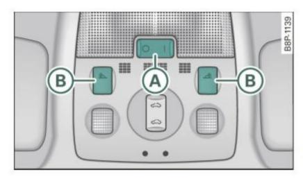
Fig. 54 Control panel above windshield: interior light switches
