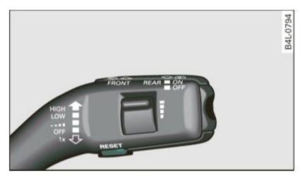
Fig. 7 Wiper lever: controls for the menu display
