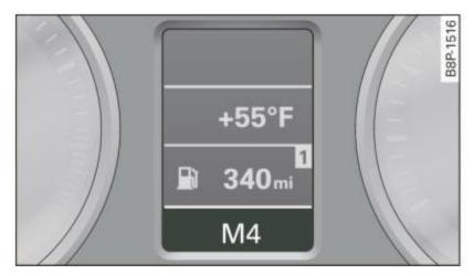
Fig. 118 Display: Manual shifting (tiptronic)
