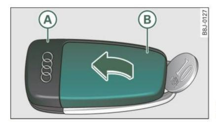
Fig. 25 Master key: opening the cover
