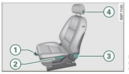
Fig. 70 Adjustment controls: locations on driver's seat
