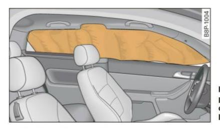
Fig. 146 Illustration of principle: Inflated side curtain airbags on the left side
