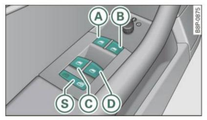
Fig. 37 Driver's door: power window switches
