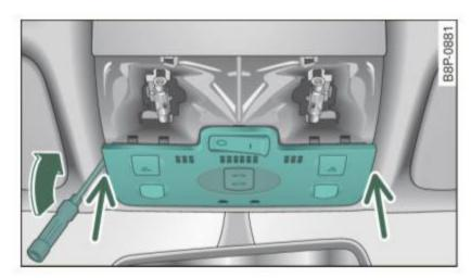
Fig. 41 Light unit in the headliner: removing the switch cover
