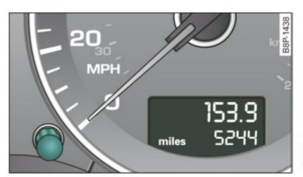
Fig. 4 Speedometer close-up: odometer display
