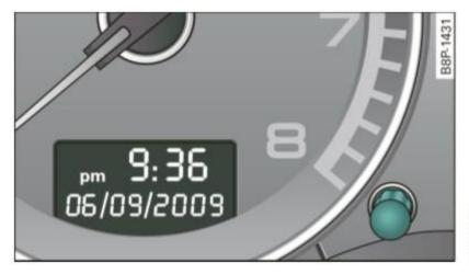
Fig. 21 Section of instrument cluster: Set/Check button
