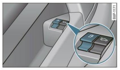
Fig. 159 Driver's door: Unlocking fuel filler flap
