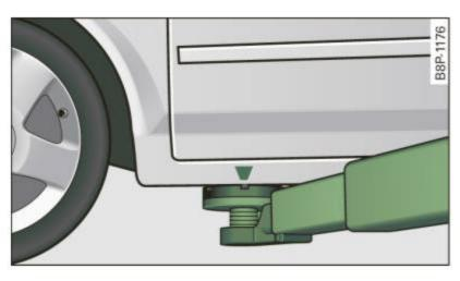
Fig. 202 Front lifting point
