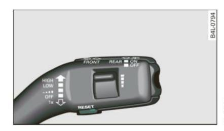
Fig. 13 Wiper lever: Controls for the menu display
