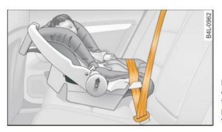
Fig. 147 Schematic overview: rearwardfacing infant seat, properly installed on the rear seat
