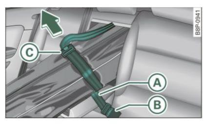
Fig. 88 Securing the ski sack at the center rear seat belt buckle
