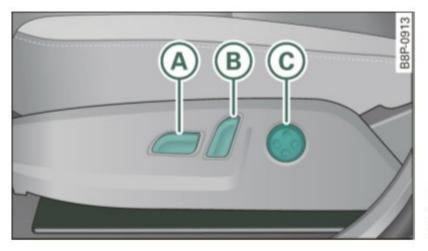
Fig. 71 Adjustment switches: locations on driver's seat
