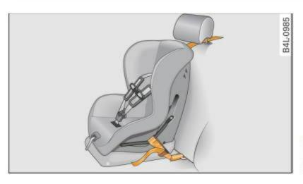
Fig. 156 Tether strap: proper routing and mounting
