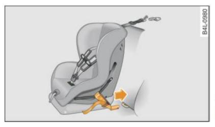
Fig. 154 Lower anchorages: proper mounting
