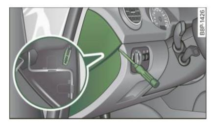
Fig. 192 End face of instrument panel: removing cover plate to access fuses
