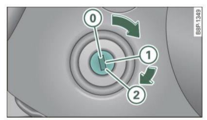
Fig. 108 Ignition lock positions
