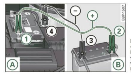
Fig. 196 Jumpstarting with the battery of another vehicle: A – discharged vehicle battery, B – booster battery
