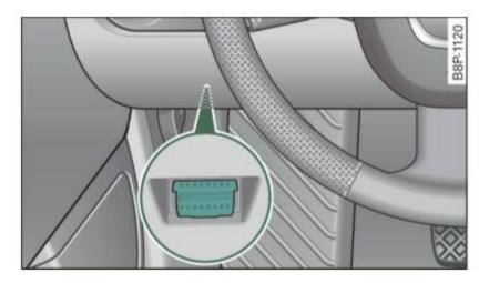
Fig. 10 Location of Data Link Connector (DLC)
