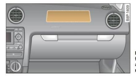
Fig. 140 Location of front passenger's airbag: in the instrument panel
