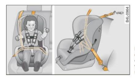
Fig. 149 Schematic overview: installation of the seat using the vehicle's safety belt system
