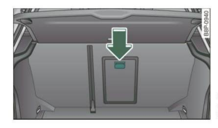
Fig. 87 Section of the rear seat from the rear: ski sack hatch cover
