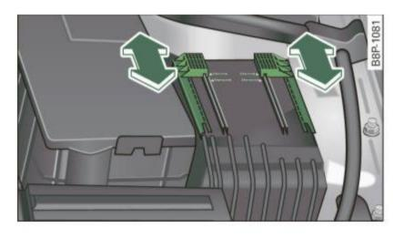
Fig. 193 Left side of engine compartment: fuse cover
