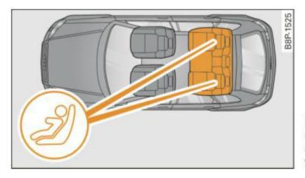
Fig. 151 Schematic overview: LATCH anchorage point locations
