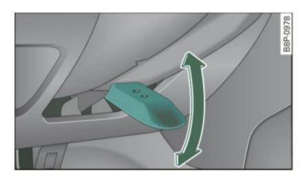
Fig. 107 Lever under the steering column
