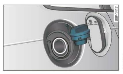
Fig. 160 Fuel cap hooked on the opened fuel filler flap
