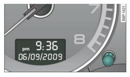
Fig. 19 Section of instrument cluster: Set/Check button
