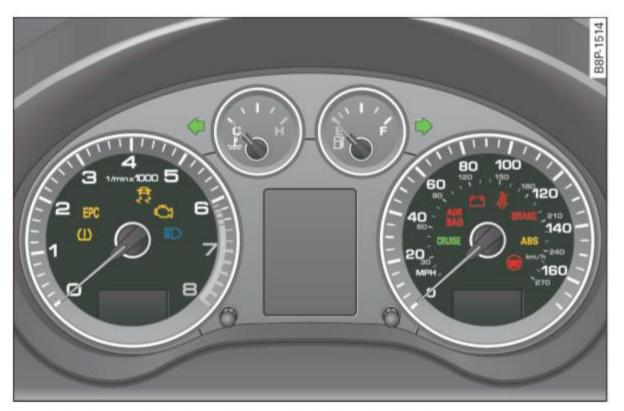
Fig. 5 Instrument cluster with warning/indicator lights
