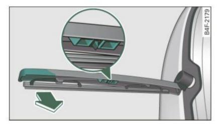
Fig. 65 Installing/rem oving wiper blade
