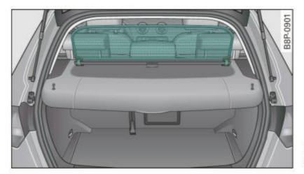
Fig. 60 Sun blind in extended position
