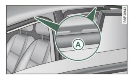
Fig. 89 Attachment points for roof rack
