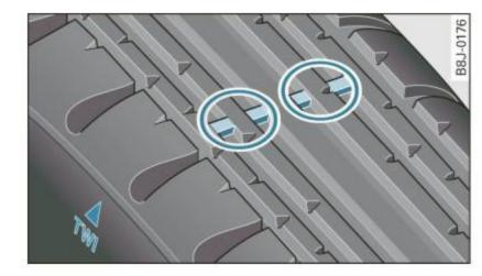
Fig. 175 Tire tread: tread wear indicators (TWI)
