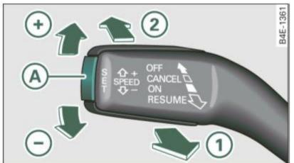
Fig. 111 Control lever with set button
