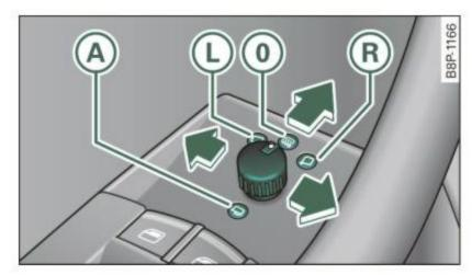
Fig. 67 Forward section of driver's armrest: power mirror controls
