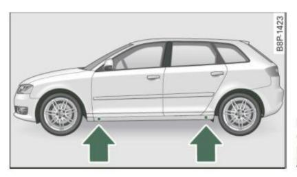
Fig. 188 Wheel change: mounting points for the lifting iack
