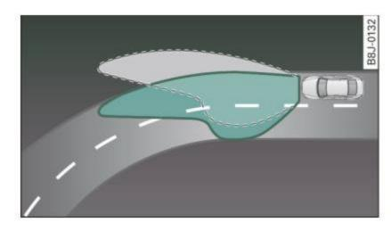
Fig. 48 Adaptive light when driving
