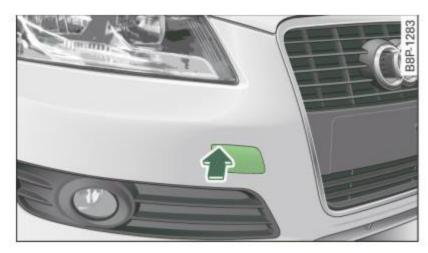
Fig. 197 Front bumper: removing the cover cap
