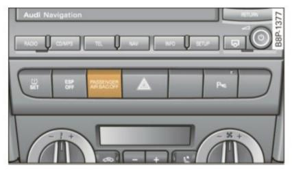
Fig. 142 Section from the center console: PASSENGER AIR BAG OFF light
