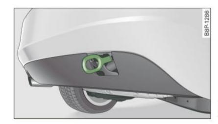
Fig. 200 Rear bumper: towing loop inserted
