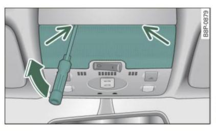
Fig. 40 Light unit in the headliner: removing the glass
