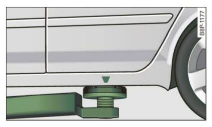
Fig. 203 Rear lifting point
