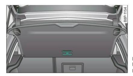
Fig. 85 Mounting hooks under the rear parcel shelf
