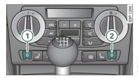
Fig. 106 Center console: thumbwheels for front seat heating
