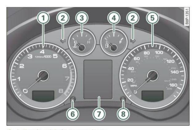
Fig. 2 Overview of the instrument cluster
