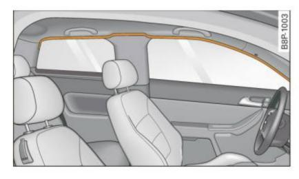
Fig. 145 Curtain airbag, driver's side: side curtain airbag location
