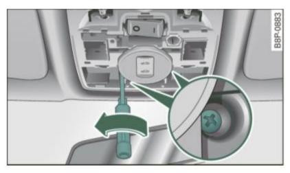
Fig. 42 Light unit in the headliner: removing screws in the light unit
