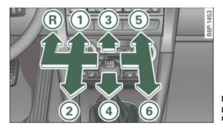
Fig. 113 Gearshift pattern: 6-speed manual transmission
