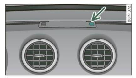
Fig. 36 Diode position in the instrument panel
