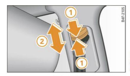
Fig. 138 Safety belt height adjustment for the front seats – looparound fittings
