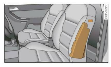
Fig. 143 Side airbag location in the driver's seat
