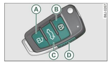
Fig. 26 Remote control: function buttons
