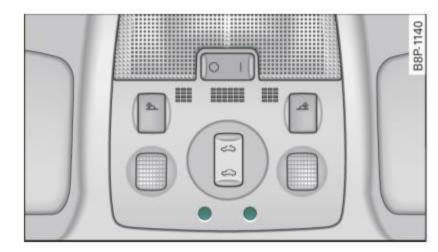
Fig. 55 Control panel above windshield: position of ambient light bulbs
