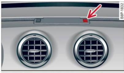
Fig. 39 Diode position in the instrument panel
