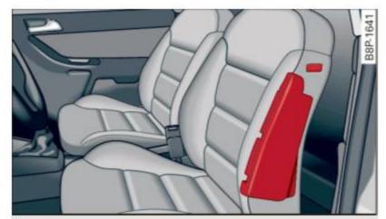
Fig. 135 Side airbag location in the driver's seat
