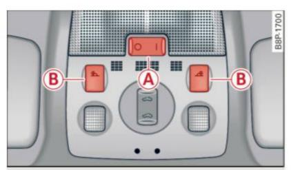
Fig. 50 Control panel above windshield: interior light switches
