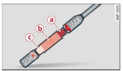
Fig. 159 Dipstick (Version A): Oil level ranges
