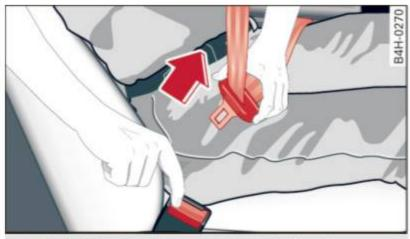
Fig. 129 Releasing the tongue from the buckle
