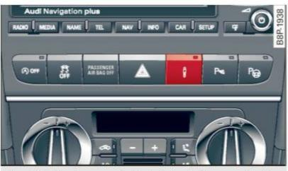
Fig. 107 Center console: Switch for Audi magnetic ride
