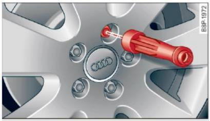
**Fig. 187** Wheel change: using the screwdriver handle (with the blade removed) to turn the bolts
