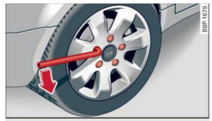
Fig. 184 Wheel change: loosening the wheel bolts
