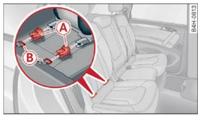
Fig. 146 Rear bench seat: installing the mount for LATCH child seats
