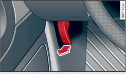
Fig. 155 Driver's side footwell: engine hood release lever
