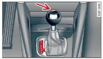
Fig. 111 Section from center console: Selector lever with release button
