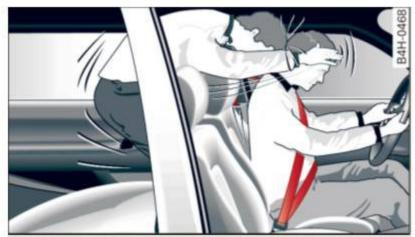
Fig. 124 A rear passenger not wearing a safety belt will fly forward and strike the driver
