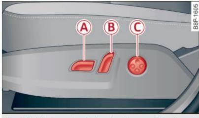
Fig. 65 Adjustment switches: locations on driver's seat
