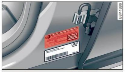
Fig. 167 Tire pressure label: located either on driver's side B-pillar or inside the fuel filler flap
