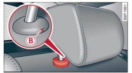
Fig. 71 Rear head restraints: release
