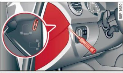
Fig. 189 Left cockpit: fuse panel cover
