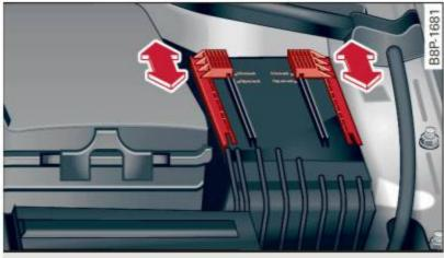
Fig. 190 Left side of engine compartment: fuse cover
