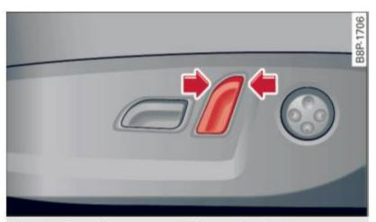
Fig. 67 Driver's seat: switch for seatback adjustment
