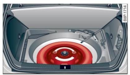
Fig. 180 Compact spare wheel in the wheel well
