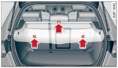
Fig. 148 Tether anchors: attachment hook locations behind the rear seatbacks
