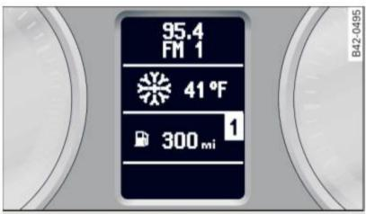
Fig. 6 Instrument cluster: center display
