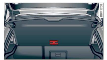
Fig. 79 Mounting hooks under the rear parcel shelf
