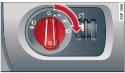
Fig. 43 Instrument panel: light switch
