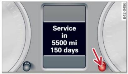
Fig. 20 Section of instrument cluster: Service interval display
