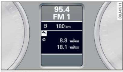
Fig. 17 Display: efficiency program
