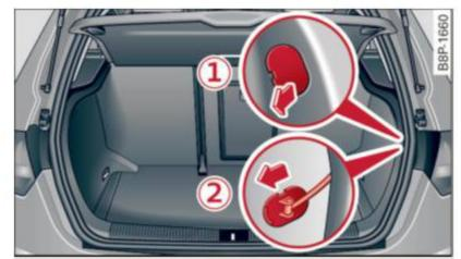
**Fig. 154** Inside the luggage compartment: Opening the fuel filler flap by hand
