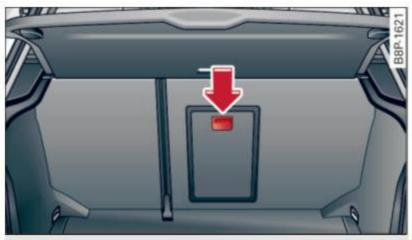
Fig. 81 Section of the rear seat from the rear: ski sack hatch cover
