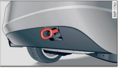
Fig. 197 Rear bumper: towing loop inserted
