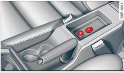
Fig. 87 Center console, front: 12-volt outlet
