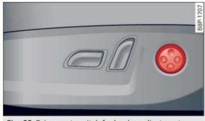
Fig. 68 Driver seat: switch for lumbar adjustment
