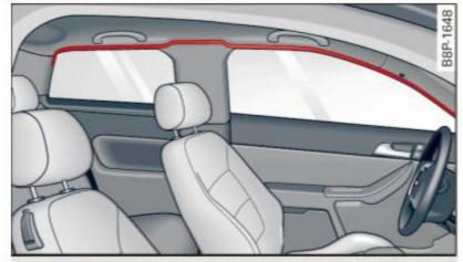
Fig. 137 Curtain airbag, driver's side: side curtain airbag location
