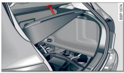
Fig. 178 Floor panel hung on the bottom of the luggage compartment cover
