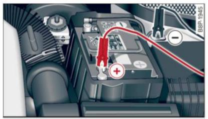
Fig. 165 Engine compartment: connectors for a charger and jump start cables
