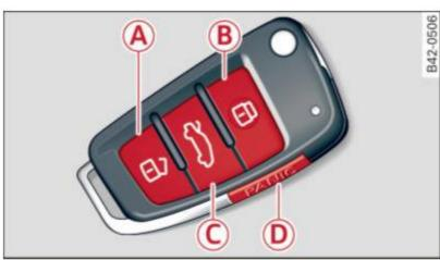
Fig. 29 Remote control: function buttons
