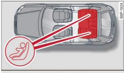
Fig. 143 Schematic overview: LATCH anchorage point locations
