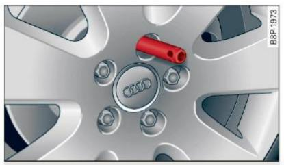
Fig. 188 Wheel change: alignment pin inside the top hole
