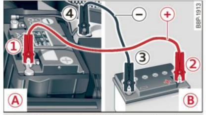
**Fig. 193** Jump-starting with the battery of another vehicle: A – discharged vehicle battery, B – booster battery
