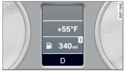
Fig. 109 Display: Selector lever positions
