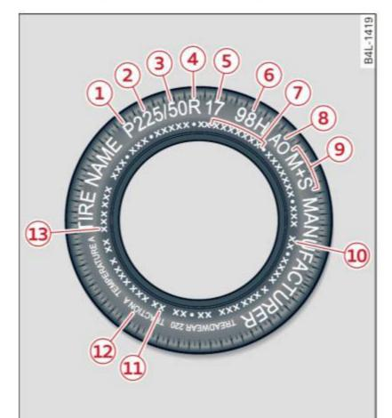
**Fig. 171** Tire specification codes on the sidewall of a tire
