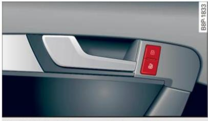
Fig. 31 Driver's door: power locking switch
