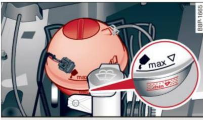
Fig. 162 Engine compartment: coolant expansion tank
