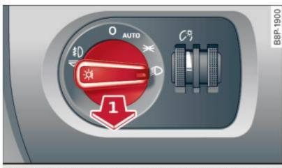
Fig. 45 Fog light activation: light switch position on vehicles WITHOUT sensor light
