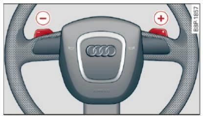
Fig. 114 Sport steering wheel with selector paddles
