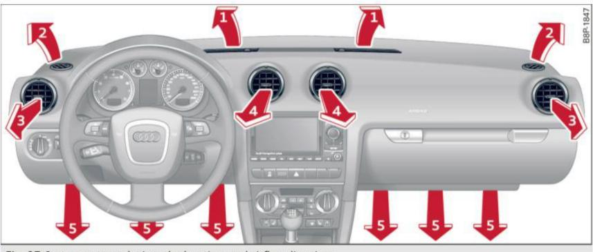
Fig. 97 Instrument panel: air outlet locations and airflow directions
