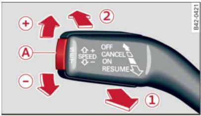
Fig. 105 Control lever with set button
