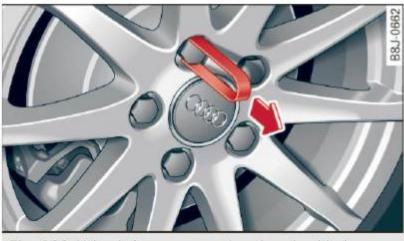
Fig. 182 Wheel change: removing the wheel bolt caps
