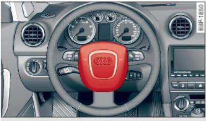
Fig. 131 Location of driver airbag: in steering wheel
