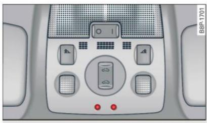
Fig. 51 Control panel above windshield: position of ambient light bulbs
