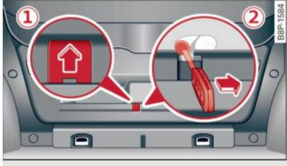
Fig. 36 Rear lid interior section: Emergency release
