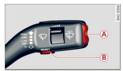
Fig. 174 Wiper lever: Controls for the menu display
