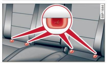
Fig. 145 Rear seats: lower anchorage bracket locations
