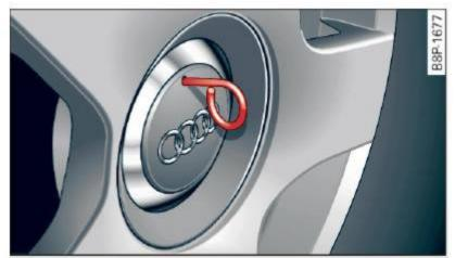
Fig. 181 Wheel change: removing the wheel cover
