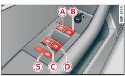
Fig. 40 Driver's door: power window switches
