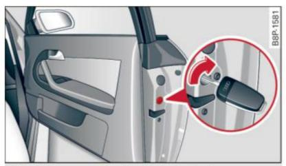
Fig. 37 Emergency locking device in the doors
