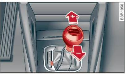
Fig. 112 Center console: Manual shifting (tiptronic)
