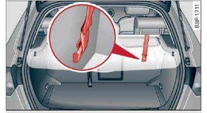
Fig. 150 Tether strap: proper routing and mounting
