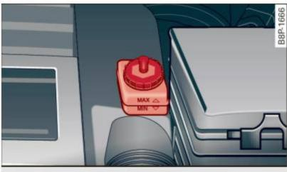
Fig. 163 Engine compartment: brake fluid reservoir
