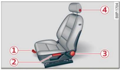
Fig. 64 Adjustment controls: locations on driver's seat
