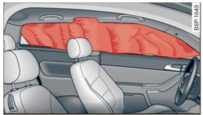
Fig. 138 Illustration of principle: Inflated side curtain airbags on the left side
