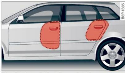
Fig. 136 Inflated side airbags on left side of vehicle, rear side airbag optional equipment
