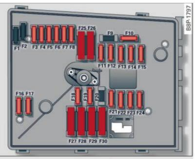
Fig. 192 Engine compartment: fuse assignment
