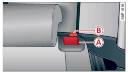
Fig. 74 Release lever for the seatback (left side)
