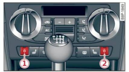
**Fig. 99** Center console: thumbwheels for front seat heating
