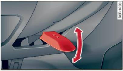
Fig. 101 Lever under the steering column
