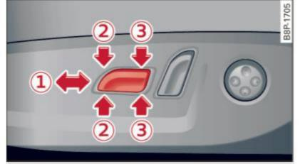
Fig. 66 Seat cushion adjustment: switch motions
