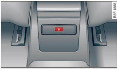
Fig. 32 Rear power locking switch
