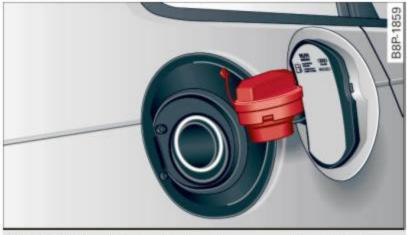
Fig. 153 Fuel cap hooked on the opened fuel filler flap
