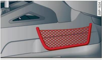
Fig. 92 Storage net in passenger's footwell
