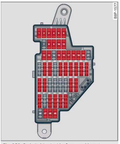
Fig. 191 Cockpit driver's side: fuse panel layout
