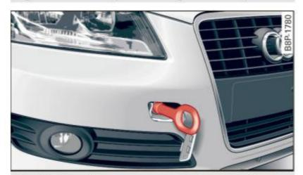
Fig. 195 Front bumper: screwing in the towing loop
