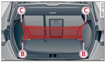
Fig. 78 Luggage compartment: cargo net attached to hooks
