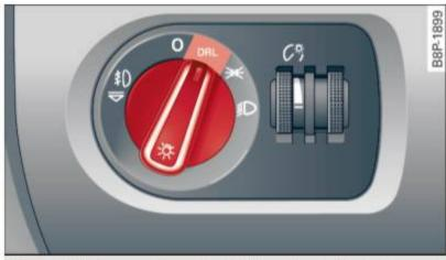
**Fig. 44** Instrument panel: Light switch with daytime running lights (DRL)
