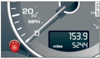
Fig. 5 Speedometer close-up: odometer display
