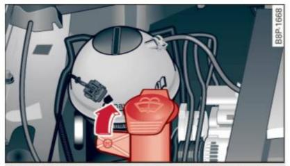
Fig. 166 Engine compartment: windshield washer fluid container
