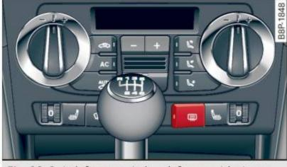
Fig. 98 Switch for rear window defogger with air-conditioning
