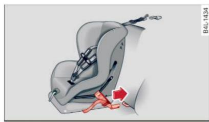
Fig. 147 Lower anchorages: proper mounting
