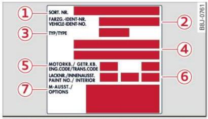
Fig. 202 The vehicle identification label – inside the luggage compartment
