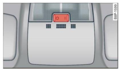
Fig. 49 Control panel above windshield: interior light switches
