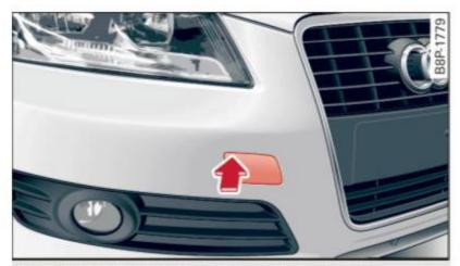
Fig. 194 Front bumper: removing the cover cap
