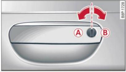
Fig. 41 Key turns for opening and closing
