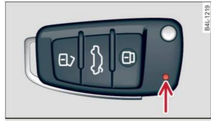
Fig. 27 Check light in the master key
