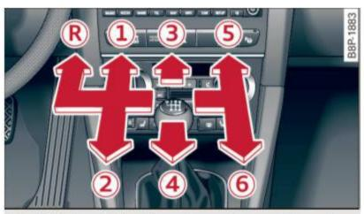
Fig. 108 Gearshift pattern: 6-speed manual transmission
