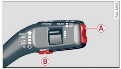
Fig. 24 Wiper lever: Trip computer controls
