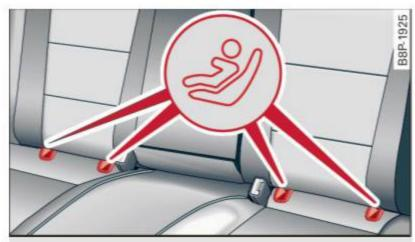
Fig. 144 Rear seatbacks: locator buttons for lower anchorages
