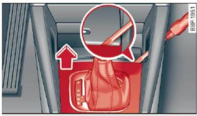
Fig. 115 Selector lever: Remove selector lever sleeve
