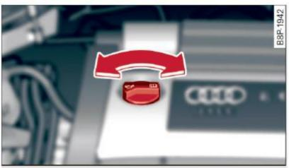
Fig. 161 Engine compartment: Oil filler cap location
