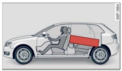
Fig. 119 Safe load positioning: heavy cargo positioned as far forward as possible.
