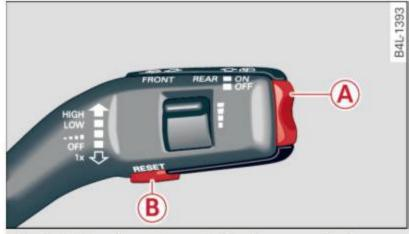
Fig. 14 Wiper lever: Controls for the menu display
