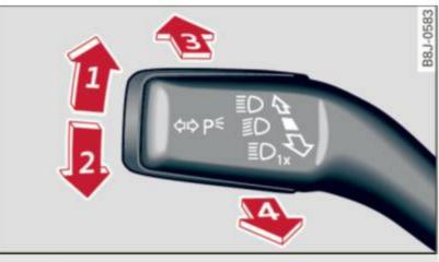
Fig. 48 Turn signal and high beam lever
