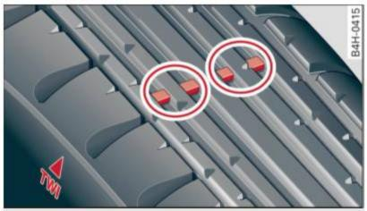
Fig. 169 Tire tread: tread wear indicators (TWI)
