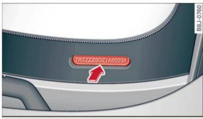
Fig. 201 Vehicle Identification Number (VIN) plate: location on driver's side dash panel
