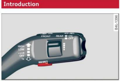
Fig. 12 Wiper lever: Controls for the menu display
