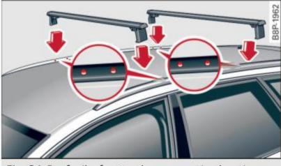
Fig. 84 Roof rails: front and rear mounting locations
