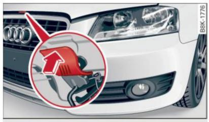
Fig. 156 Engine hood release lever
