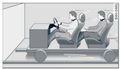
Fig. 121 Unbelted occupants in a vehicle heading for a wall
