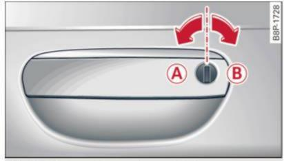
Fig. 30 Key turns for opening and closing.
