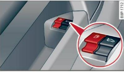
Fig. 152 Driver's door: Unlocking fuel filler flap
