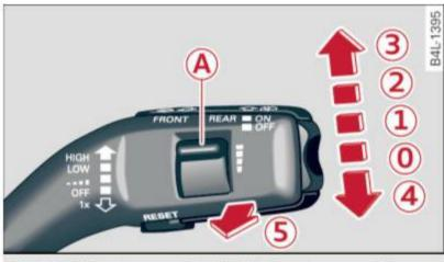
Fig. 57 Wiper lever: windshield wiper lever positions
