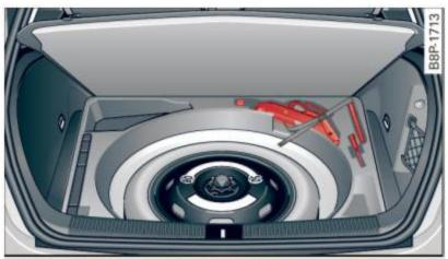
Fig. 179 Vehicle tool kit and jack
