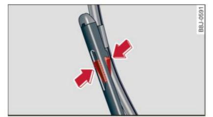
Fig. 59 Unlatching wiper blades
