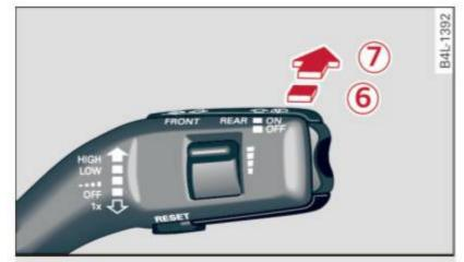
Fig. 58 Wiper lever: activating the rear window wiper and washer
