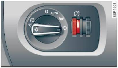
Fig. 46 Instrument panel illumination
