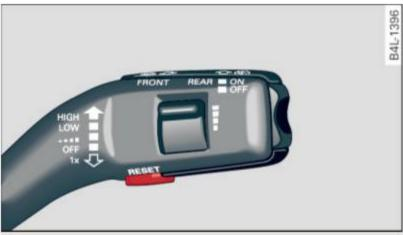
Fig. 7 Wiper lever: controls for the menu display
