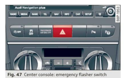
Press the switch ▲ ⇒ fig. 47, to switch the emergency flasher on or off.
