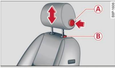
Fig. 69 Driver's seat head restraint: adjusting the height
