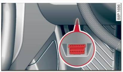
Fig. 9 Location of Data Link Connector (DLC)
