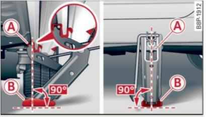
Fig. 186 Close-up: proper positioning of lifting jack
