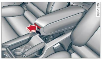
Fig. 72 Between the front seats: armrest folded down
