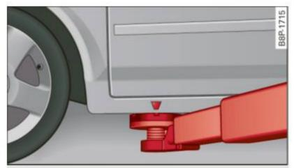
Fig. 199 Front lifting point
