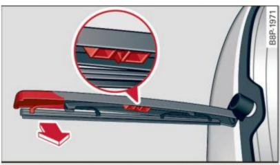
Fig. 61 Installing/removing wiper blade
