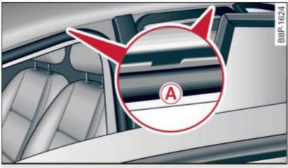
Fig. 83 Attachment points for roof rack
