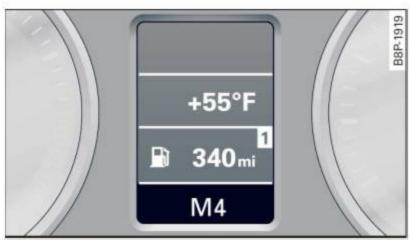
Fig. 113 Display: Manual shifting (tiptronic)
