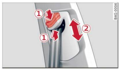
Fig. 130 Safety belt height adjustment for the front seats – loop-around fittings
