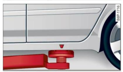
Fig. 200 Rear lifting point
