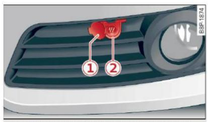
Fig. 100 In the left front bumper: engine preheater connection socket
