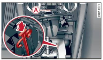
**Fig. 116** Selector lever: emergency release from the Park position
