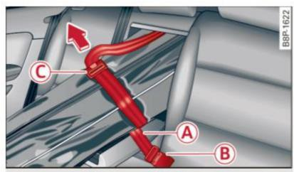
Fig. 82 Securing the ski sack at the center rear seat belt buckle
