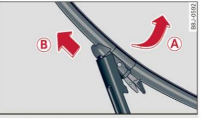
Fig. 60 Removing wiper blades
