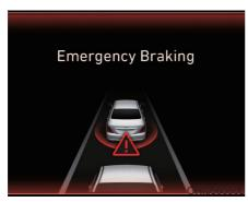
This warning message appears on the LCD display and the head up display (if equipped) with a warning chime. Additionally, some vehicle system intervention occurs by the engine management system to help decelerate the vehicle.
