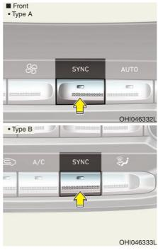
Adjusting the driver and passenger side temperature and air flow direction individually
