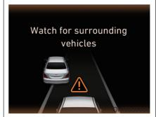
If the vehicle ahead (vehicle speed: less than 30km/h) disappears to the next lane, the warning chime will sound and a message "Watch for surrounding vehicles" will appear. Adjust your vehicle speed for vehicles or objects that can suddenly appear in front of you by depressing the brake pedal.
