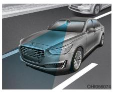
The Lane Keeping Assist System detects lane markers on the road, and assists the driver's steering to help keep the vehicle between lanes. When the system detects the vehicle straying from its lane, it alerts the driver with a visual and steering wheel vibration warning, while applying a slight counter-steering torque, trying to prevent the vehicle from moving out of its lane.
