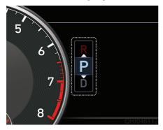
The pop-up that indicates the current gear position is displayed in the cluster for about 2 seconds when shifting into other positions (P/R/N/D).
