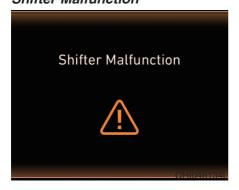
The warning message appears on the LCD display, when the transmission or the shift lever does not properly operate in the P (Park) position. In this case, we recommend you to immediately have the vehicle inspected by an authorized retailer of Genesis Branded products.
