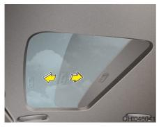
The sunshade will automatically open with the glass panel when the glass panel moves. Close it manually if you want it closed.
