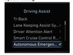
The driver can activate the AEB by placing the Engine Start/Stop button to the ON position and by selecting 'User Settings → Driving Assist → Autonomous Emergency Braking'. The AEB deactivates, when the driver cancels the system setting.
