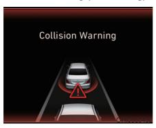
This warning message appears on the LCD display and the head up display (if equipped) with a warning chime.
