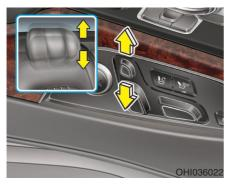
Adjusting the height up and down (power, if equipped)
