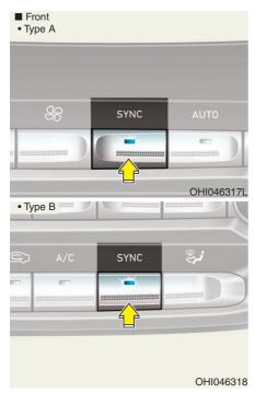
Adjusting the driver and passenger side temperature and air flow direction equally
