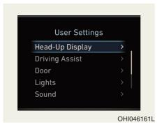
In this mode, you can change the setting of the instrument cluster, doors, lamps, etc.
