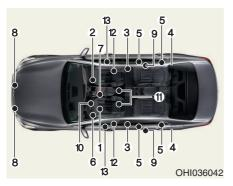
The SRS consists of the following components:
