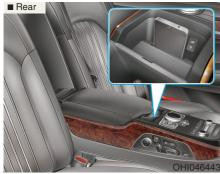
There are two wireless cellular phone charging systems both inside the front console and inside the rear console. Those are available when all doors are closed, and when the Engine Start/Stop button is in the ACC/ON position.
