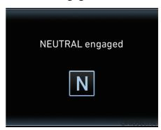
The message appears on the LCD display, when the N (Neutral) position is engaged.
