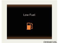
This warning message is displayed if the fuel tank is almost out of fuel.
