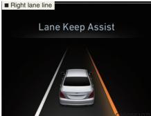
If all the conditions to activate LKAS is not satisfied, the system will convert to LDWS (Lane Departure Warning System) and warn the driver only when the driver crosses the lane lines.
