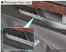
The Seat Position Memory System is provided to store and recall the following memory settings with a simple button operation.
