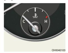
This gauge indicates the temperature of the engine coolant when the Engine Start/Stop button is in the ON position.
