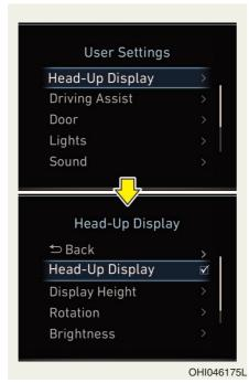
To activate the head-up display, select "Head-Up Display" on the "User Settings mode" in the cluster. If you do not select "Head-Up Display", the head-up display will be deactivated.
