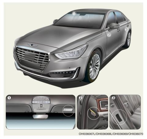
Air bag warning labels are attached to alert the driver and passengers of potential risks of the air bag system.
