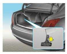
If the fuel filler door does not open using the remote fuel filler door release button, you can open it manually. Pull the handle of the release located on the left side of the luggage compartment outward slightly.
