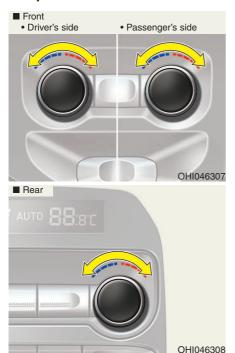
The temperature will increase to the maximum (HI) by turning the knob to the right. The temperature will decrease to the minimum (Lo) by turning the knob to the left. The temperature will increase or decrease by 0.5°C (1°F). When set to the lowest temperature setting, the air conditioning will operate continuously.
