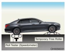
An AWD vehicle should not be tested on a 2WD roll tester. If a 2WD roll tester must be used, perform the following procedure:
