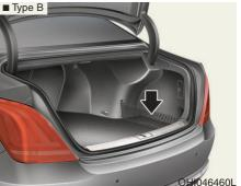
To keep items from shifting in the trunk, you can use the holders located in the trunk to attach the luggage net.
