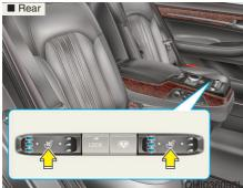
The seat coolers are provided to cool the seats by blowing air through small vent holes on the surface of the seat cushions and seatbacks.
