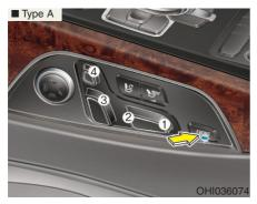
Press the FRONT button. When the FRONT indicator illuminates, a rear seat passenger can control the front passenger's seat position back and forth (1), seat cushion height (2), seat-back angle (3), and headrest position (4).
