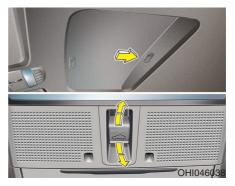
Pressing the sunroof control lever backward or forward momentarily to the second detent position completely opens or closes the sunroof even when the switch is released. To stop the sunroof at the desired position while the sunroof is in operation, press the sunroof control lever backward or forward and release the switch.
