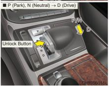
This is the normal driving position. The transmission will automatically shift through a 8-gear sequence, providing the best fuel economy and power.
