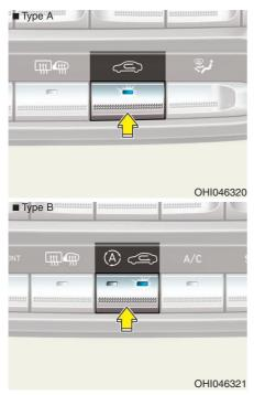
This is used to select the outside (fresh) air position or recirculated air position.
