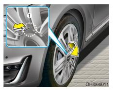
Insert the tool (1) into the hole and pull out the wheel cover. (if equipped)
