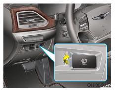
To apply the EPB (Electronic Parking Brake):
