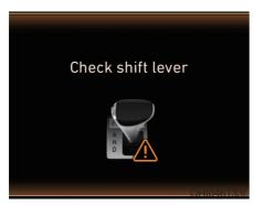
The warning message appears on the LCD display, when there is a malfunction with one of the key transmission shifter components.
