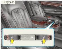
While the engine is running, push the switch to warm the seat.
