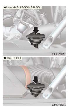
Check the condition and connections of all cooling system hoses and heater hoses. Replace any swollen or deteriorated hoses.
