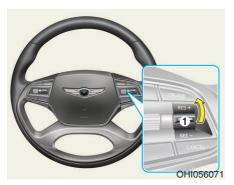
Push the toggle switch (1) up (RES+). If the vehicle speed is over 30 km/h (20 mph), the vehicle will resume the preset speed.
