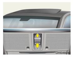
To open the sunroof, push the sunroof control lever upward to the second detent. The sunroof will tilt all the way open.
