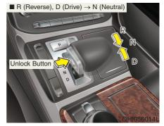
The wheels and transmission are not engaged.
