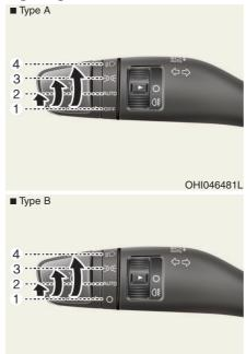
To operate the lights, turn the knob at the end of the control lever to one of the following positions:
