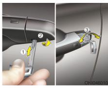
First, remove the cover (1~2), and then turn the key toward the rear of the vehicle to unlock and toward the front of the vehicle to lock (3).
