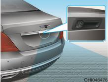
The Rear View Camera will activate when the engine is running and the shift lever is in the R (Reverse) position.
