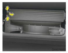
3. Remove the climate control air filter case while pressing the lock on the left side of the cover.
