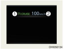
The indicator is displayed when the cruise control system is enabled (1) and the cruise control speed is set (2).
