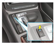
The Around View Monitoring (AVM) system is a driving assist system. It guides the driver to safely park the vehicle by providing an around view image on the screen.
