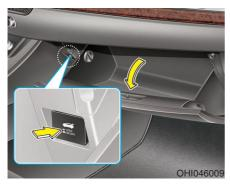
When the trunk lid control button is in the UNLOCK (button not pressed) position, the power trunk can be controlled with the power trunk main control button, power trunk open, close button, and the smart key.
