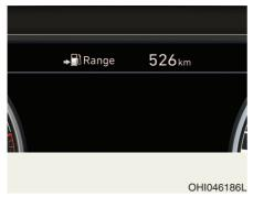
The range is the estimated distance the vehicle can be driven with the remaining fuel in the fuel tank.
