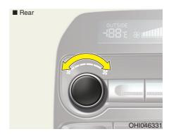
Turn the knob to the right (\$\square\$) to increase the fan speed and airflow. Turn the knob to the left (\$\square\$) to decrease fan speed and airflow.
