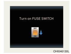
This warning message is displayed if the fuse switch located on the fuse box under the steering wheel is OFF. If this message is displayed, turn the fuse switch on.
