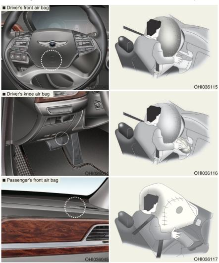
The purpose of the SRS is to provide the vehicle's driver and front passengers with additional protection than that offered by the seat belt system alone in case of a frontal impact of sufficient severity.
