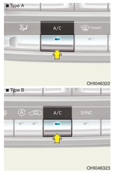
Push the A/C button to turn the air conditioning system on (indicator light will illuminate).
