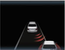
The Smart Blind Spot Detection System may apply braking power, when an approaching vehicle is detected within a certain distance next to/behind your vehicle.
