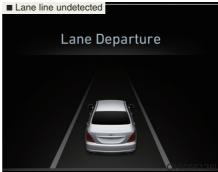
If your vehicle speed exceeds 60 km/h (38 mph) and the LDWS button is ON, the system is enabled. If your vehicle departs from the projected lane in front of you, the LDWS operates as follows:
