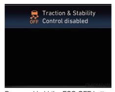
Press and hold the ESC OFF button continuously for more than 3 seconds. The ESC OFF indicator light and message (Vehicles equipped with the AEB system, the AEB warning light (ﷺ) illuminates. For more information, refer to "Autonomous Emergency Braking (AEB)" in this chapter.) illuminates and a warning chime sounds. In this state, both the traction control function of ESC (engine management) and the brake control function of ESC (braking management) are disabled.
