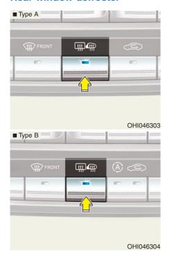
The defroster heats the window to remove frost, fog and thin ice from the interior and exterior of the rear window, while engine is running.
