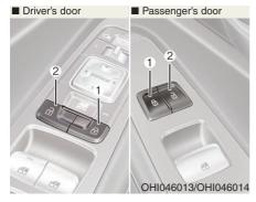
When pressing the  $( \widehat{\underline{}_{1}} )$  portion (1) of the switch, all vehicle doors will lock. When pressing the  $( \widehat{\underline{}_{1}} )$  portion (2) of the switch, all vehicle doors will unlock. If the smart key is in the vehicle and any door is opened, the doors will not lock even though the lock button (1) of the central door lock switch is pressed.
