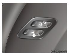
Additional switches are provided to move the front passenger seat forward and backward (1), and adjust the seatback angle (2) from the rear seats.
