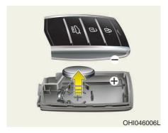
Battery Type: CR2032 To replace the battery:
