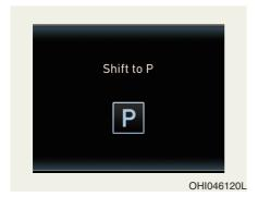
This warning message is displayed if you try to turn off the engine without the shift lever in P (Park) position.
