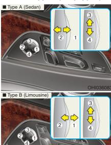
The lumbar support can be adjusted by pressing the lumbar support switch. Press the front portion of the switch (1) to increase support or the rear portion of the switch (2) to decrease support.
