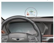
The Head-Up Display is a transparent display which projects a shadow of information of the instrument cluster and navigation on the windshield glass.
