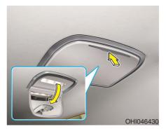
Press the vanity mirror on the vehicle ceiling. Then, it automatically turns ON the rear vanity mirror lamp while opening the cover.
