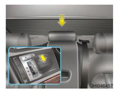
The rear curtain will be lowered automatically when you shift the shift lever into R (Reverse) and raised automatically when you shift the shift lever from R (Reverse) into P (Park).
