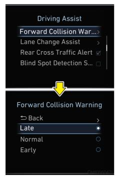
The driver can select the initial warning activation time in the User Settings in the LCD display. The options for the initial Forward Collision Warning includes the following:
