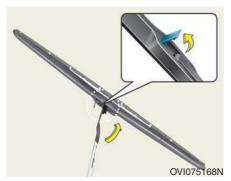
2. Open the wiper blade clip and slightly rotate the wiper blade assembly to expose the plastic locking clip.
