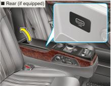
You can use an AUX port to connect audio devices and USB port to plug in USB and also in iPod® port. (Rear multimedia jack: USB only)
