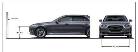
H1: Height between the head lamp bulb center and ground (Low beam)
