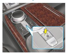
When the ignition switch is in the ON position or when the engine is running, press the heated steering wheel button to warm the steering wheel. The indicator on the button will illuminate.
