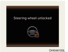
This warning message is displayed if the steering wheel does not lock while the Engine Start/Stop button changes to the OFF position.
