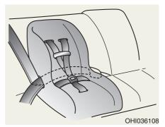
Installing a child restraint with a lap/shoulder belt
