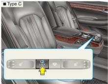
You can activate or deactivate the rear seat control by using the LOCK button on the rear armrest.
