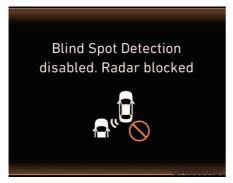
Blind Spot Detection disabled. Radar blocked
