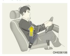
The purpose of the pre-active seat belt is to tighten the seat belt when a collision is sensed, during emergency braking, or when a loss of control is sensed.
