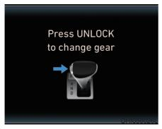
The warning message appears on the LCD display, when the [UNLOCK] button is not pressed while shifting the gear. We recommend you press the [UNLOCK] button and then shift the gear.
