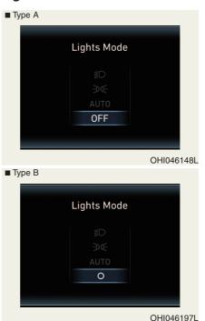
This indicator displays which exterior light is selected using the lighting control.
