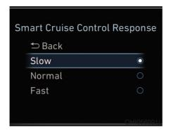
The sensitivity of vehicle speed when following the front vehicle to maintain the set distance can be adjusted. Go to the 'User Settings → Driving Assist → Smart Cruise Control Response → Slow/Normal/Fast' on the LCD display. You may select one of the three stages you prefer.
