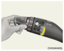
To turn on the rear fog lamp: Position the light switch in the headlamp position, and then turn the light switch (1) to the rear fog lamp position.
