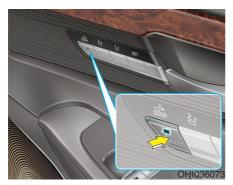
A front seat moves slightly rearward, when a passenger opens a front door with the DOOR indicator illuminated.
