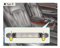
A rear seat passenger can control the front passenger's seat position back and forth (1) and seatback angle (2).
