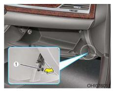
1. Open the glove box and remove the support pin (1).
