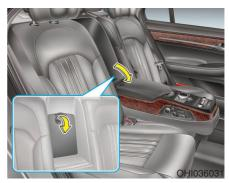
Additional cargo space is provided to accommodate long/narrow cargo (skis, poles, etc.) not able to fit properly in the trunk when closed.
