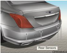
The Parking Assist System assists the driver during movement of the vehicle by chiming if any object is sensed within approximately 100 cm (40 in) in front and 120 cm (47 in) behind the vehicle.
