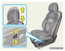
Adjusting the height up and down Push the control switch up to raise or down to lower the headrest. Release the switch once the headrest reaches the desired position.
