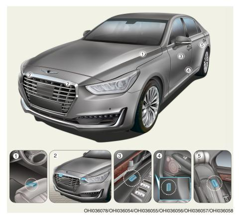
1. SRS control module /Rollover sensor
