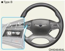
The steering wheel audio control switch installed for your convenience.
