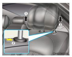
Adjusting the height up and down (manual, if equipped)
