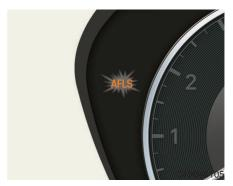
If the AFLS malfunction indicator comes on, the AFLS is not working properly.
