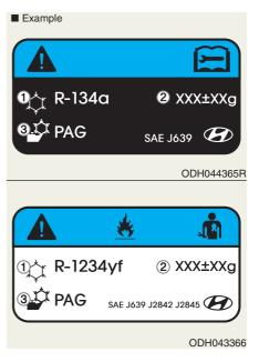
The actual Air Conditioning refrigerant label in the vehicle may differ from the illustration.
