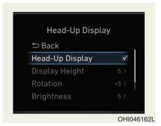
The driver can set the Head-Up Display menus by using the Users Settings mode on the LCD display. For more information, refer to "LCD Display" in this chapter.
