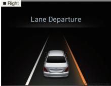
A visual warning appears on the cluster LCD display. Either the left lane line or the right lane line in the cluster LCD display will blink depending on which direction the vehicle is veering. If you leave the lane, the steering wheel will vibrate.
