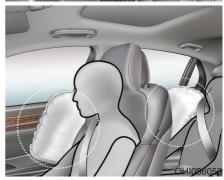
Your vehicle is equipped with a side air bag in each front and outboard rear seat. The purpose of the air bag is to provide the vehicle's driver and/or the front and outboard rear passenger with additional protection than that offered by the seat belt alone.
