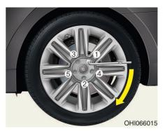
14. Use the wheel lug nut wrench to tighten the lug nuts in the order shown. Double-check each lug nut until they are tight. After changing tires, we recommend that an authorized retailer of Genesis Branded products tighten the lug nuts to their proper torque as soon as possible. The wheel lug nut should be tightened to 11~13 kgf·m (79~94 lbf·ft).
