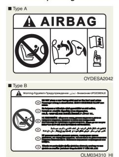
Never install a child restraint in the front passenger's seat. An inflating air bag can forcefully strike a child or restraint resulting in serious or fatal injury.
