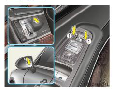
When you move the shift lever to the R (Reverse) position, the outside rearview mirror(s) will rotate downwards to aid with driving in reverse.
