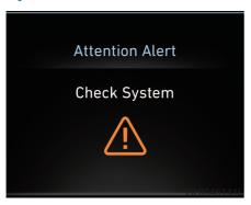
When the "Check System" warning message appears, the system is not working properly. In this case, we recommend you to have the vehicle inspected by an authorized retailer of Genesis Branded products.
