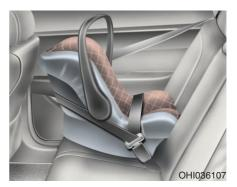
A rear-facing child restraint provides restraint with the seating surface against the back of the child. The harness system holds the child in place, and in an accident, acts to keep the child positioned in the restraint and reduce the stress to the fragile neck and spinal cord.
