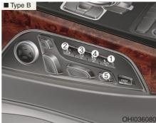
Press the switch (1) to adjust both the front passenger's seat and the rear seat, as follows.
