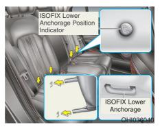
The ISOFIX lower anchorages position indicator symbols are located on the left and right rear seat backs to identify the position of the ISOFIX lower anchorages in your vehicle (see arrows in illustration).
