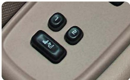
**Memory Seats** (Optional): Memory seat controls are located on the driver door. They program and recall driver seat position and outside mirror settings for up to two drivers.
