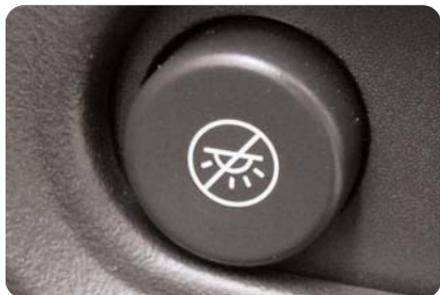
To disable the dome lamps when a door is open, press the dome lamp override button. The button is located below the exterior lamps knob. The button also disables entry lighting until it is pushed again or the remote keyless entry transmitter is used to unlock the vehicle.
