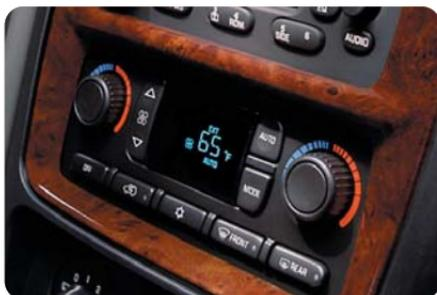
Your vehicle may be equipped with a climate control system that automatically maintains the desired temperature individually for the driver and front seat passenger. Independent rear seat fan and air distribution controls are also included for increased rear-passenger comfort. A memory feature for up to two drivers is also included in this optional system.
