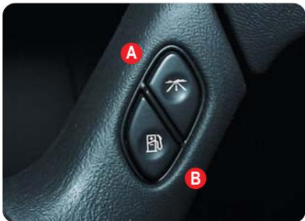
**A. Trip Information Button:** Press this button to access each of the odometer, TRIP A, TRIP B and TIMER functions.
