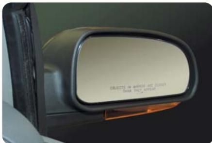
**Power (Optional):** Twist the control knob toward the mirror you want to adjust, move the knob in the direction you want the mirror to go, and when both mirrors have been adjusted, twist the control knob to the center position.
