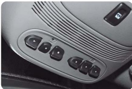
This programmable transmitter can store three frequencies for items such as a garage door opener, entry door lock or security system. With the ignition OFF, program the transmitter as follows:
