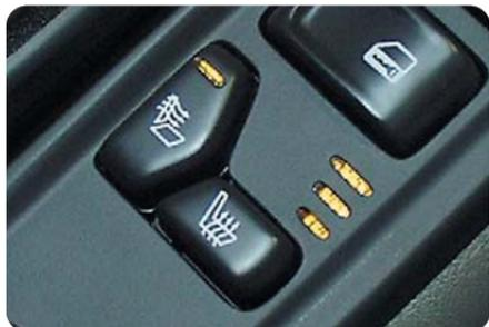
**Heated Seats** (Optional): The heated seat controls are located on the front door armrests. Controls can be set to heat the seatback only or the seatback and the seat cushion. The three lights next to the controls indicate LO, MED or HI settings. Push the vertical switch to activate heat for the seatback only. Push the horizontal switch to heat the whole seat. The engine must be running for the heated seat feature to work.
