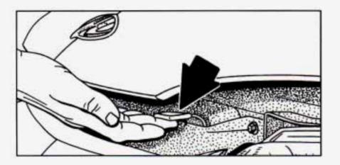
Then go to the front of the vehicle and pull up on the underhood release.
