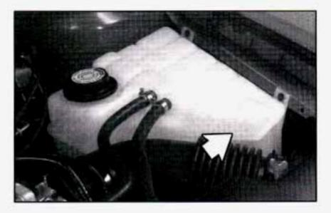
If the message LOW ENGINE COOLANT is displayed on your message center, it means you're low on engine coolant.
