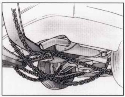
Position the lower-sling crossbar just ahead of the front edge of the rear bumper.
