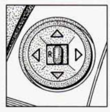
The controls on the far left of the instrument panel control both outside rearview mirrors. Move the center switch to the left to select the driver's side rearview mirror, or to the right to select the passenger's side rearview mirror. Then press the arrows to adjust each mirror so that you can just see the side of your vehicle when you are sitting in a comfortable driving position.
