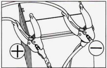
Don't let the other end touch metal. Connect it to the positive (+) terminal of the good battery. Use a remote positive (+) terminal if the vehicle has one.
