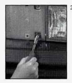
Use a 10 mm socket to remove the four bolts. There are two bolts on each side of the cover.
