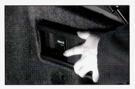
Close the door by sliding it all the way to the left. If the door is left partially open, the changer will not operate and an error will occur. When the door is closed, the changer will begin checking for discs in the magazine. This will continue for up to two minutes depending on the number of discs loaded.
