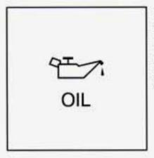
If the CHECK OIL LEVEL message or the oil warning light on the instrument panel comes on, it means you need to check your engine oil level right away.
