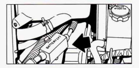
Open the hoods and locate the other vehicle's battery and the Aurora's remote positive (+) jump starting terminal in the box on the passenger side of the engine compartment. (Your Aurora's battery isn't under the hood.)
