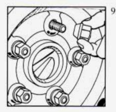
Replace the wheel nuts with the rounded end of the nuts toward the wheel. Tighten each nut by hand until the wheel is held against the hub.
