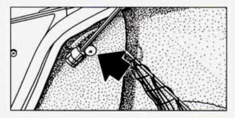
In the trunk, remove the convenience net from the hooks. Next remove the plastic screws holding the carpeting in place and pull back the carpeting.
