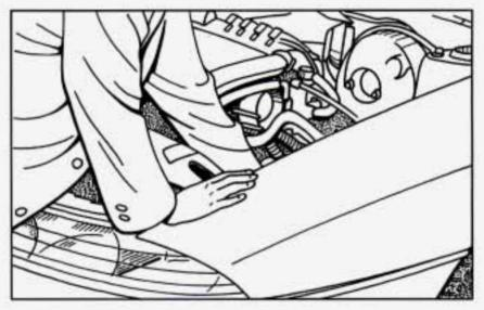
Twist the bulb assembly one-sixth of a turn counterclockwise and pull out the bulb assembly.
