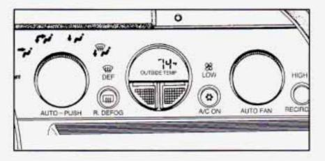
Your Aurora is equipped with a Dual Zone Automatic Electronic Climate Control System. You can use the automatic setting or override the automatic setting by using the manual controls. Your vehicle also has the flow-through ventilation system described later in this section. If the display ever starts flashing after the automatic electronic climate control system is started, there is a problem with the electronic climate control system and you should see your dealer for service.
