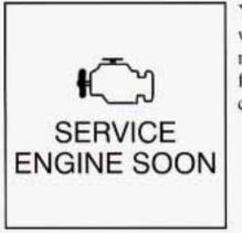
Your Aurora is equipped with a computer which monitors operation of the fuel, ignition and emission control systems.
