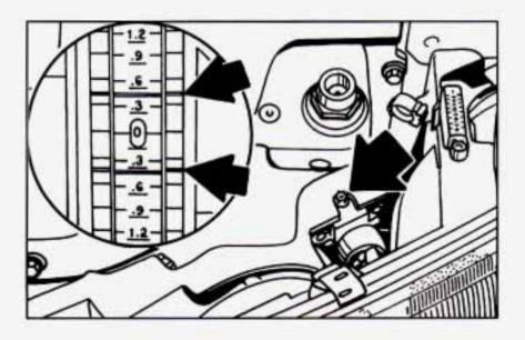
Check the vertical aim for each headlamp. The vehicle must be on a level surface. Turn the vertical aiming screw until the bubble in the level is centered at 0 (zero).
