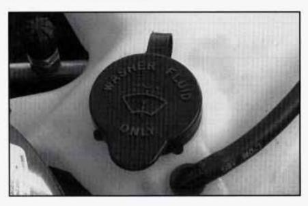
There are two windshield washer fluid tanks. The upper tank (shown above) will empty first. When the lower tank contains 0.5 quarts (0.5 liters) or less, the message LOW WASHER FLUID will be displayed on the Driver Information Center. Open the cap labeled WASHER FLUID ONLY. Add washer fluid until the tank is full.
