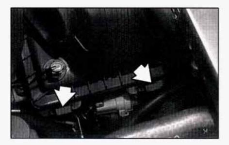
Unsnap the two clamps by pushing down on the top of the air cleaner cover and pushing in on the clamps toward the center of the cover. Then remove the cover.
