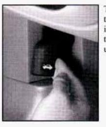
To open the hood, first pull the hood release handle inside the vehicle, located to the left of the steering wheel under the instrument panel.
