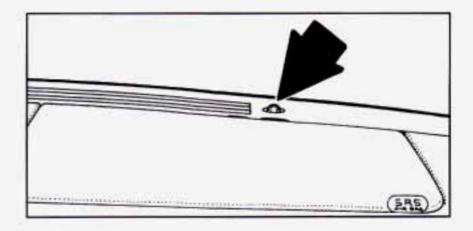
Your automatic electronic climate control system has two sun sensors located on the top of the instrument panel that detect direct sunlight. To keep you and your passengers comfortable, the system may supply cooler air to the side toward the sun. Be careful not to put anything over these sun sensors. The automatic electronic climate control system may not operate correctly if these sensors are covered.
