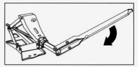
Turn the wheel wrench clockwise by hand to raise the jack head a few inches.
