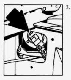
Unclip the bulb assembly from the wiring harness and replace the bulb assembly.
