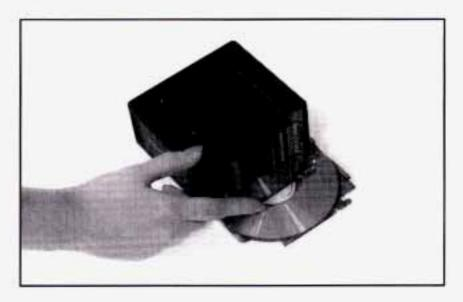
You must first load the magazine with discs before you can play a compact disc. Each of the 12 trays holds one disc. Press the button on the back of the magazine and pull gently on one of the trays. Load the trays from bottom to top, placing a disc on the tray with the label side down. If you load a disc label side up, the disc will not play and an error will occur. Gently push the tray back into the magazine slot. Repeat this procedure for loading up to 12 discs in the magazine.
