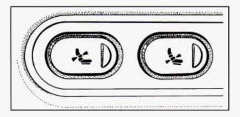
The power lumbar controls are located on the driver's and passenger's door panels.
