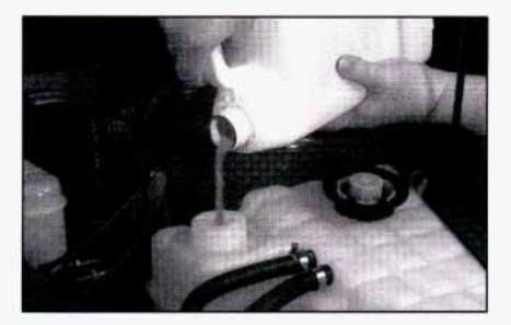
Then fill the coolant surge tank with the proper mix, up to FULL COLD.
