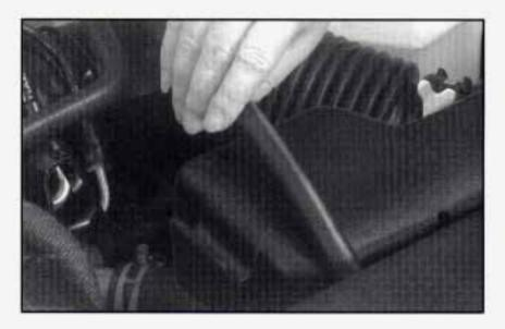
1. Remove hose from resonator channel.
