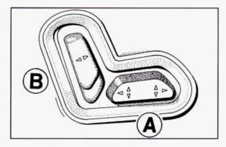
The power seat controls are located on the driver's and passenger's door panels. Horizontal Control (A): Raise the front of the seat by raising the forward edge of the button. Lower the front of the seat by lowering the forward edge of the button. Move the seat forward by moving the whole button toward the front of the vehicle.
