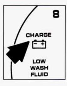
The CHARGE light will come on when you turn on the ignition, but the engine is not running, as a check to show you it is working.
