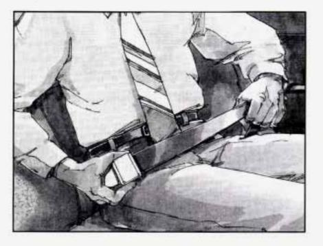
When you sit in the center seating position, you have a lap safety belt, which has no retractor. To make the belt longer, tilt the latch plate and pull it along the belt. To make the belt shorter, pull its free end as shown until the belt is snug.
