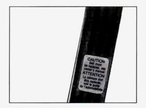
If belts are cut or damaged, replace them. Collision damage also may mean you will need to have safety belt or seat parts repaired or replaced. New parts and repairs may be necessary even if the belt wasn't being used at the time of the collision.
