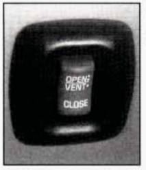
Open the sunshade by hand when using the vent position. Press the rear of the switch again to open the glass panel and the sunshade. Press the switch again to stop the panel in any position.
