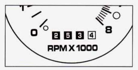
The trip odometer can tell you how far you have driven since you last reset it. To reset the trip odometer to zero, press the knob to the right of the gage.
