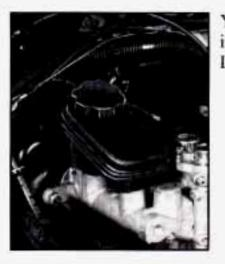
Your brake master cylinder is here. It is filled with DOT-3 brake fluid.
