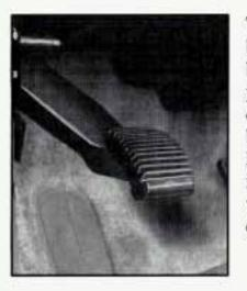
To set the parking brake hold the regular brake pedal down with your right foot. Push down the parking brake pedal with your left foot. If the ignition is on, the brake system warning light will come on.
