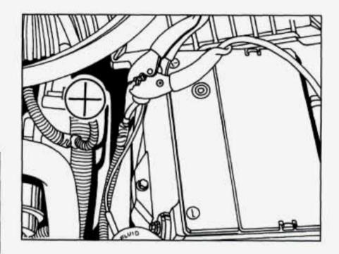
Connect the red positive (+) cable to the positive (+) terminal of the vehicle with the dead battery. Use a remote positive (+) terminal if the vehicle has one.
