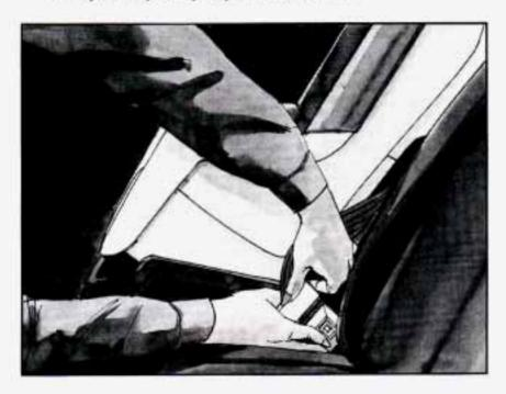
To tighten the belt, pull up on the shoulder belt while you push down on the child restraint.
