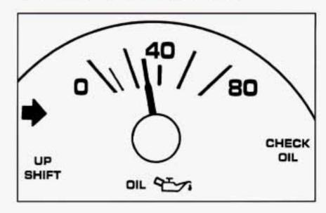
The oil pressure gage shows the engine oil pressure in psi (pounds per square inch) when the engine is running. Canadian vehicles indicate pressure in kPa. Oil pressure may vary with engine speed, outside temperature and oil viscosity, but readings above the red warning zone indicate the normal operating range.
