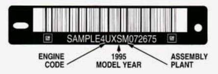
This is the legal identifier for your Oldsmobile. It appears on a plate in the front corner of the instrument panel, on the driver's side. You can see it if you look through the windshield from outside your vehicle. The VIN also appears on the Vehicle Certification and Service Parts labels and the certificates of title and registration.
