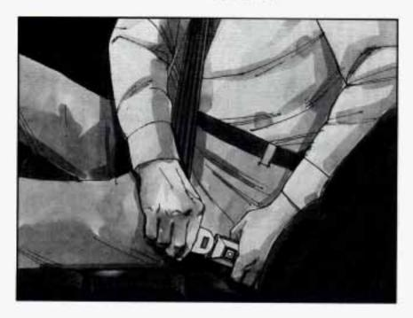
Pick up the latch plate and pull the belt across you. Don't let it get twisted. 2. Push the latch plate into the buckle until it clicks.
