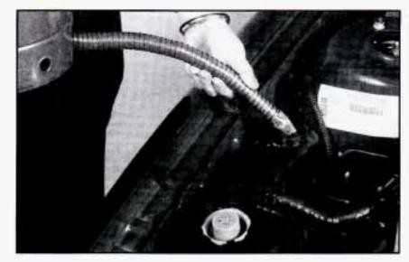
Then fill the coolant surge tank with the proper mix, up to FULL COLD, or just above the small cylinder at the base of the opening.
