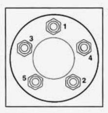
Tighten the wheel nuts firmly in a criss-cross sequence, as shown. Don't try to put a wheel cover on your compact spare tire. It won't fit. Store the wheel cover and wheel nut caps in the trunk until you have the flat tire repaired or replaced.
