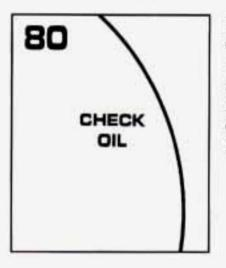
Your engine is equipped with an oil level monitoring system. When the ignition key is turned on, the CHECK OIL light will briefly flash.
