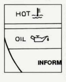
If you have a low engine oil pressure problem, this light will stay on after you start your engine, or come on when you are driving. This indicates that your engine is not receiving enough oil. The engine could be low on oil, or could have some other oil problem. Have it fixed immediately.
