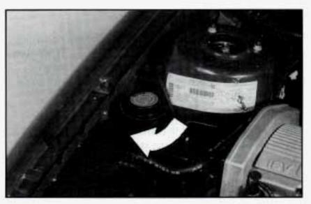
Then replace the pressure cap. Be sure the pressure cap is tight.
