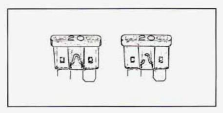
Look at the silver-colored band inside the fuse. If the band is broken or melted, replace the fuse. Be sure you replace a bad fuse with a new one of the correct size.
