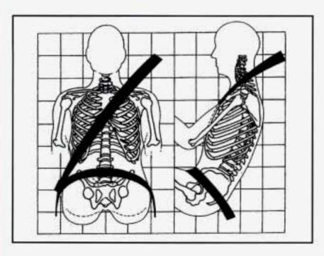
The lap belt should be worn as low on the hips as possible. In a crash, this applies force to the strong pelvic bones. And you'd be less likely to slide under the lap belt. If you slid under it, the belt would apply force at your abdomen. This could cause serious or even fatal injuries. The shoulder belt should go over the shoulder and across the chest. These parts of the body are best able to take belt restraining forces.
