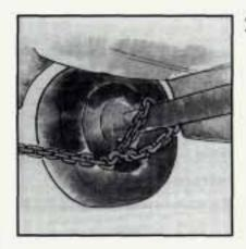
Attach a separate chain to each side of the axle inboard of the spring.
