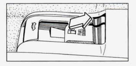
To open the fuel door, pull the fuel access handle on the floor by the driver's seat.
