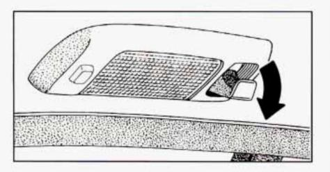
Push down on the tab marked with a hanger symbol to fold down the garment hook.
