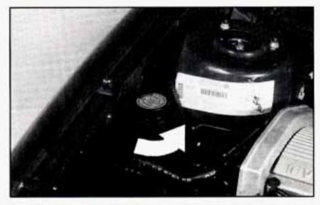
You can remove the coolant surge tank pressure cap when the cooling system, including the coolant surge tank pressure cap and upper radiator hose, is no longer hot. Turn the pressure cap slowly about one-quarter turn to the left and then stop. If you hear a hiss, wait for that to stop. A hiss means there is still some pressure left.
