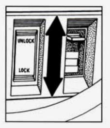
From the inside, to lock the door, slide the locking lever down.
