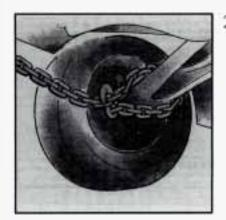
Attach a separate safety chain around the outboard end of each lower control arm.
