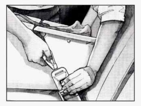
To make it tight, pull the belt while you push down on the child restraint. If the belt won't stay tight, switch it end for end.
