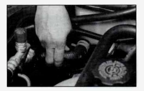
With the coolant surge tank pressure cap off, start the engine and let it run until you can feel the upper radiator hose getting hot. Watch out for the engine fan.
