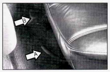
There are two levers at the front of the seat. The left lever adjusts the seat forward and back. The right lever adjusts the angle of the front of the seat.
