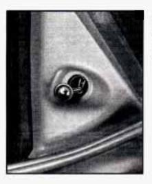
Adjust the driver side outside mirror with the control lever on the driver's door.
