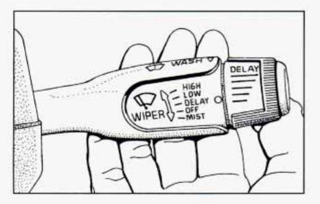
To wash your windshield, pull the stalk toward you until the washers begin. When you release the stalk the washers will stop, but the wipers will either stop or will resume the delay speed you were using before.
