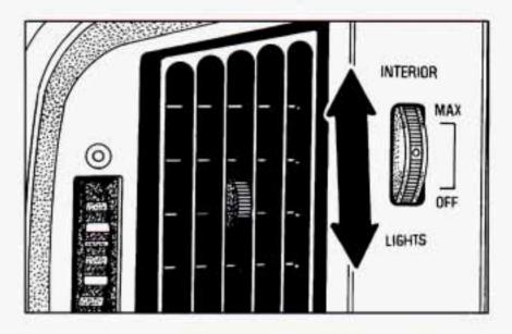
You can brighten or dim the instrument cluster lights by rotating the wheel. Rotate the wheel all the way down to turn off the instrument cluster lights and displays.
