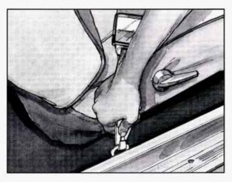
Push the spring on the hook near the door and remove the special belt.
