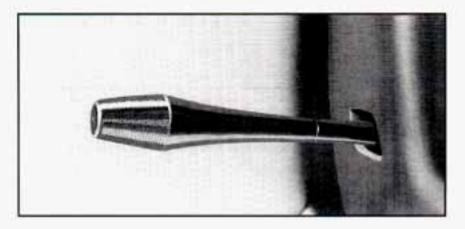
A tilt steering wheel allows you to adjust the steering wheel before you drive.
