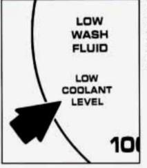
If this light comes on and stays on, the vehicle should promptly be pulled off the road and the coolant level checked.
