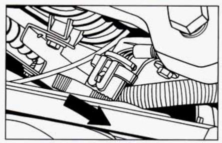
Twist the lock ring clockwise 1/6 turn and pull out the bulb assembly.
