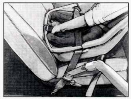
Push and pull the child restraint in different directions to be sure it is secure.
