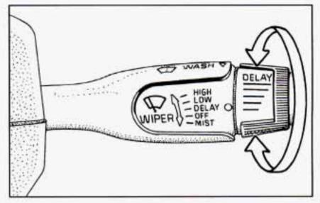
Move the stalk to DELAY, then rotate the inner band and choose the delay you want. Rotate the inner band up for shorter delay times between wiper cycles. Rotate the band down for a longer delay time between wiper cycles.
