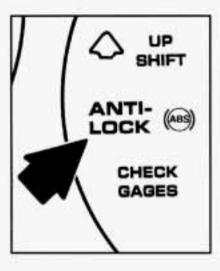
With the anti-lock brake system, this light will come on when you start your engine and it will stay on for three seconds. That's normal. If the light doesn't come on, have it fixed so it will be ready to warn you if there is a problem.
