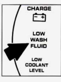
The LOW WASH FLUID light will come on when you turn on the ignition, and the fluid container is less than one-third full.
