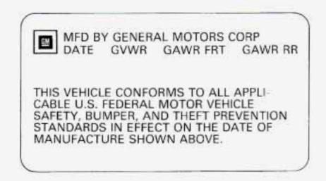
The other label is the Certification label, found on the rear edge of the driver's door. It tells you the gross weight capacity of your vehicle, called the GVWR (Gross Vehicle Weight Rating). The GVWR includes the weight of the vehicle, all occupants, fuel and cargo. Never exceed the GVWR for your vehicle, or the Gross Axle Weight Rating (GAWR) for either the front or rear axle. And, if you do have a heavy load, you should spread it out. Don't carry more than 132 lbs. (60 kg) in your trunk.
