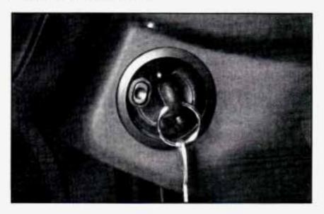
To remove the key, turn the key to the OFF position. While pressing the key release button in, turn the key to the LOCK position. Pull the key straight out.
