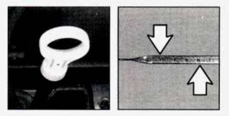
The engine oil dipstick handle is yellow. The dipstick handle for the 2.3L L-4 is located behind the engine. The dipstick for the 3.1L V-6 is located in front of the engine behind the fan.
