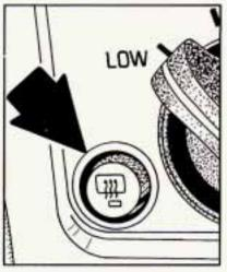
The rear window defogger uses a warming grid to remove fog from the rear window.
