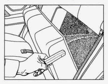
To fold down the rear seat, pull forward on the seat tab. Push the seatback up to return it to its original position. To make sure the seatback is secure, push it into a fully upright position.
