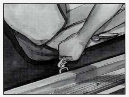
It will stay on the door, ready to be rebuckled for use by adults or older children. Put the belt's special latch plate into the vehicle's safety belt buckle.
