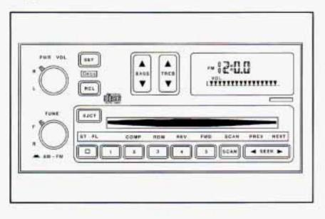
The digital display indicates information on time or radio station frequency, the AM or FM radio band, whether the station is in stereo, and other radio functions.
