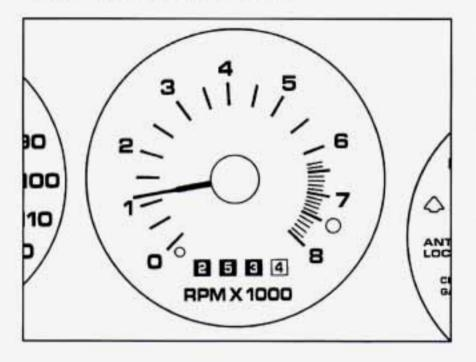
The tachometer shows your engine speed in revolutions per minute (rpm).
