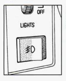
The button for your fog lamps is below the instrument panel intensity control.
