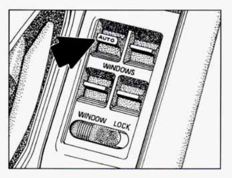
With power windows, switches on the driver's armrest control each of the windows when the ignition is on. In addition, each passenger door has a control switch for its own window.
