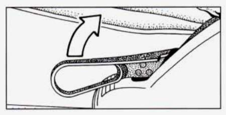
To adjust the seatback, lift the lever on the outer side of the seat and move the seatback where you want it. Release the lever to lock the seatback.
