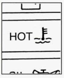
This light tells you that your engine coolant has overheated or your radiator cooling fan is not working.
