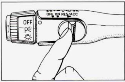
Suppose you set your cruise control at a desired speed and then you apply the brake or clutch pedal. This, of course, shuts off the cruise control. But you don't need to reset it. Once you're going about 25 mph (40 km/h) or more, you can move the cruise control switch from ON to RES/ACC (Resume/Accelerate) for about half a second.
