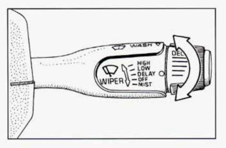
You control the windshield wipers by moving the stalk with the wiper symbol on it up or down.
