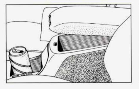
The front armrest opens into a storage area for cassette tapes, gloves, etc. To open it, push in the button and lift the front edge.
