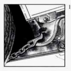
Attach T-hook chains into the slots in the bottom of the floor pan, just behind the front wheels, on both sides.
