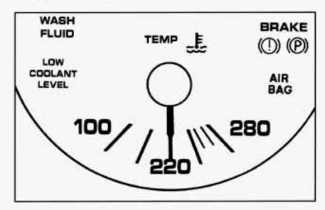
This gage shows the engine coolant temperature. If the gage pointer moves into the red area, your engine is too hot! It means that your engine coolant has overheated.
